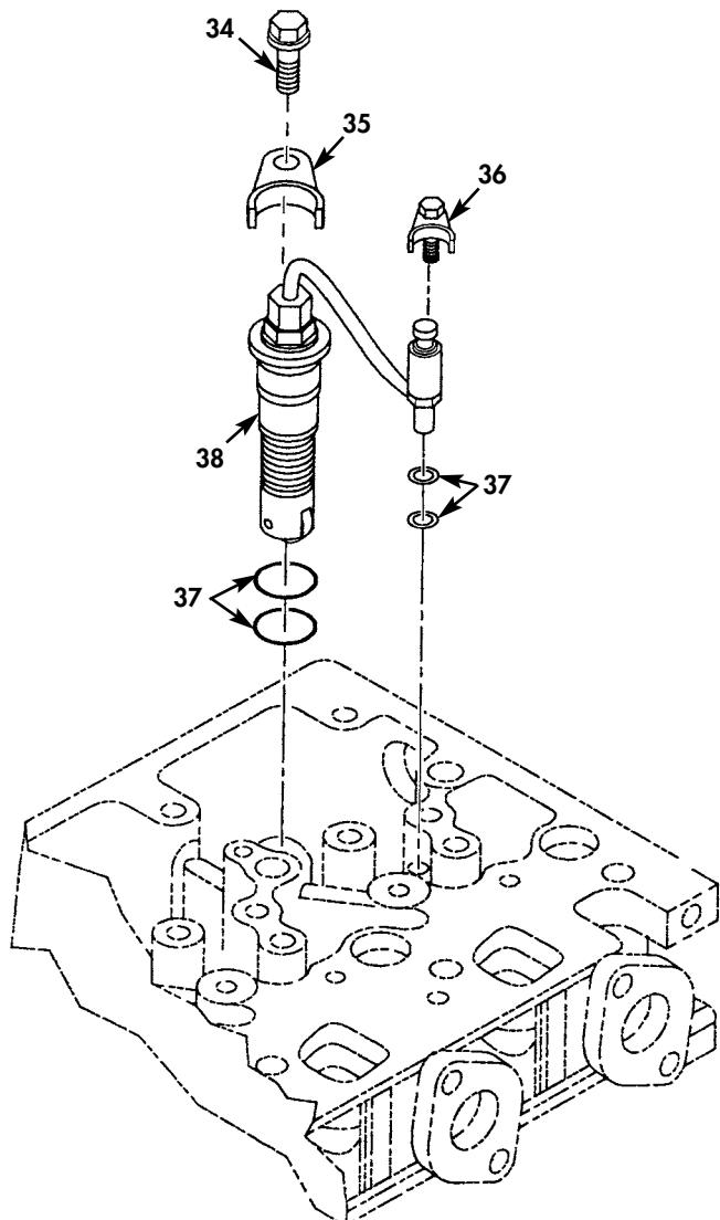
Figure 20. Fuel Injection System (Sheet 3 of 4).
