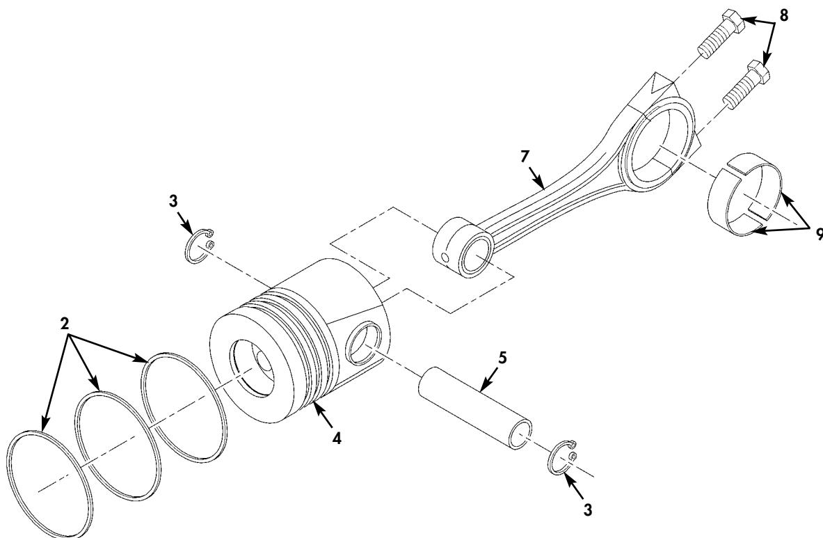
Figure 22. Pistons and Connecting Rods.
