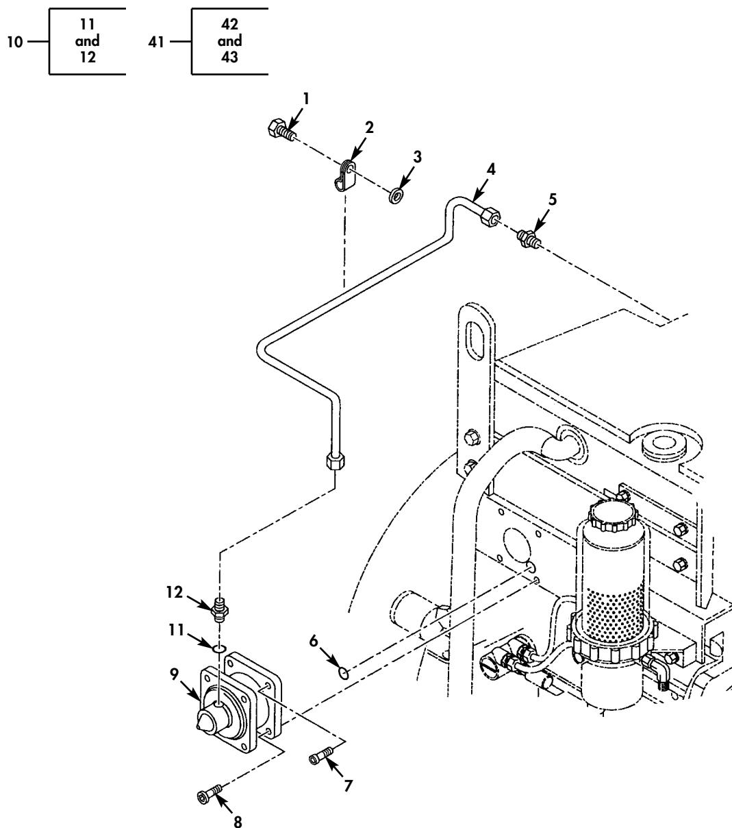
Figure 20. Fuel Injection System (Sheet 1 of 4).
