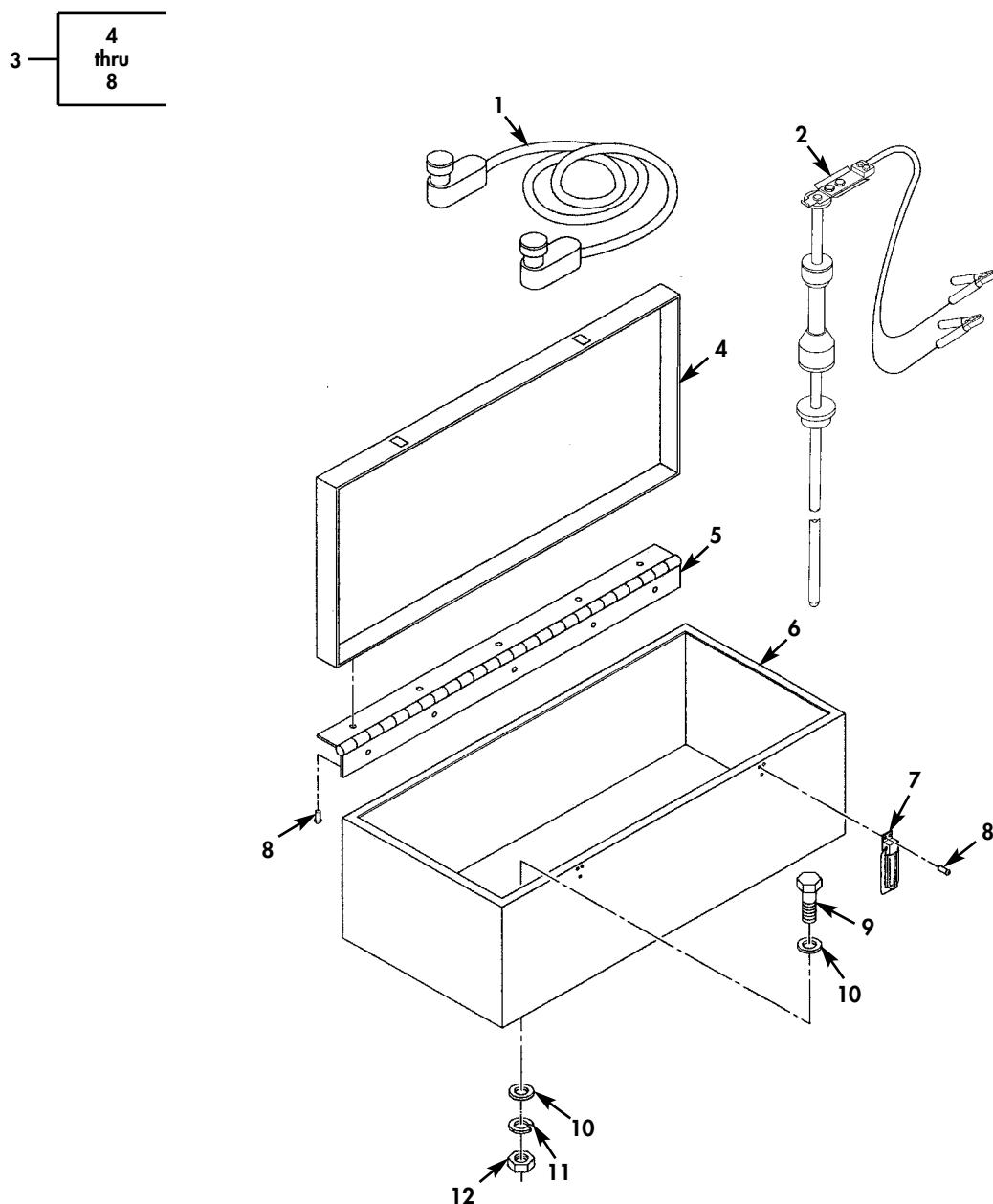
Figure 55. Toolbox, Intervehicular Cable, and Ground Rod Assembly.
