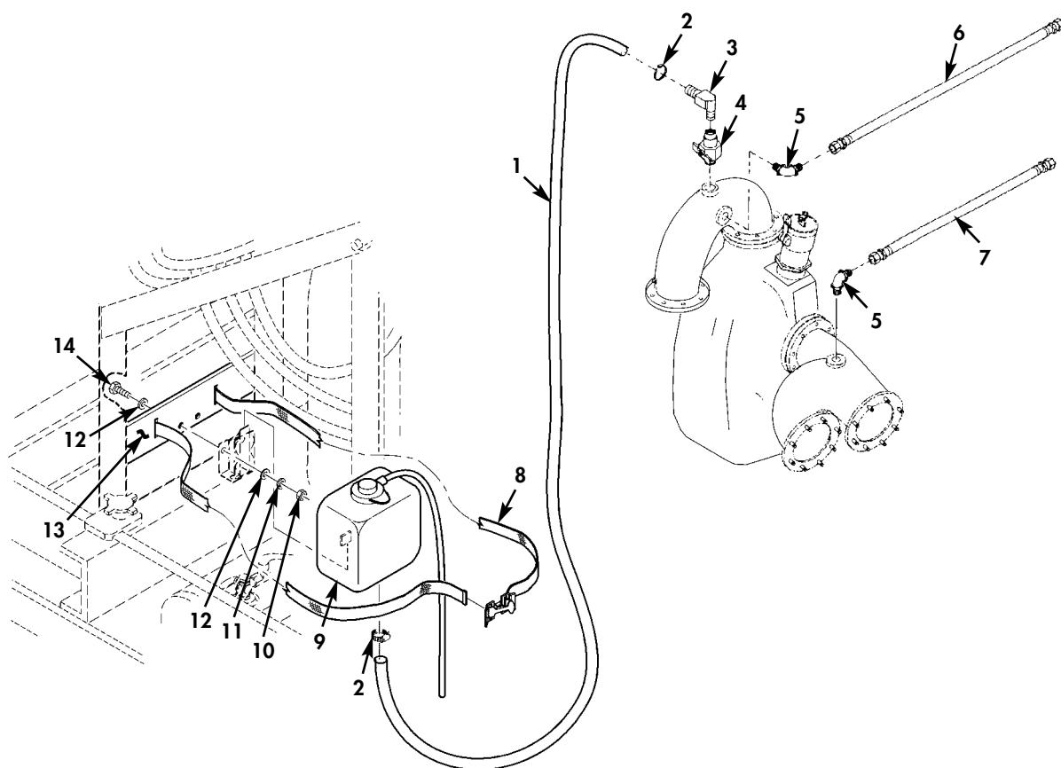
Figure 46. Transducer Hoses, Manifold Vent, and Overflow Bottle.
