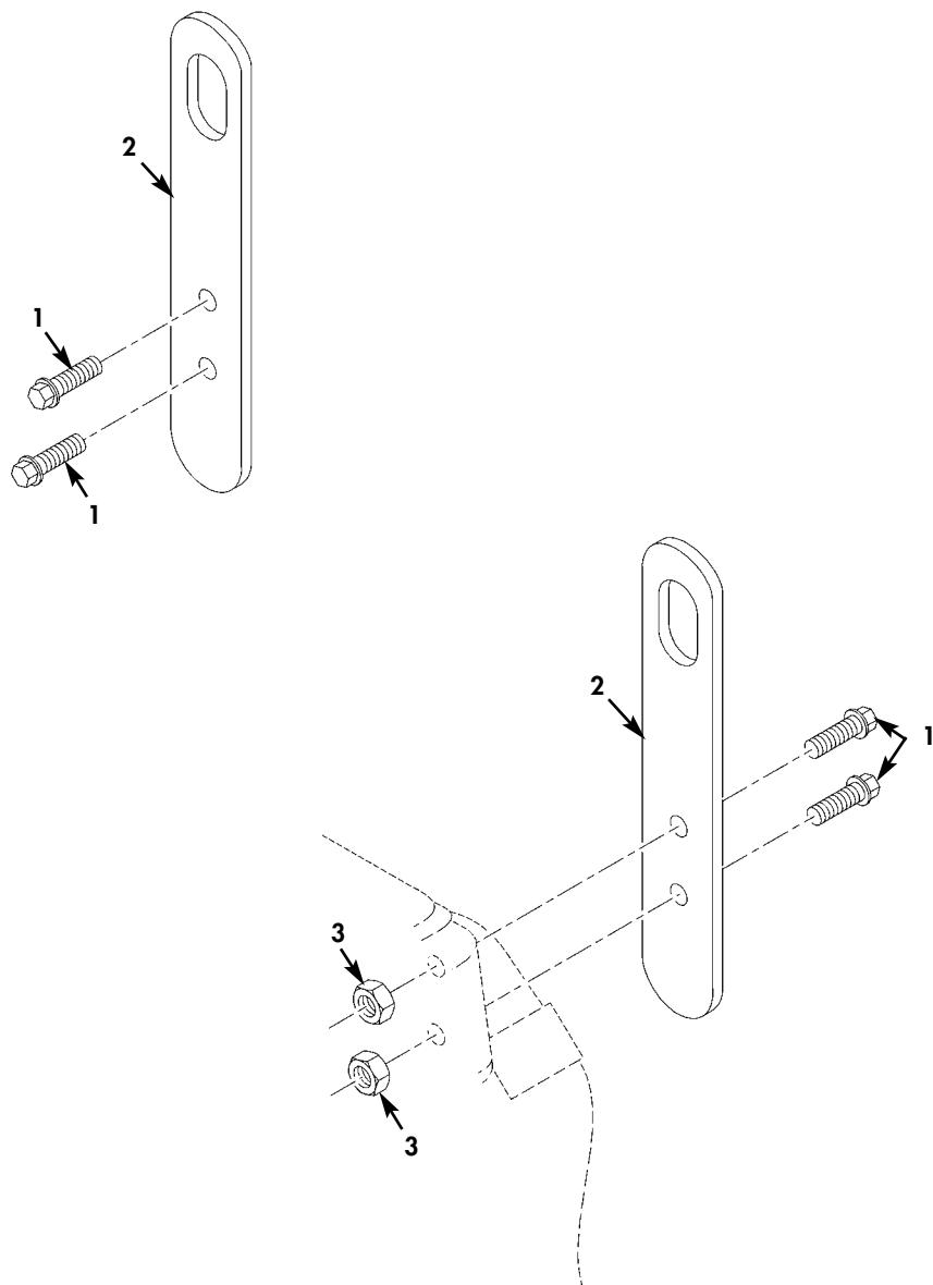
Figure 15. Engine Lifting Brackets.
