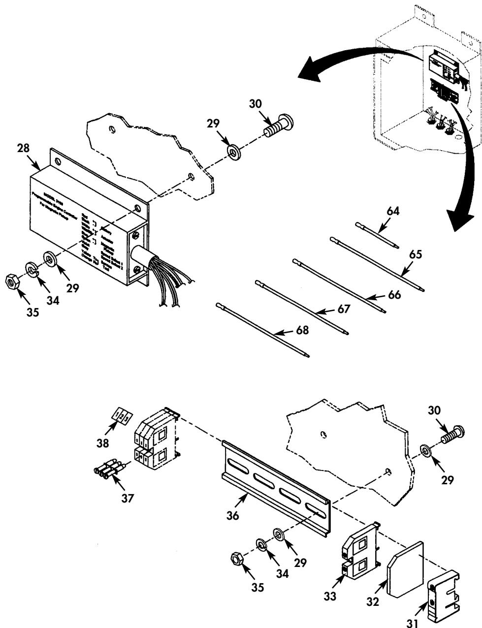
Figure 53. Control Box Assembly (Sheet 3 of 5).
