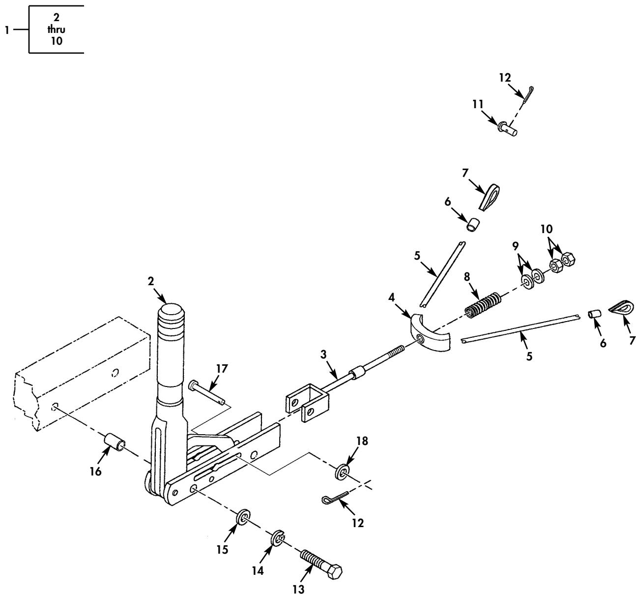
Figure 3. Handbrake.
