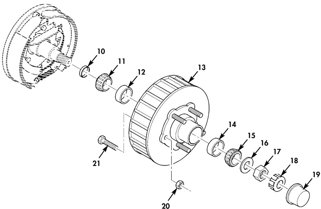
Figure 1. Axle Assembly (Sheet 2 of 3).
