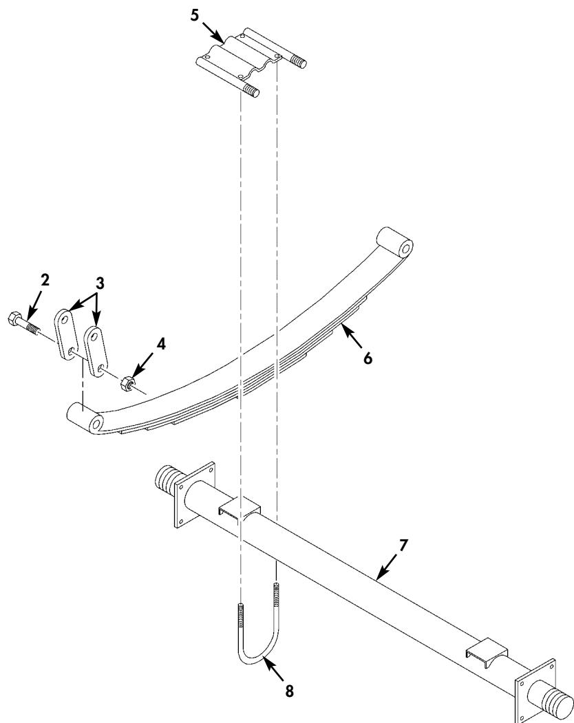
Figure 1. Axle Assembly (Sheet 1 of 3).
