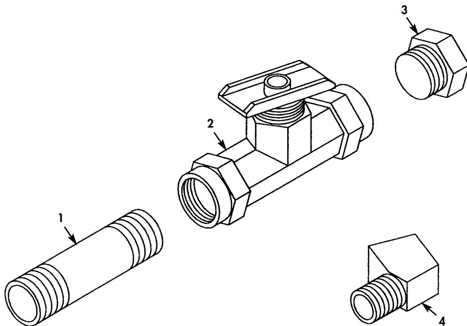
Figure 28. Needle Valve and Elbow.
