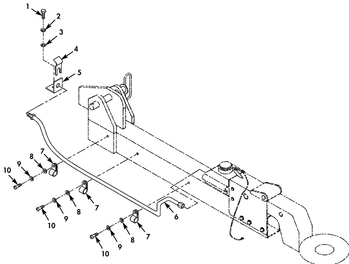
Figure 4. Brake Lines (Sheet 1 of 3).
