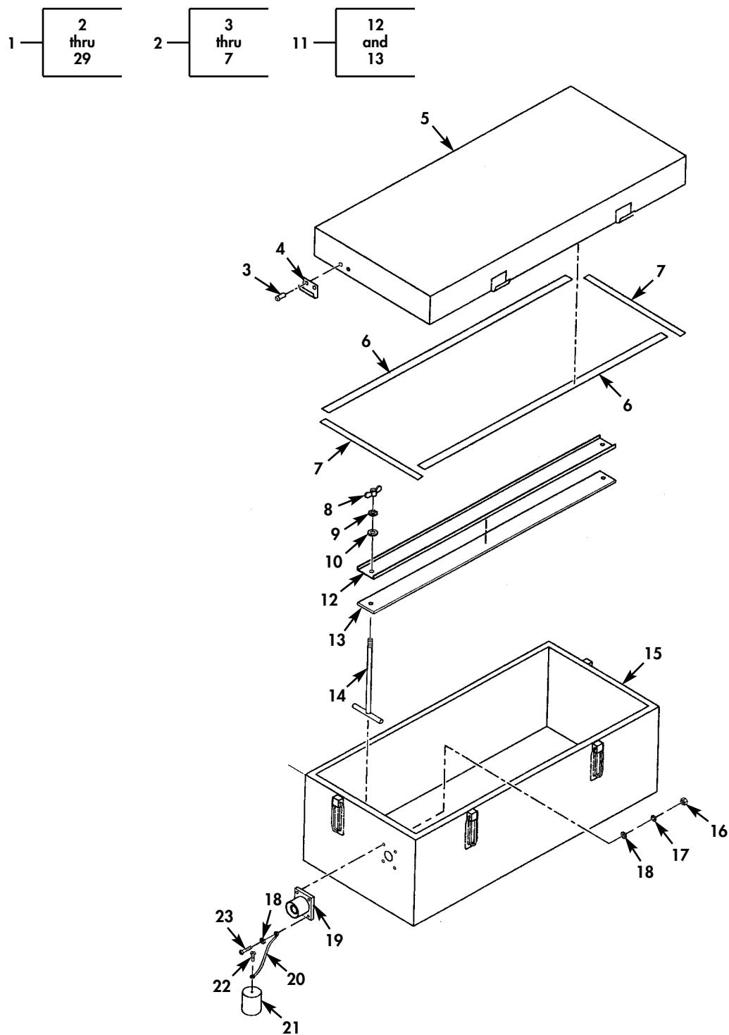
Figure 54. Battery and Battery Box (Sheet 1 of 3).
