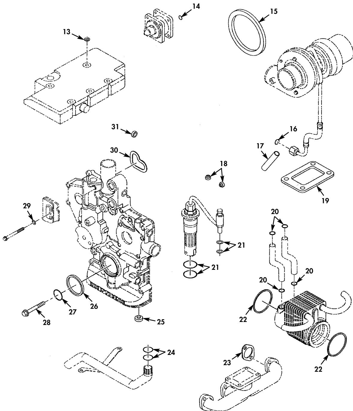
Figure 56. Engine Overhaul Kits (Sheet 2 of 3).
