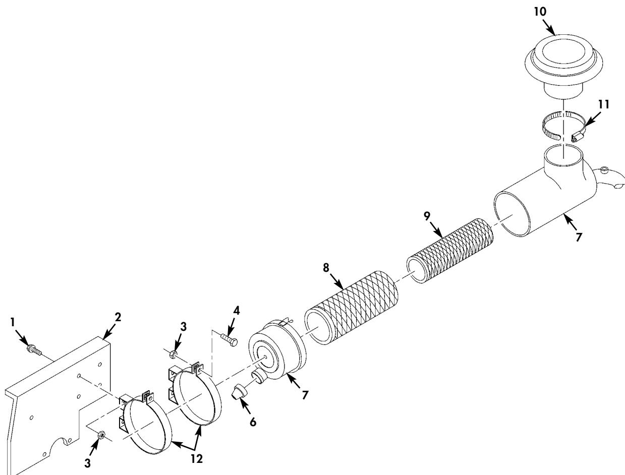
Figure 24. Air Intake (Sheet 1 of 2).
