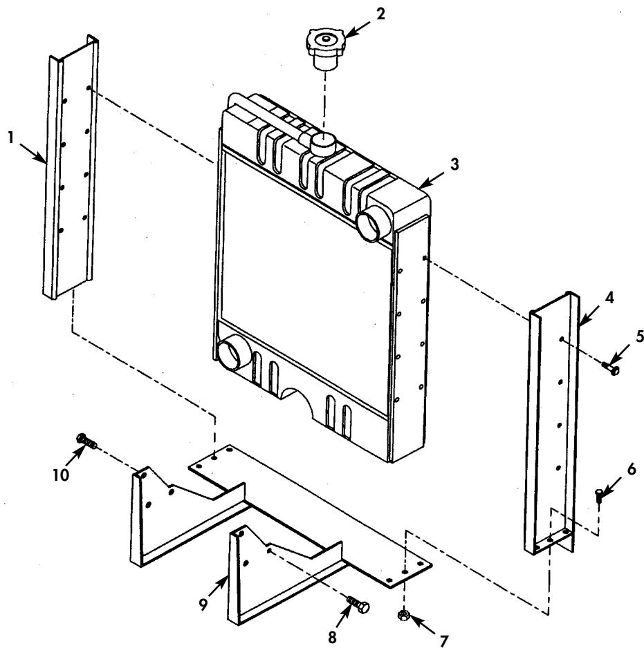
Figure 35. Radiator (Sheet 1 of 3).
