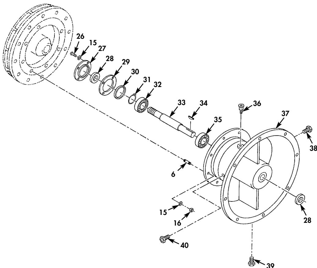
Figure 7. Centrifugal Pump (Sheet 3 of 5).
