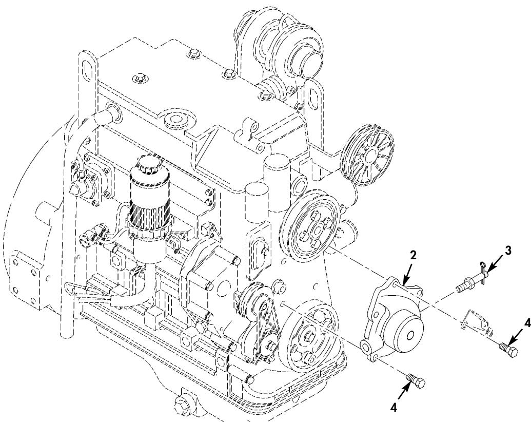
Figure 30. Engine Cooling System Pump.
