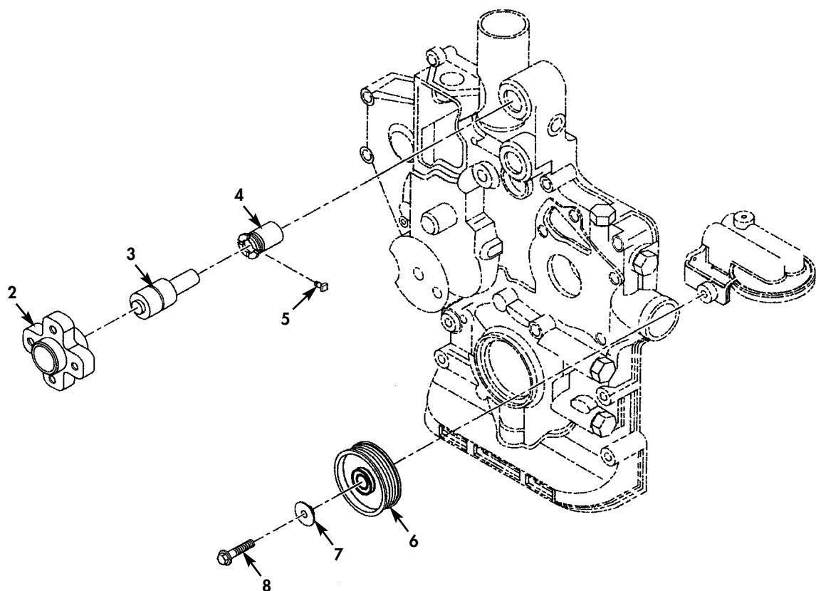
Figure 32. Fan Drive and Idler Pulley.
