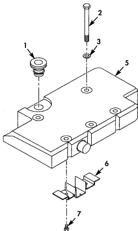
Figure 17. Rocker Arm Cover Assembly.
