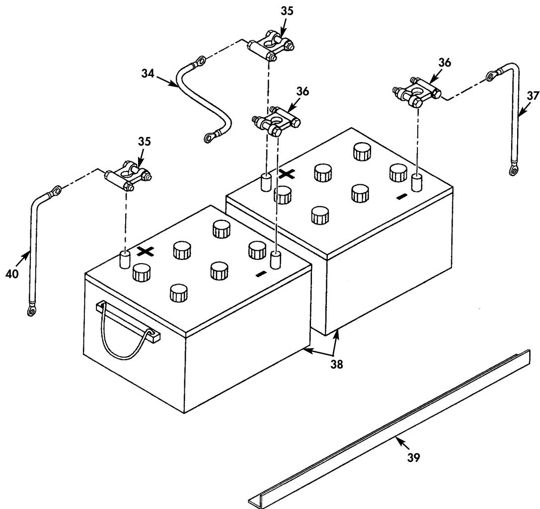
Figure 54. Battery and Battery Box (Sheet 3 of 3).
