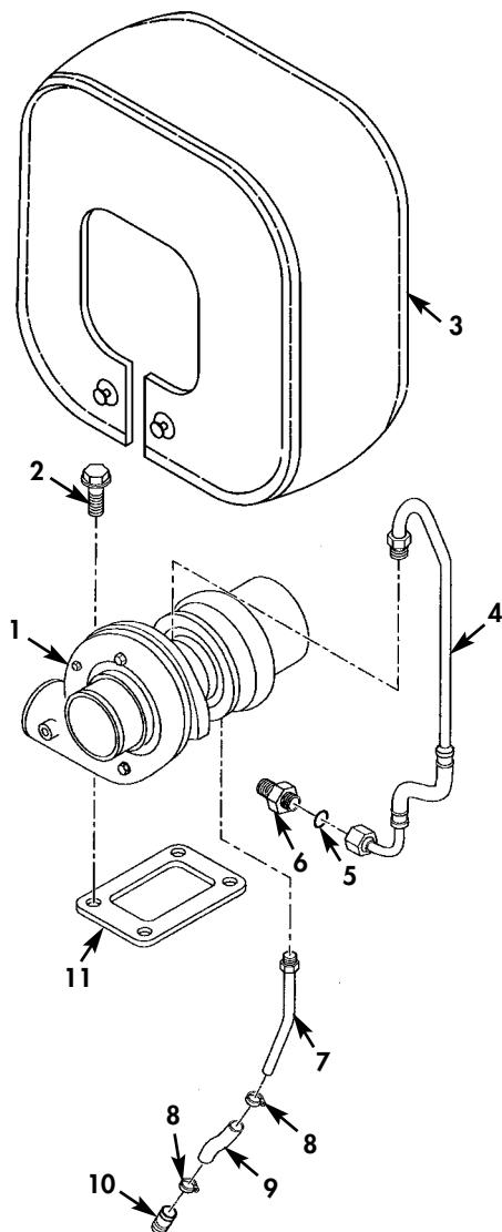
Figure 16. Turbocharger.
