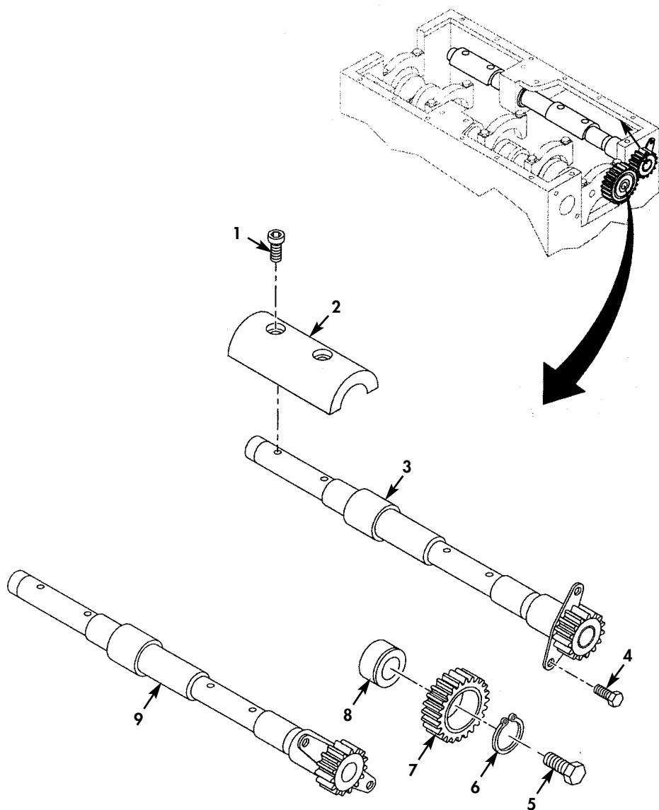
Figure 12. Balancer Shafts.
