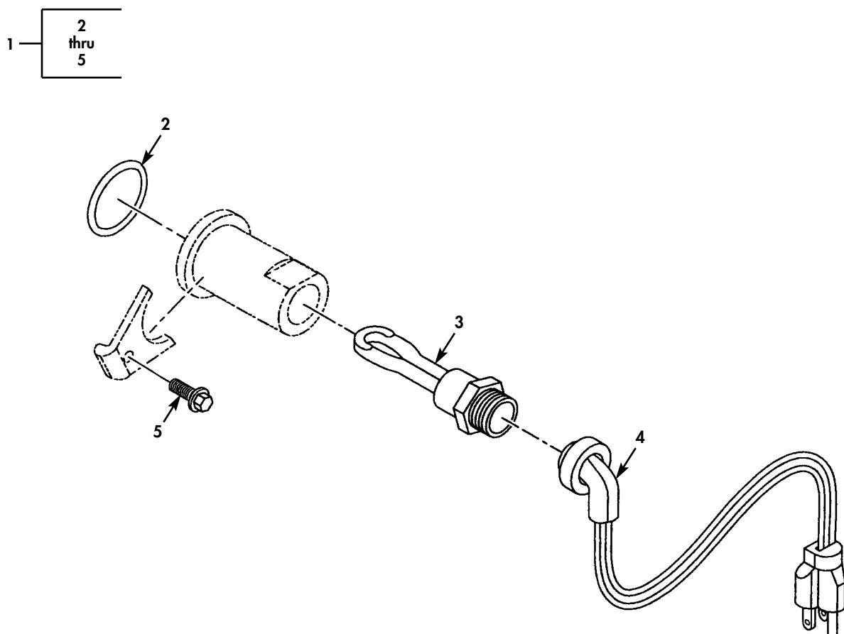
Figure 34. Engine Coolant Heater.
