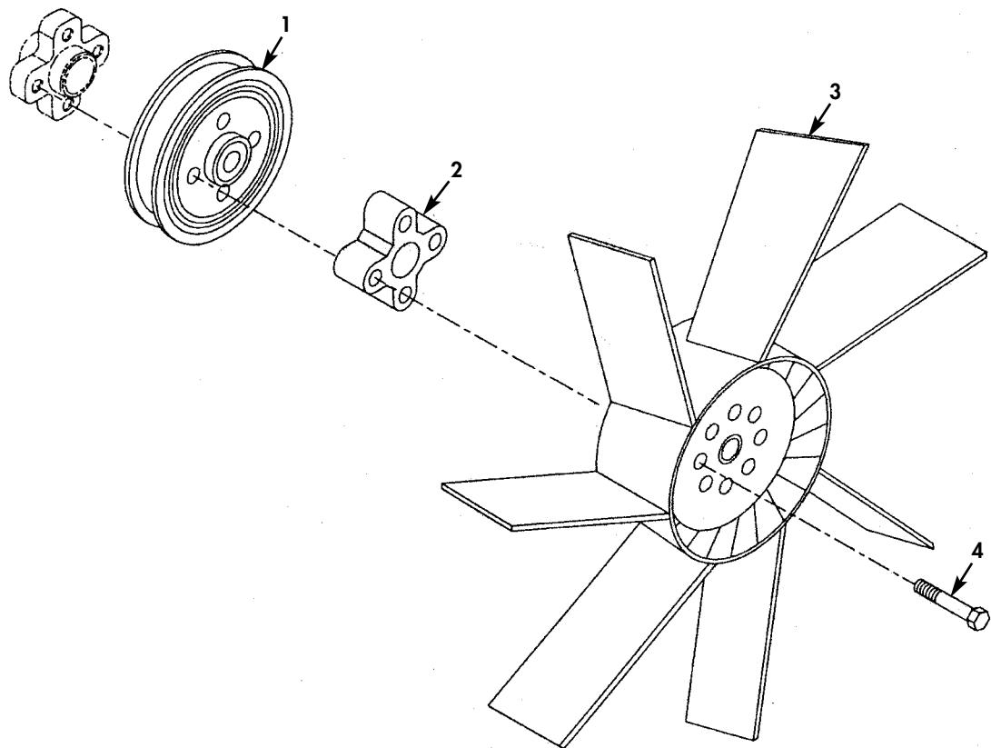
Figure 36. Fan Pulley and Cooling Fan.
