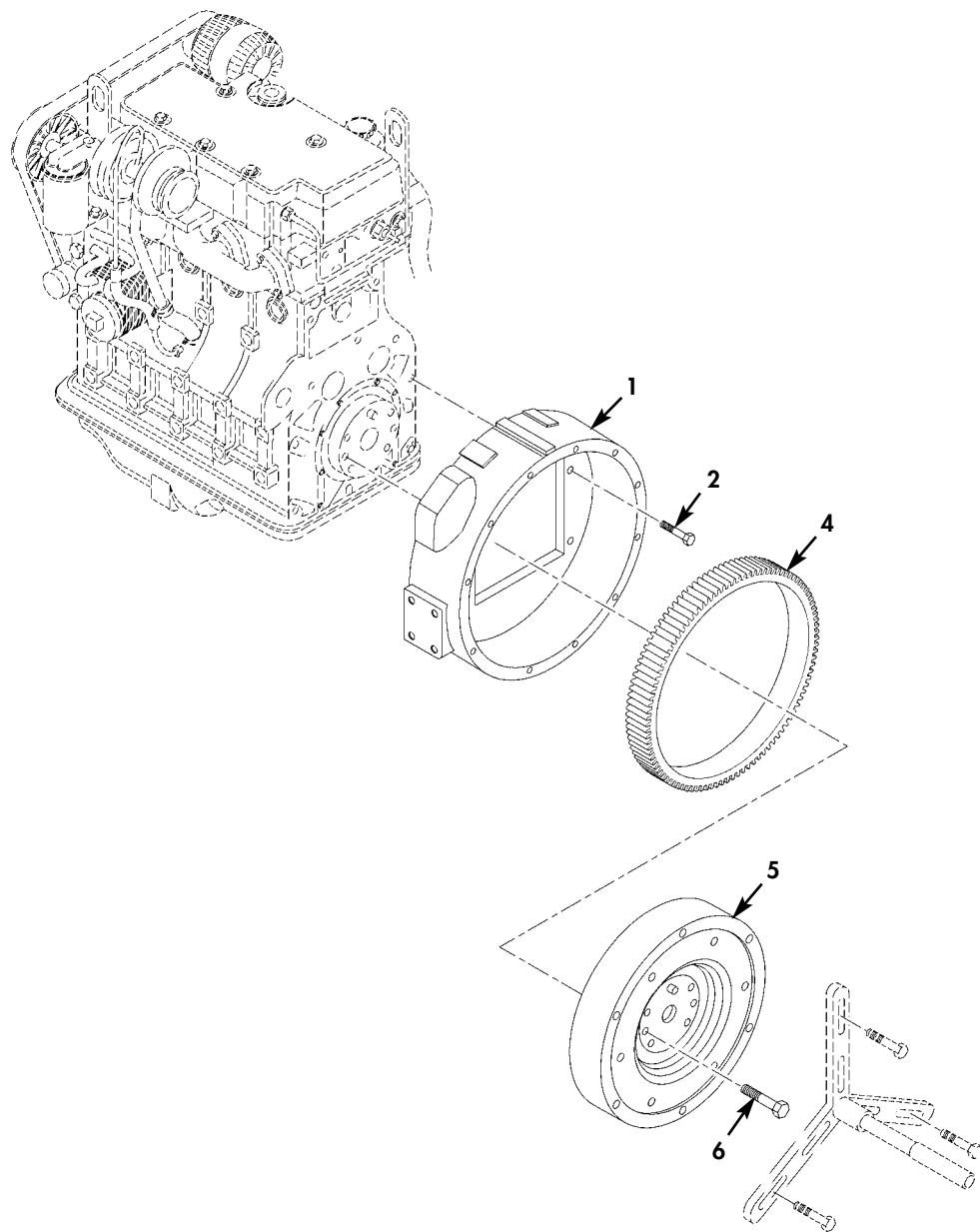
Figure 10. Flywheel and Flywheel Housing.
