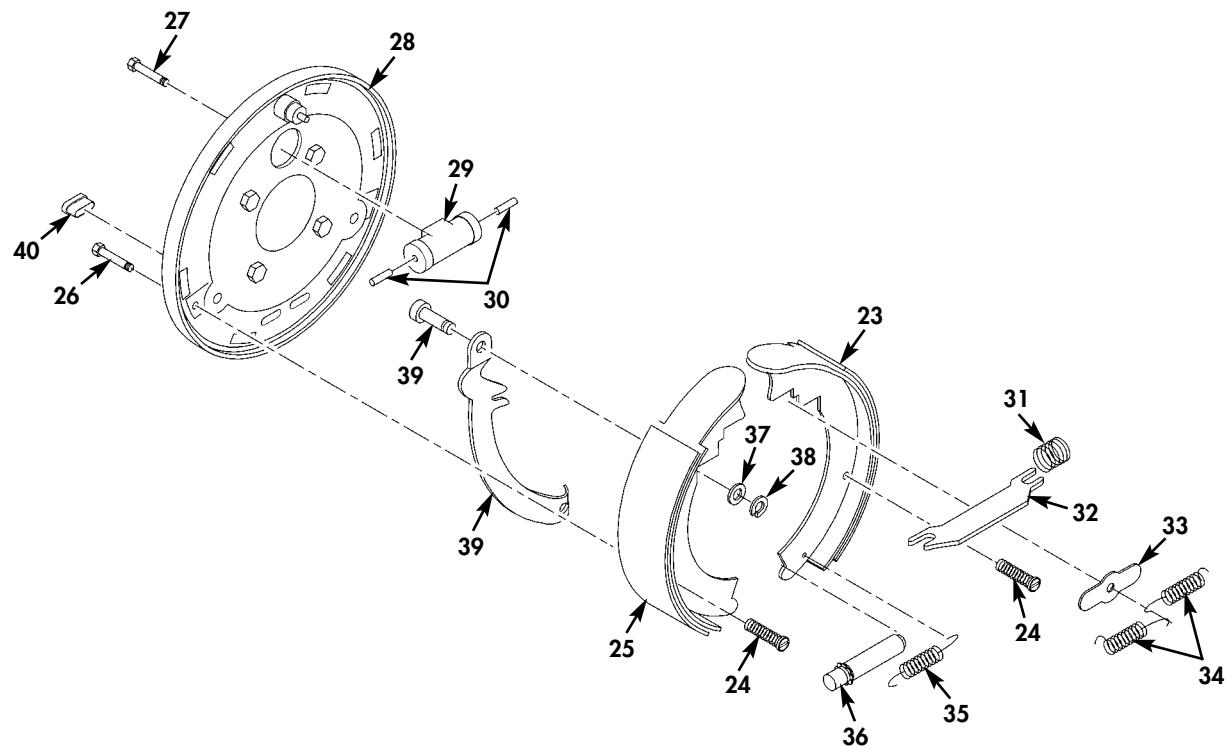
Figure 1. Axle Assembly (Sheet 3 of 3).
