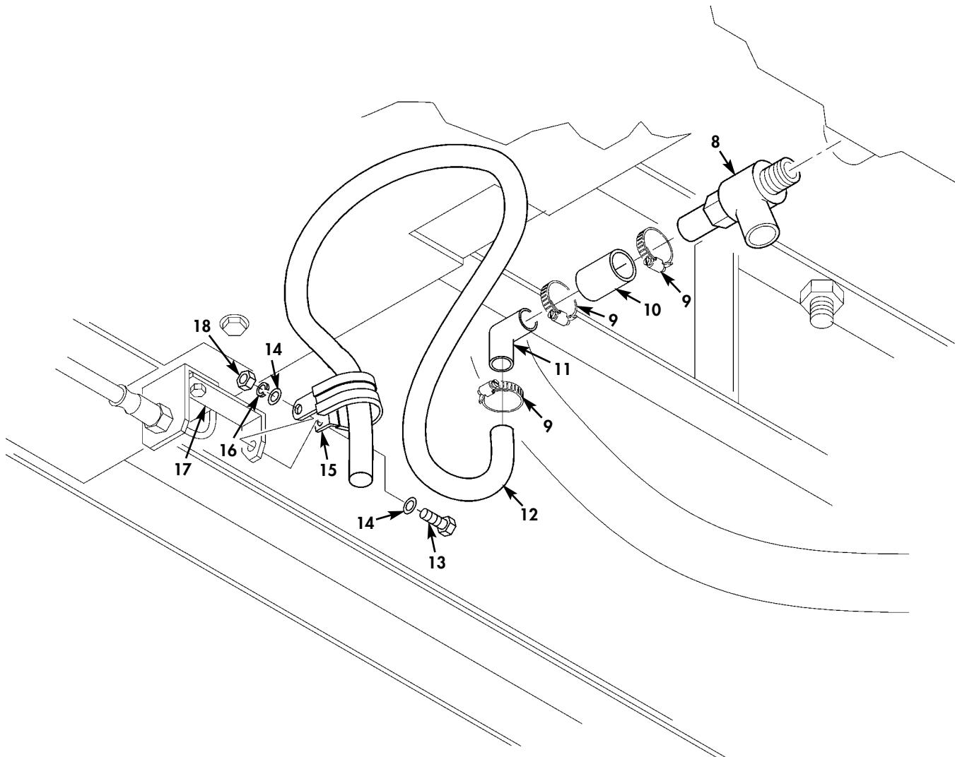
Figure 26. Oil Pan and Drain Hose (Sheet 2 of 2).
