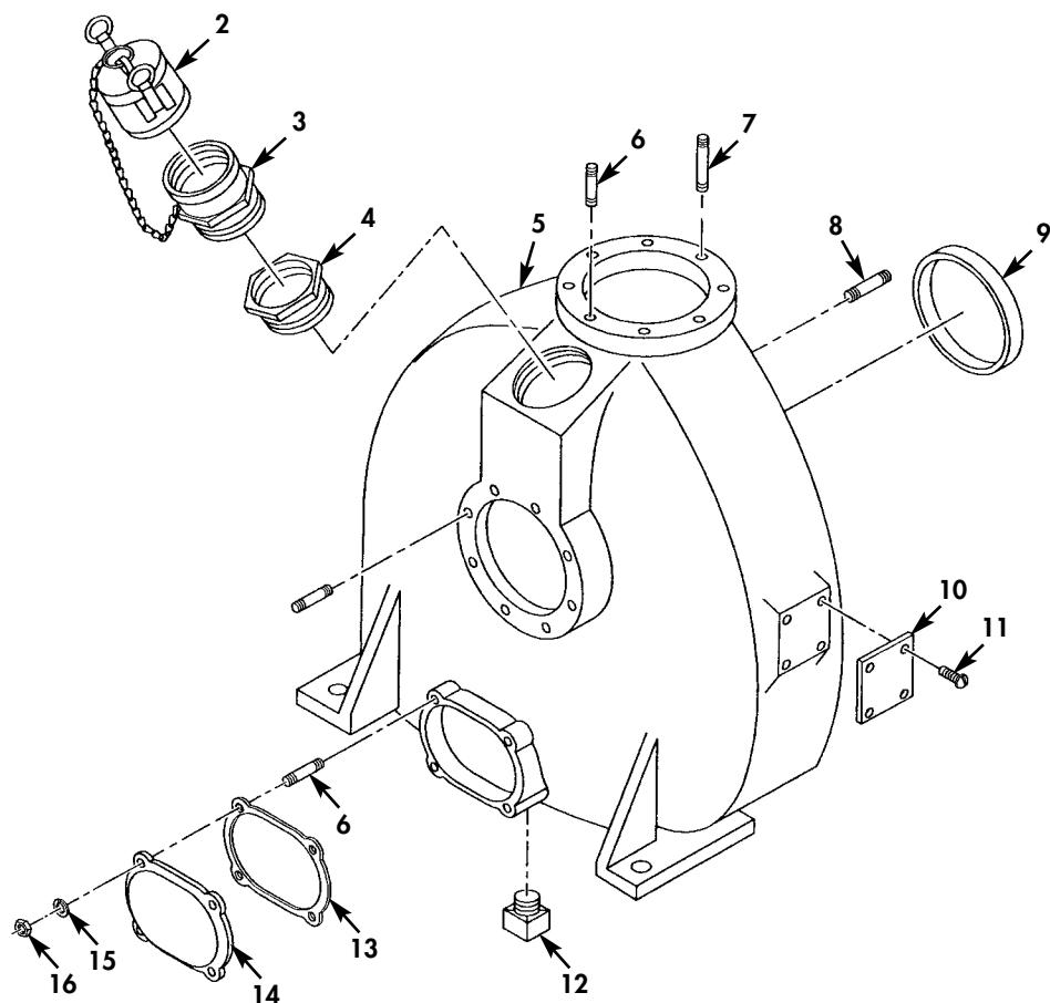
Figure 7. Centrifugal Pump (Sheet 1 of 5).
