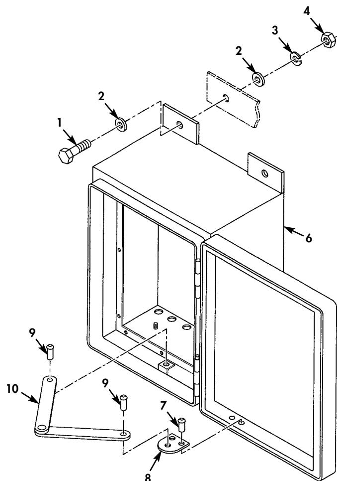
Figure 53. Control Box Assembly (Sheet 1 of 5).
