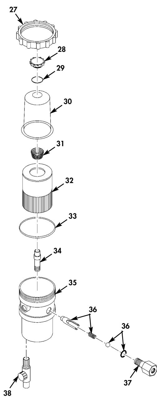
Figure 19. Fuel Pump and Fuel / Water Separator (Sheet 2 of 2).
