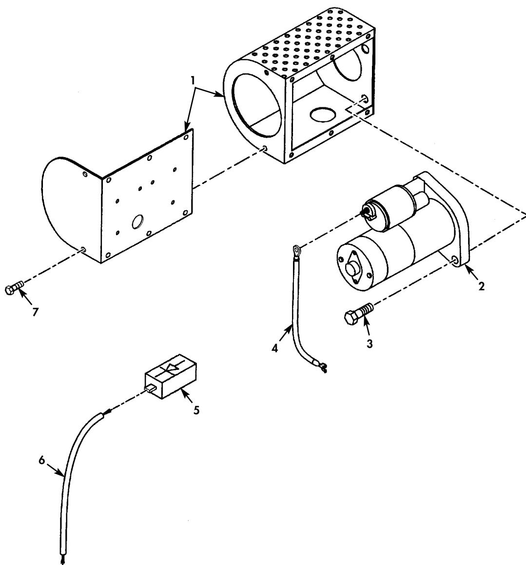
Figure 43. Starter Group and Electrical Relay Box (Sheet 1 of 2).
