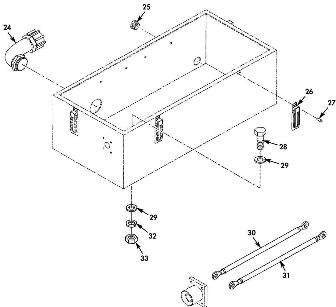
Figure 54. Battery and Battery Box (Sheet 2 of 3).
