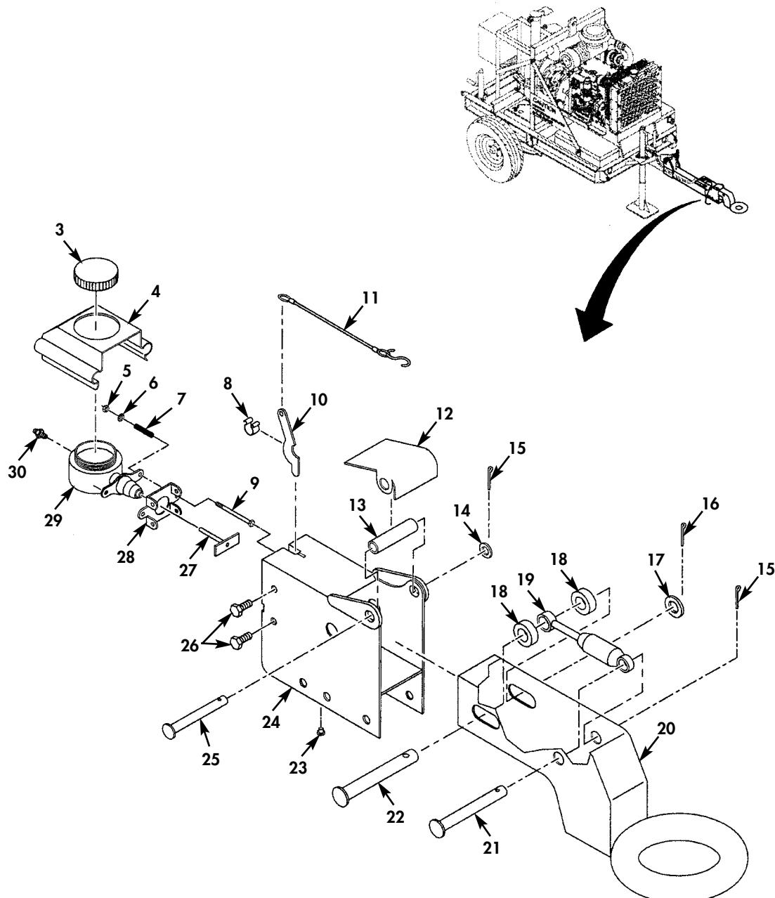
Figure 47. Tongue Assembly (Sheet 1 of 2).
