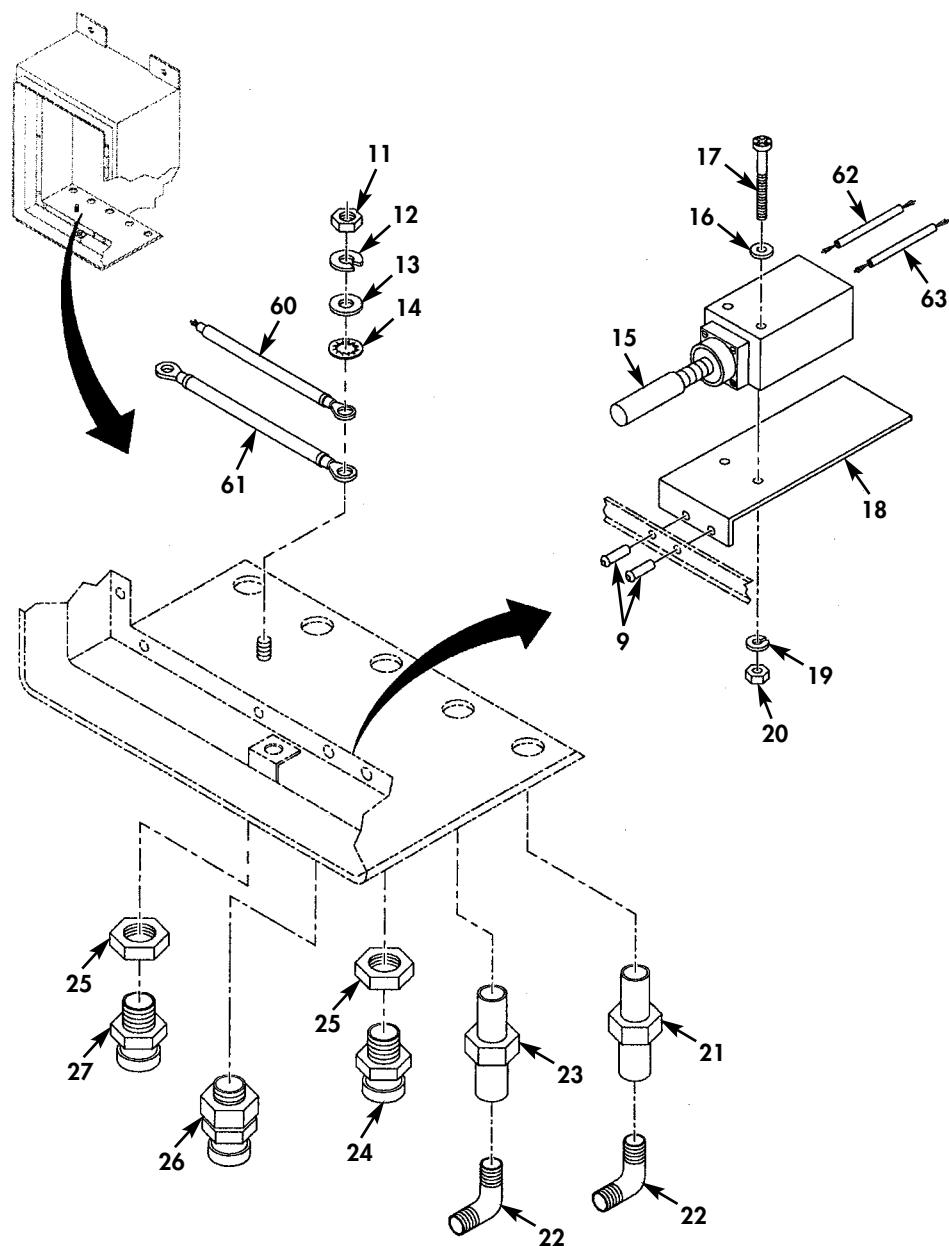
Figure 53. Control Box Assembly (Sheet 2 of 5).
