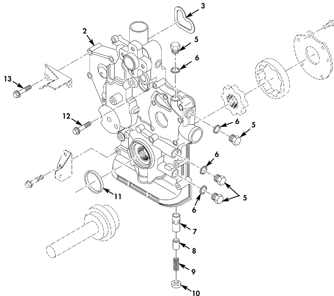
Figure 21. Timing Gear Cover.
