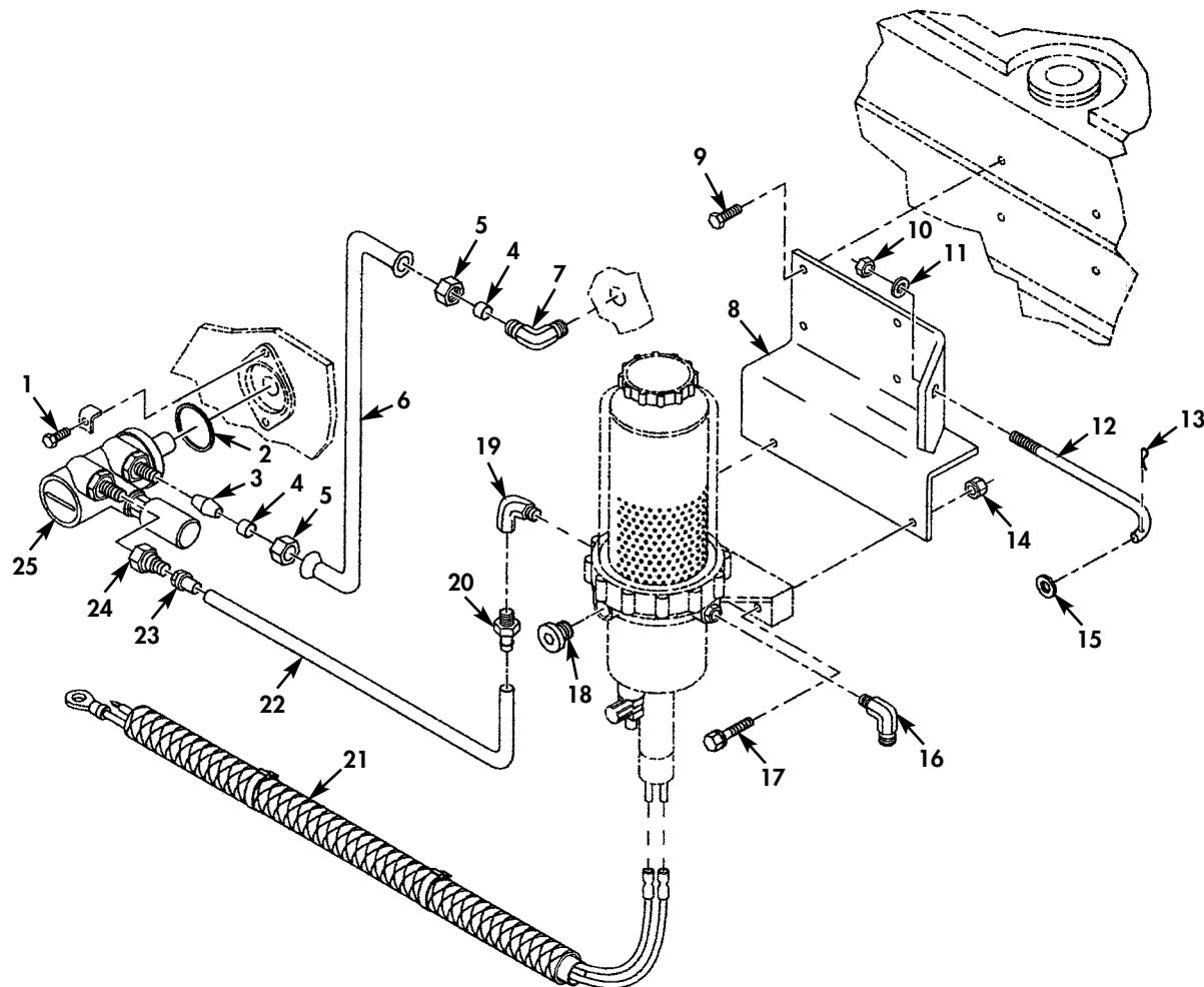
Figure 19. Fuel Pump and Fuel / Water Separator (Sheet 1 of 2).
