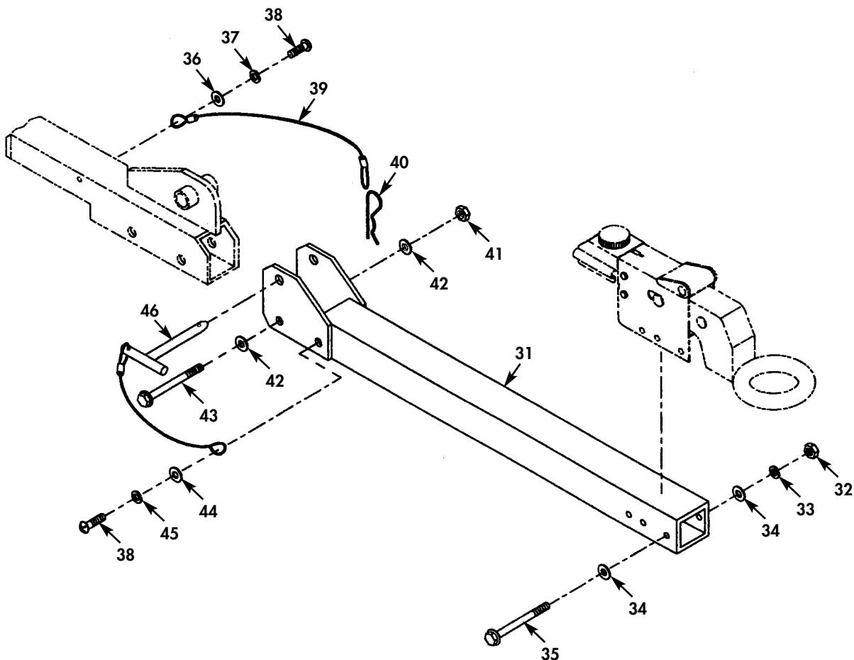
Figure 47. Tongue Assembly (Sheet 2 of 2).
