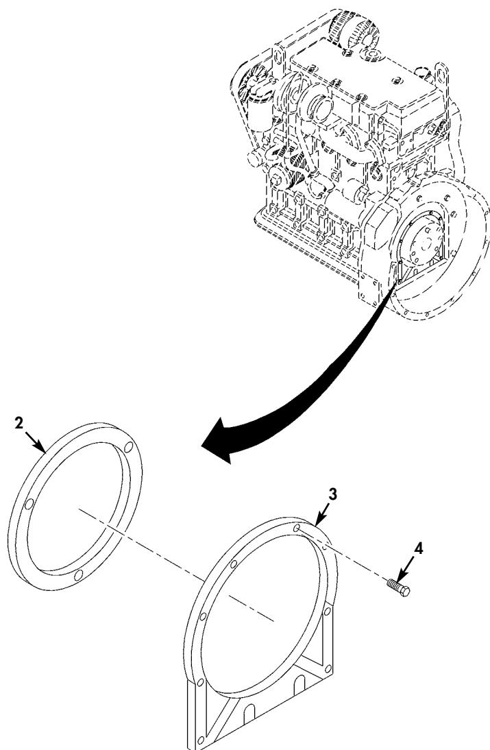
Figure 29. Rear Oil Seal.
