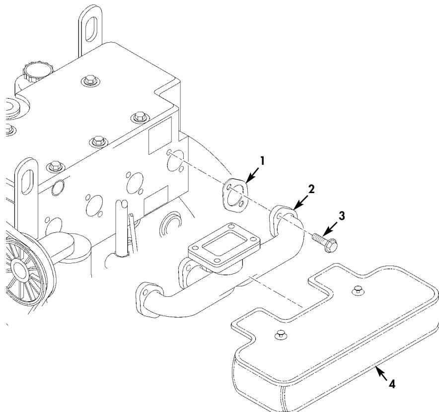
Figure 38. Exhaust Manifold.
