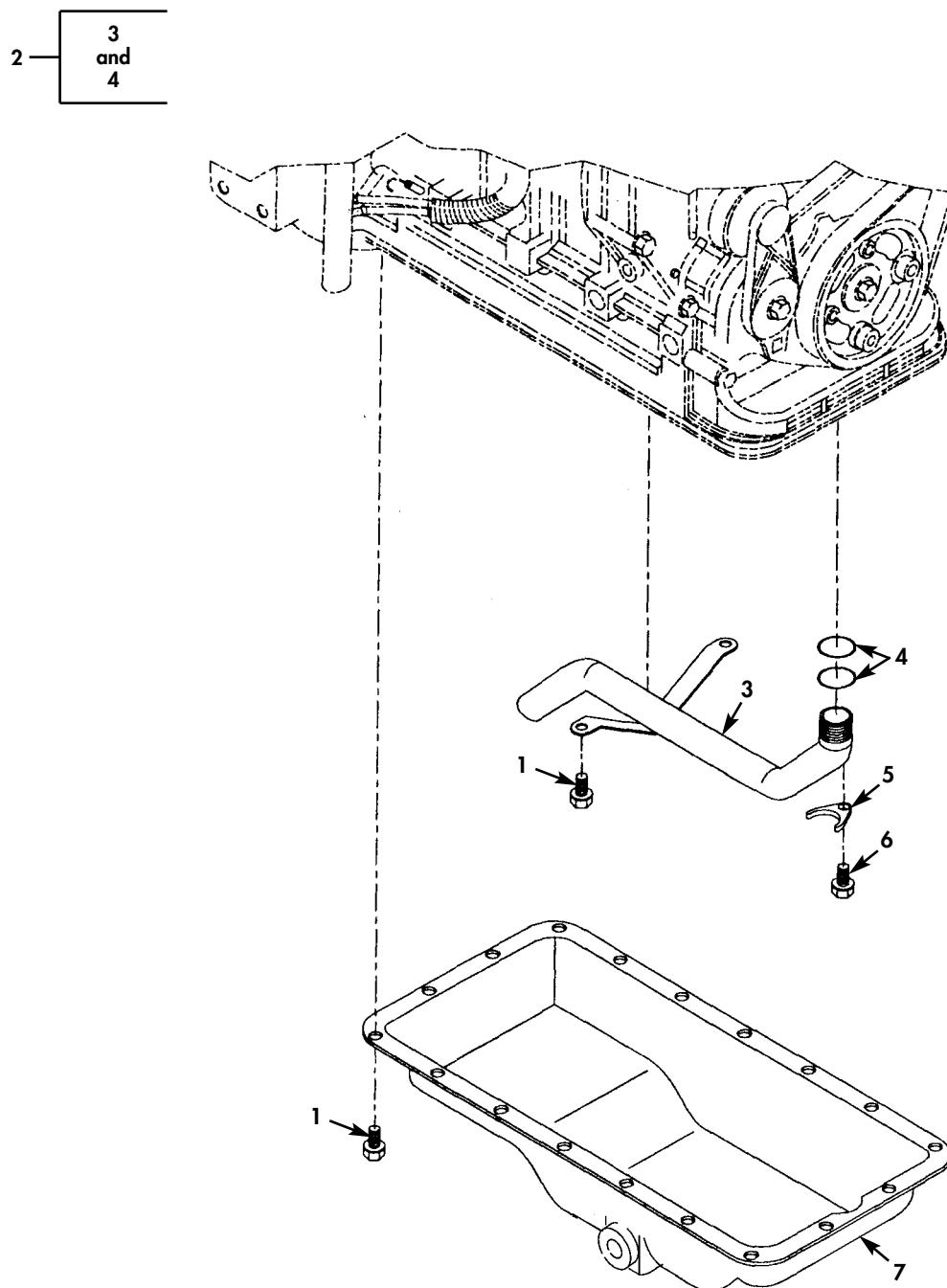
Figure 26. Oil Pan and Drain Hose (Sheet 1 of 2).
