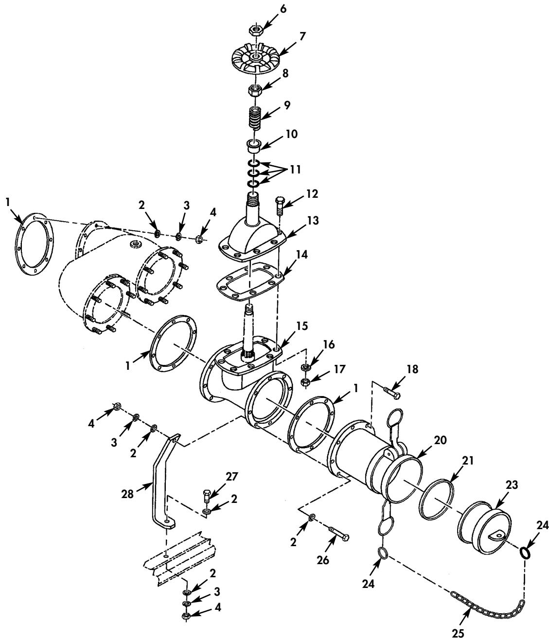
Figure 44. Suction End Gate Valves.
