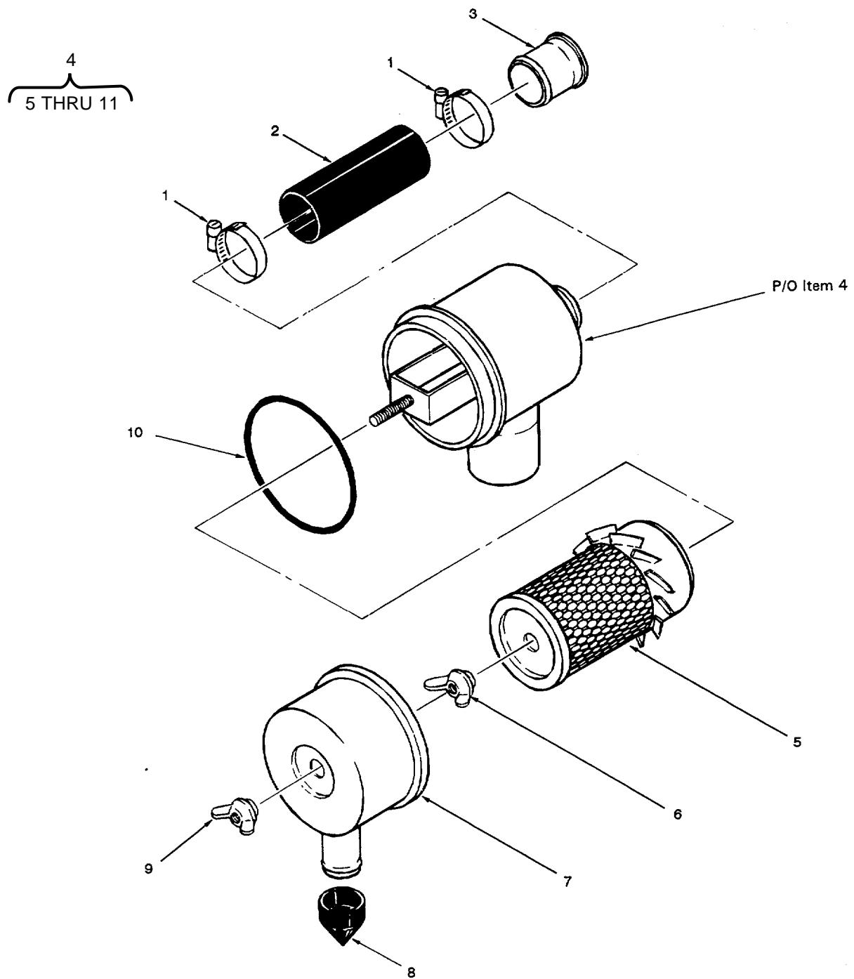
Figure 19. Air Filter Assembly
