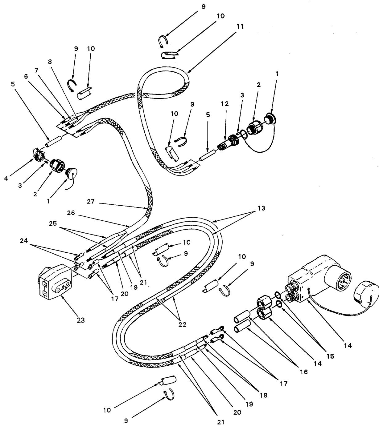
Figure 17. Cable Assembly (W202), Battery Power
