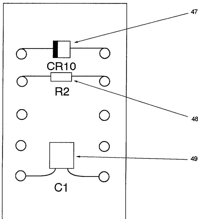
Figure 21 (Sheet 2 of 6). Control Panel Assembly-TB1 Components
