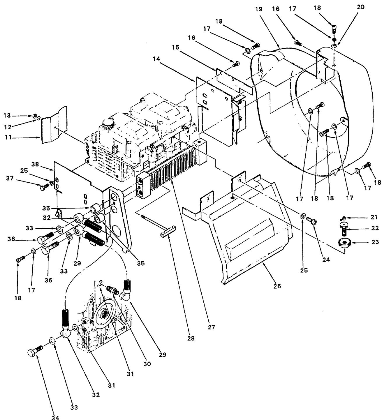
Figure 10 (Sheet 2 of 13). Engine Assembly - Shrouds and Gates
