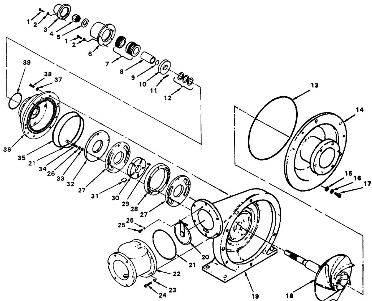
Figure 8. Fuel Transfer Pump Assembly
