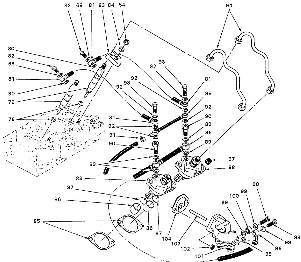
Figure 10 (Sheet 5 of 13). Engine Assembly - Fuel System Components
