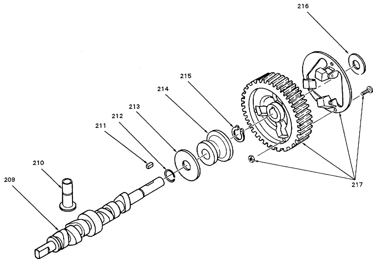
Figure 10 (Sheet 12 of 13). Engine Assembly - Camshaft Assembly
