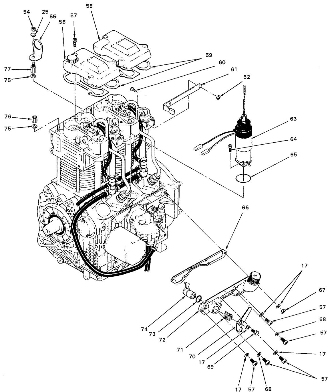
Figure 10 (Sheet 4 of 13) Engine Assembly - Valve and Fuel Covers, Fuel Solenoid
