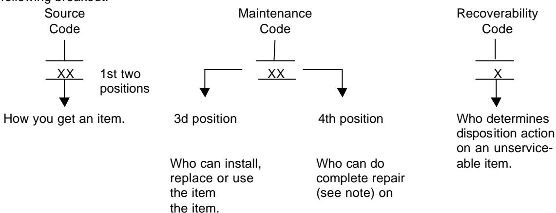
\*Complete Repair. Maintenance capacity, capability, and authority to perform all corrective maintenance tasks of the "Repair" function in a use/user environment in order to restore serviceability to a failed item.
