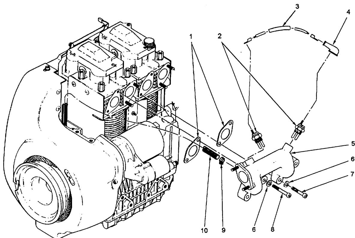
Figure 10 (Sheet 1 of 13). Engine Assembly - Intake Manifold
