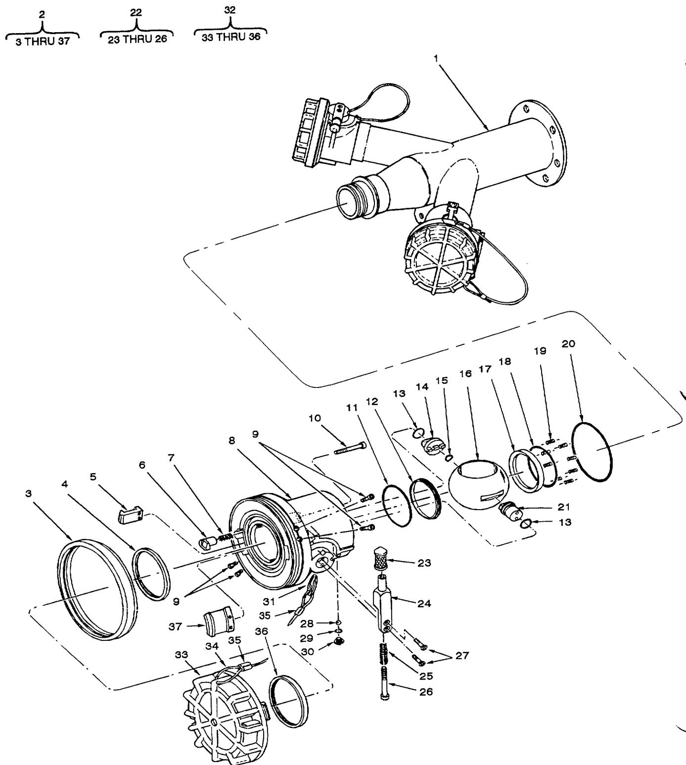
Figure 7. Inlet Manifold Assembly
