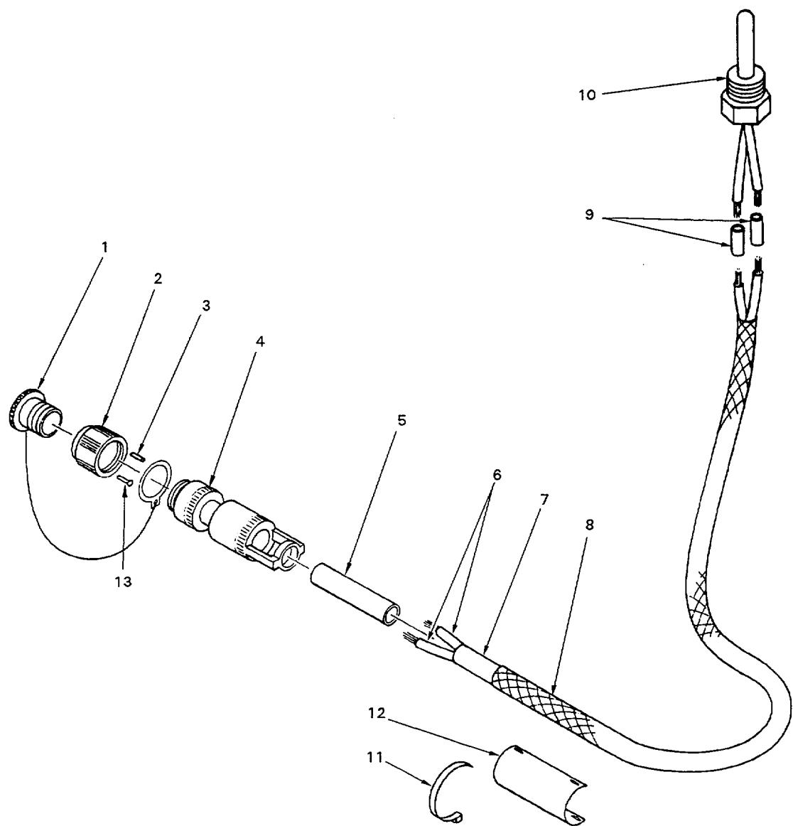
Figure 2. Cable Assembly W103
