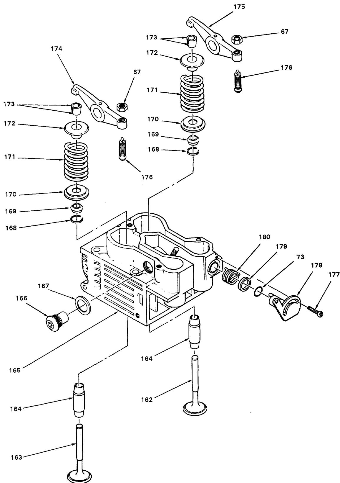
Figure 10 (Sheet 9 of 13). Engine Assembly - Cylinder Head Assembly
