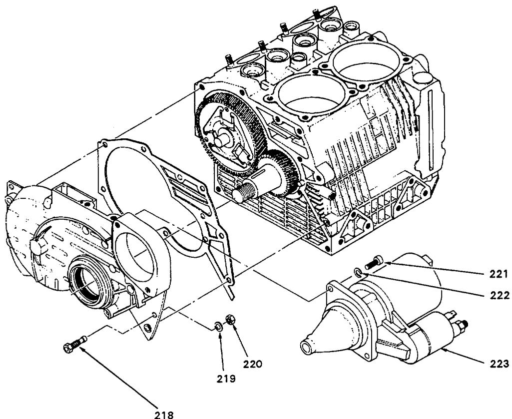
Figure 10 (Sheet 13 of 13). Engine Assembly - Starter, RFI Fitting
