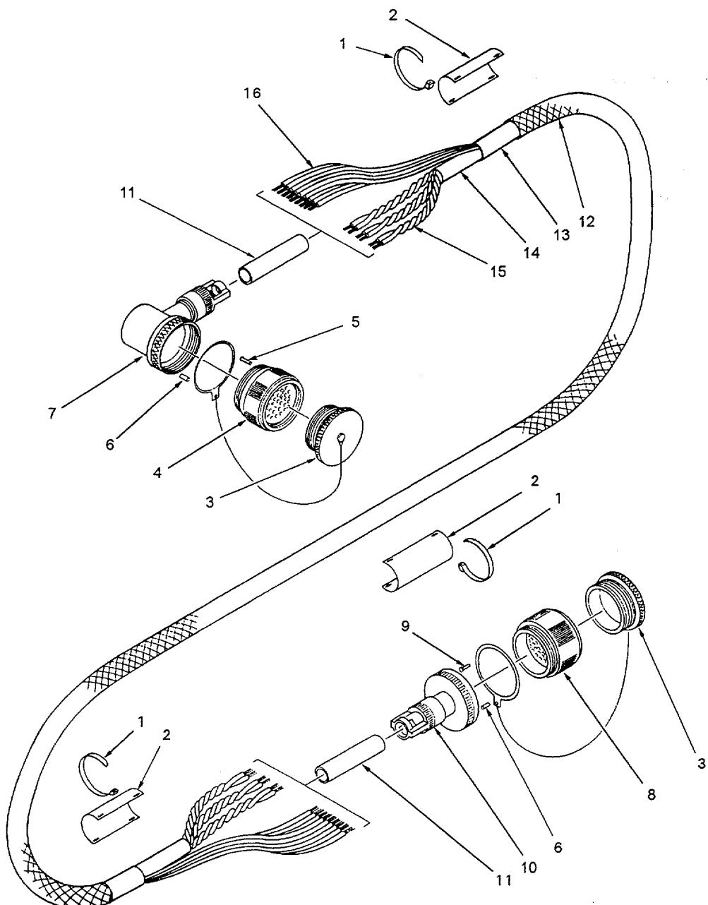
Figure 18. Cable Assembly (W201), Control
