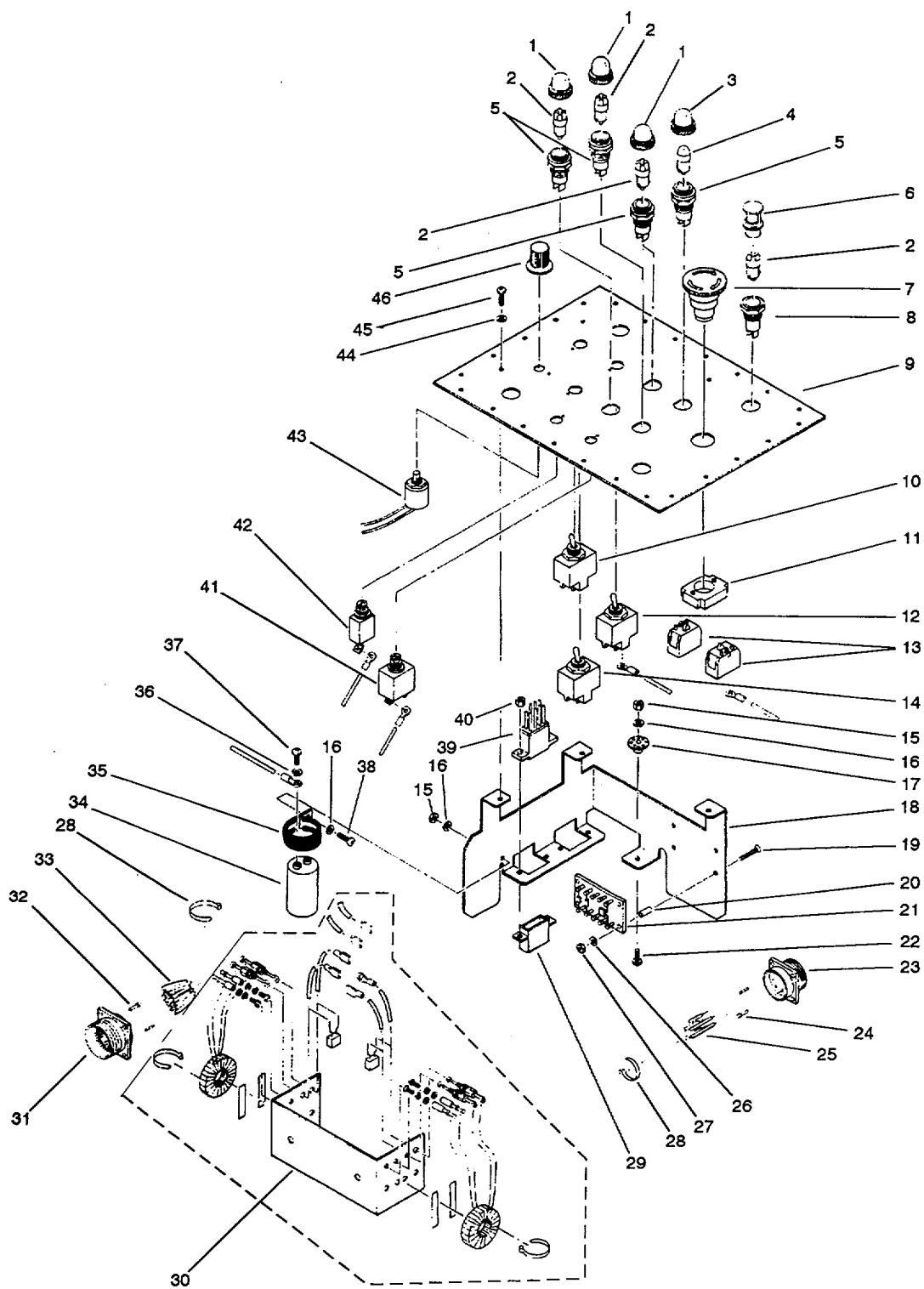
Figure 21 (Sheet 1 of 6). Control Panel Assembly
