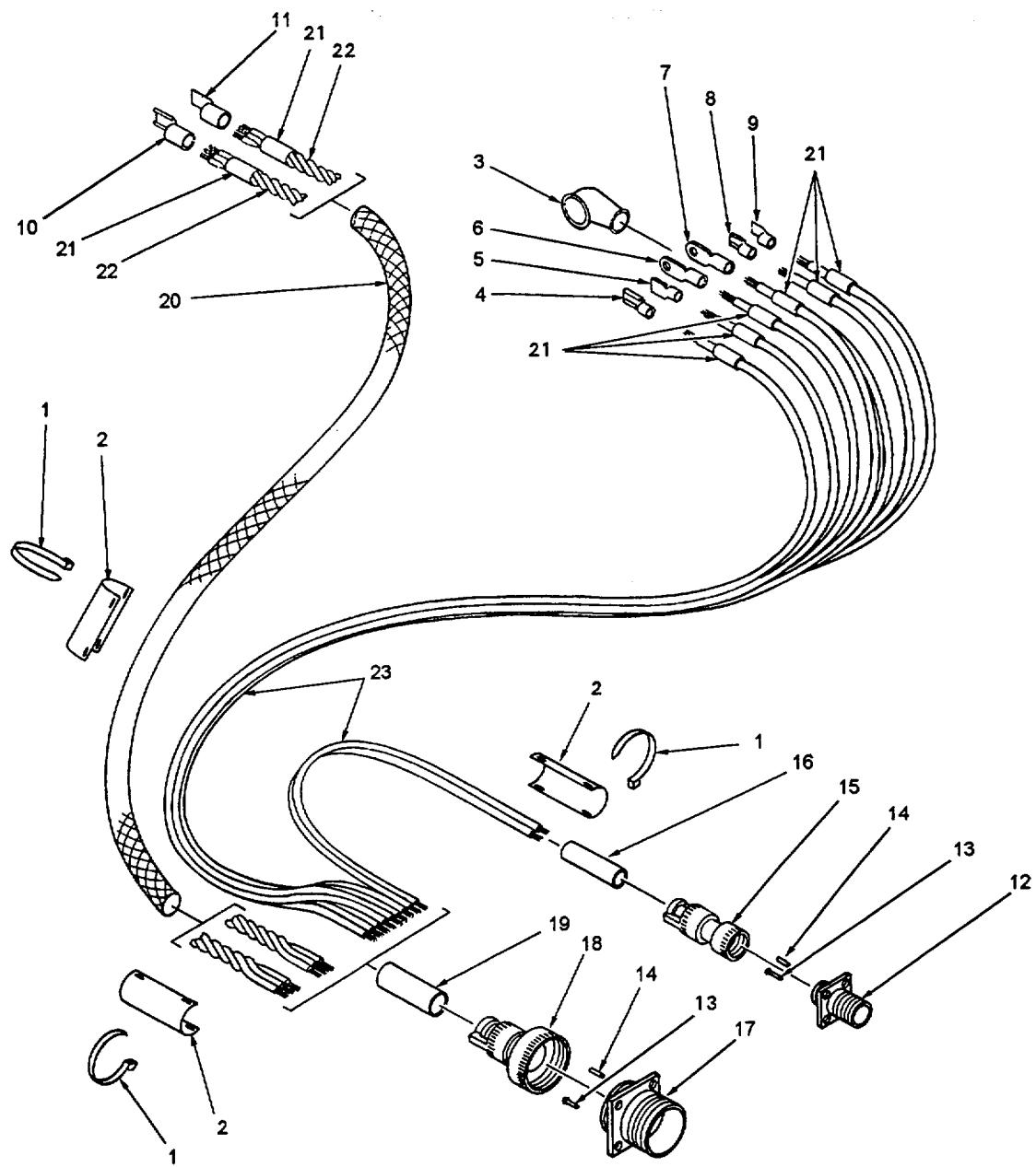
Figure 11. Cable Assembly (W101), Engine Module
