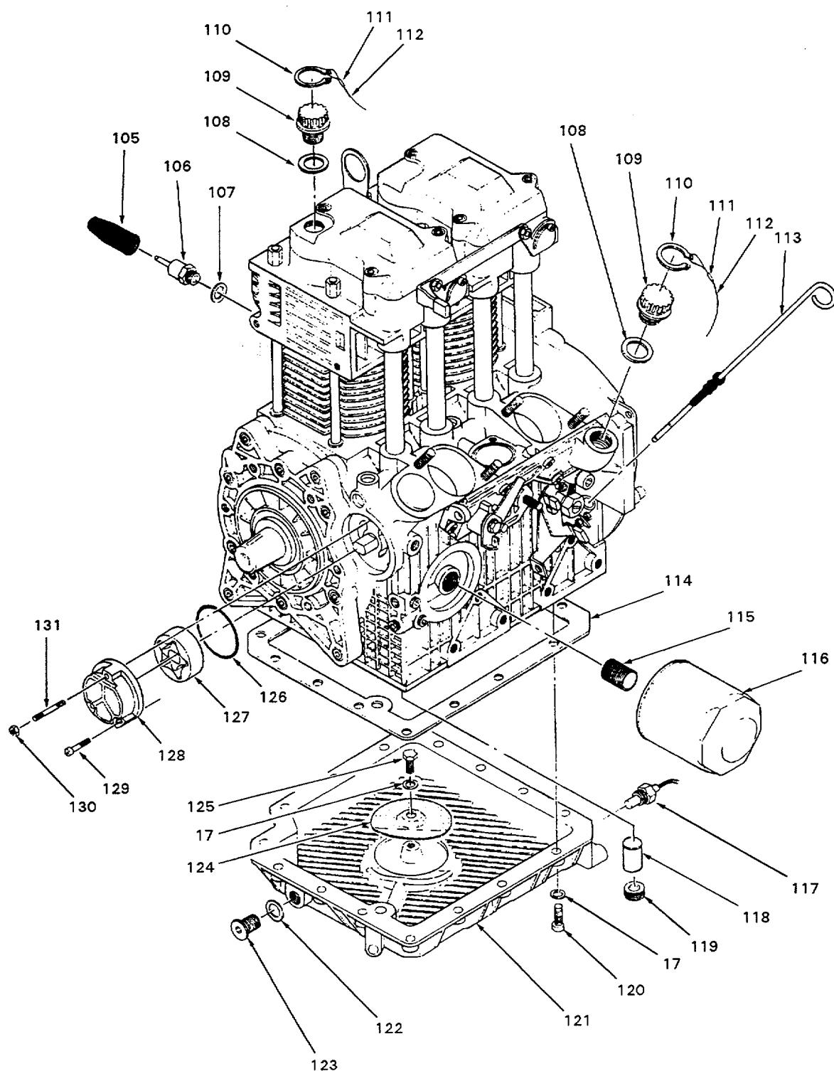
Figure 10 (Sheet 6 of 13). Engine Assembly - Oil System Components
