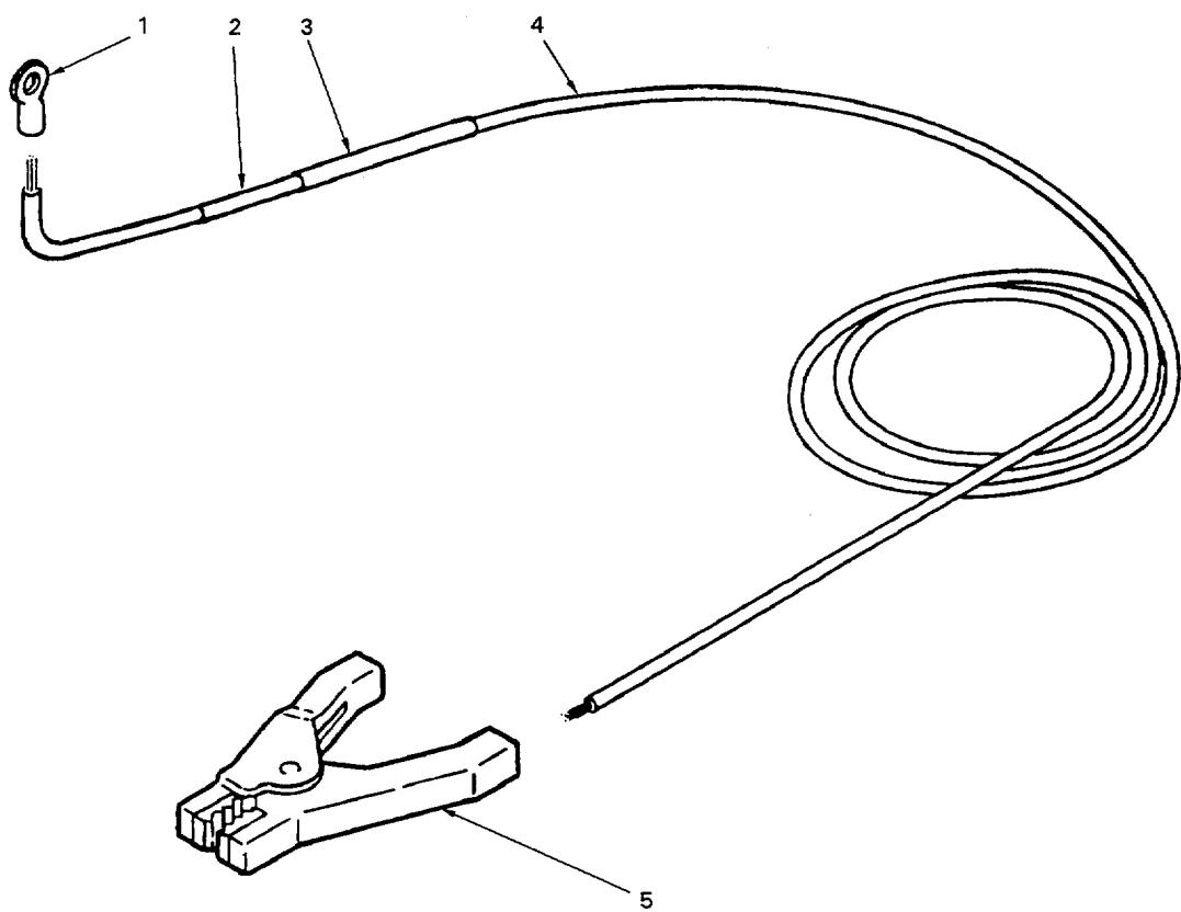
Figure 3. Cable Assembly, Ground
