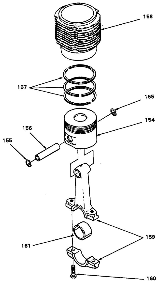
Figure 10 (Sheet 8 of 13). Engine Assembly - Cylinder-Piston Assembly
