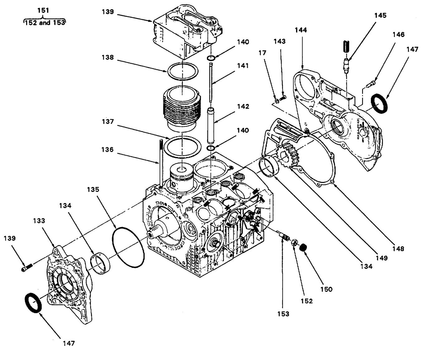
Figure 10 (Sheet 7 of 13). Engine Assembly - End Covers and Top End Components
