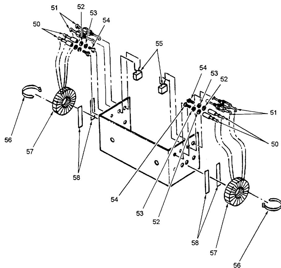
Figure 21 (Sheet 3 of 6). Control Panel Assembly-RFI Components
