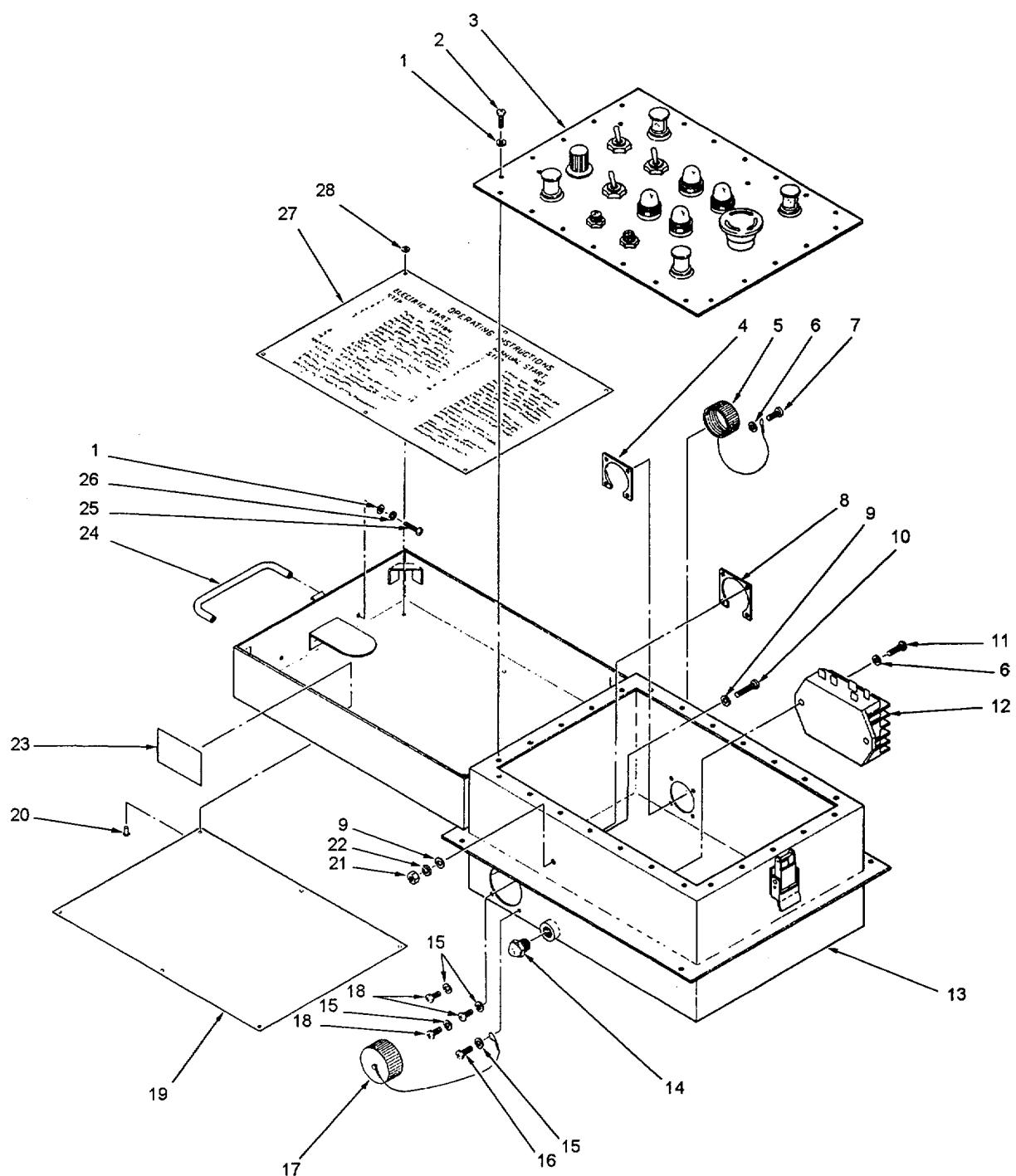
Figure 20. Control Box Assembly
