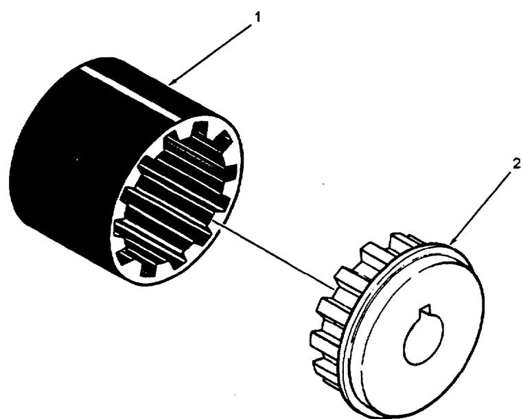
*Figure 13. Flexible Coupling Assembly*
