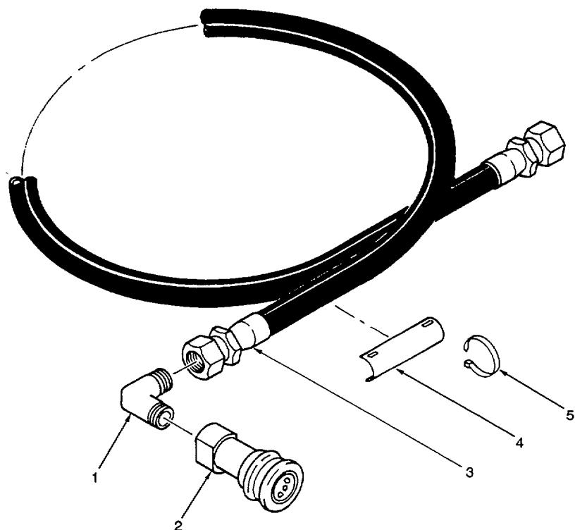
*Figure 4. Fuel Line Assembly (Return)*
