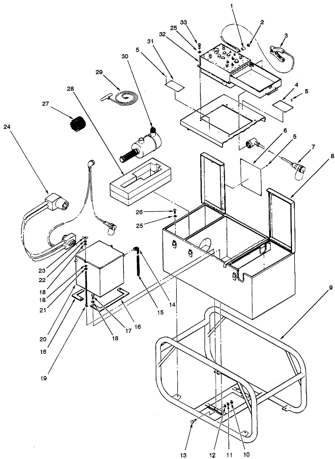
Figure 16. Accessory Module Assembly
