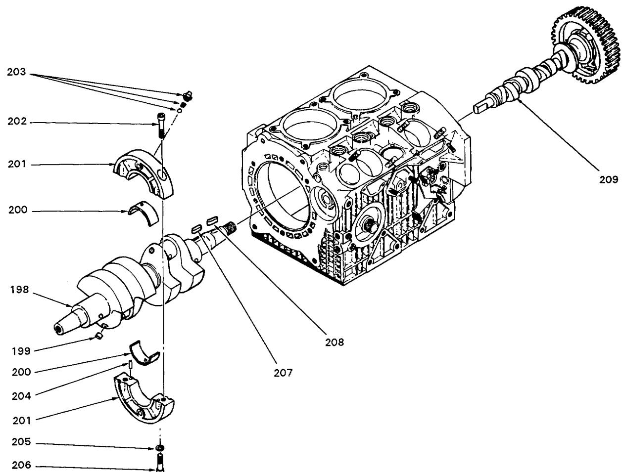
Figure 10 (Sheet 11 of 13). Engine Assembly - Camshaft, Crankshaft Assembly
