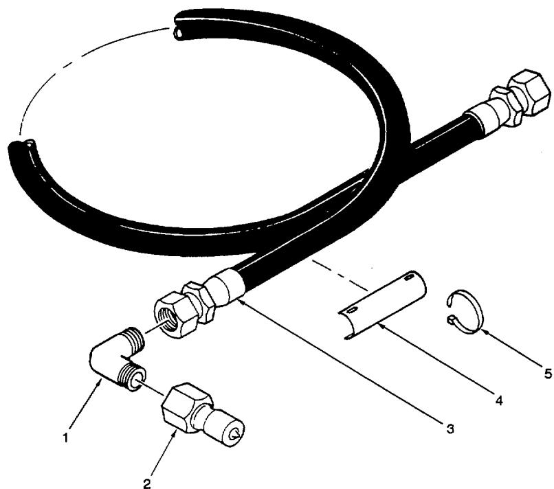
*Figure 5. Fuel Line Assembly (Supply)*
