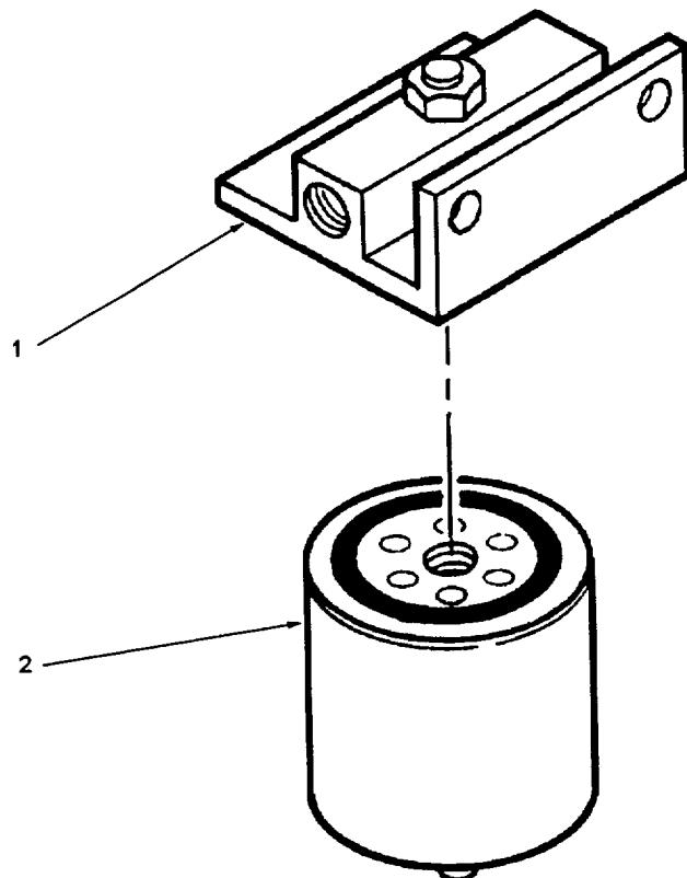
*Figure 14. Fuel Filter Assembly*
