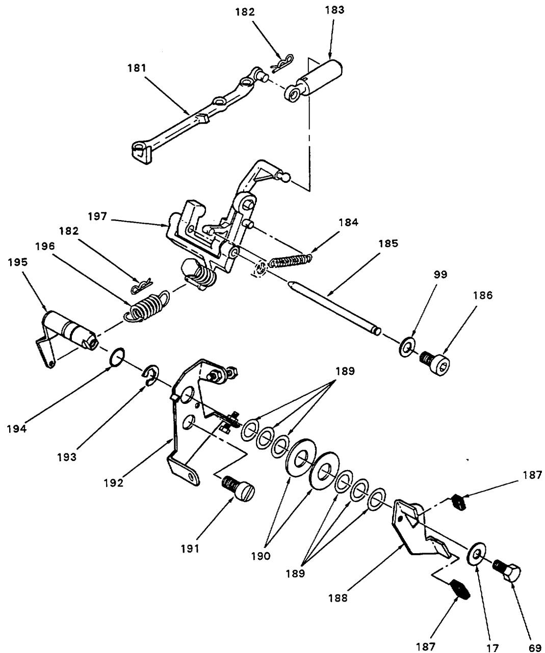
Figure 10 (Sheet 10 of 13). Engine Assembly - Governor Assembly
