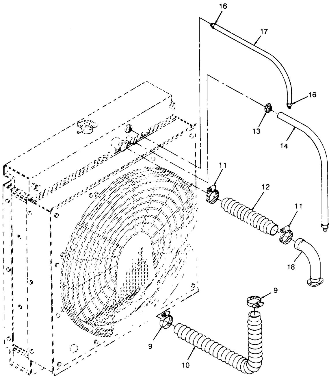
Figure 50. Radiator Assembly (Sheet 2 of 3)
