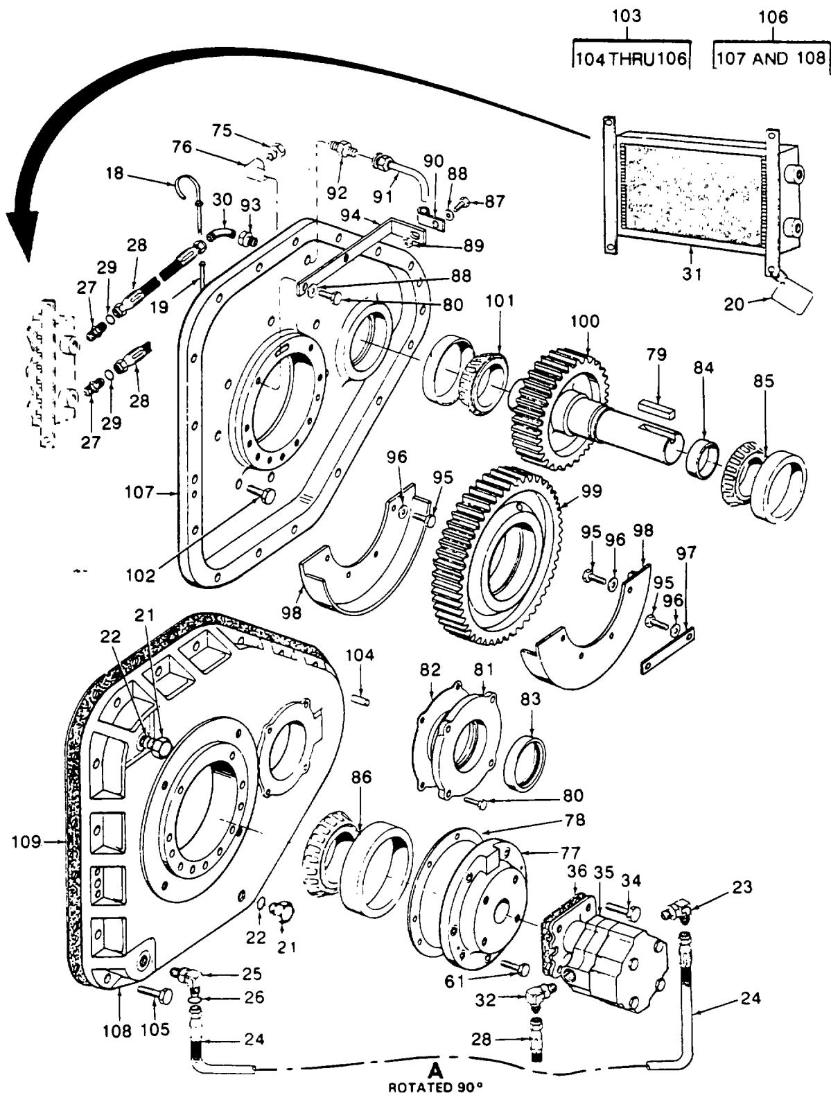
Figure 49. Speed Increaser (Sheet 2 of 3)
