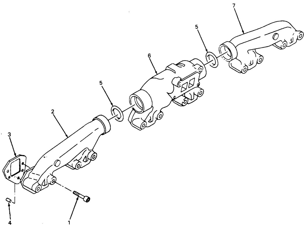
Figure 62. Exhaust Manifold
