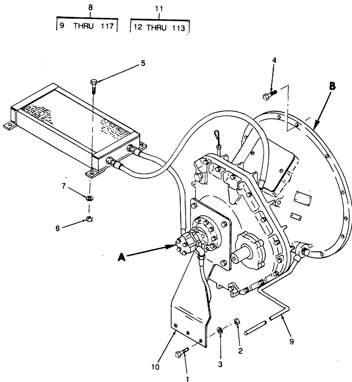
Figure 49. Speed Increaser (Sheet 1 of 3)
