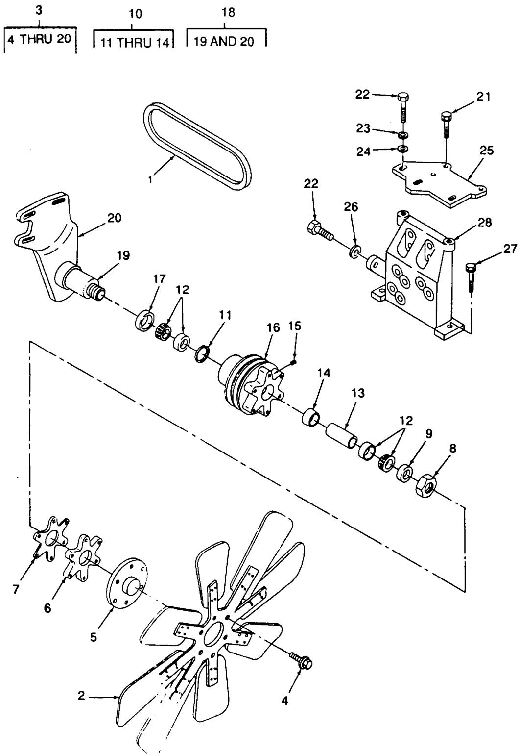
Figure 64. Fan Hub and Fan Bracket
