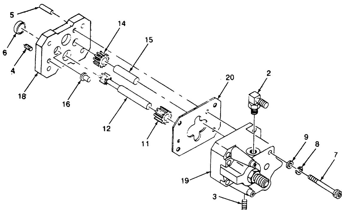
Figure 72. Gear Pump
