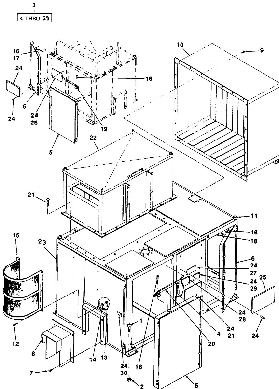
Figure 7. Engine Enclosure
