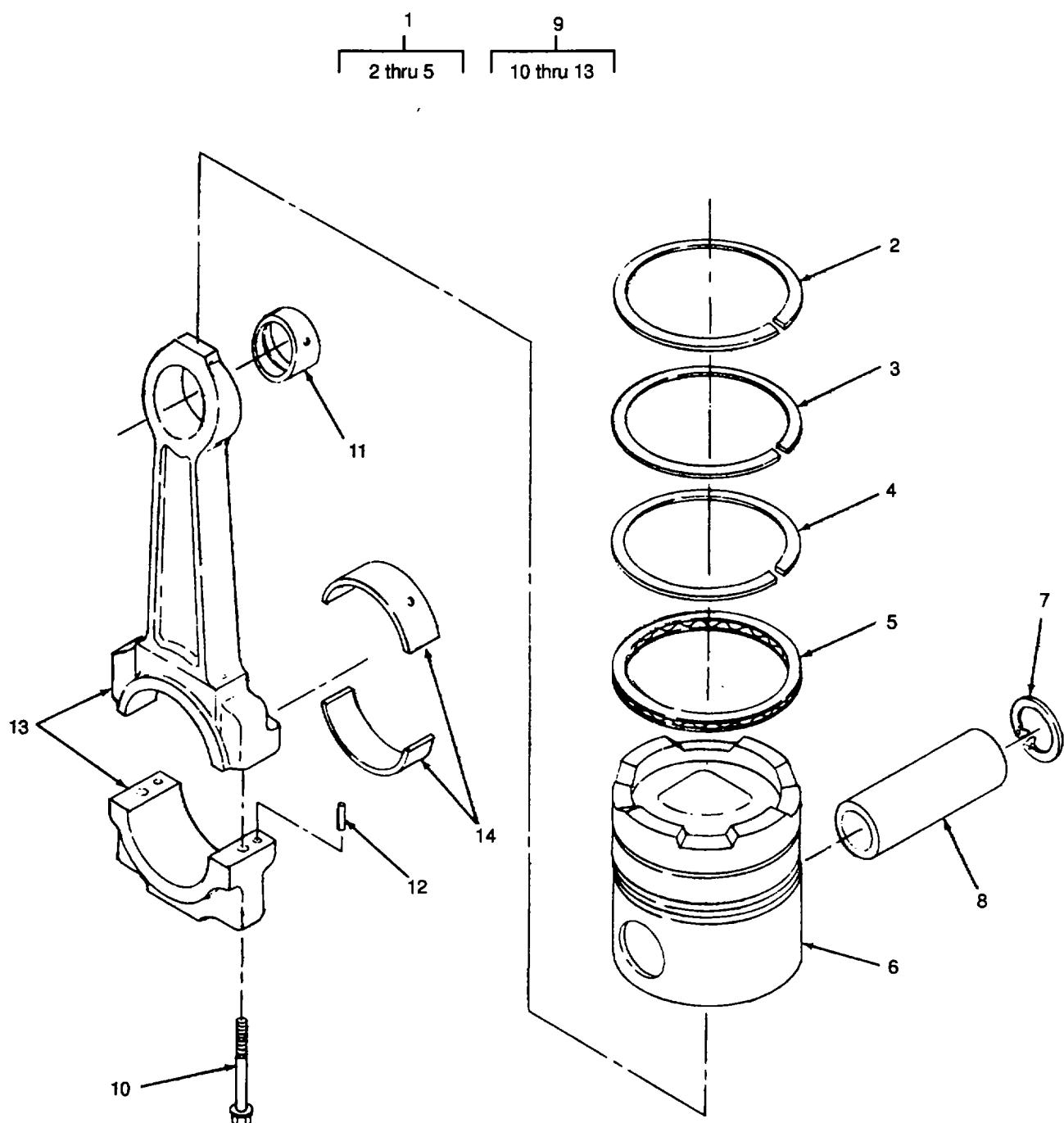
Figure 89. Connecting Rod and Piston.
