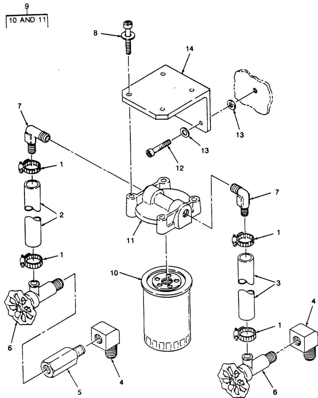
Figure 60. Corrosion Resistor
