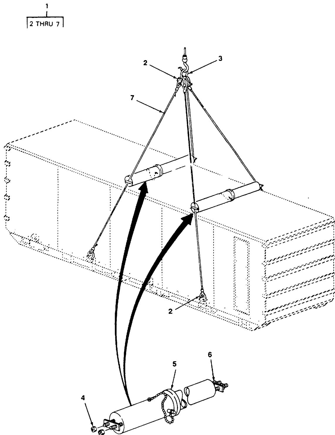
Figure 3. Bail Lifting Assembly
