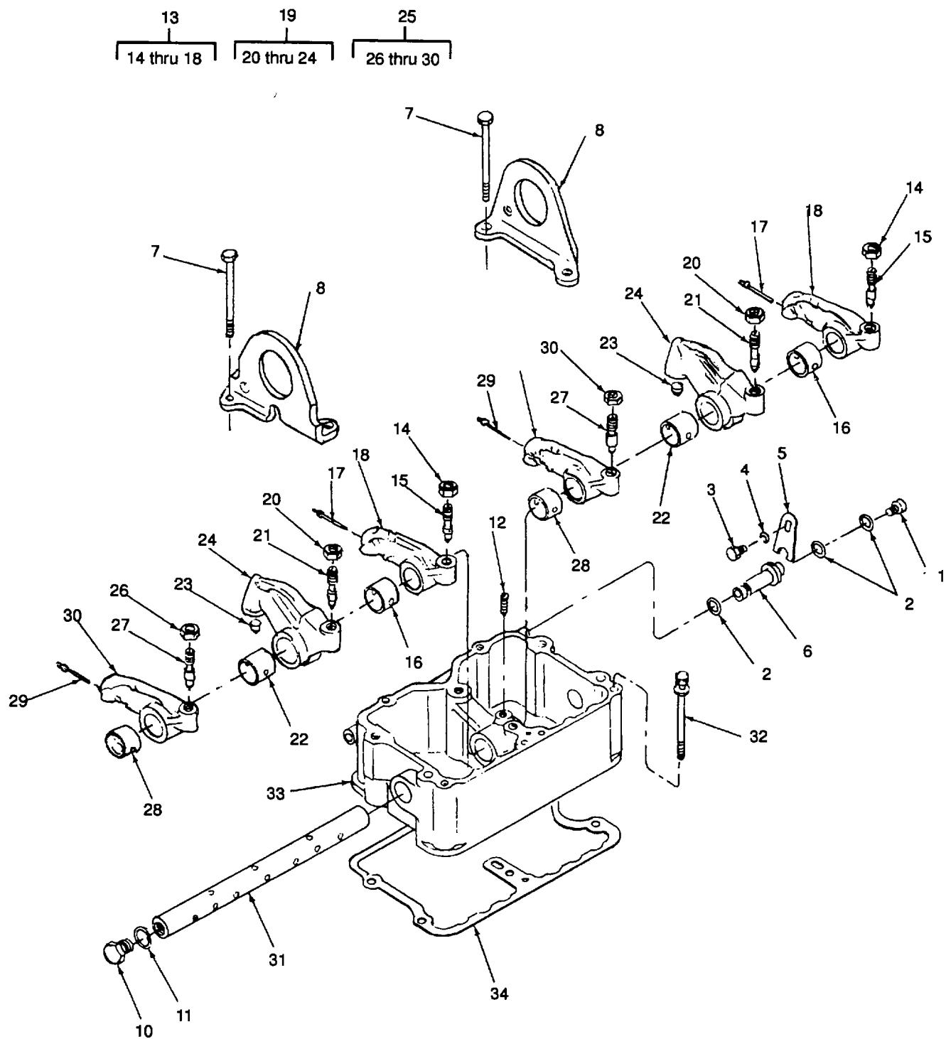
Figure 80. Rocker Lever Housing.
