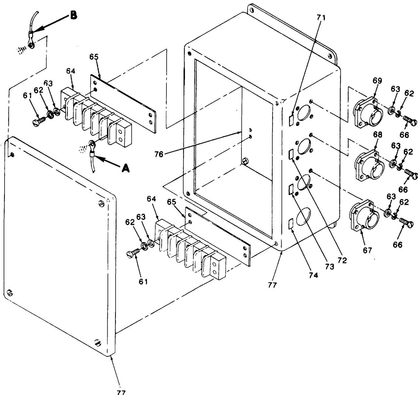
Figure 18. Junction Box No. 1 (Sheet 1 of 2)
