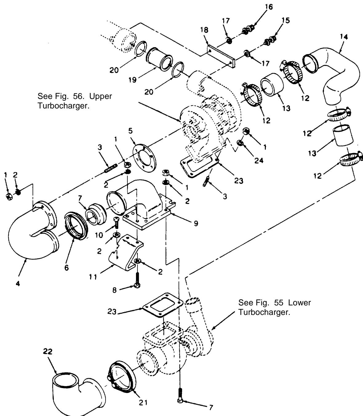
Figure 54. Turbocharger Mounting
