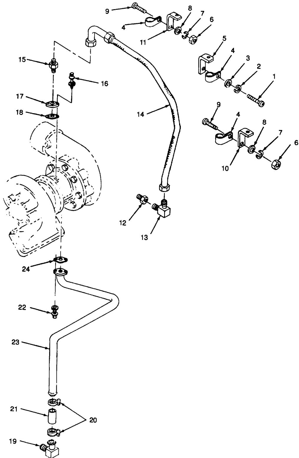
Figure 53. Turbocharger Plumbing (Sheet 1 of 2).
