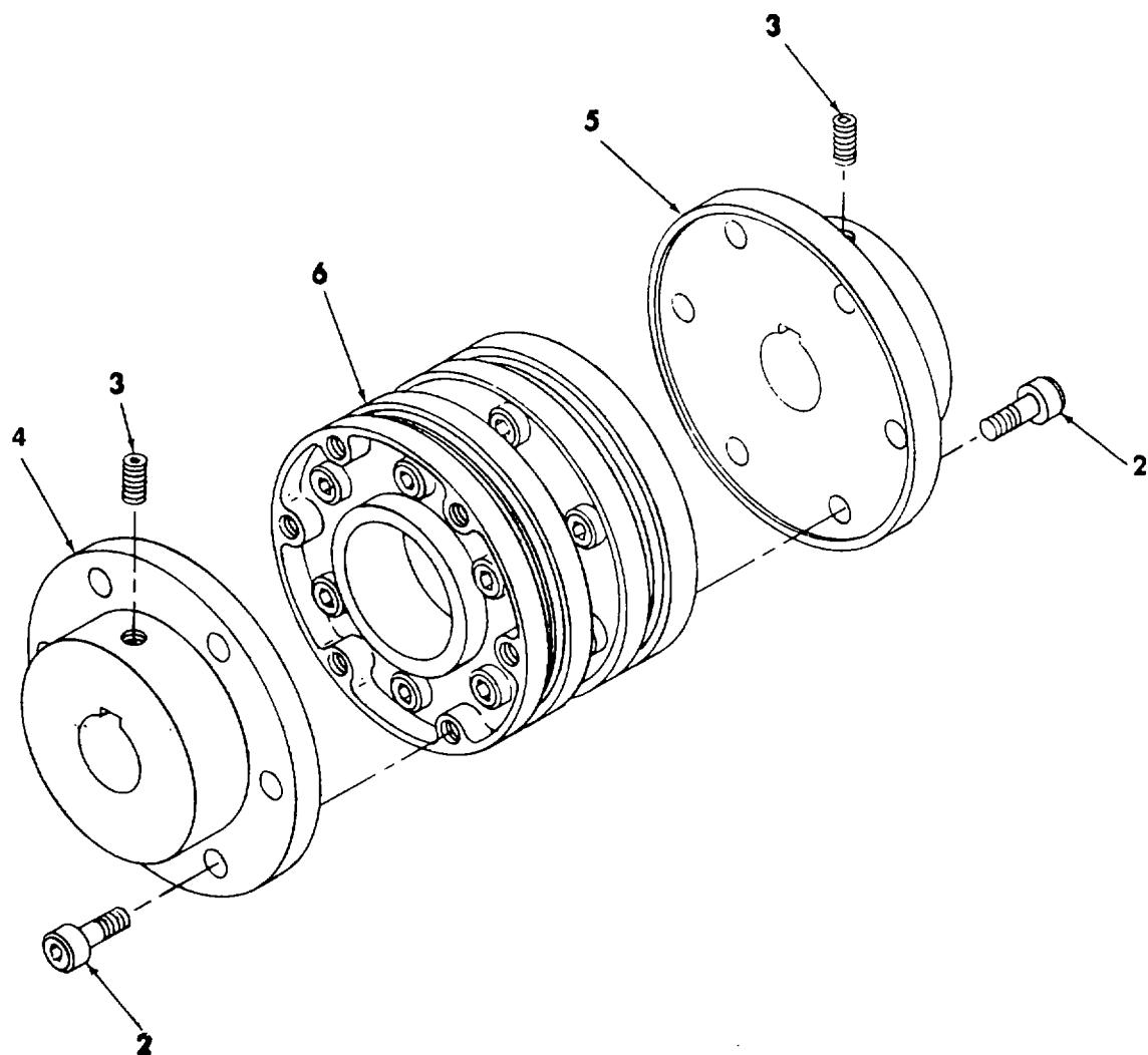
Figure 8. Flexible Coupling
