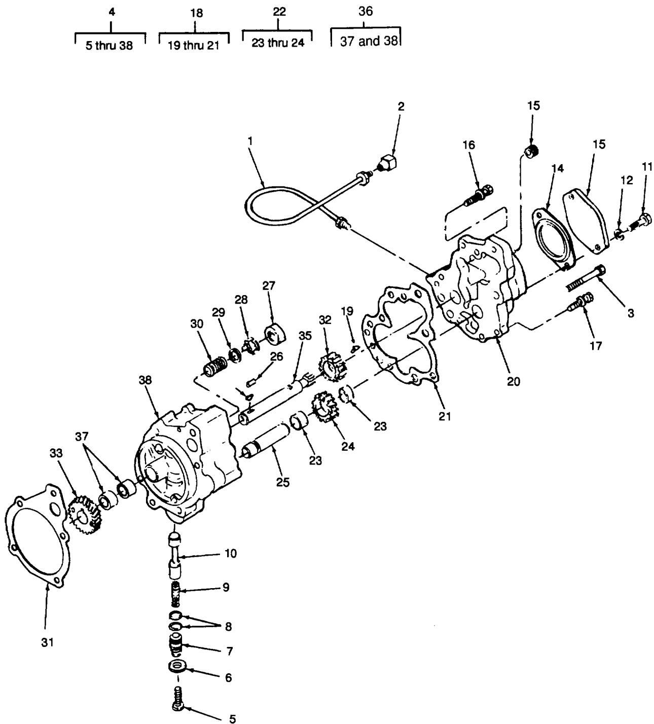
Figure 77. Lube Oil Assembly.
