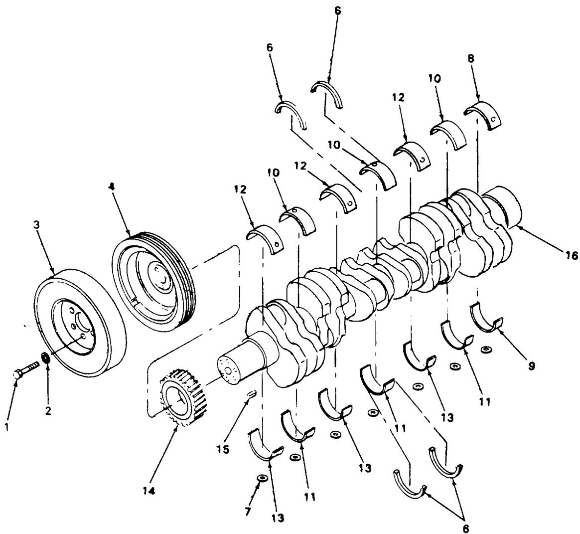
Figure 90. Crankshaft
