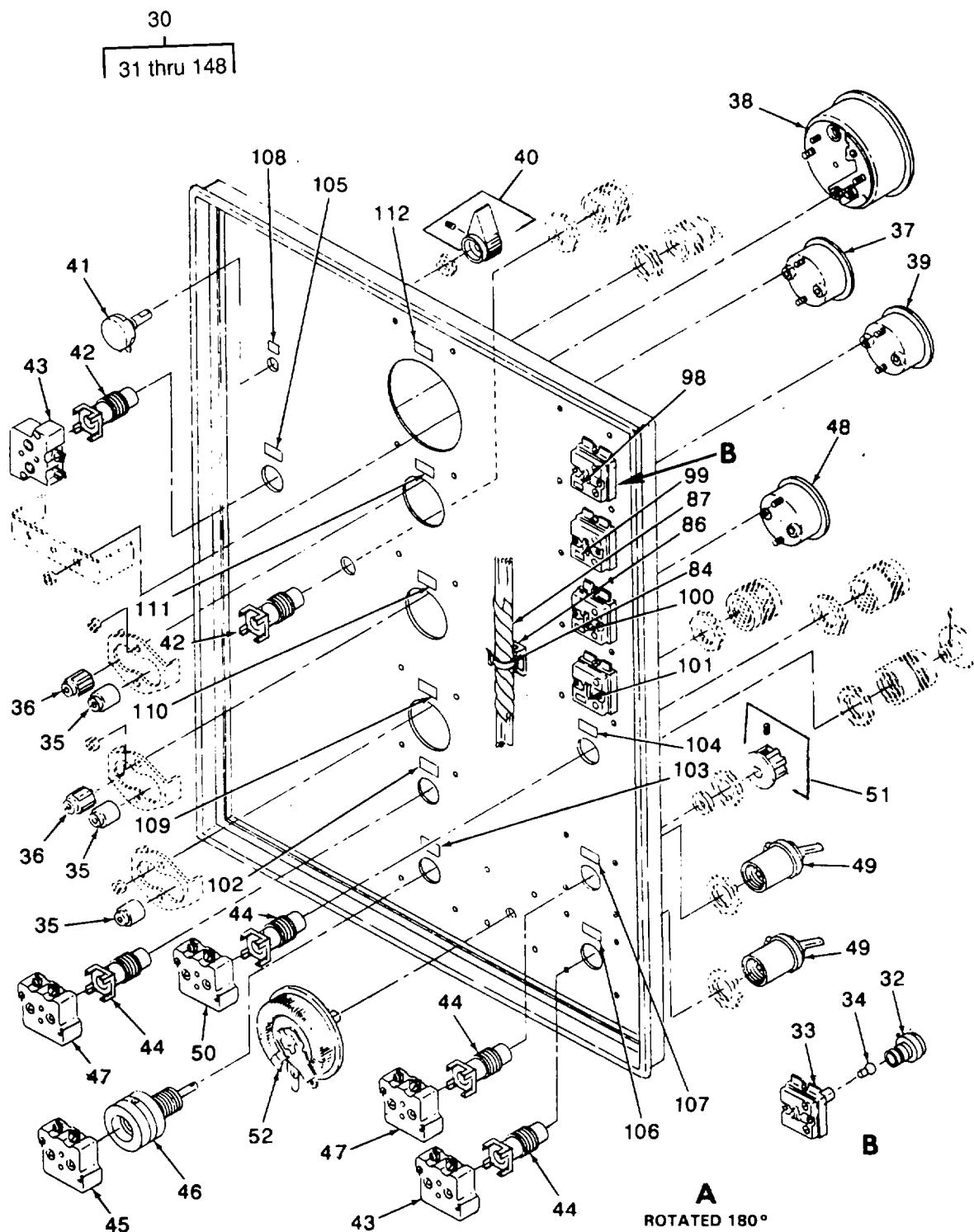
Figure 13. Control Panel Assembly (Sheet 2 of 3)
