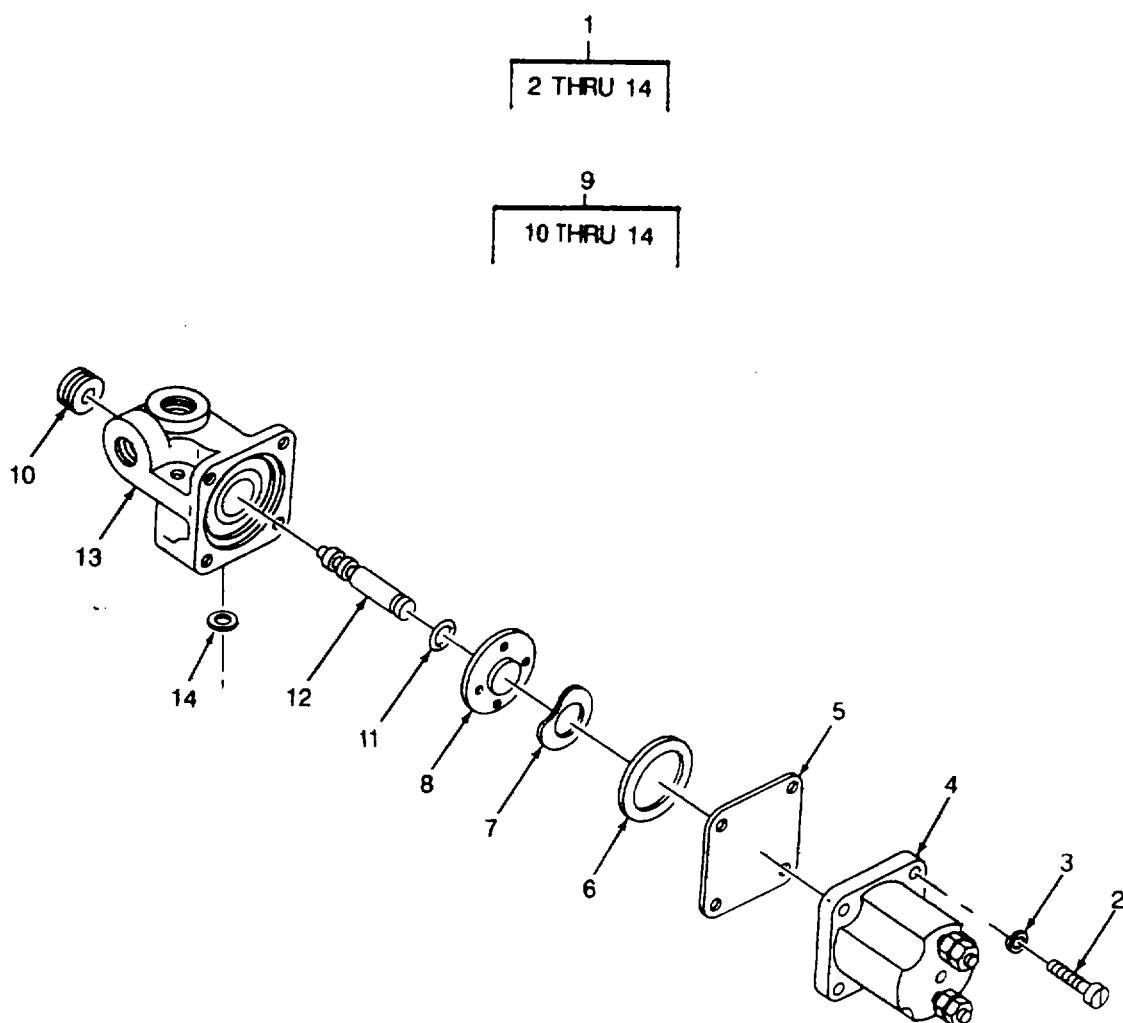
Figure 71. Shutoff Valve
