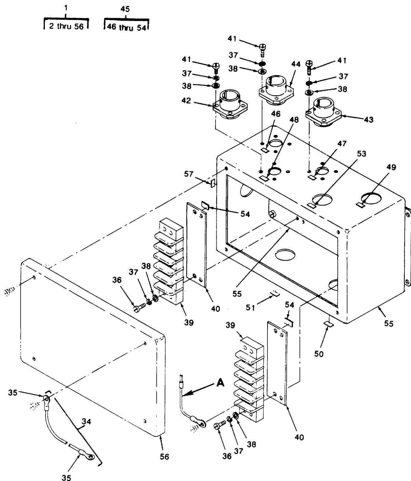
Figure 19. Junction Box No. 2 (Sheet 1 of 2)
