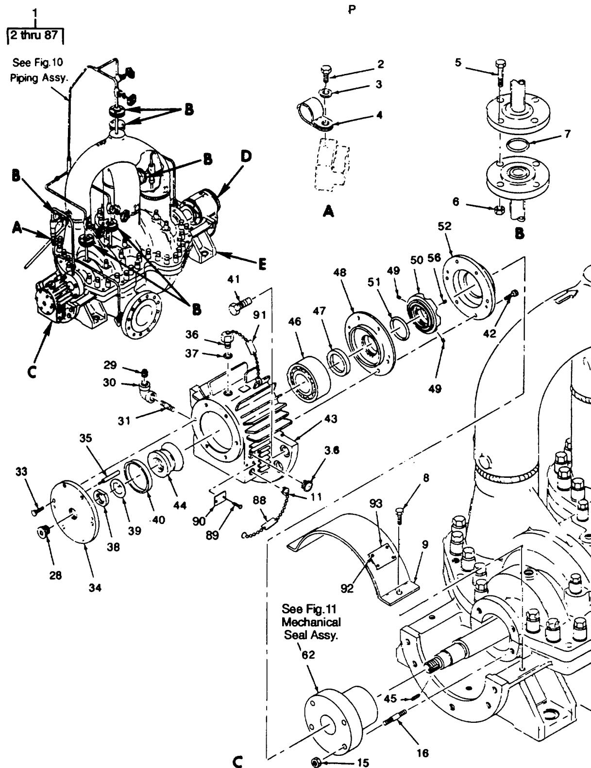
Figure 9. Pump Assembly (Sheet 1 of 4)
