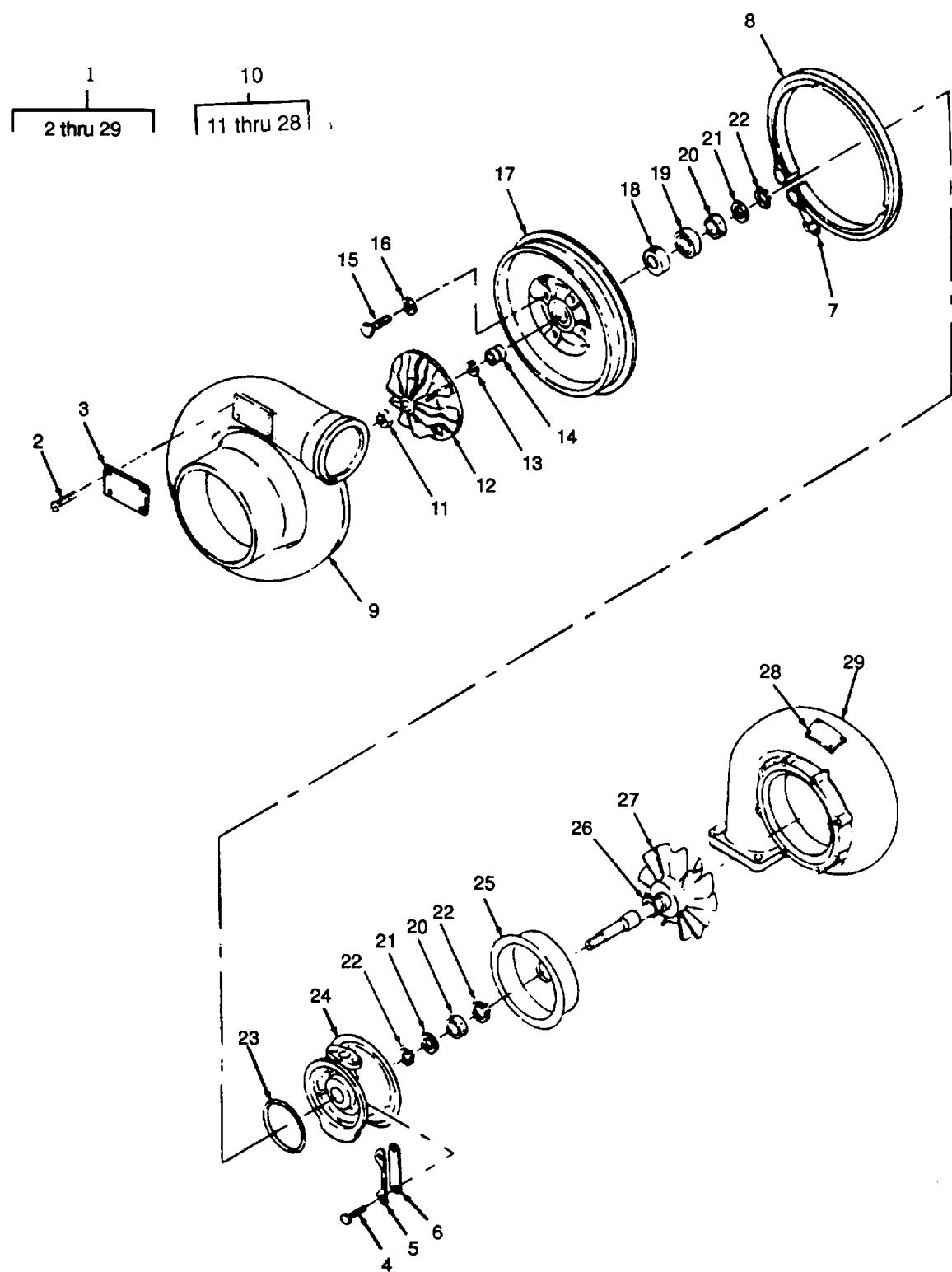
Figure 55. Lower Turbocharger.
