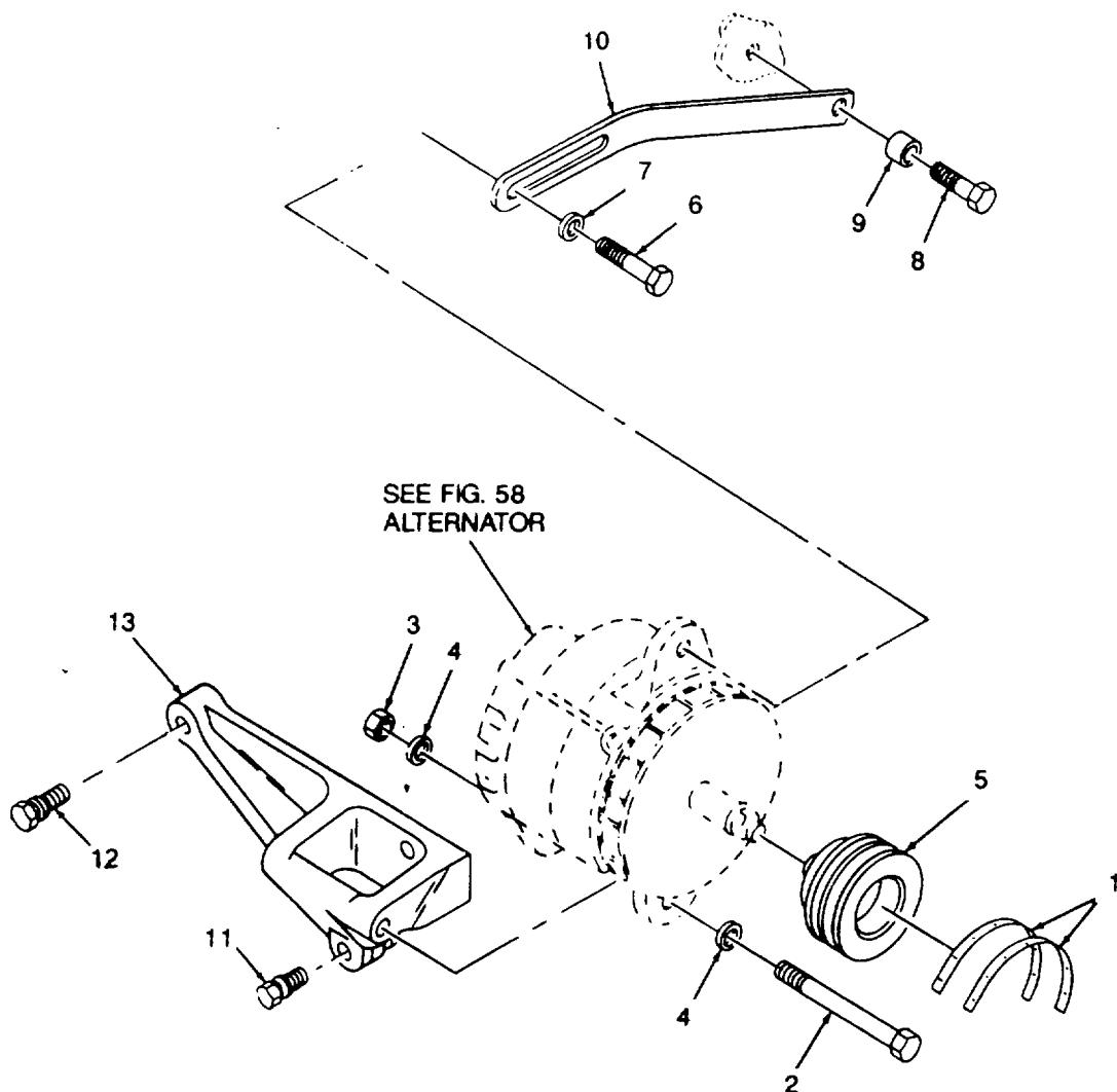
Figure 57. Alternator Mounting
