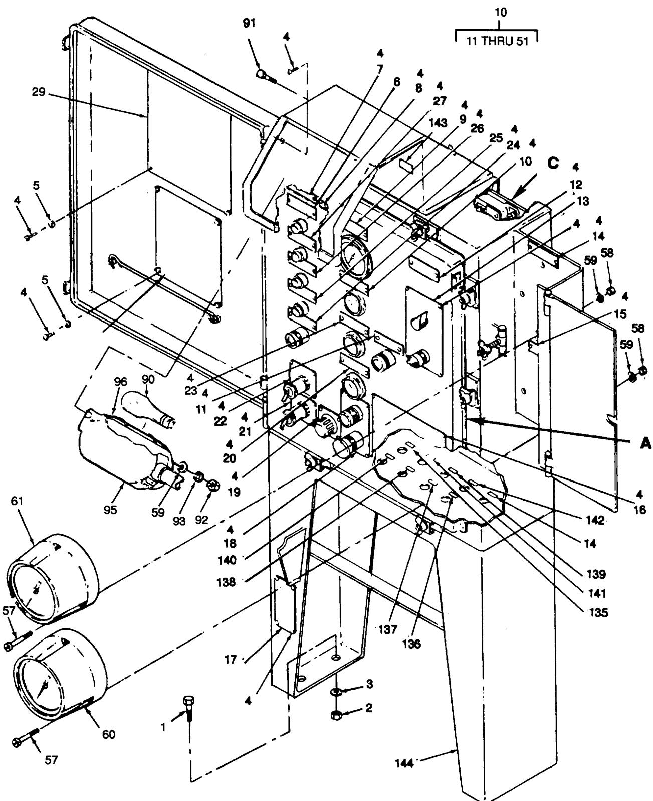
*Figure 13. Control Panel Assembly (Sheet 1 of 3).*
