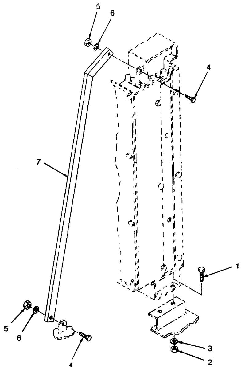
Figure 50. Radiator Assembly (Sheet 1 of 3)
