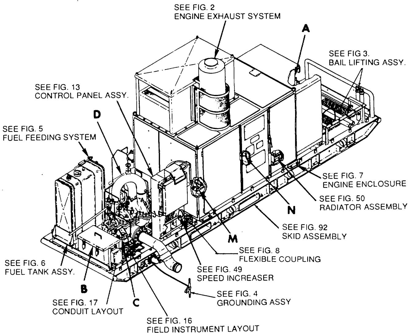
Figure 1. Pumping Assembly, 800 GPM, Mainline (Sheet 1 of 2).
