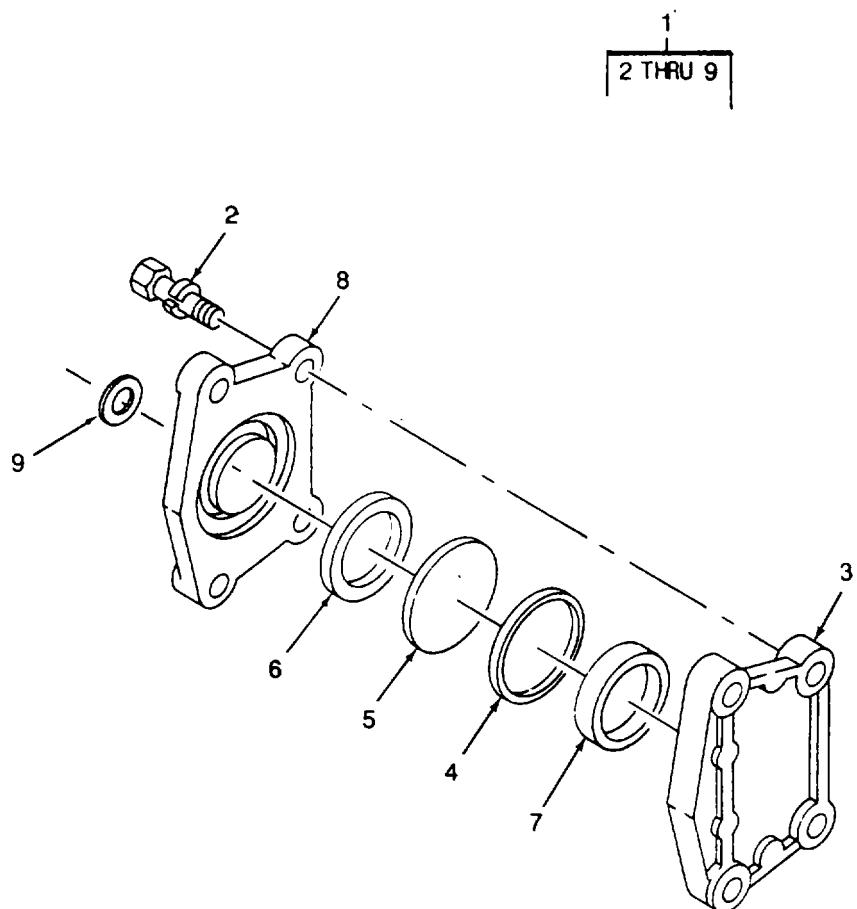
Figure 70. Fuel Pump Damper
