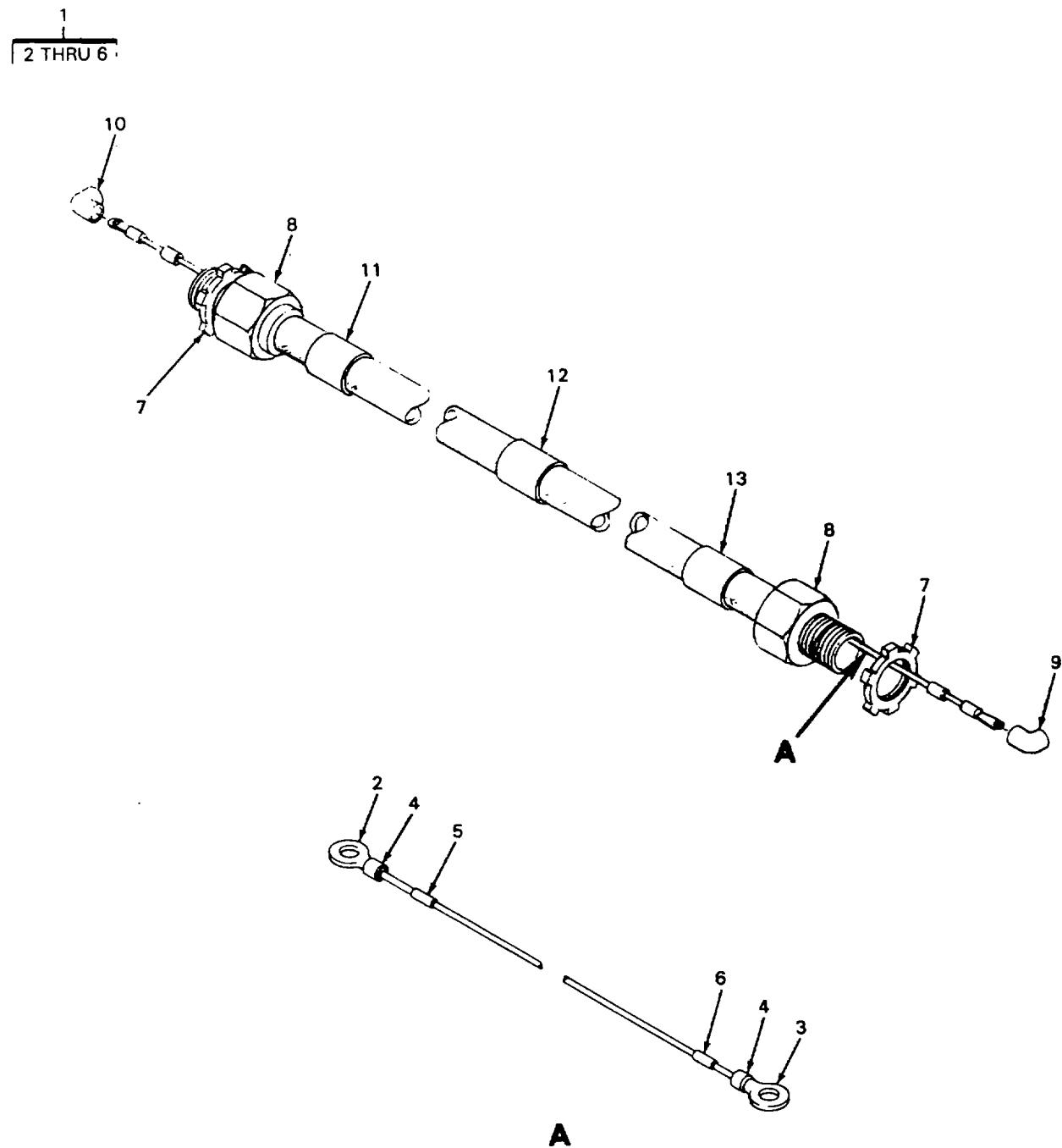
Figure 33. Cable Connection C014
