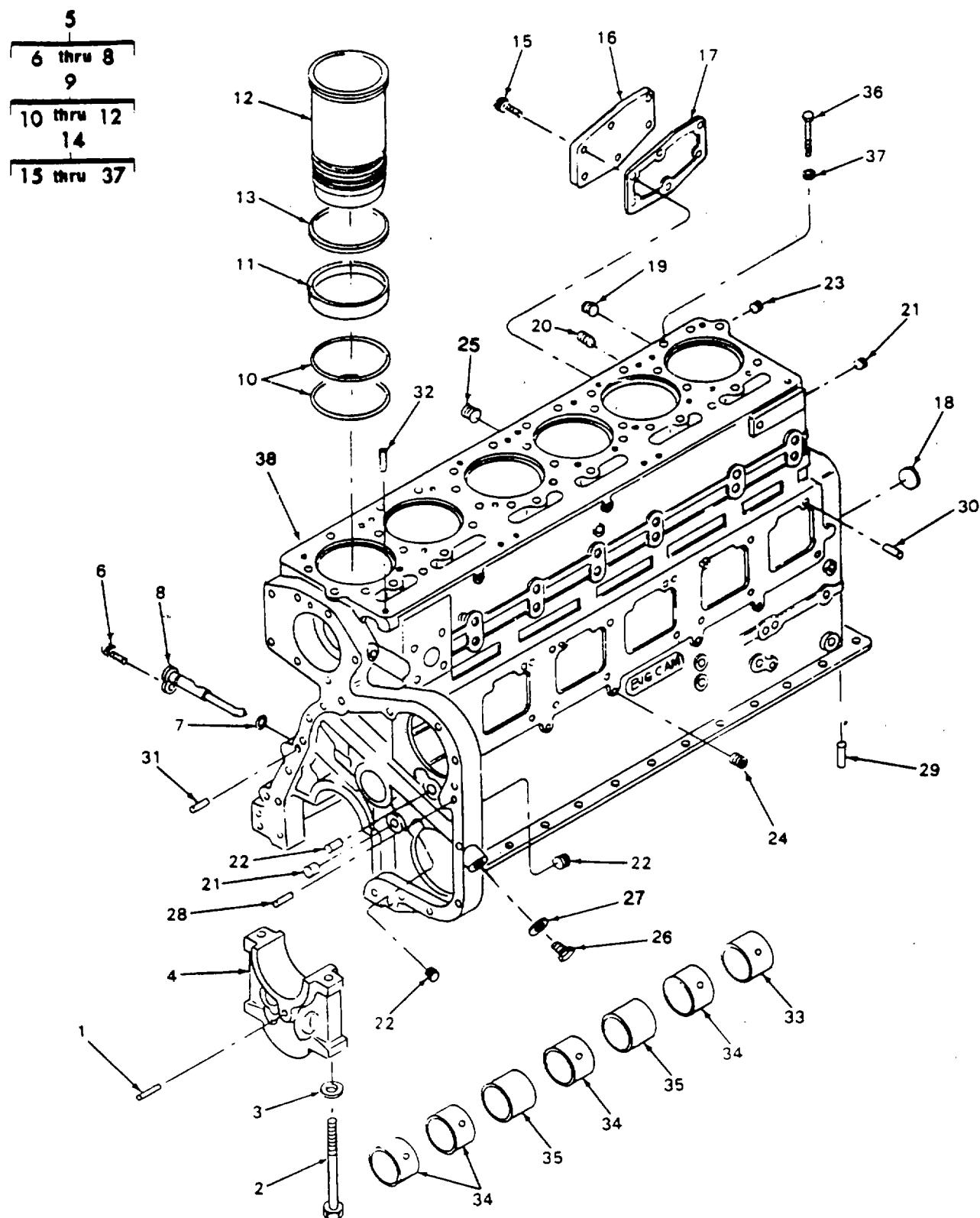
Figure 91. Cylinder Block
