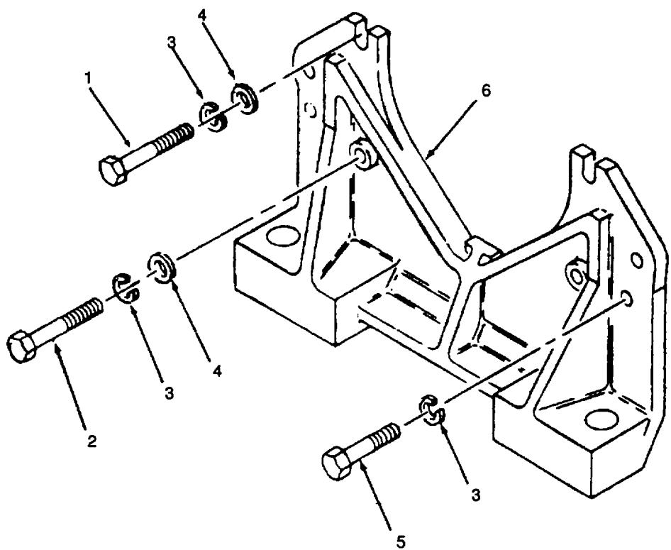
Figure 86. Front Engine Support.
