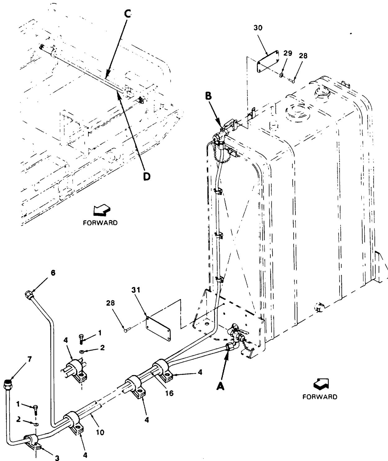
Figure 5. Fuel Feeding System (Sheet 1 of 2)
