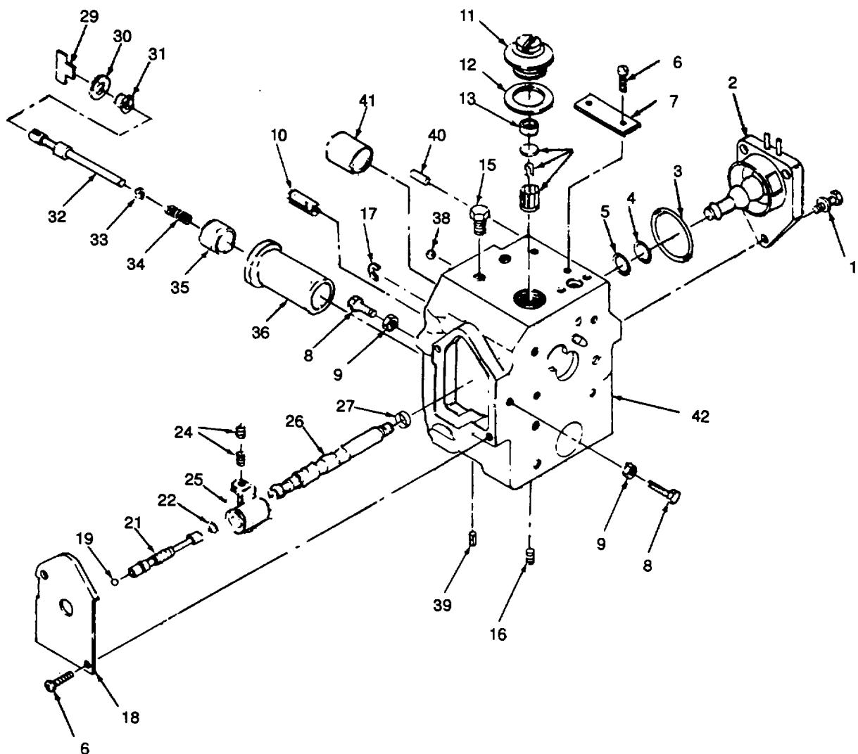
Figure 75. Fuel Pump Housing.
