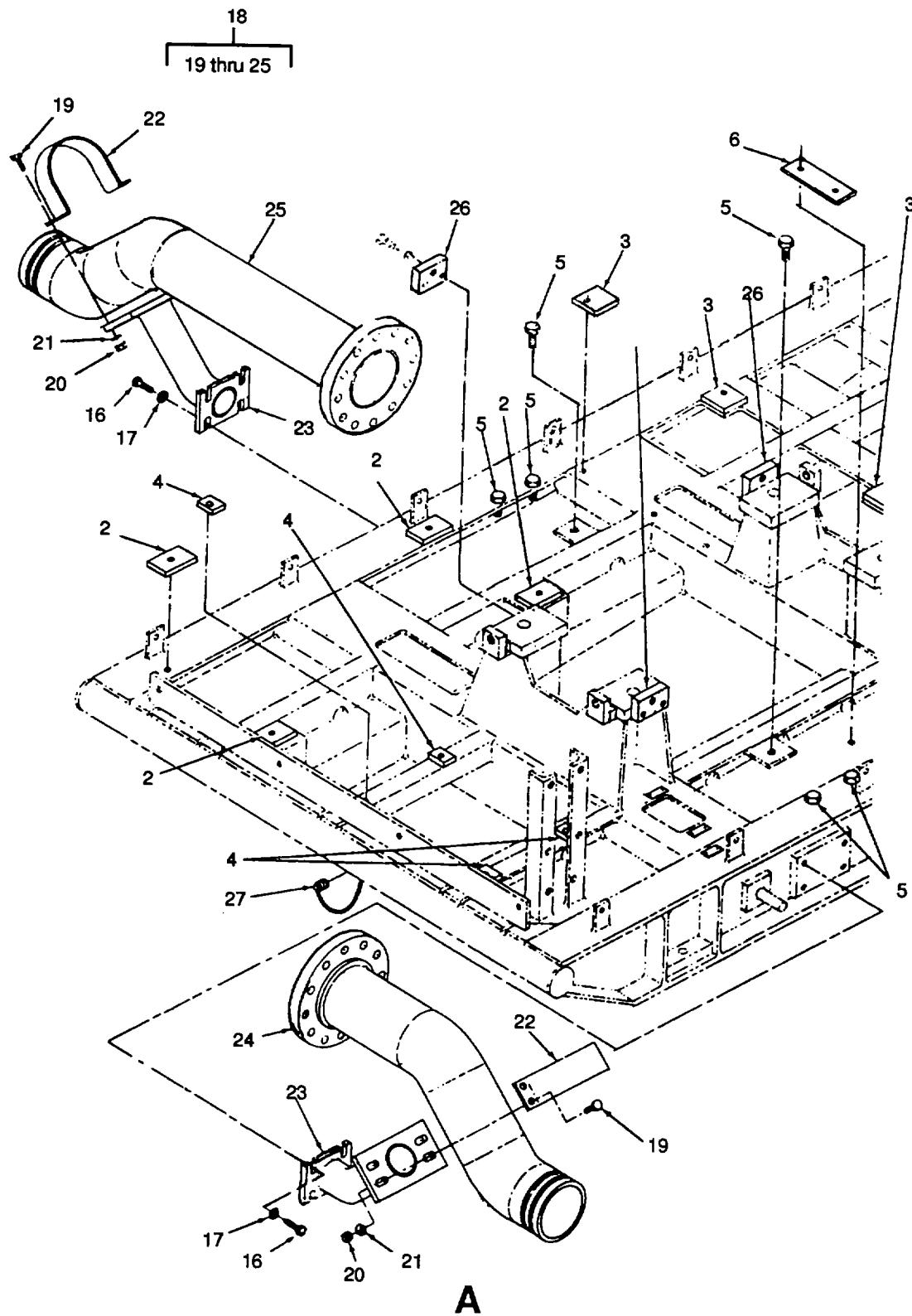
Figure 92. Skid Assembly (Sheet 2 of 4).
