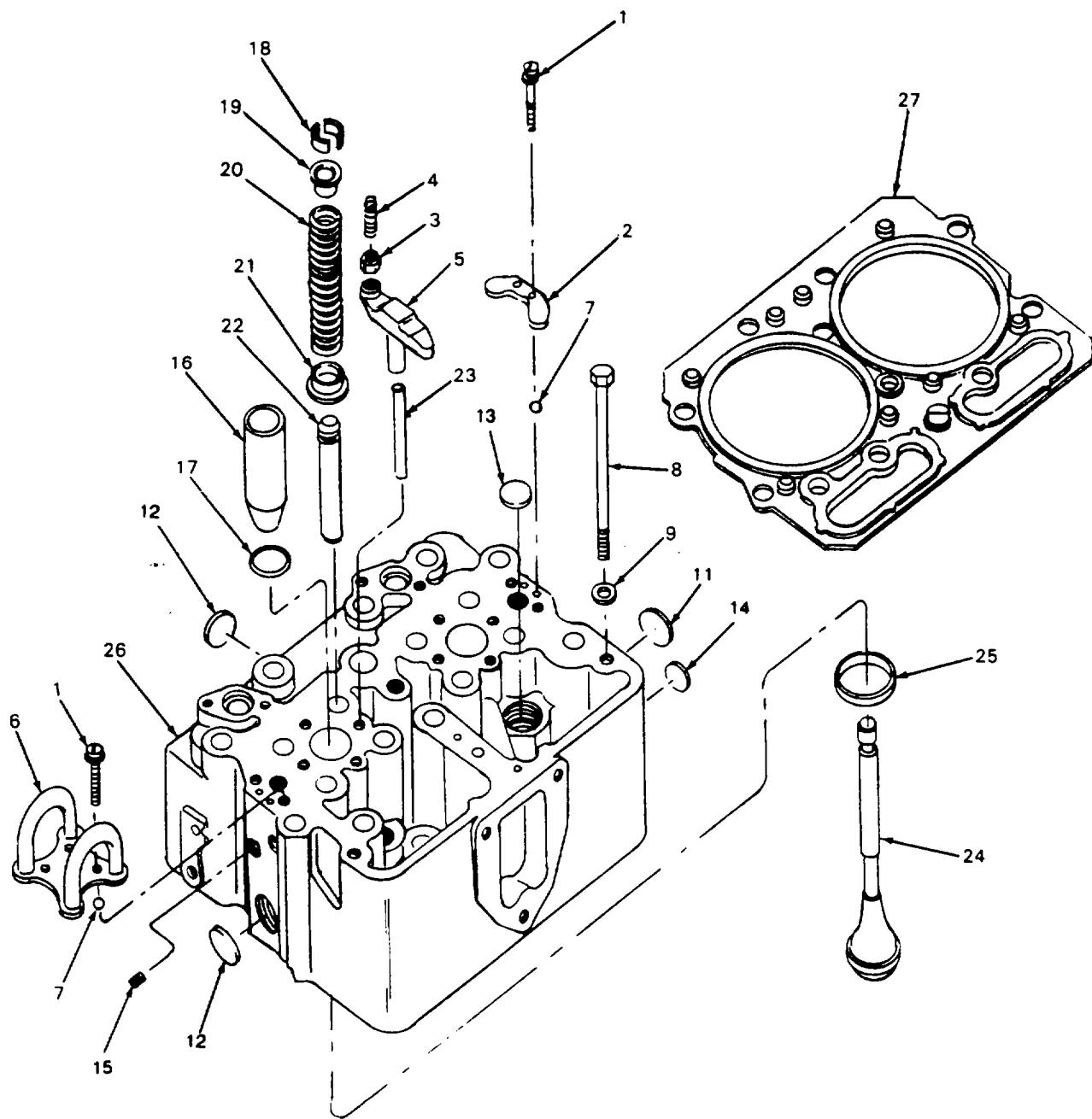
Figure 83. Cylinder Head
