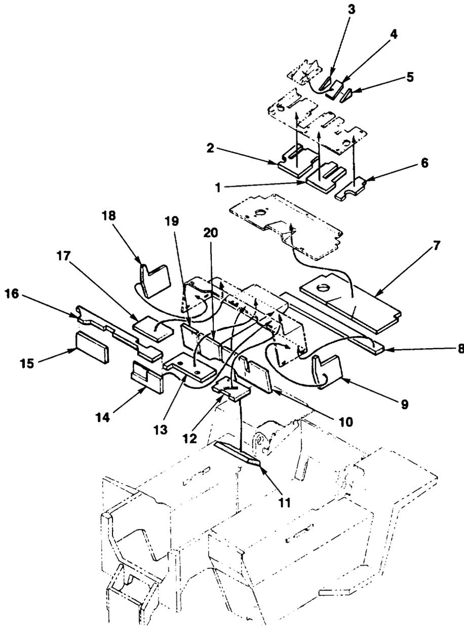
FIG. 107. INSULATION INSTALLATION
