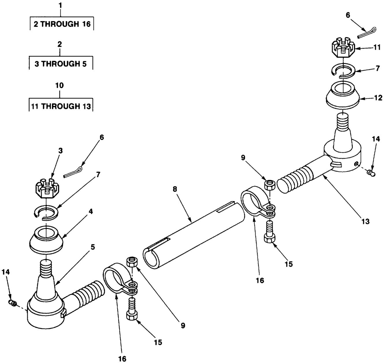
FIG. 95. TIE ROD ASSEMBLY
