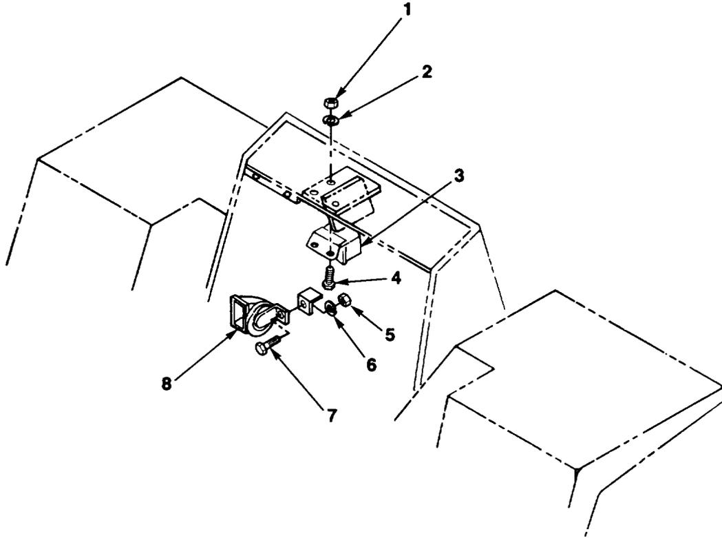
FIG. 49. HORN INSTALLATION
