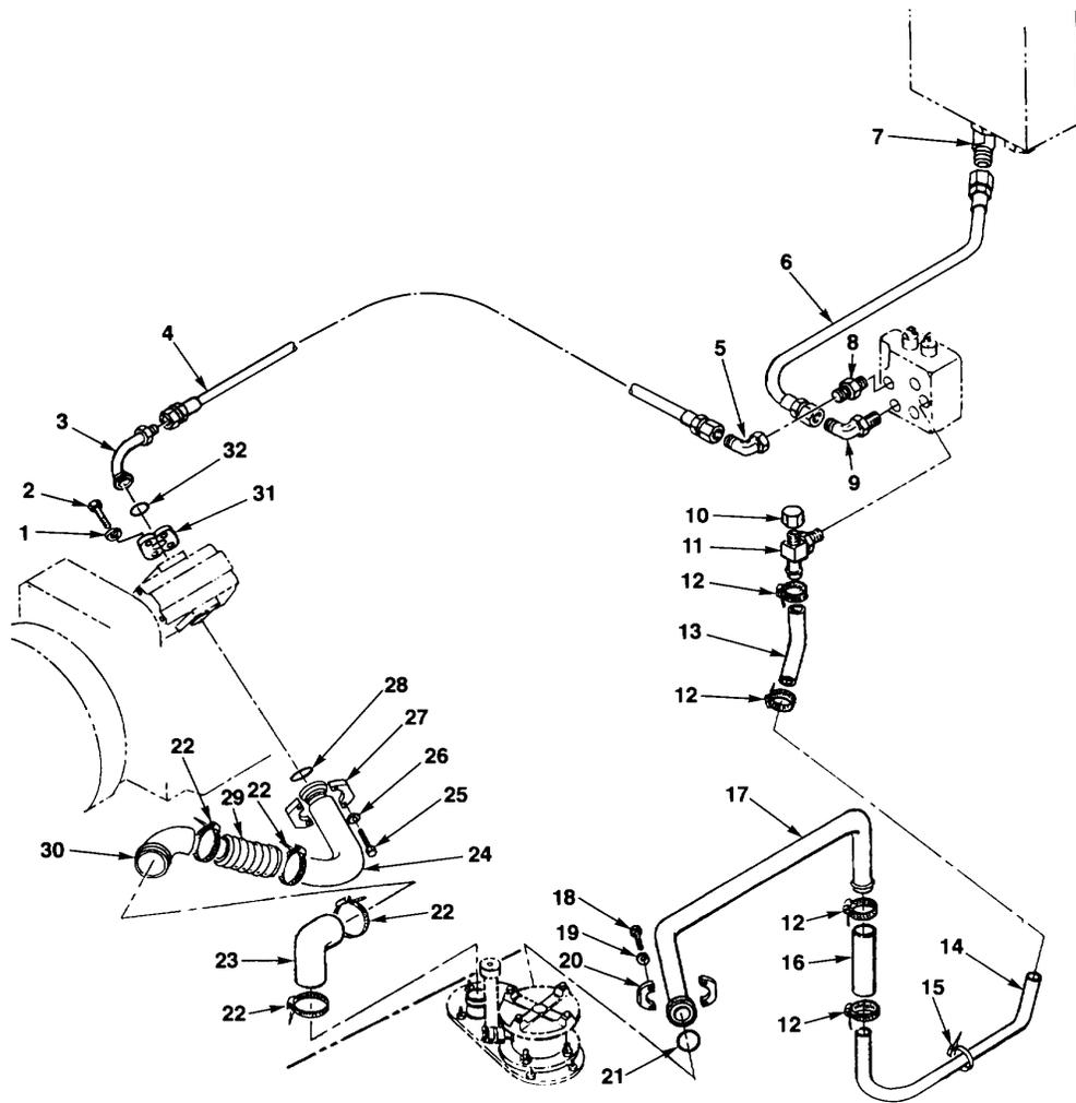
FIG. 139. MAIN HYDRAULIC LINES AND FITTINGS
