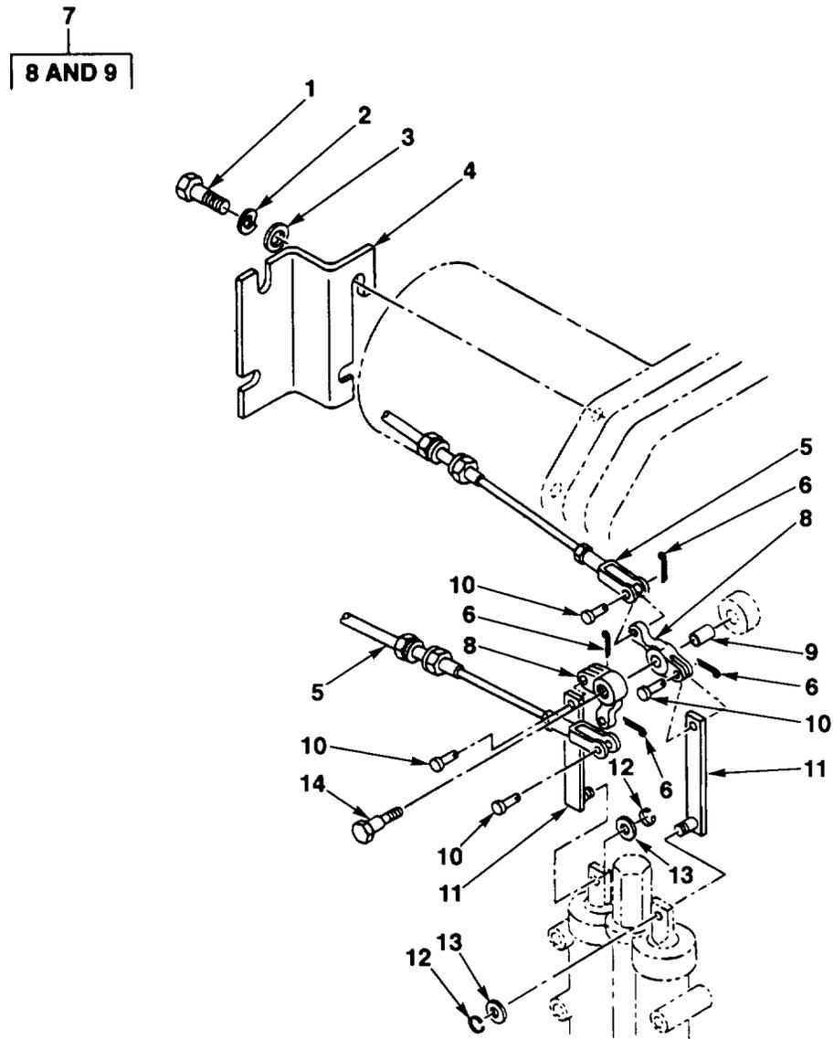
FIG. 56. DIRECTIONAL AND SHIFT CABLE LINKAGE
