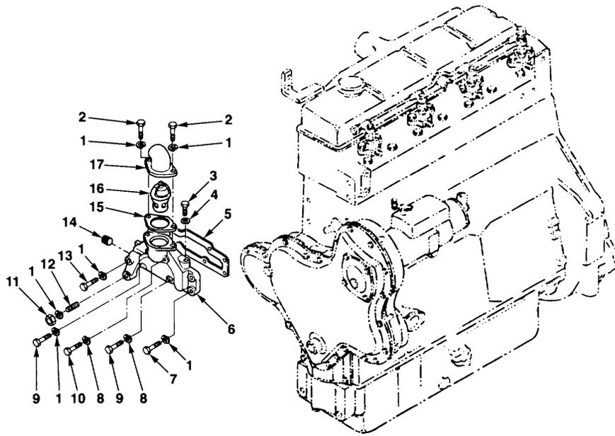
FIG. 35. THERMOSTAT HOUSING, HOSES AND FITTINGS
