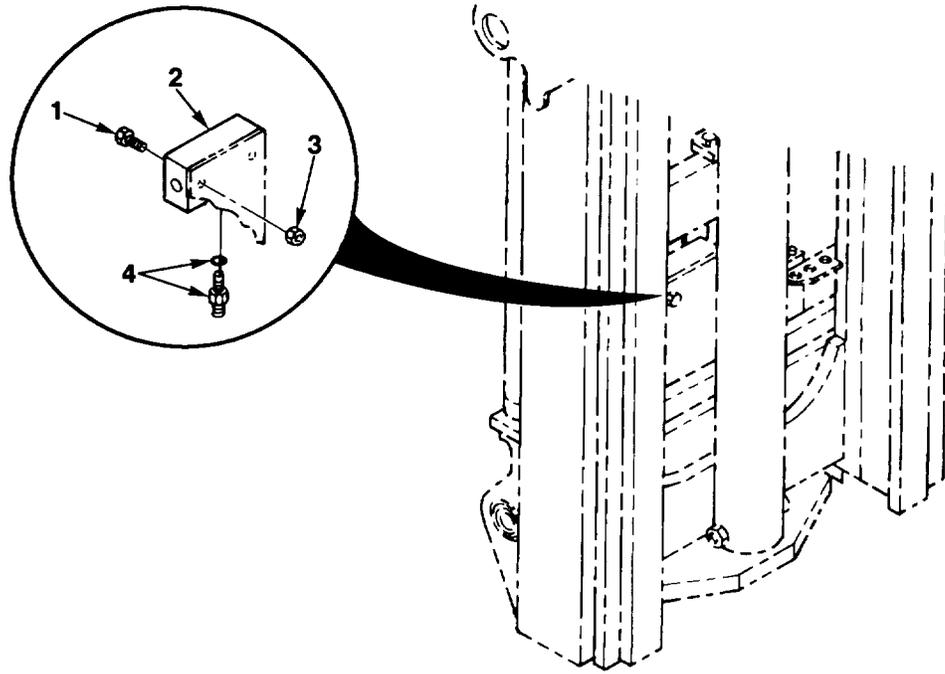
FIG. 127. LOWERING CONTROL VALVE INSTALLATION
