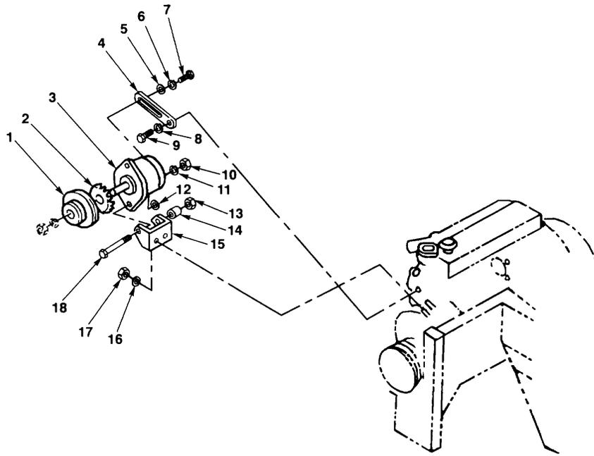
FIG. 39. ALTERNATOR MOUNTING
