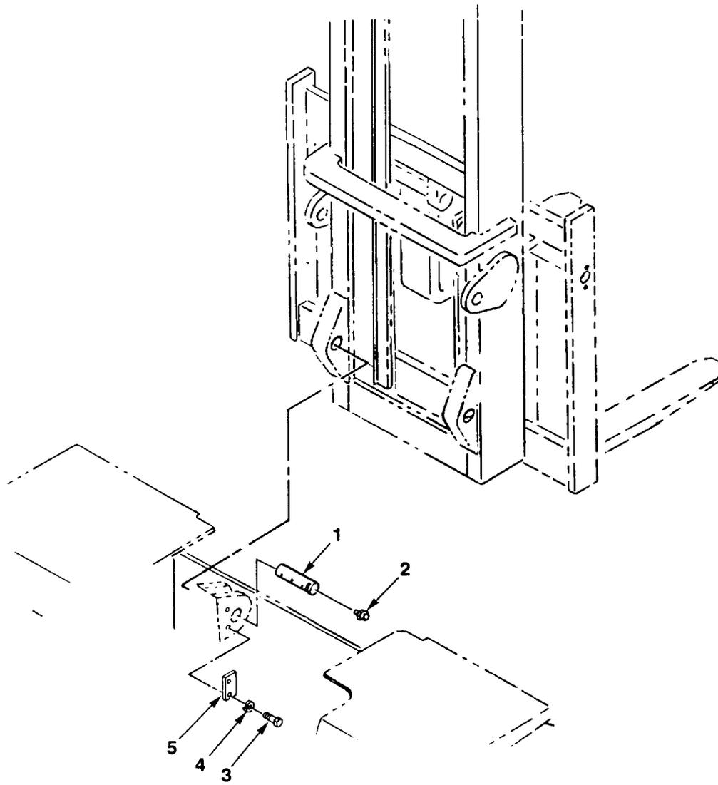
FIG. 116. MAST AND CARRIAGE INSTALLATION
