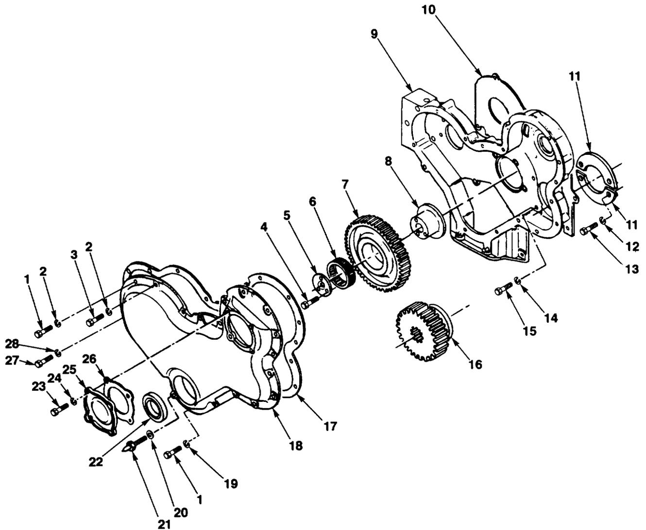
FIG. 10. TIMING GEAR COVER AND IDLER GEAR
