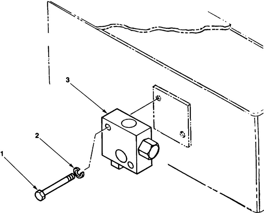
FIG. 123. PRIORITY VALVE ASSEMBLY
