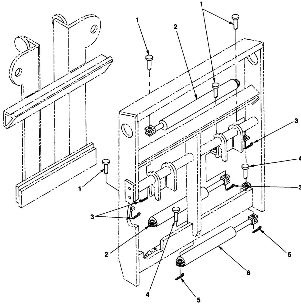
FIG. 133. CARRIAGE ASSEMBLY CYLINDER INSTALLATION
