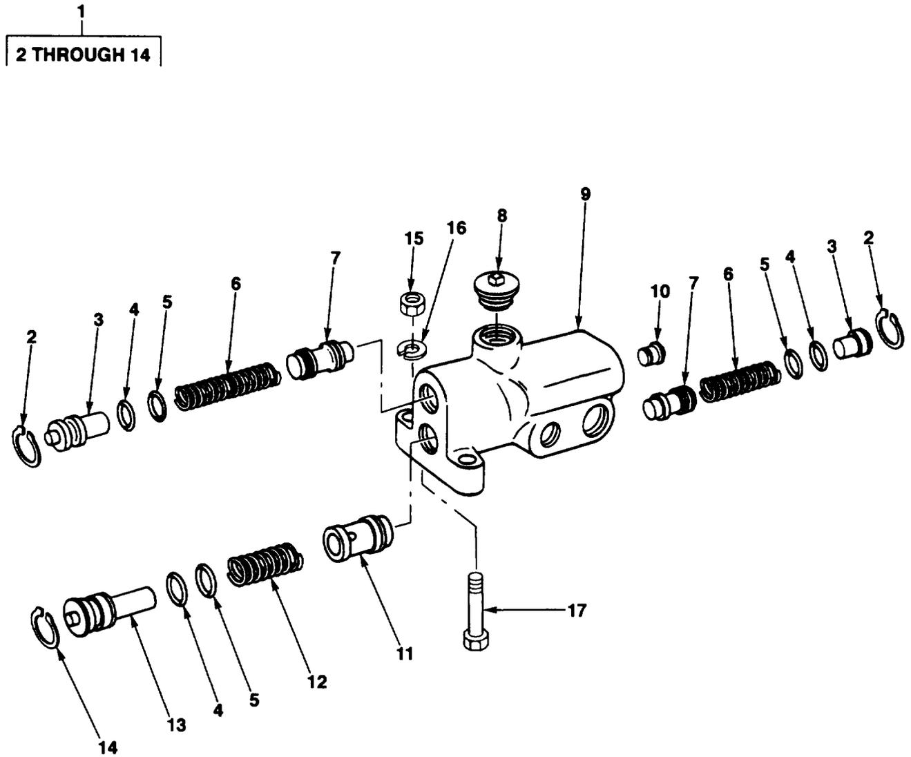
FIG. 122. TILT LOCK VALVE ASSEMBLY
