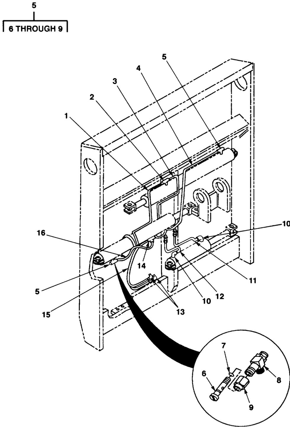
FIG. 141. CARRIAGE ASSEMBLY LINES AND FITTINGS
