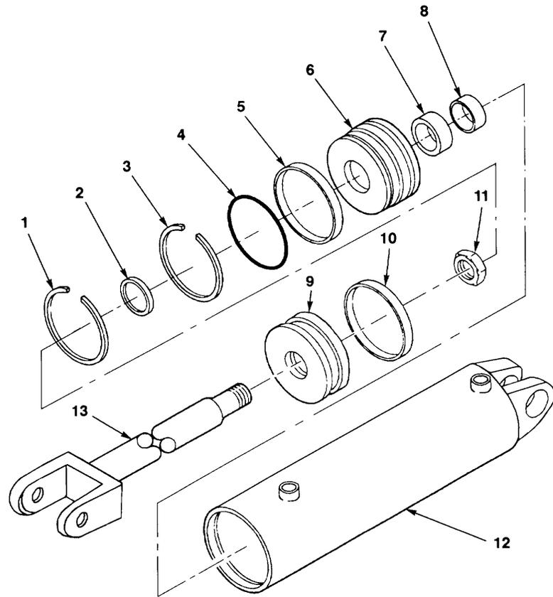
FIG. 134. CARRIAGE SIDE SHIFT CYLINDER ASSEMBLY
