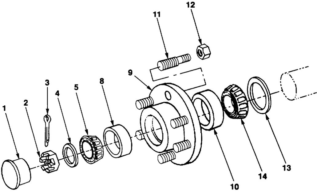
FIG. 90. STEERING AXLE HUB ASSEMBLY AND WHEEL BEARINGS
