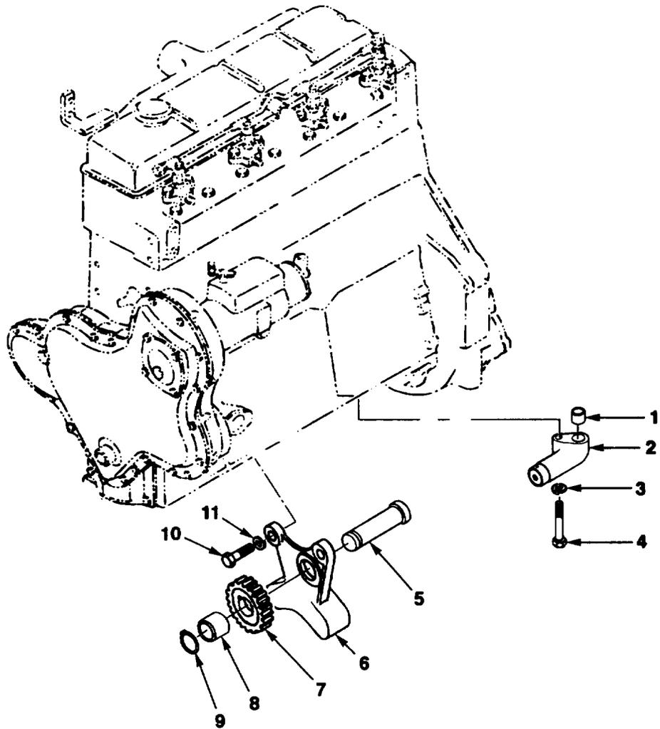
FIG. 15. OIL PUMP AND PRESSURE RELIEF VALVE
