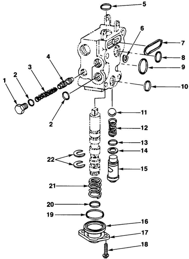
FIG. 125. INLET SECTION AUXILIARY CONTROL VALVE
