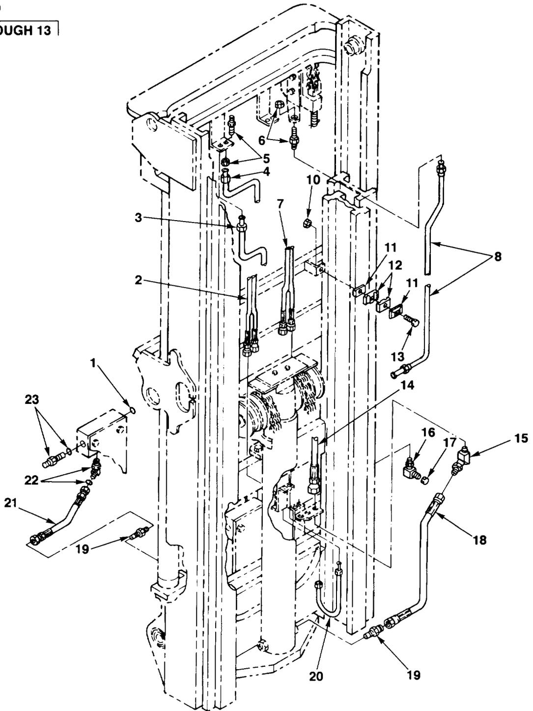
FIG. 145. THREE STAGE UPRIGHT ASSEMBLY LINES AND FITTINGS
