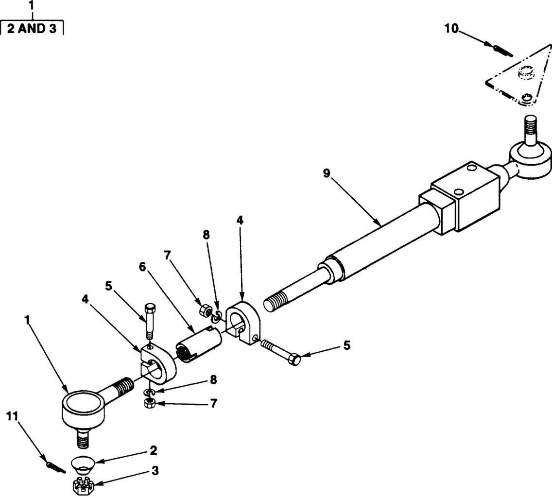
FIG. 98. STEERING CYLINDER INSTALLATION
