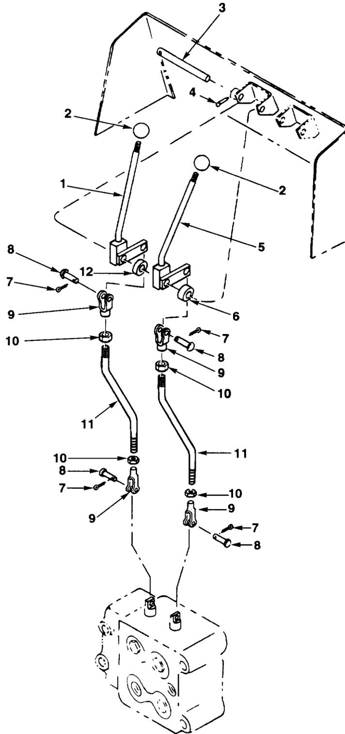
FIG. 128. MAIN CONTROL VALVE LEVERS AND LINKAGES
