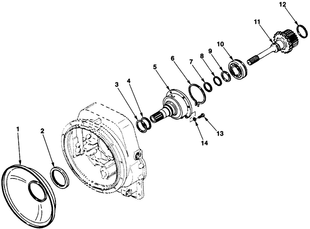
FIG. 62. TURBINE SHAFT, STATOR SUPPORT AND OIL BAFFLE
