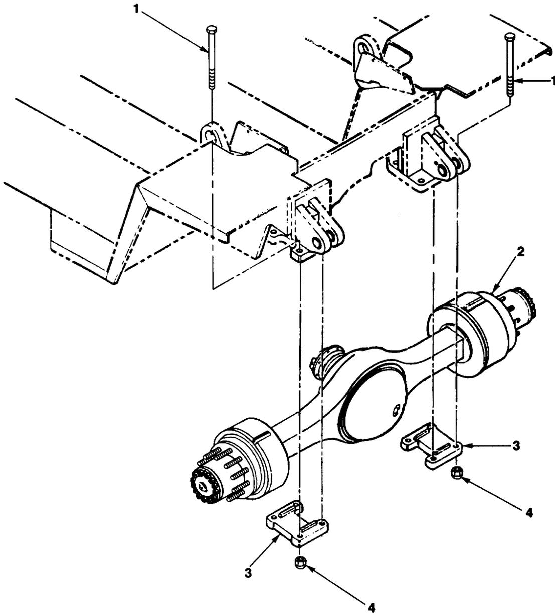
FIG. 74. DRIVE AXLE INSTALLATION
