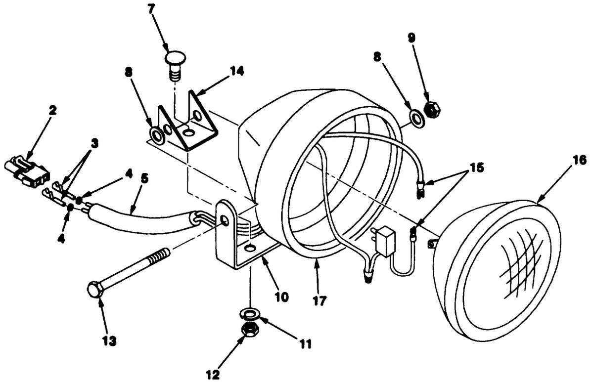
FIG. 46. FLOODLIGHT ASSEMBLY
