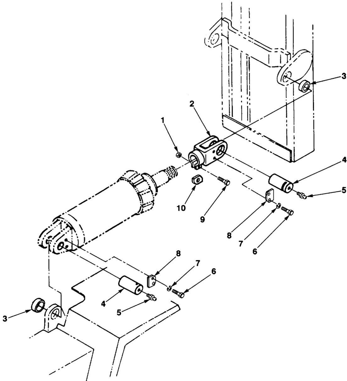
FIG. 130. TILT CYLINDER INSTALLATION
