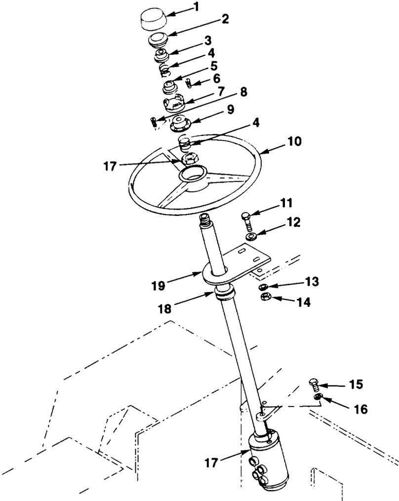
FIG. 93. HORN, STEERING WHEEL AND GEAR INSTALLATION
