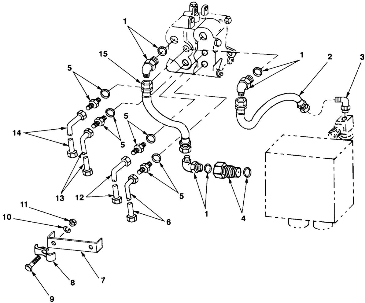
FIG. 142. AUXILIARY CONTROL VALVE LINES AND FITTINGS
