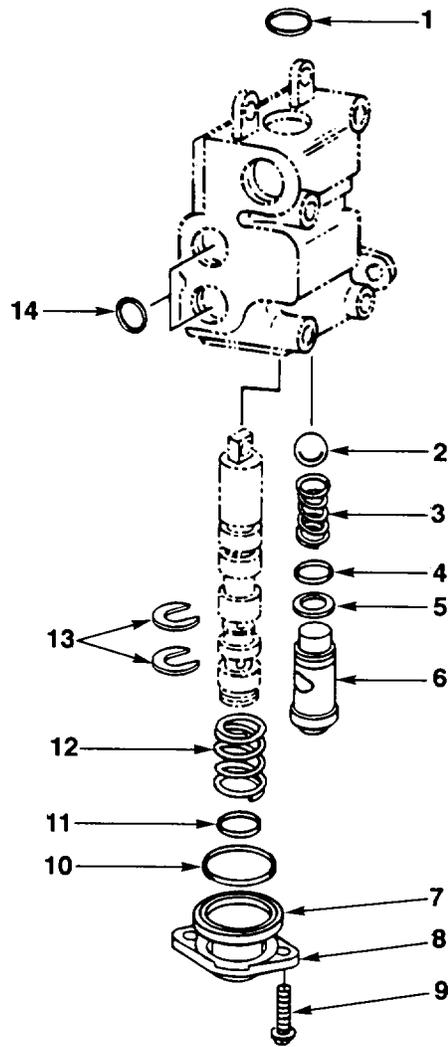
FIG. 126. OUTLET SECTION AUXILIARY CONTROL VALVE
