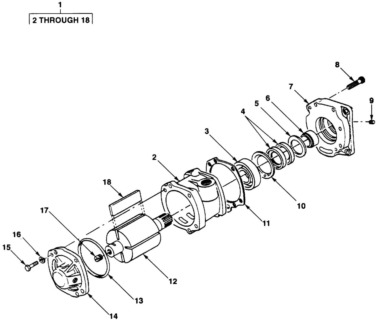
FIG. 84. ROTARY VACUUM PUMP ASSEMBLY
