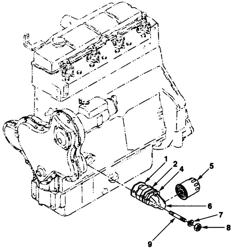
FIG. 13. ENGINE OIL FILTER
