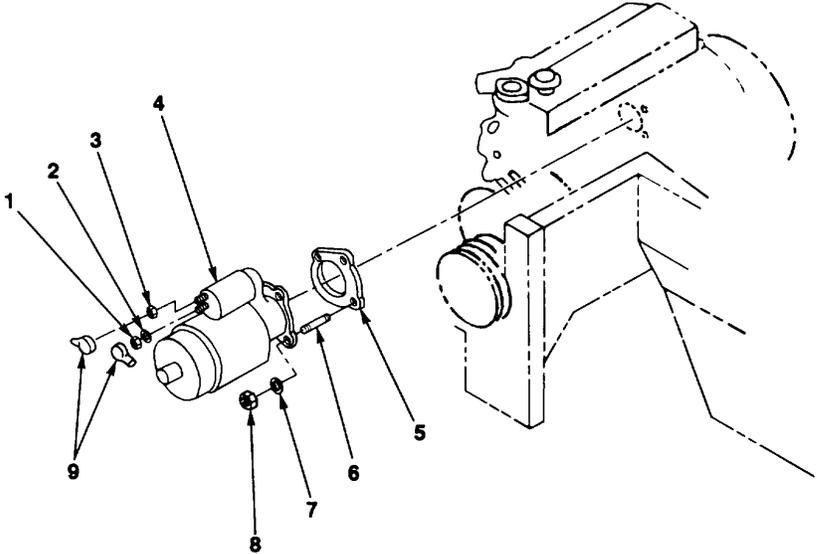
FIG. 40. STARTER MOTOR INSTALLATION
