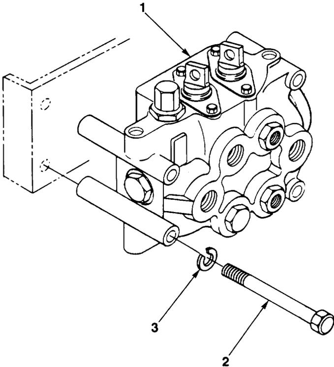
FIG. 119. MAIN CONTROL VALVE INSTALLATION
