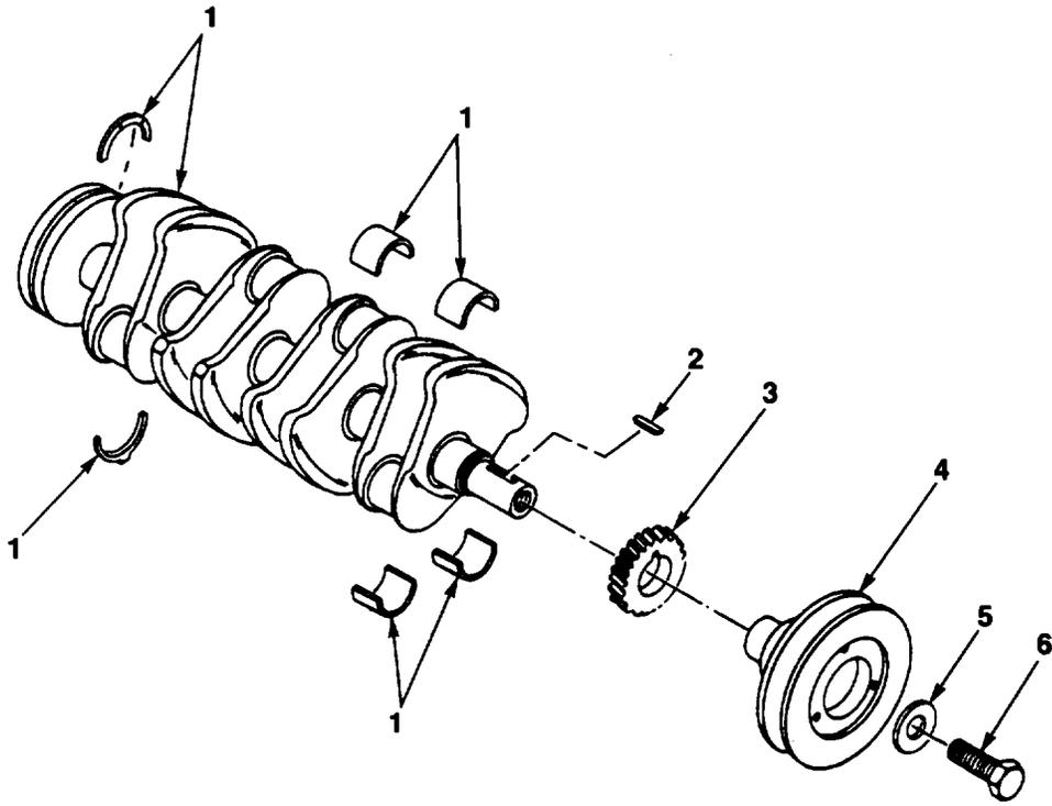
FIG. 4. CRANKSHAFT AND FRONT DRIVE ASSEMBLY
