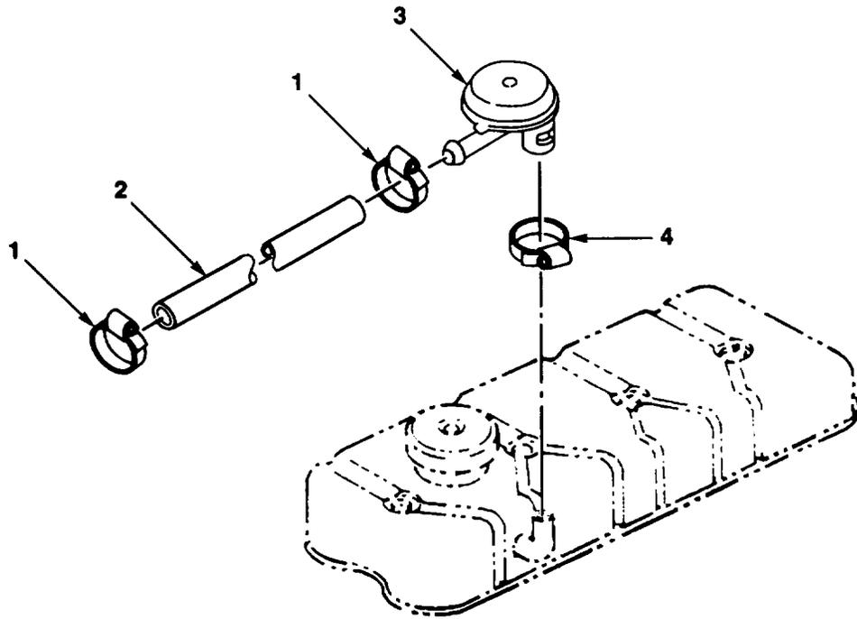
FIG. 12. CRANKCASE BREATHER HOSE AND VENT
