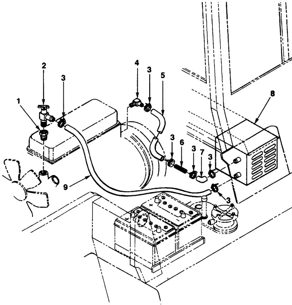
FIG. 114. HEATER INSTALLATION
