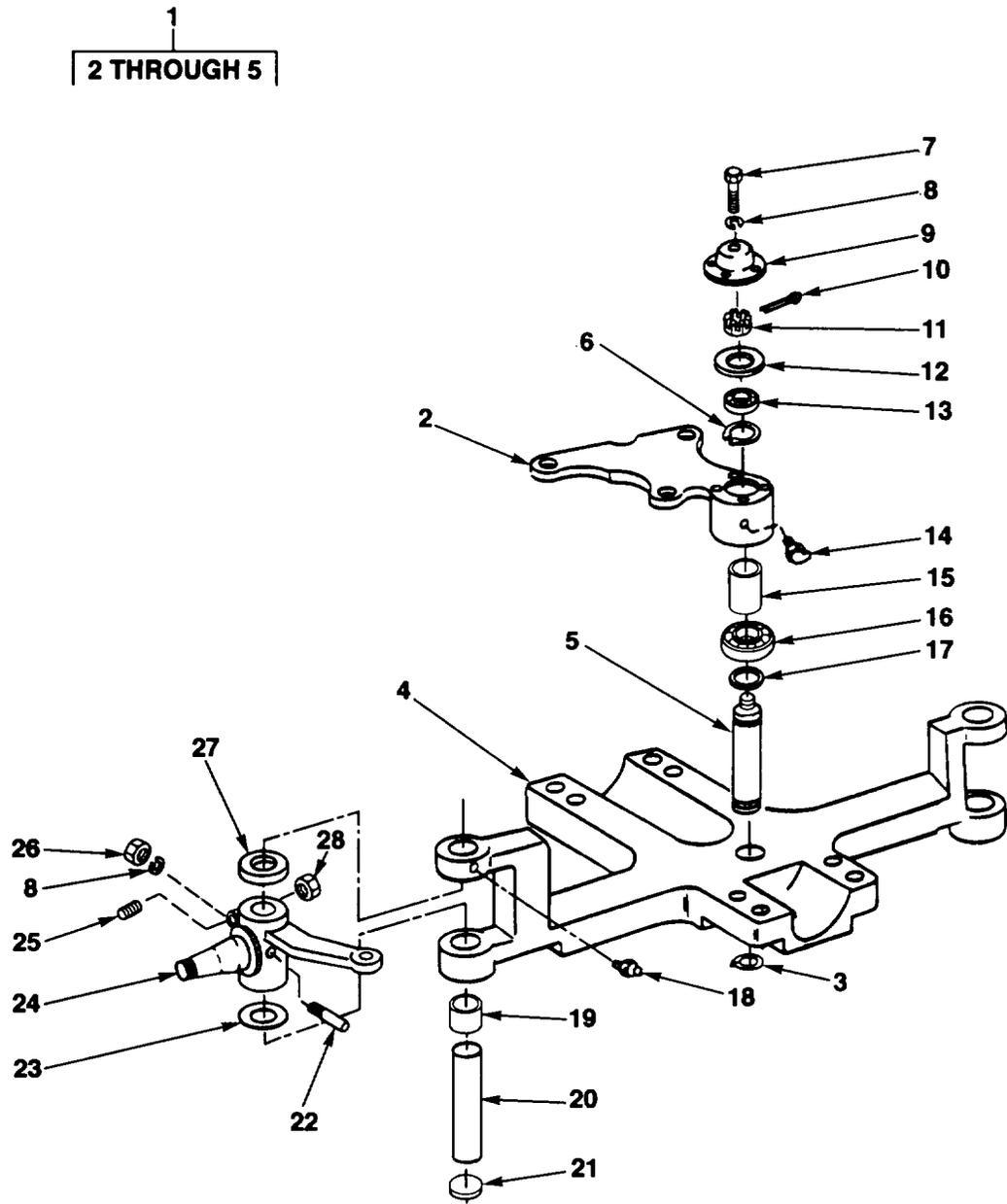
FIG. 78. STEERING AXLE ASSEMBLY
