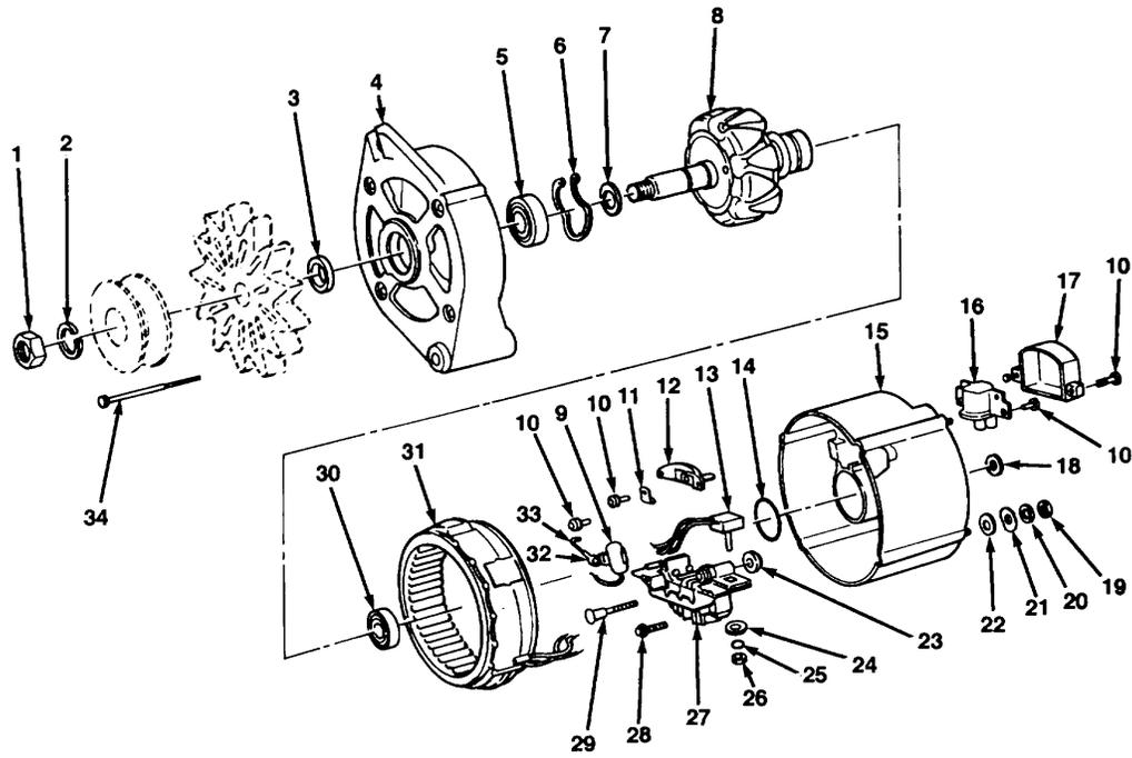
FIG. 38. ALTERNATOR ASSEMBLY
