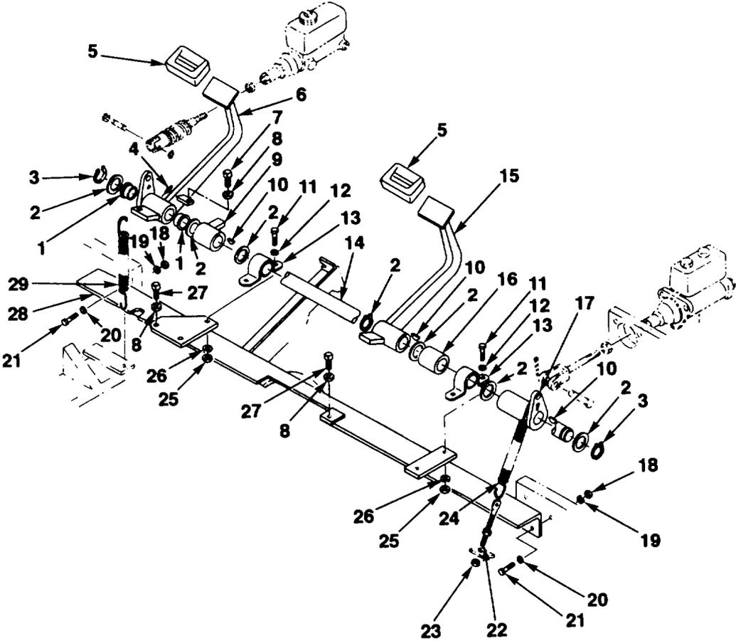
FIG. 86. SERVICE AND INCHING PEDALS AND LINKAGE
