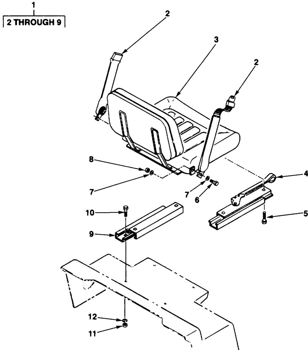
FIG. 108. SEAT BELT AND SEAT MOUNTING
