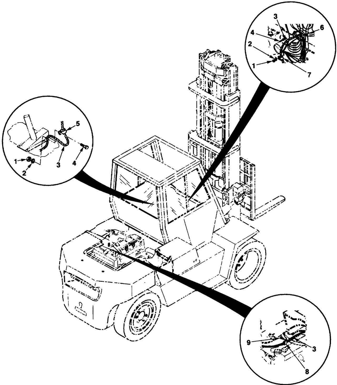
FIG. 55. MAIN WIRING HARNESS
