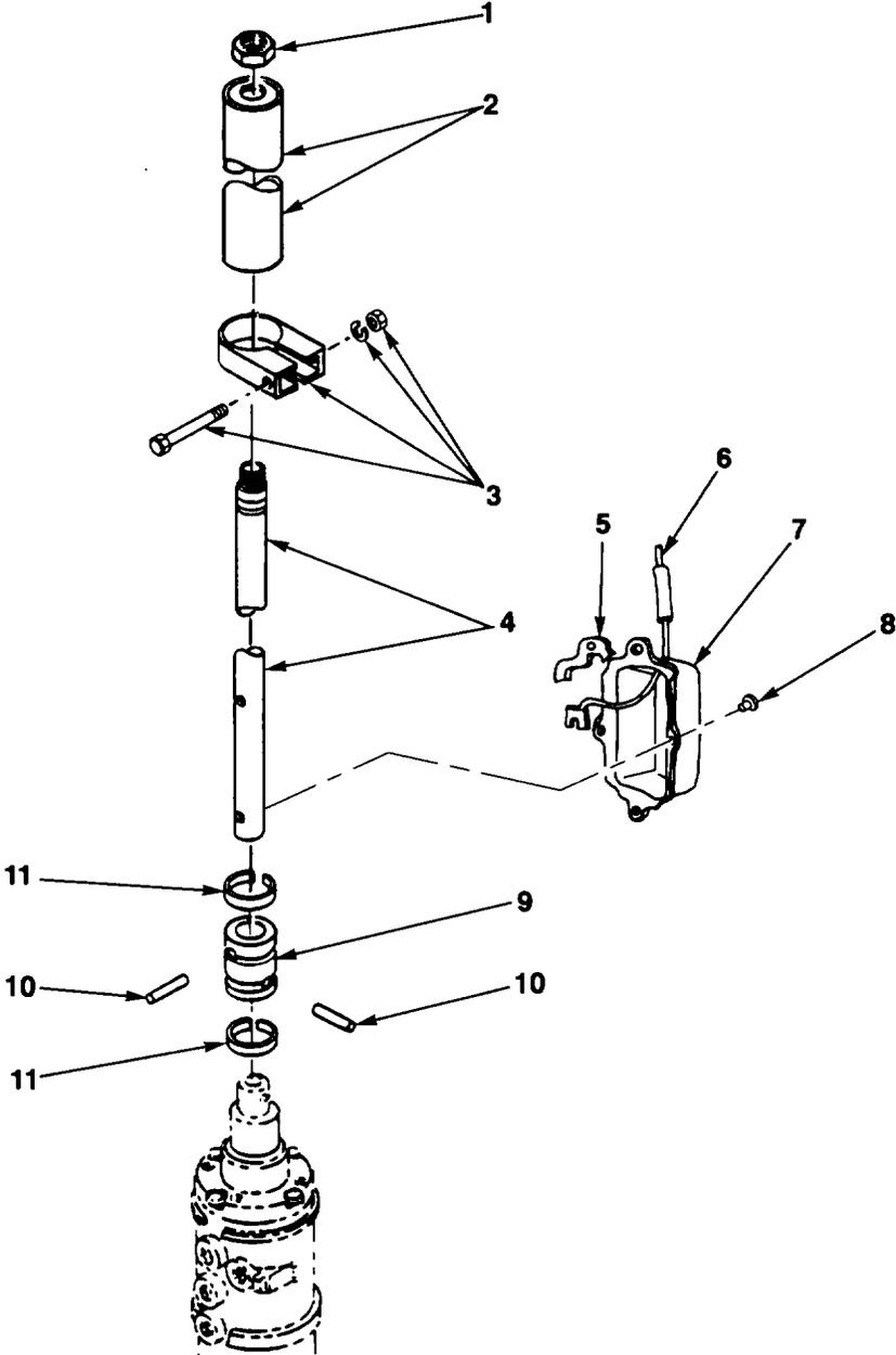
FIG. 94. STEERING COLUMN ASSEMBLY
