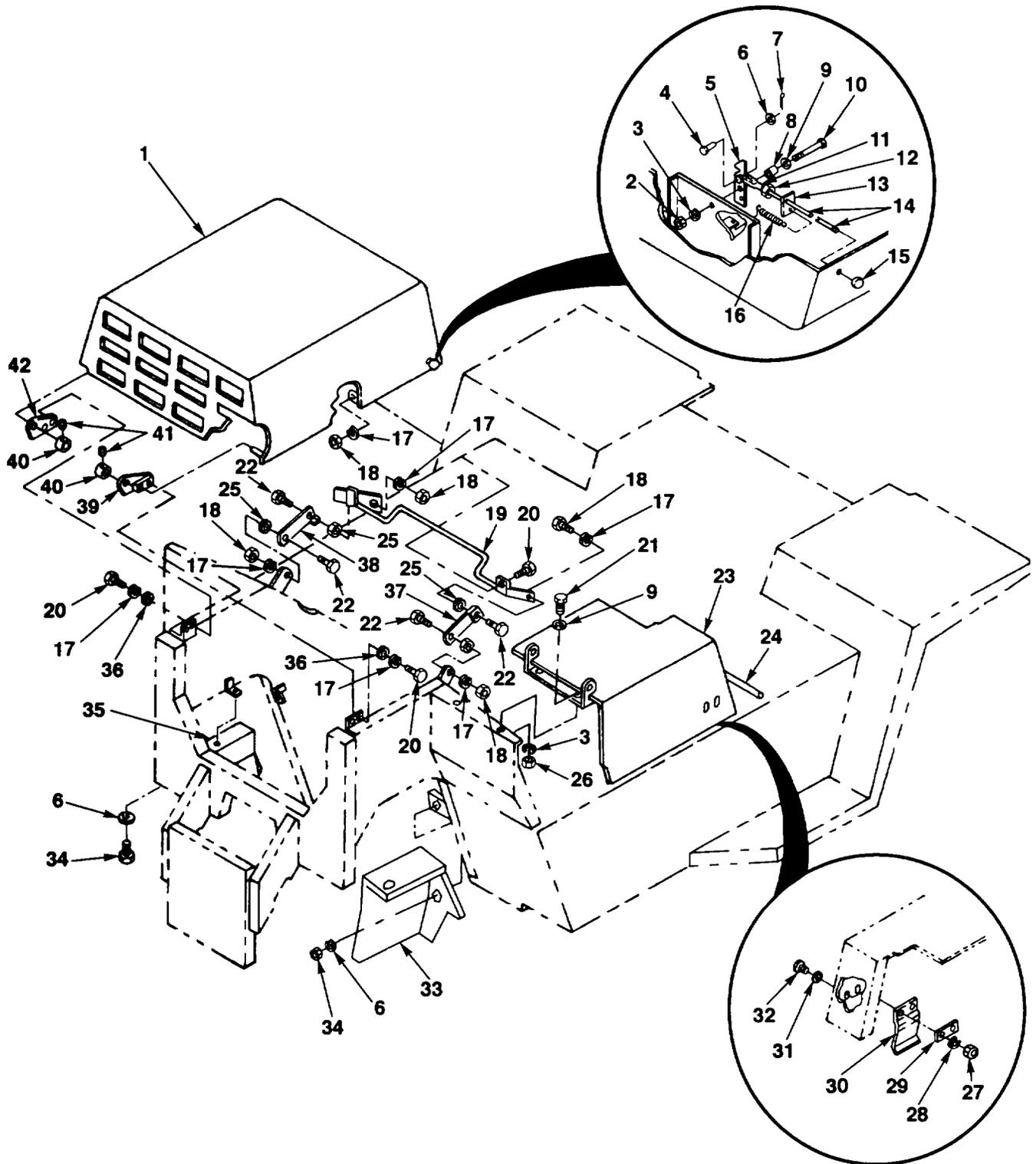
FIG. 104. HOOD AND LATCH ASSEMBLY
