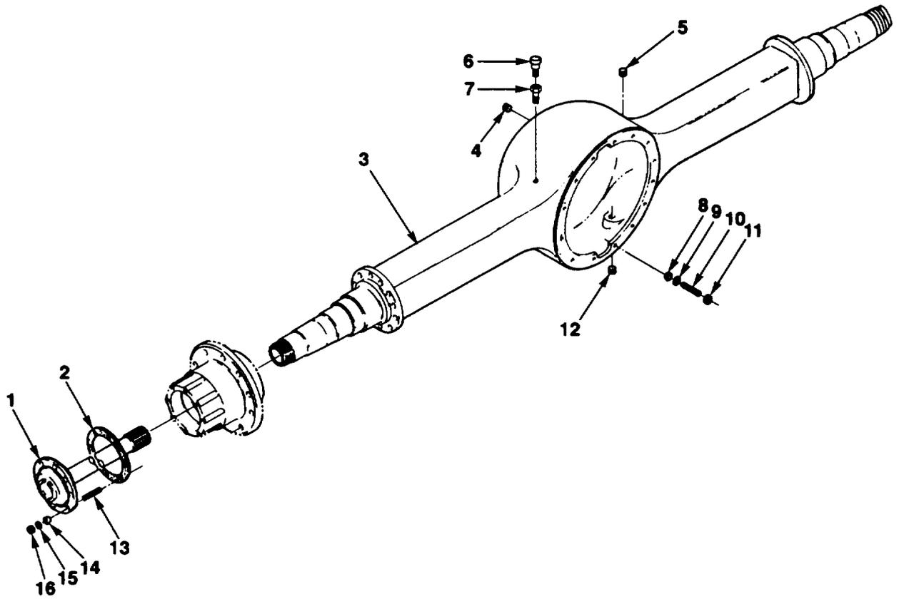
FIG. 75. DRIVE AXLE ASSEMBLY
