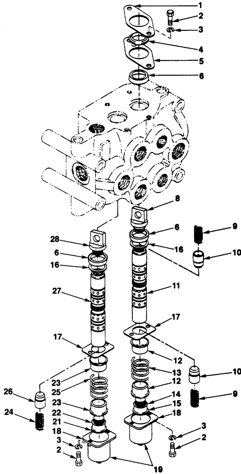
FIG. 121. MAIN CONTROL VALVE, DA AND SA PLUNGER ASSEMBLY
