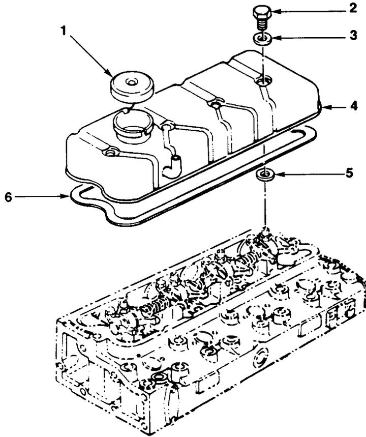
FIG. 8. VALVE COVER ASSEMBLY
