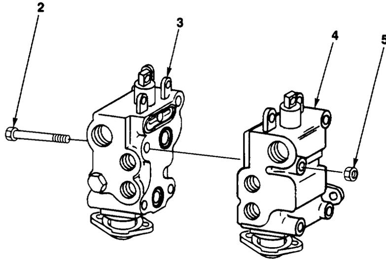
FIG. 124. AUXILIARY CONTROL VALVE ASSEMBLY
