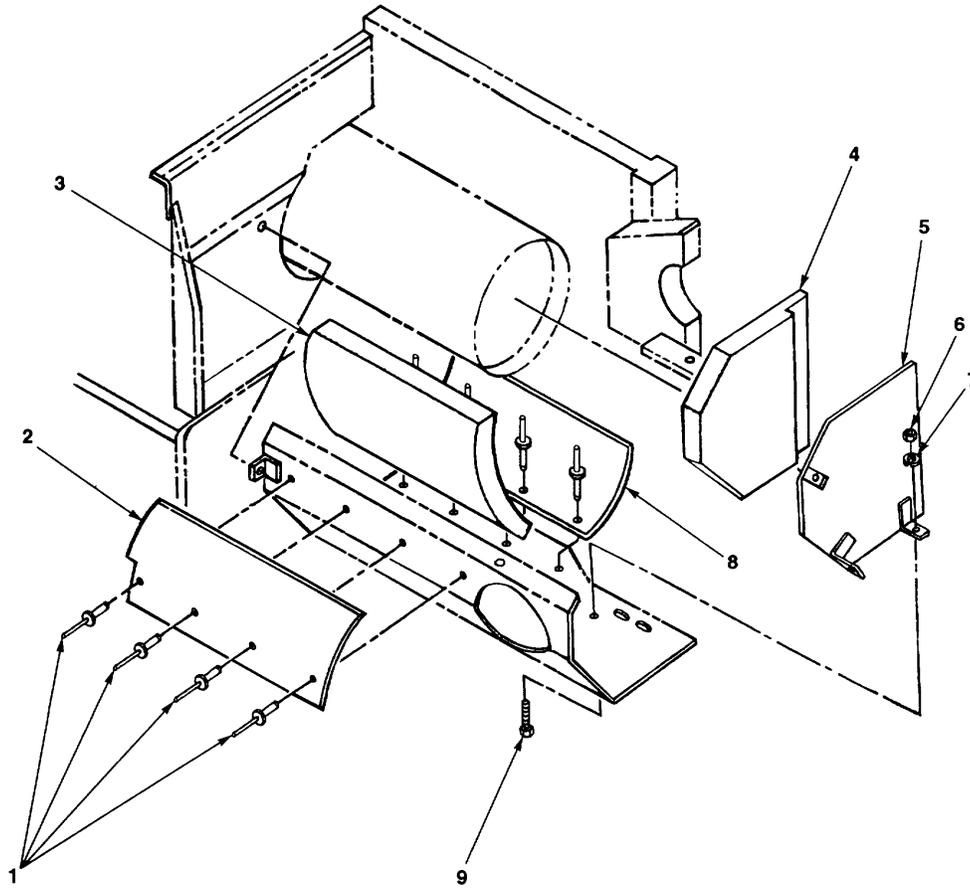
FIG. 33. EXHAUST HEAT SHIELD AND INSULATION
