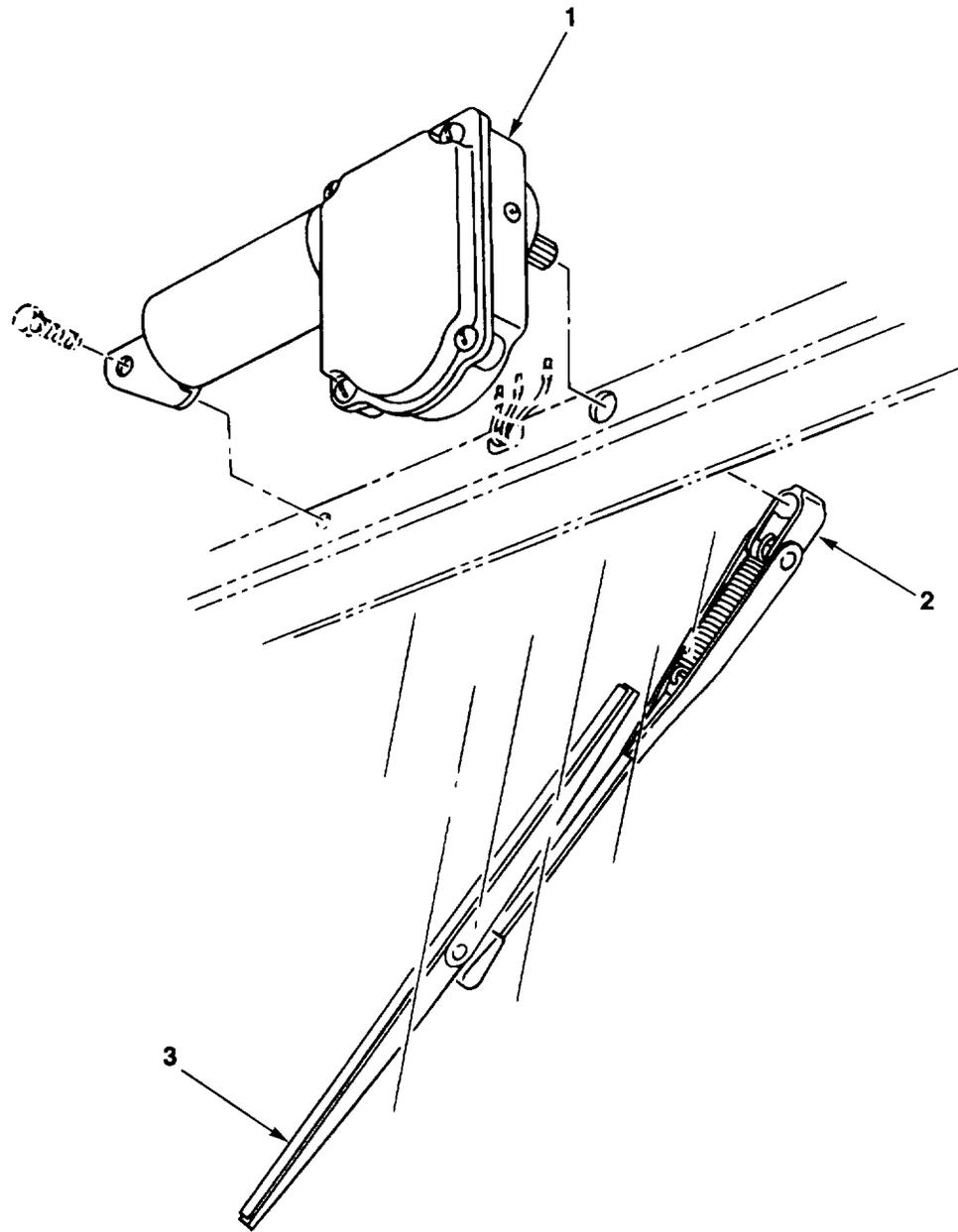
FIG. 111. REAR WINDOW WIPER ASSEMBLY
