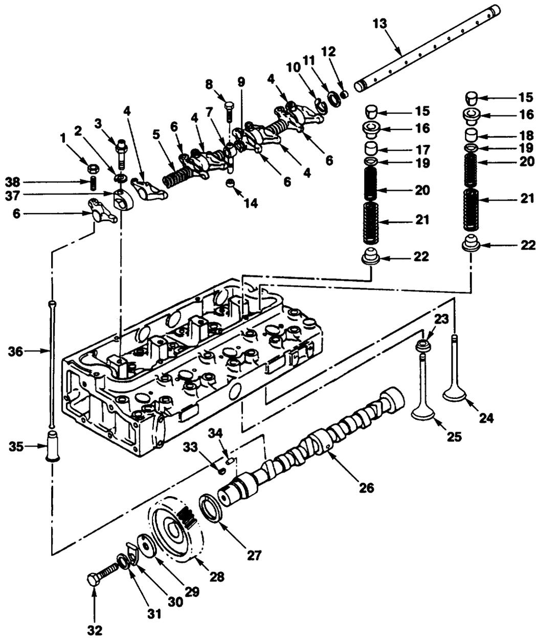
FIG. 9. VALVE, ROCKER ARMS, PUSHRODS AND CAMSHAFT
