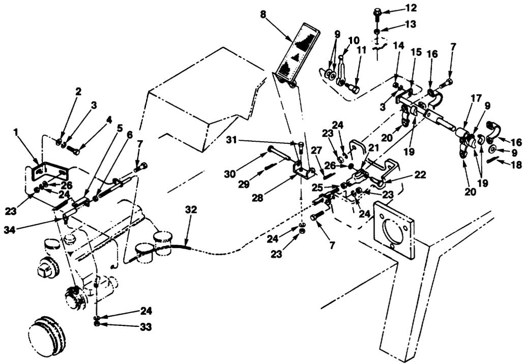
FIG. 31. ACCELERATOR PEDAL AND LINKAGE
