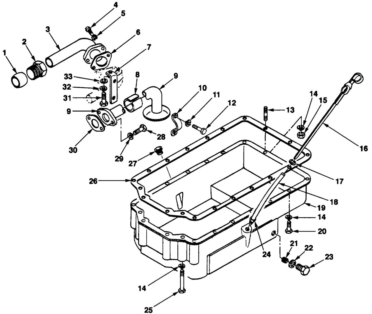
FIG. 14. OIL PAN AND DIPSTICK ASSEMBLY
