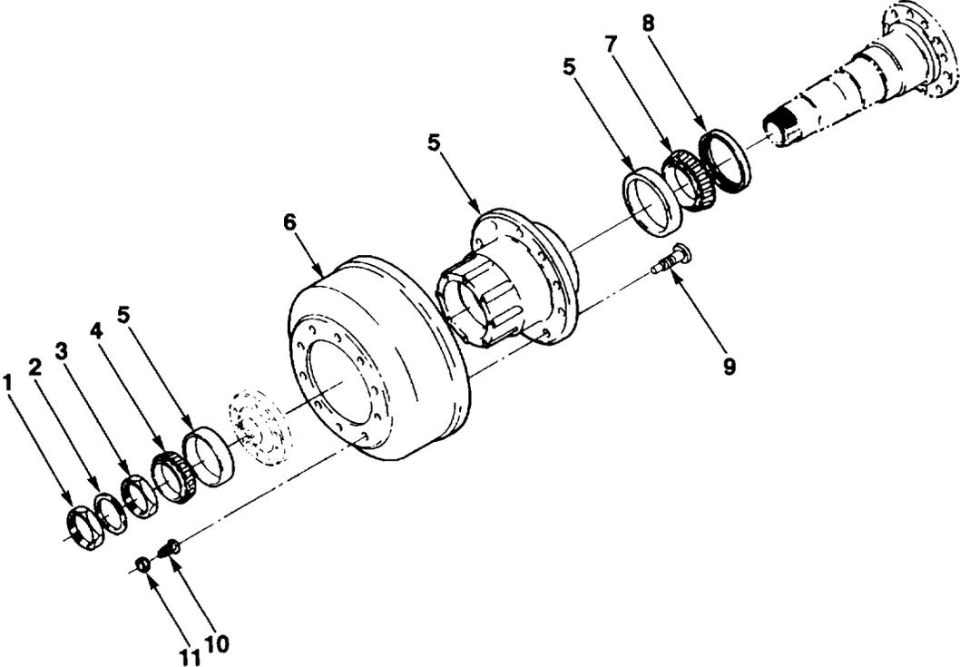
FIG. 88. DRIVE AXLE HUB ASSEMBLY AND DRUM
