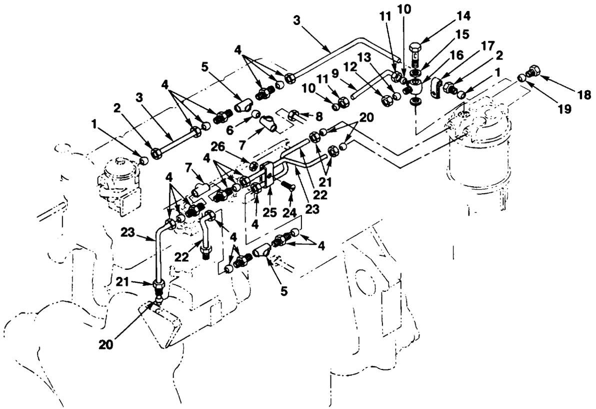
FIG. 18. ENGINE FUEL LINES AND FITTINGS
