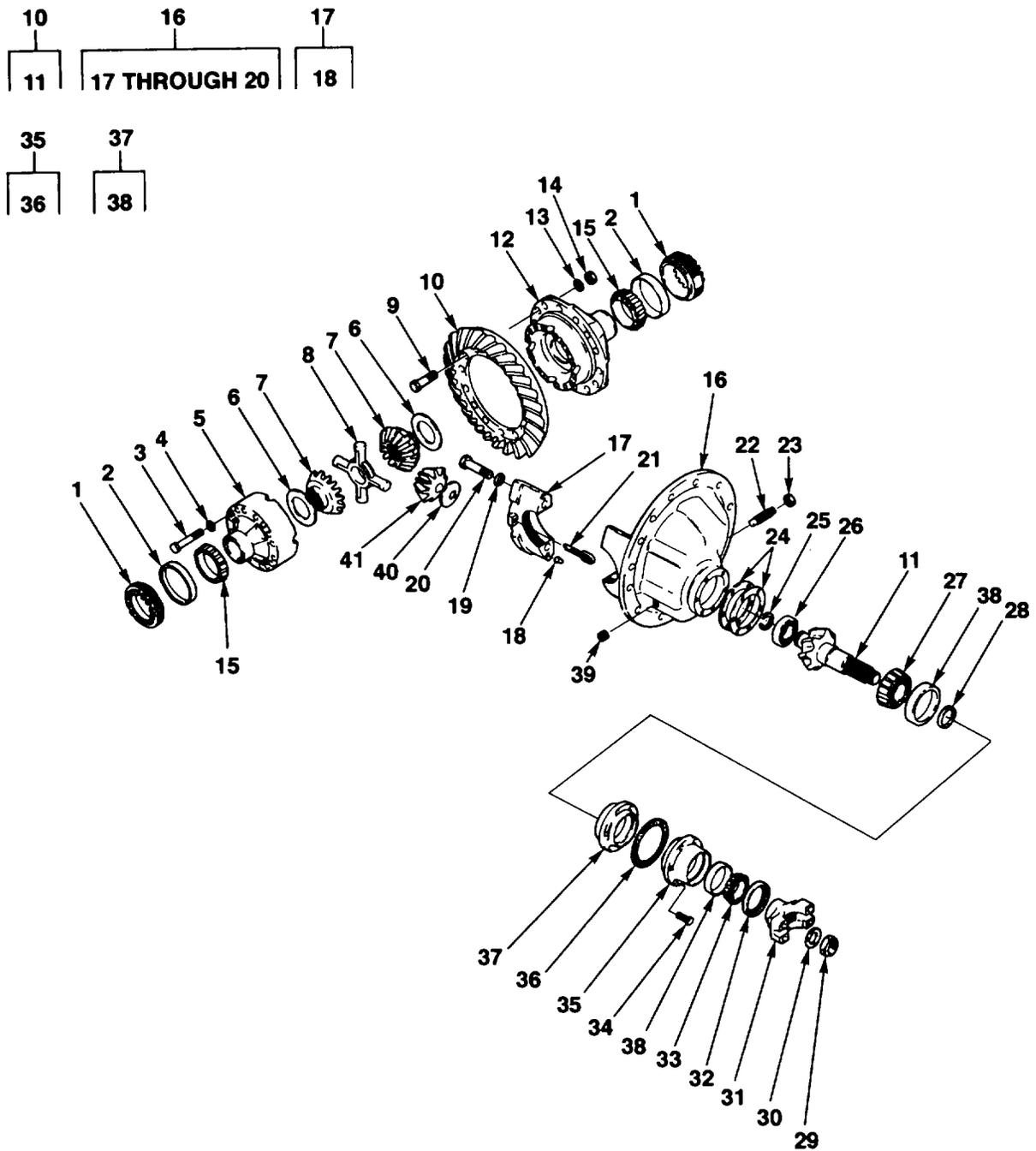
FIG. 76. DIFFERENTIAL CARRIER ASSEMBLY
