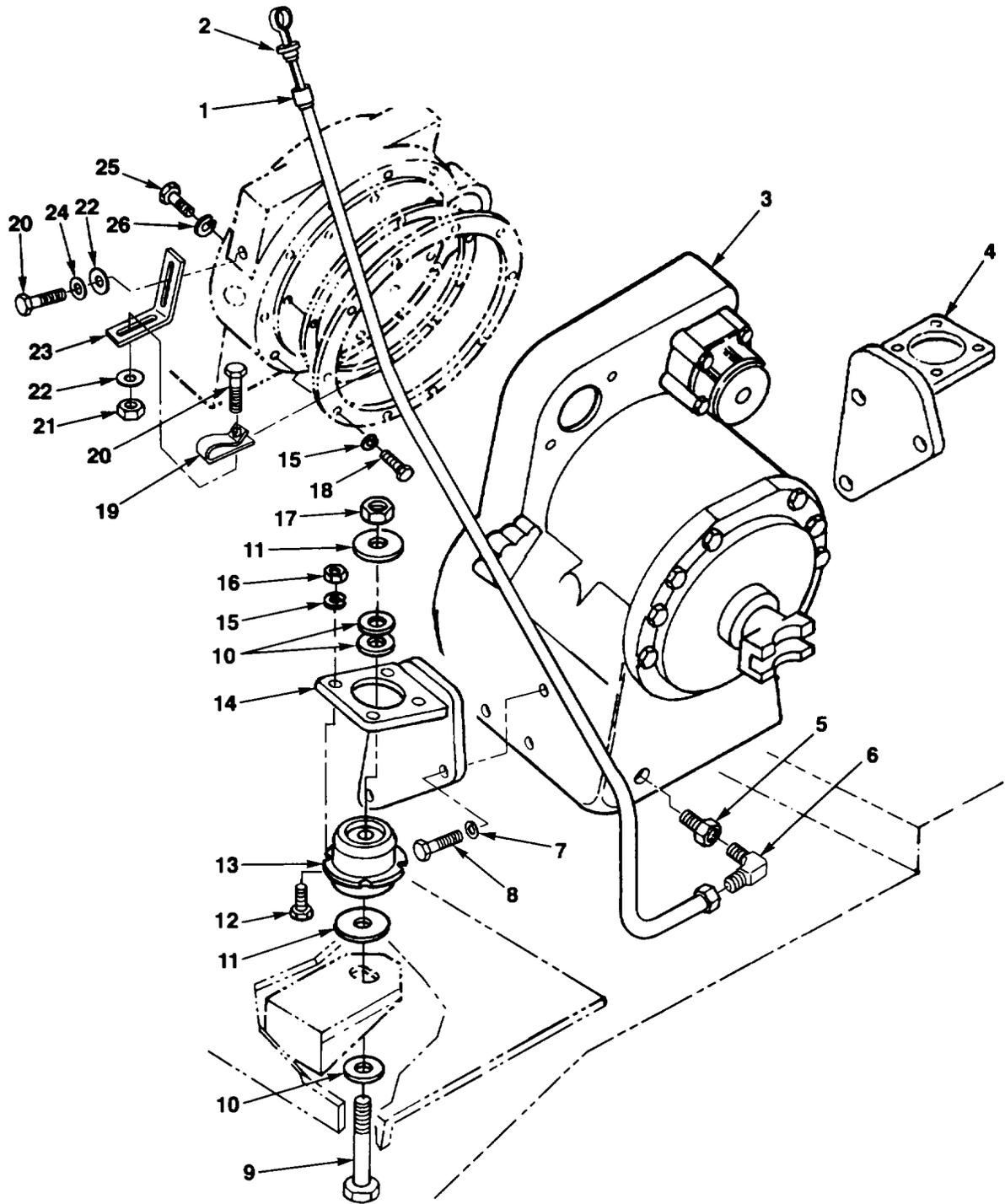
FIG. 60. TRANSMISSION INSTALLATION
