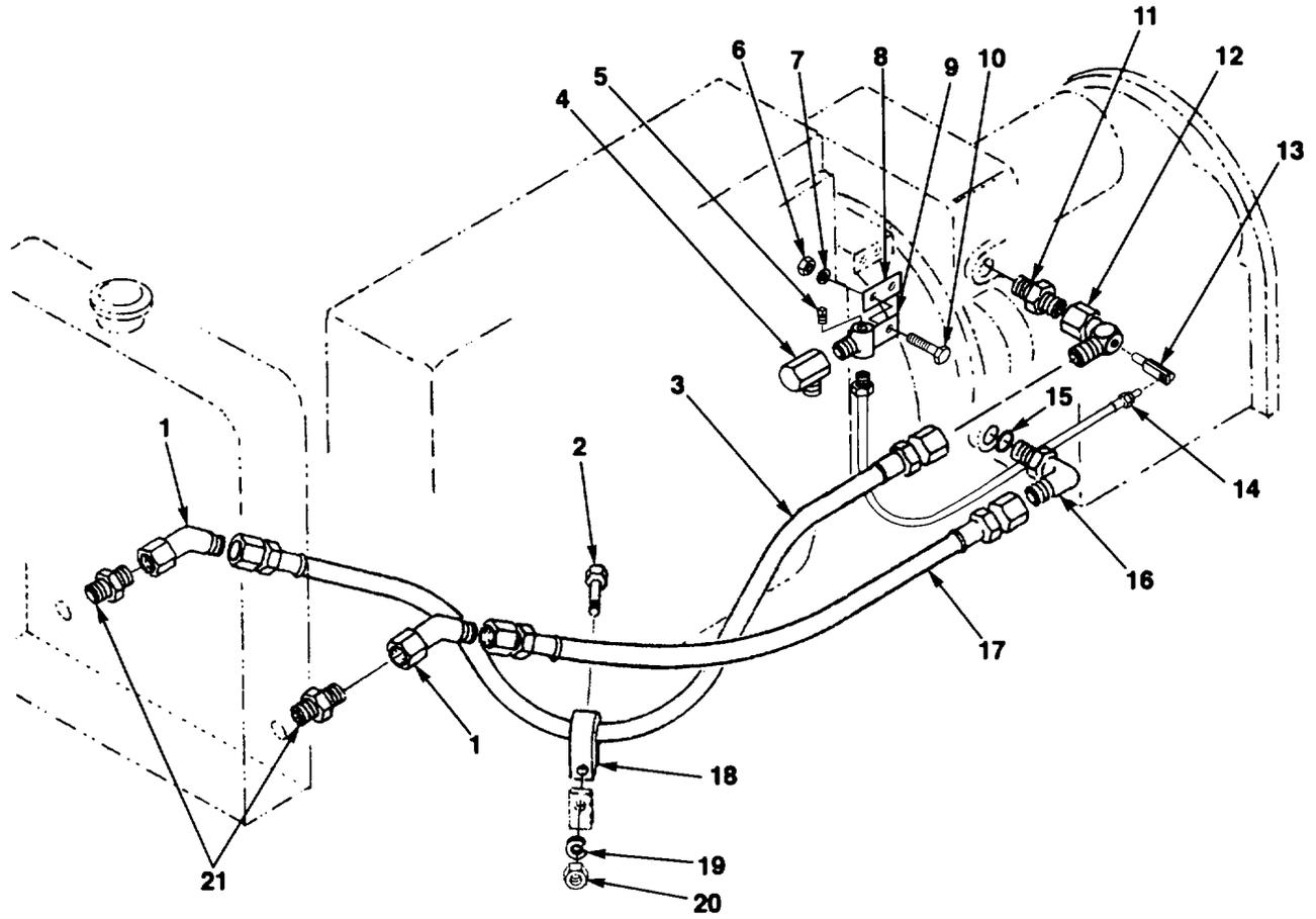
FIG. 70. TRANSMISSION LINES AND FITTINGS
