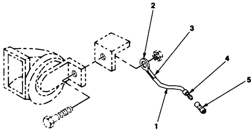
FIG. 52. HORN GROUND WIRING
