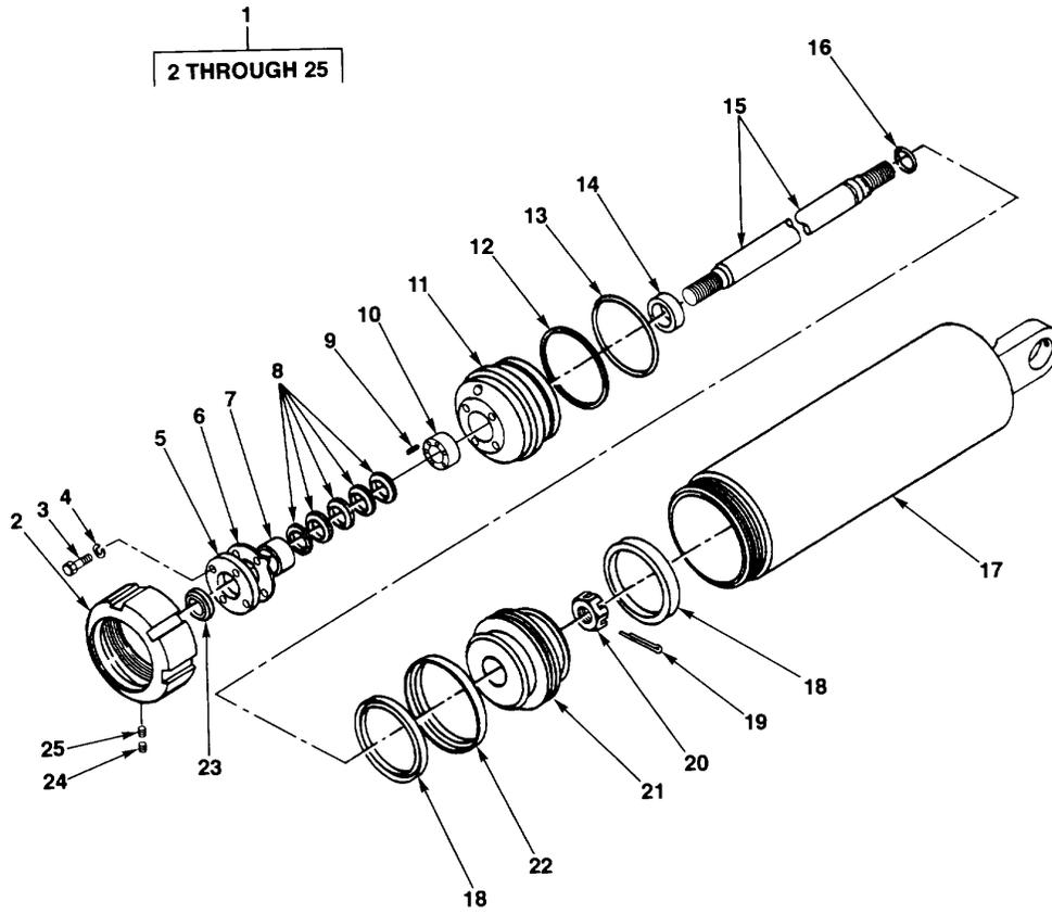
FIG. 131. TILT CYLINDER ASSEMBLY
