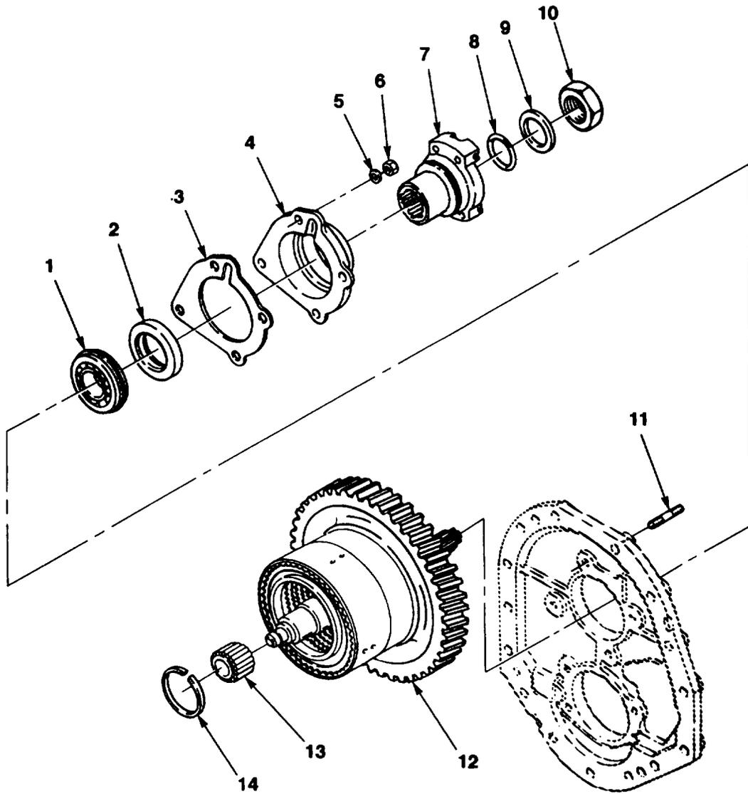
FIG. 61. OUTPUT SHAFT
