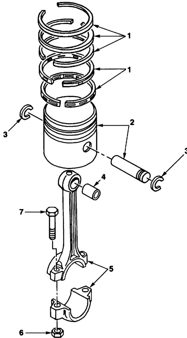
FIG. 7. PISTON AND CONNECTING ROD
