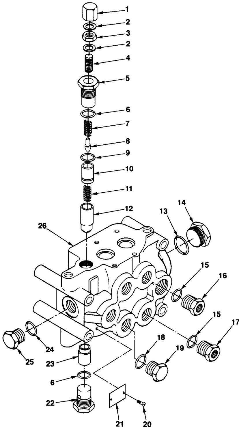
FIG. 120. MAIN CONTROL VALVE, PLUGS AND RELIEF VALVE
