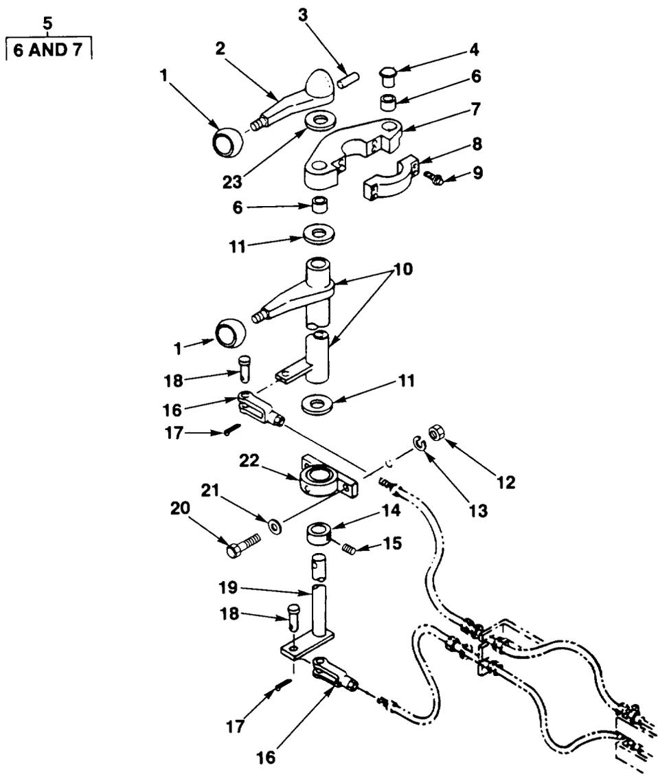
FIG. 57. DIRECTIONAL AND SHIFT LINKAGE CONTROLS
