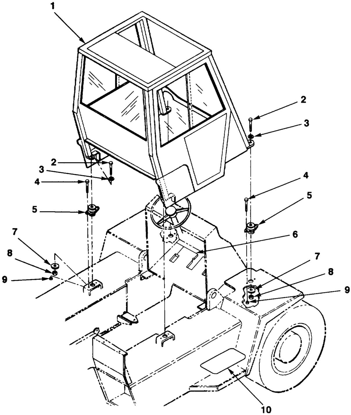
FIG. 102. CAB INSTALLATION
