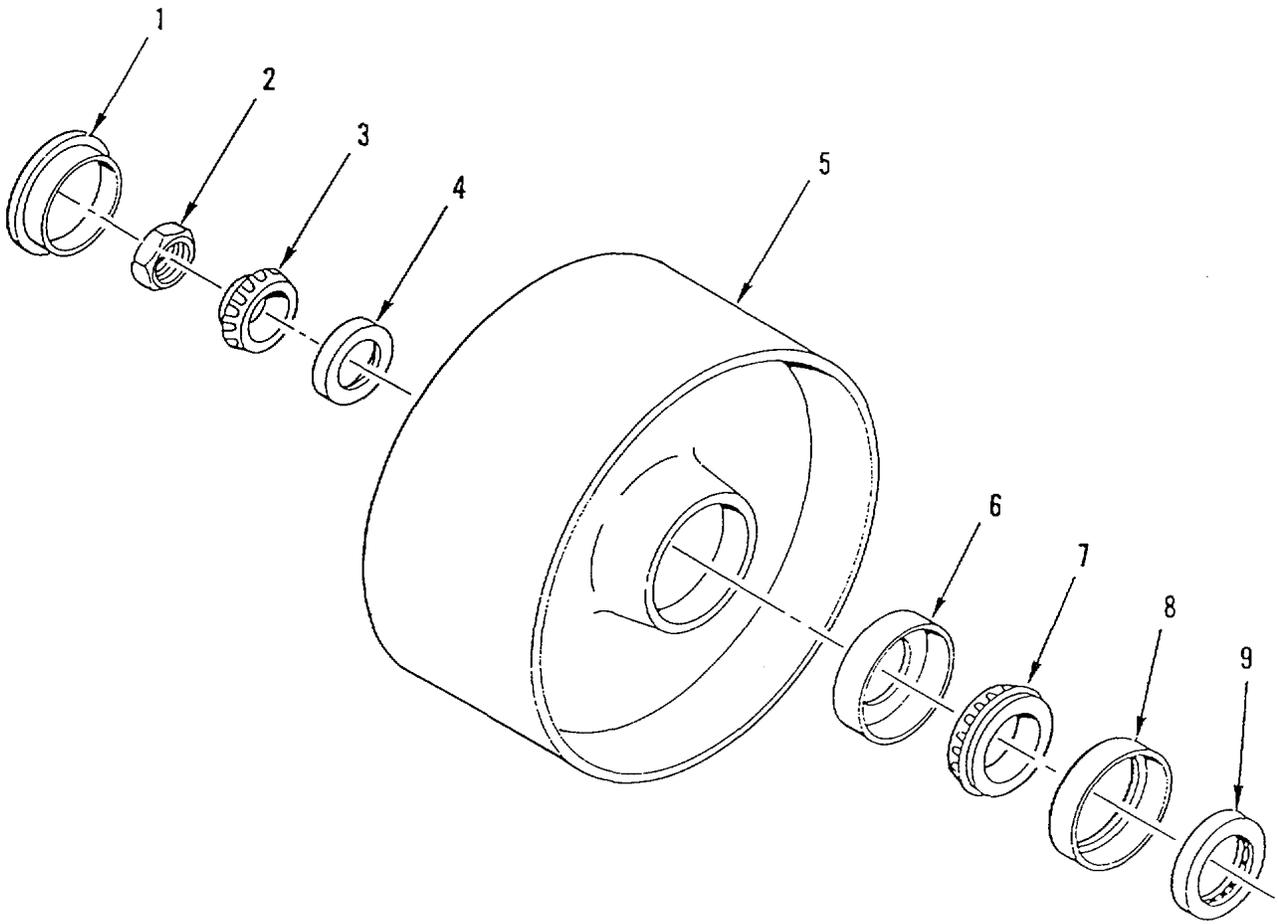
Figure 31. Steering Axle Wheel Assembly
