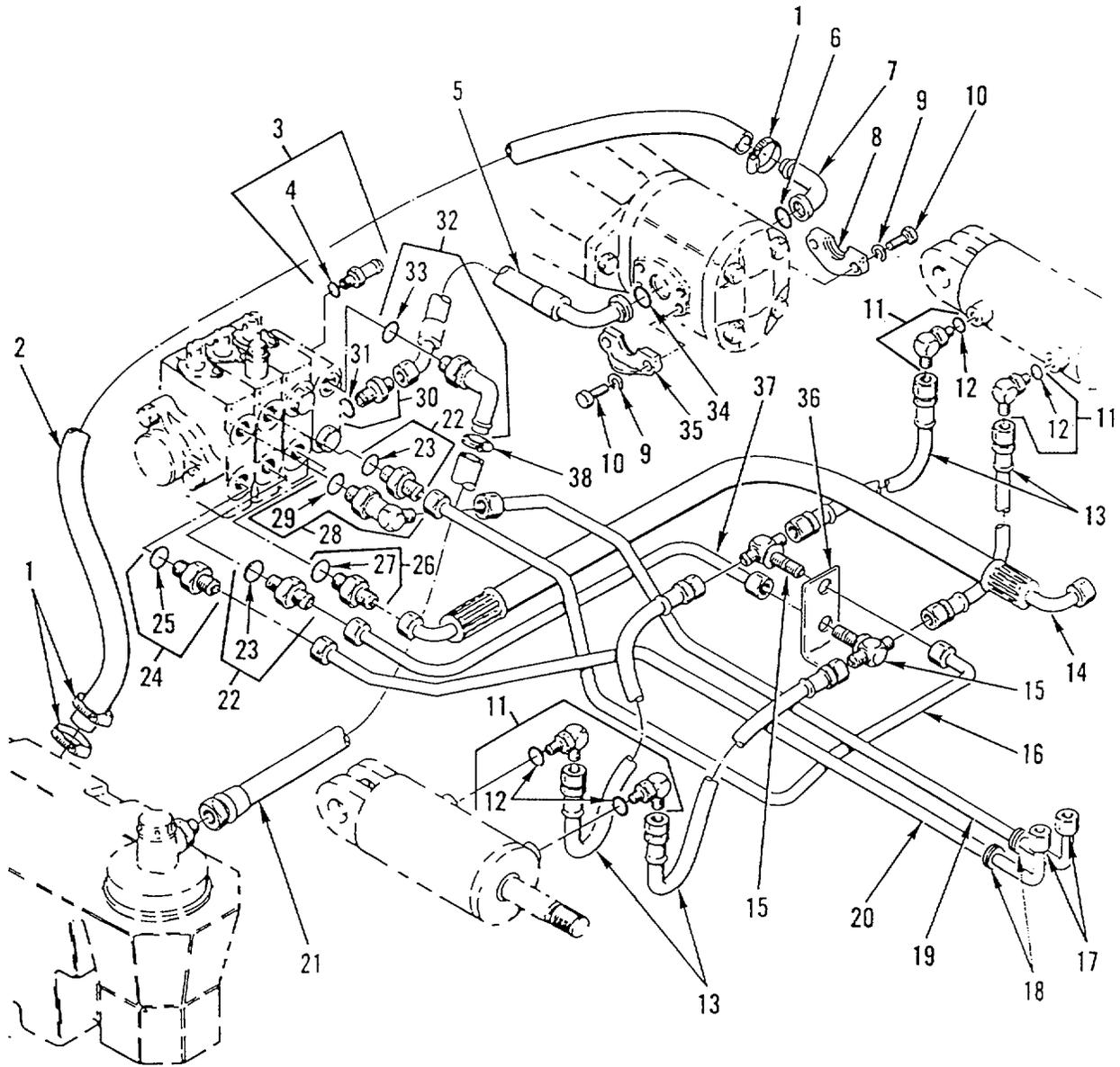
Figure 61. Hydraulic Assembly
