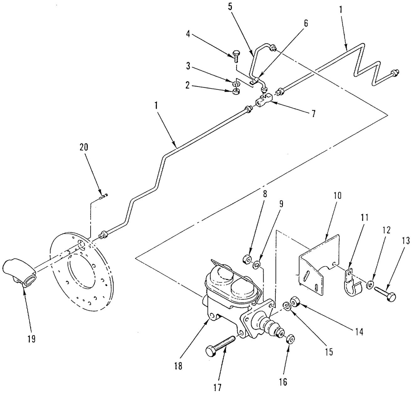
Figure 28. Service Brake Linkage
