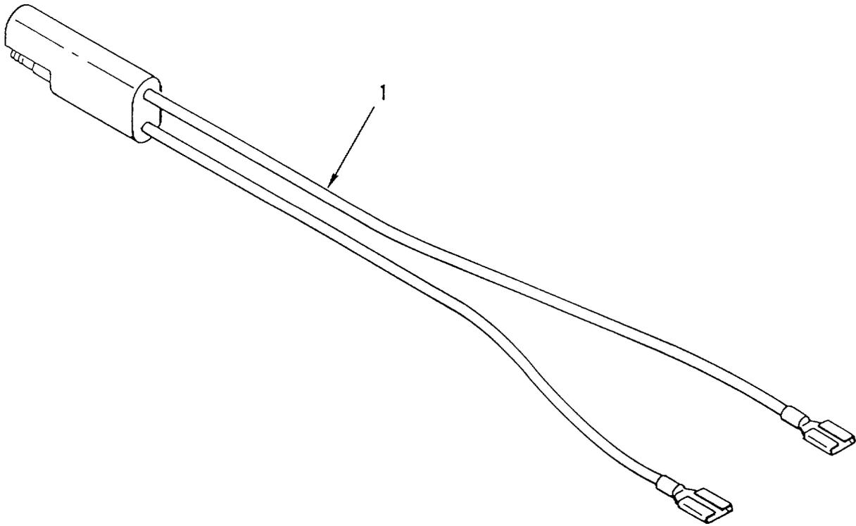
Figure 15. Seat Brake Wiring Harness
