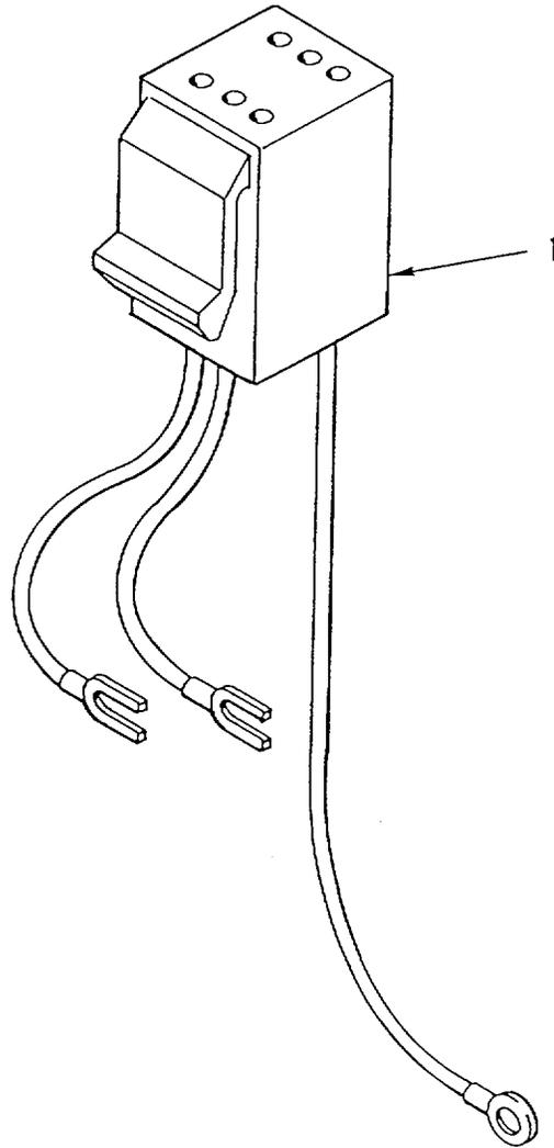
Figure 18. Control Panel Wiring Harness
