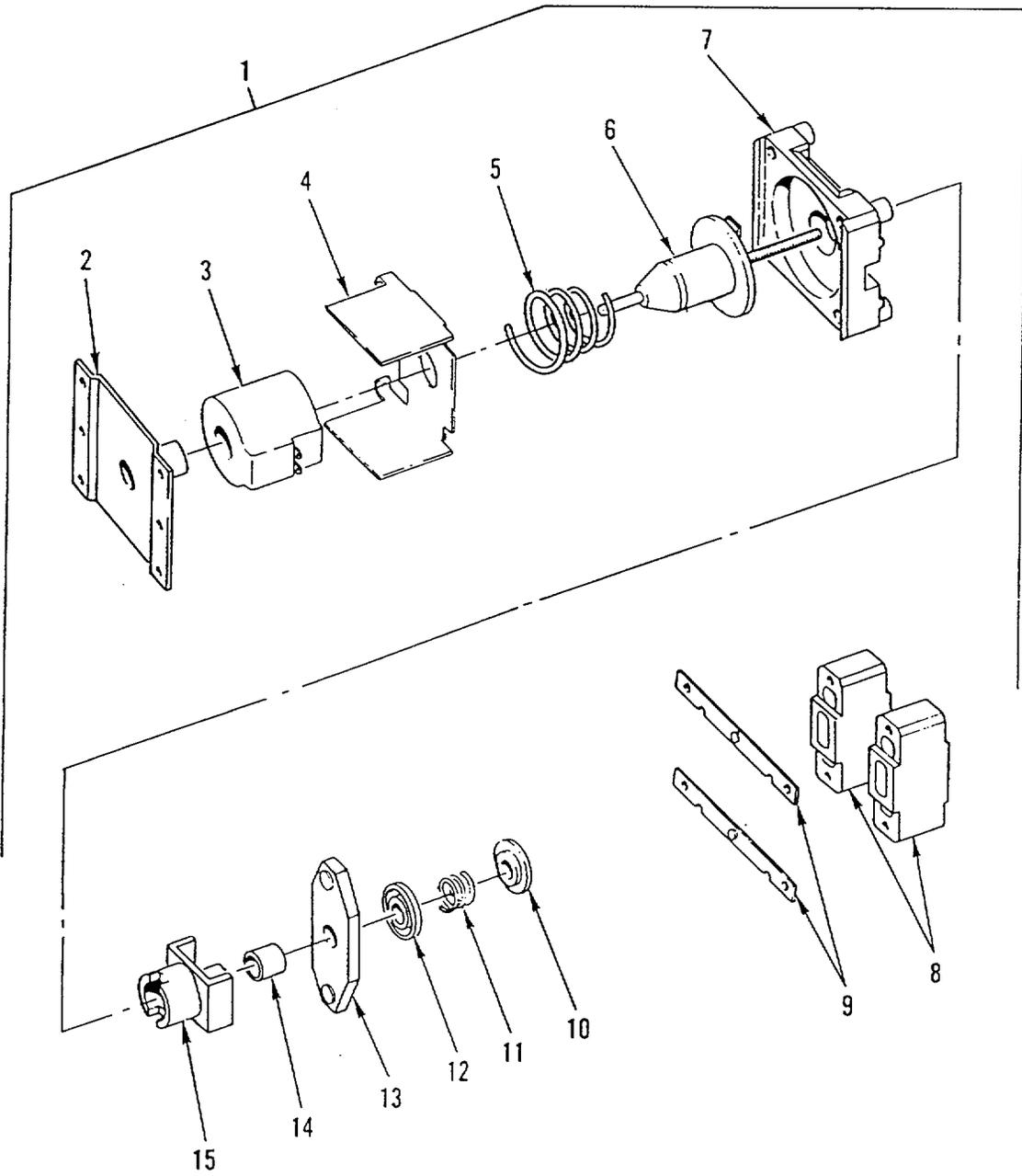
Figure 77. 1a/FW/Pump Contactor
