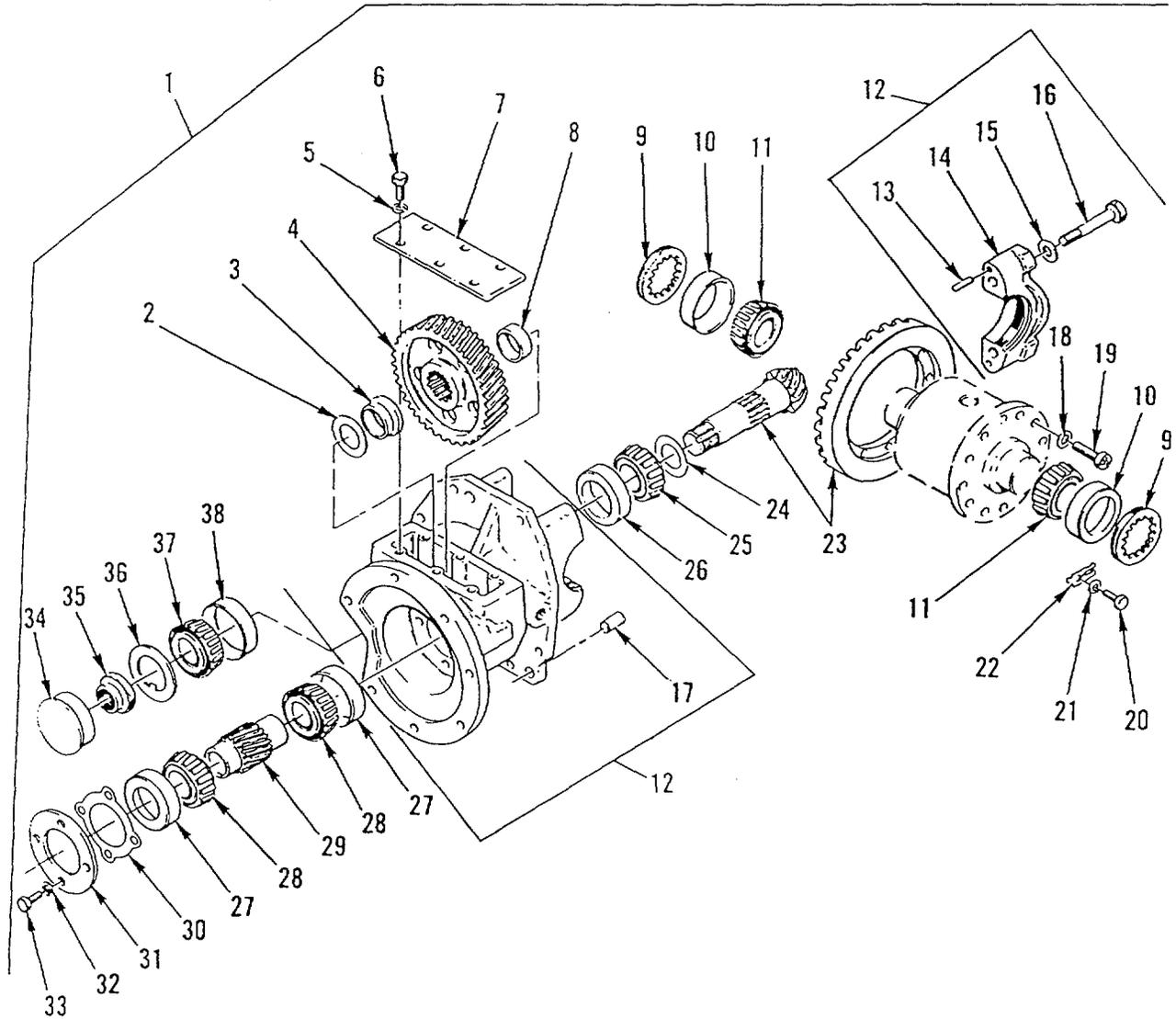
Figure 19. Transmission Assembly
