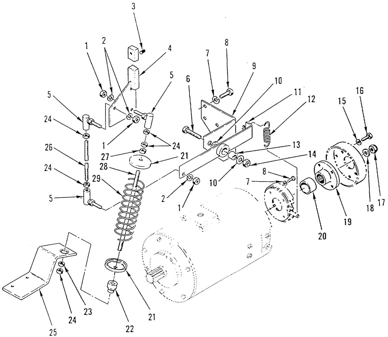
Figure 25. Seat Brake Linkage
