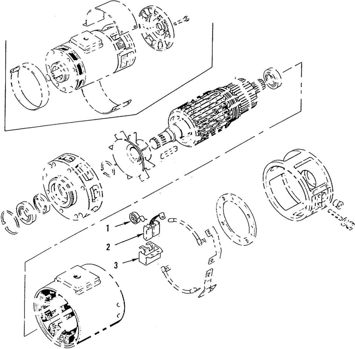
Figure 71. Traction Motor Brushes
