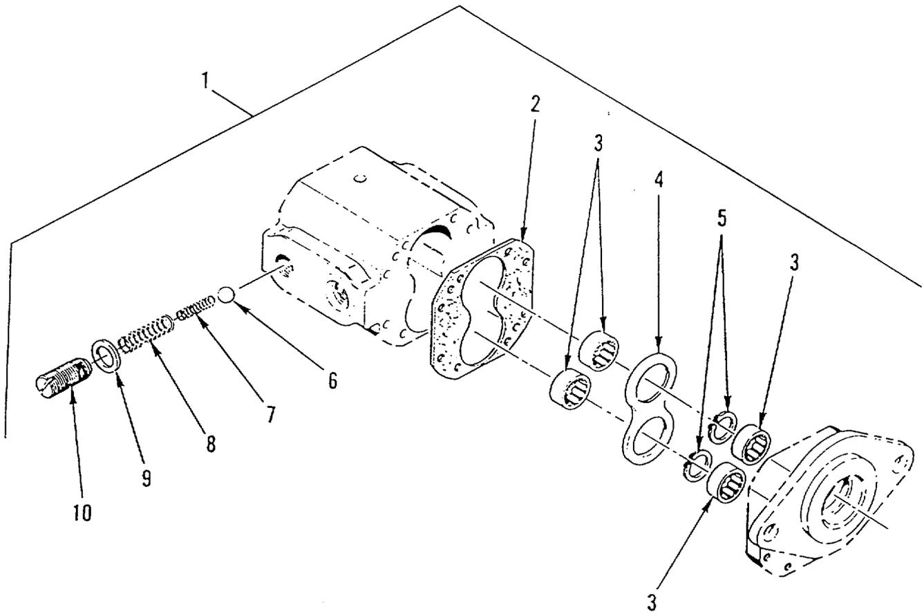
Figure 34. Steering Pump Assembly
