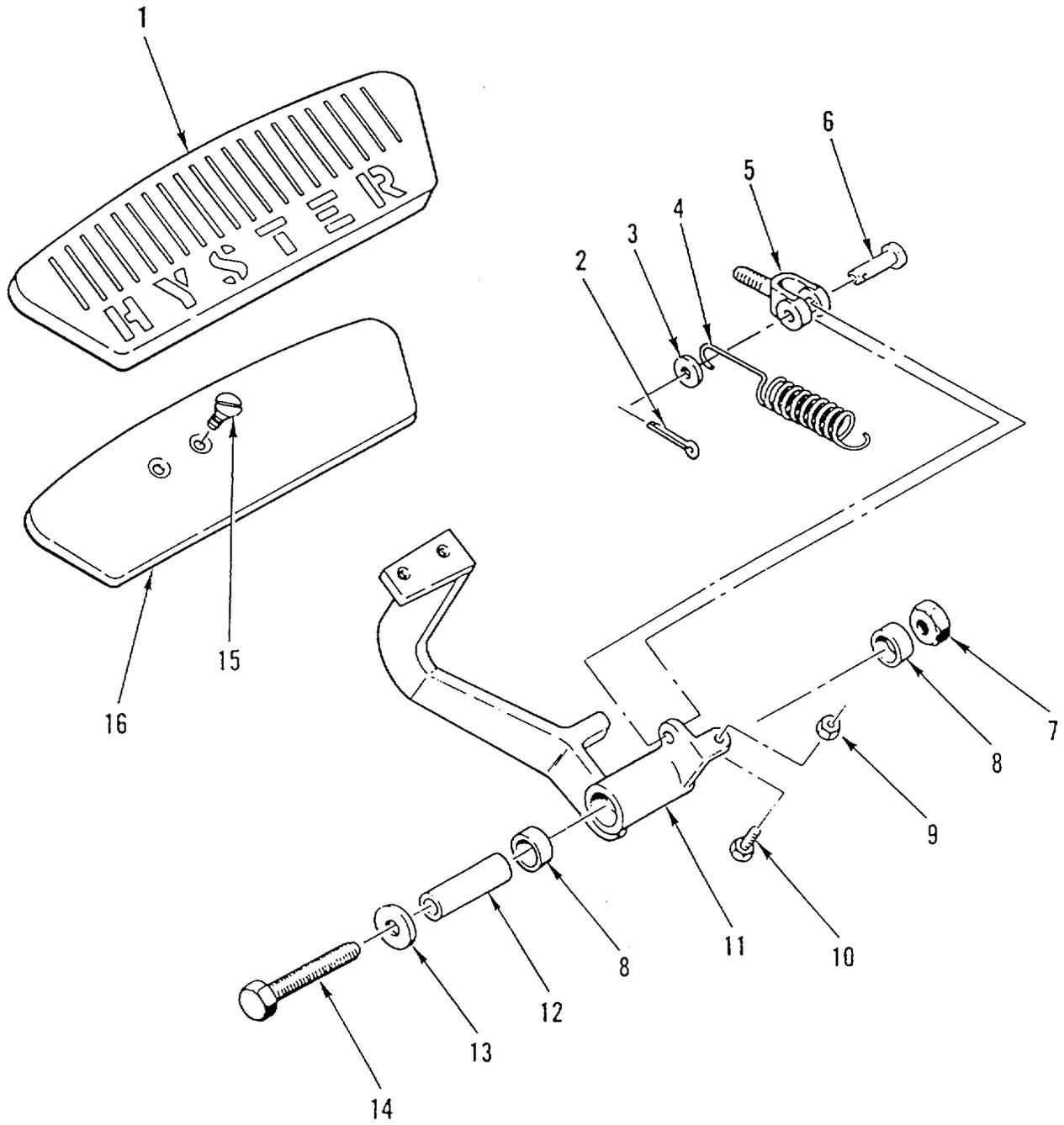
Figure 29. Service Brake Pedal
