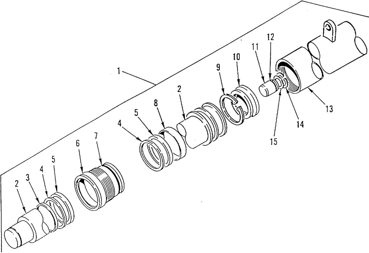
Figure 53. Main Lift Cylinder
