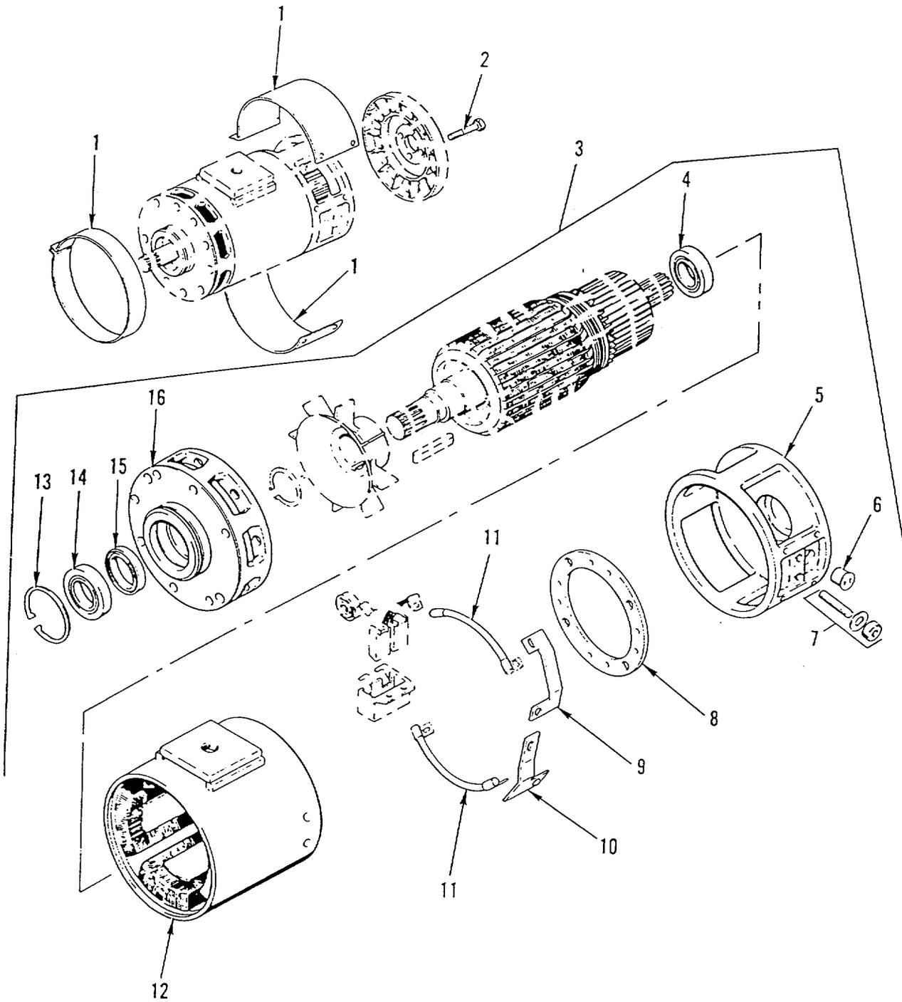
Figure 65. Traction Motor
