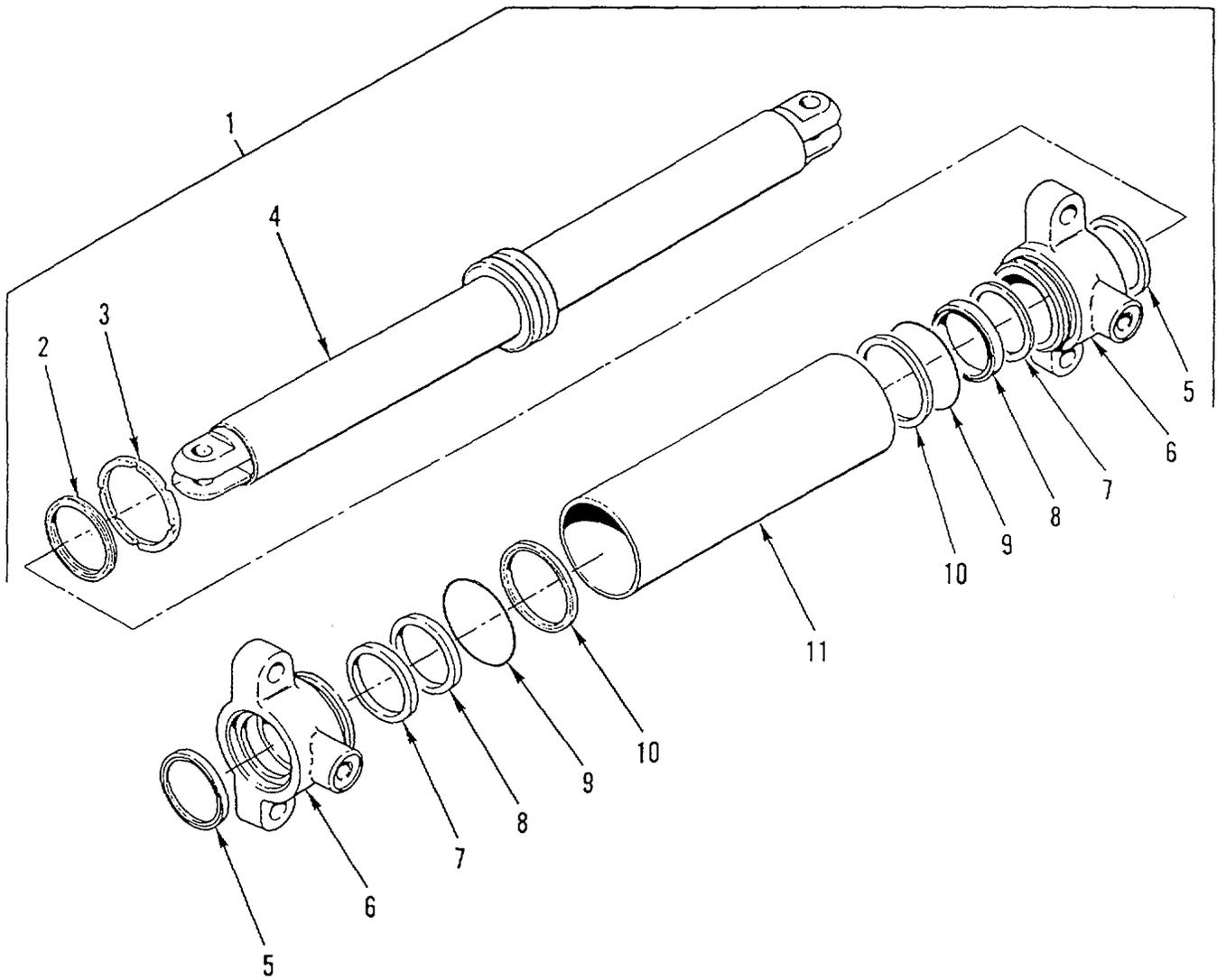
Figure 36. Steering Cylinder
