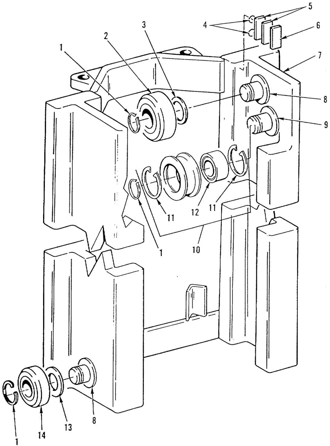
Figure 50. Intermediate Assembly
