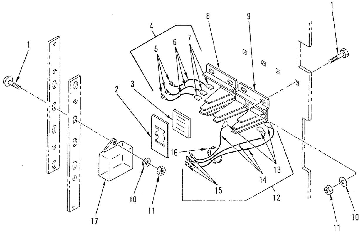
Figure 80. Control Valve Blade Switches
