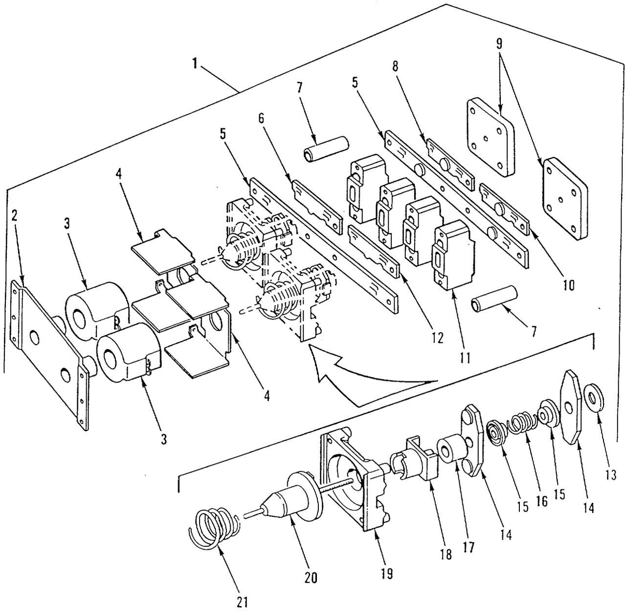
Figure 76. Forward/Reverse Contactor
