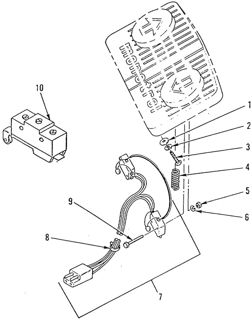
Figure 81. Directional Control Switch
