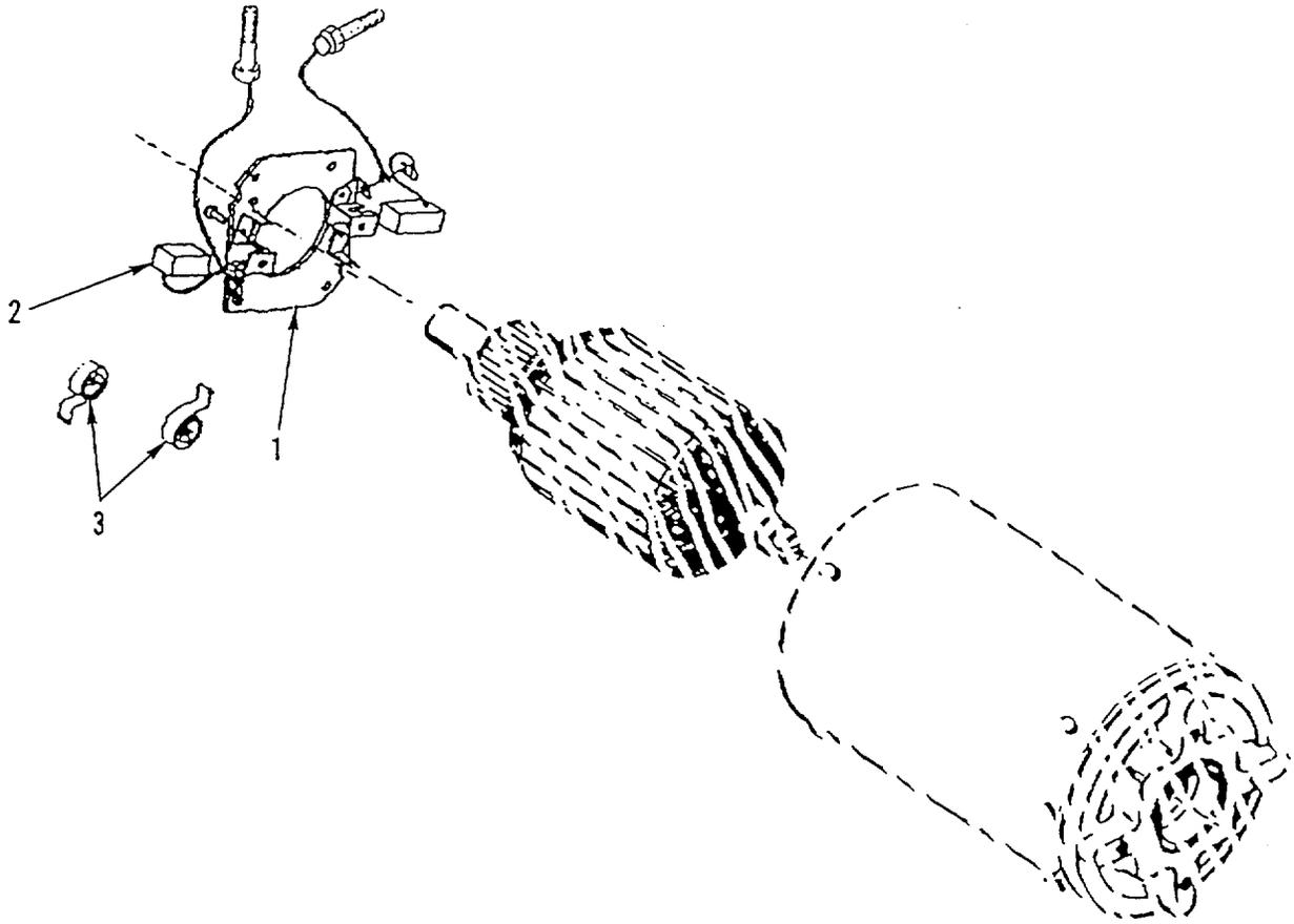
Figure 70. Steering Pump Motor Brushes
