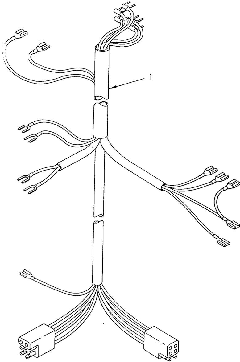
Figure 16. Steering Column Wiring Harness
