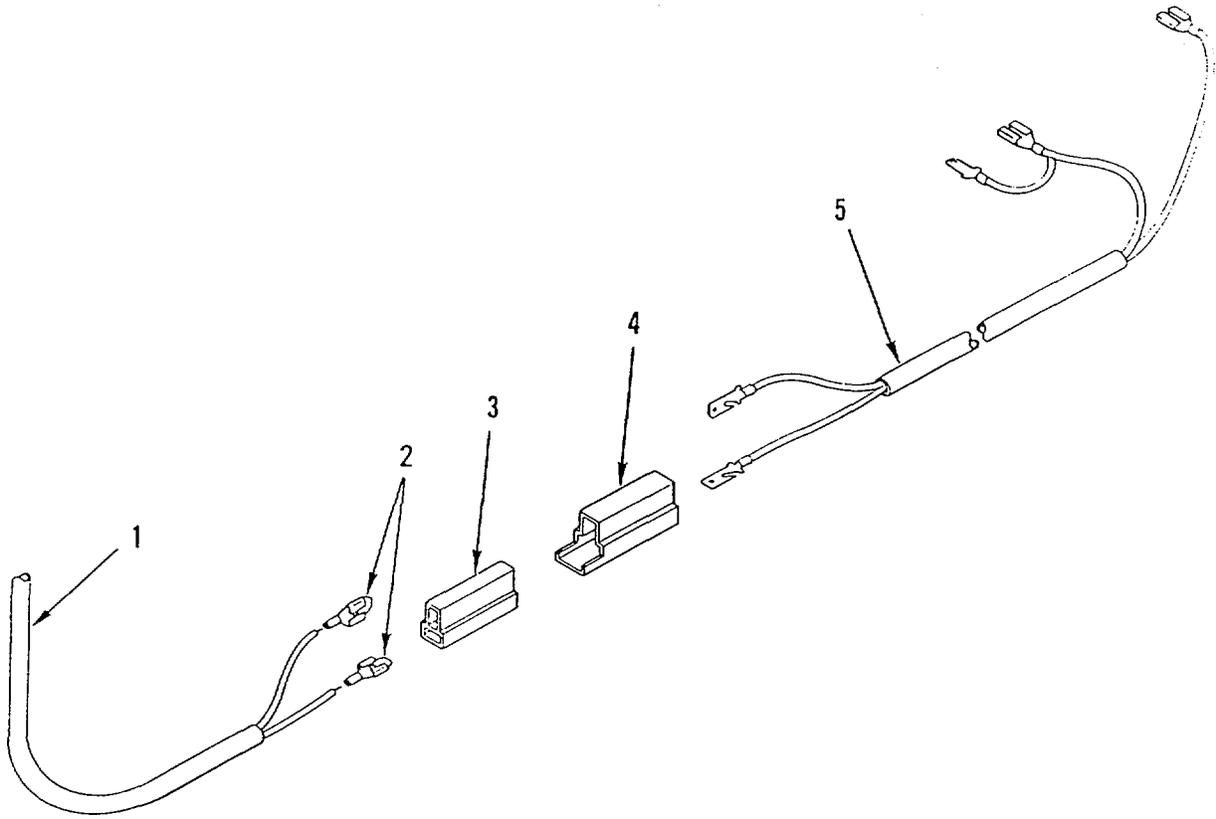
Figure 13. Headlight Wiring Harness
