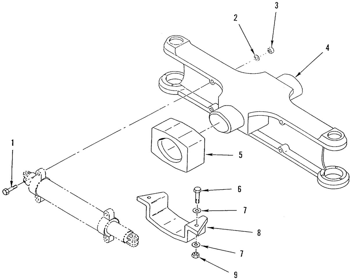
Figure 22. Steering Axle
