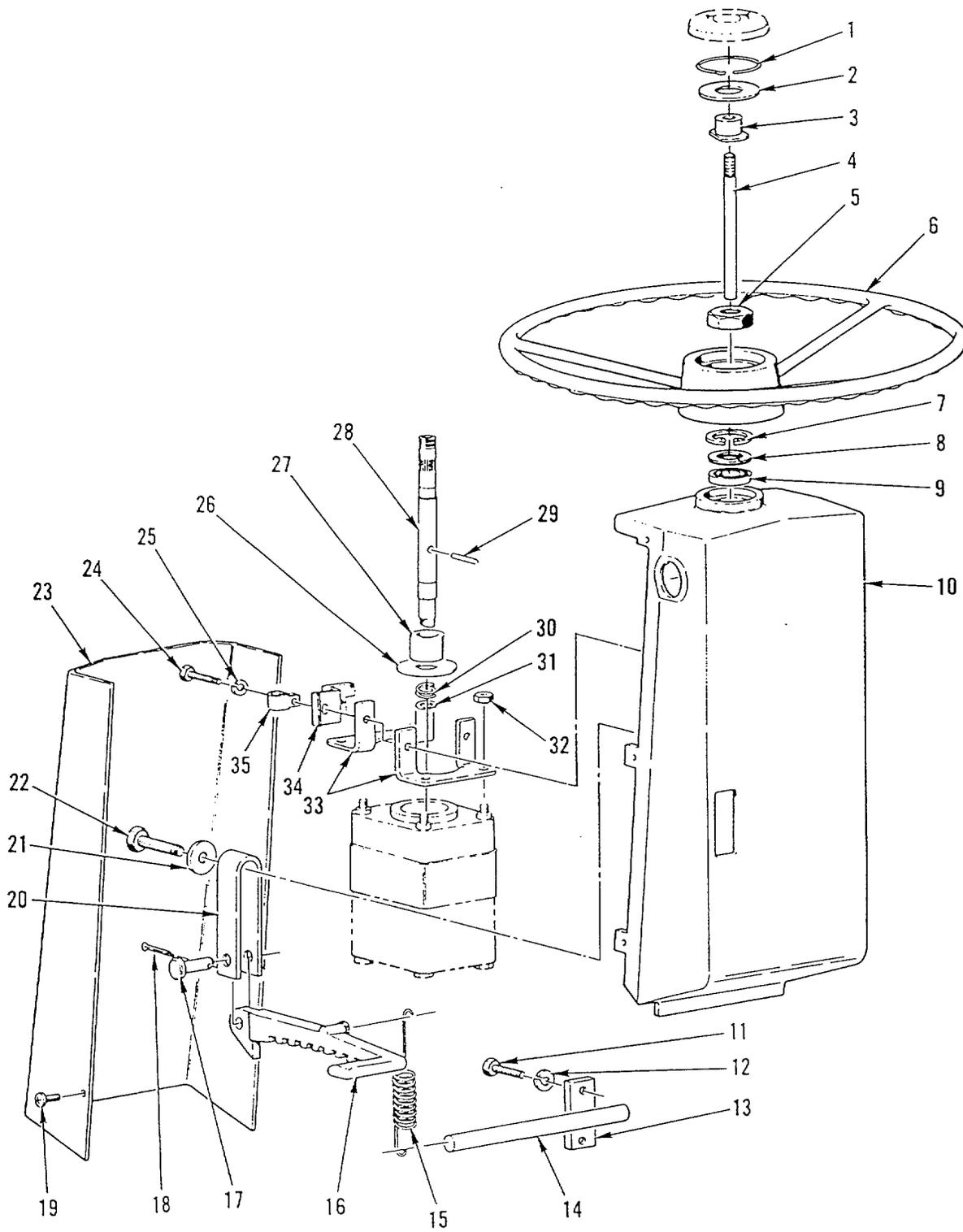
Figure 33. Steering Column Assembly
