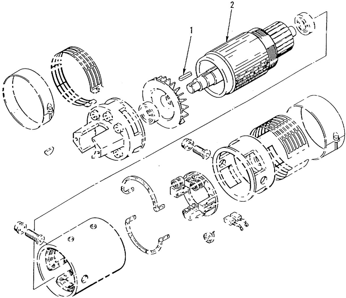
Figure 66. Hydraulic Pump Motor Armature
