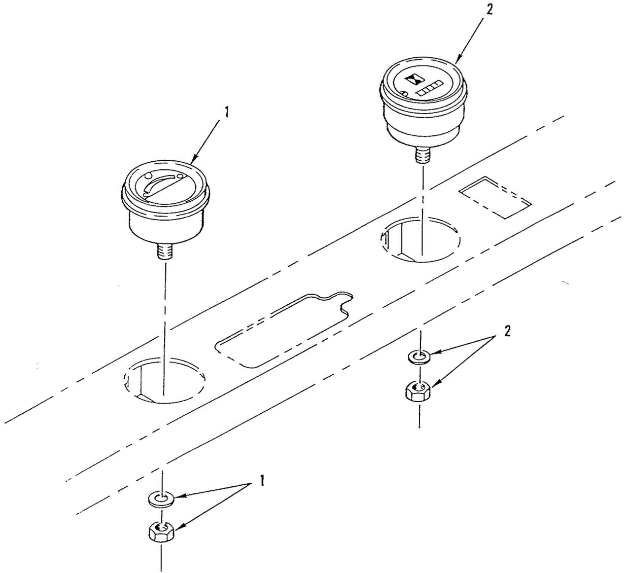
Figure 1. Instrument Installation
