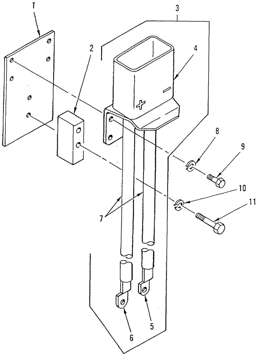
Figure 9. Battery Connector
