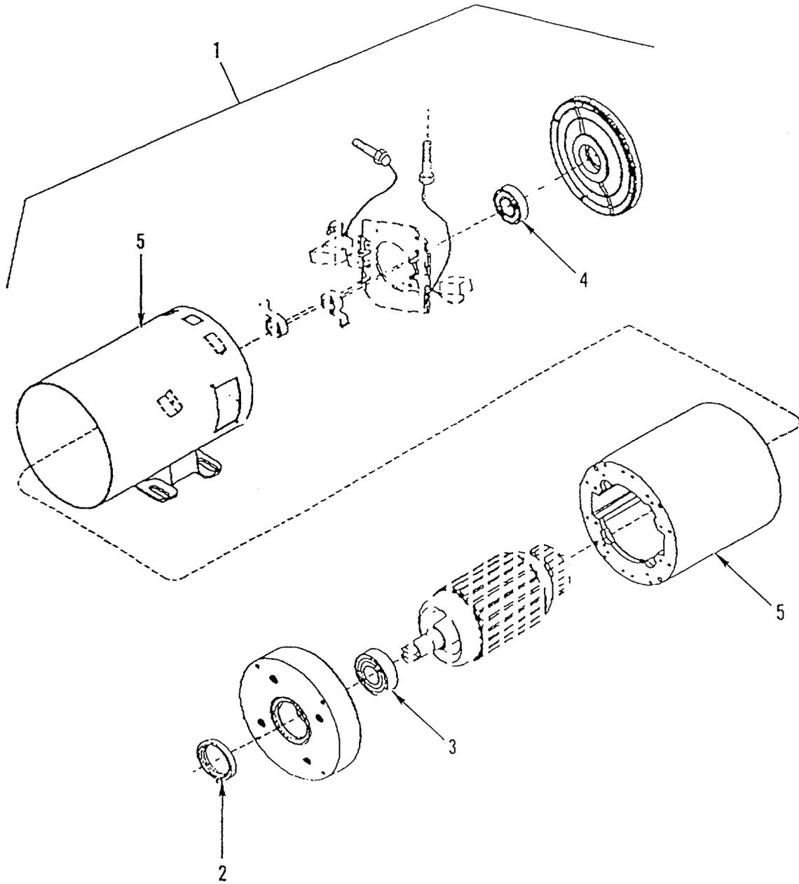
Figure 64. Steering Motor
