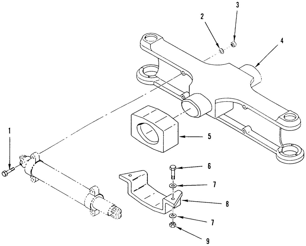
Figure 22. Steering Axle
