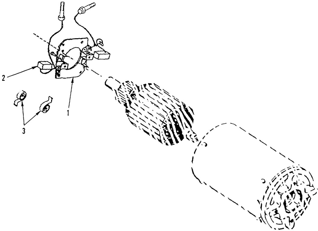
Figure 70. Steering Pump Motor Brushes
