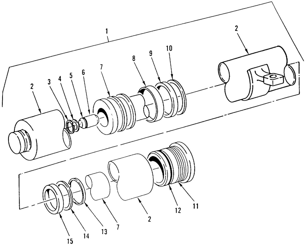
Figure 55. Free Lift Cylinder
