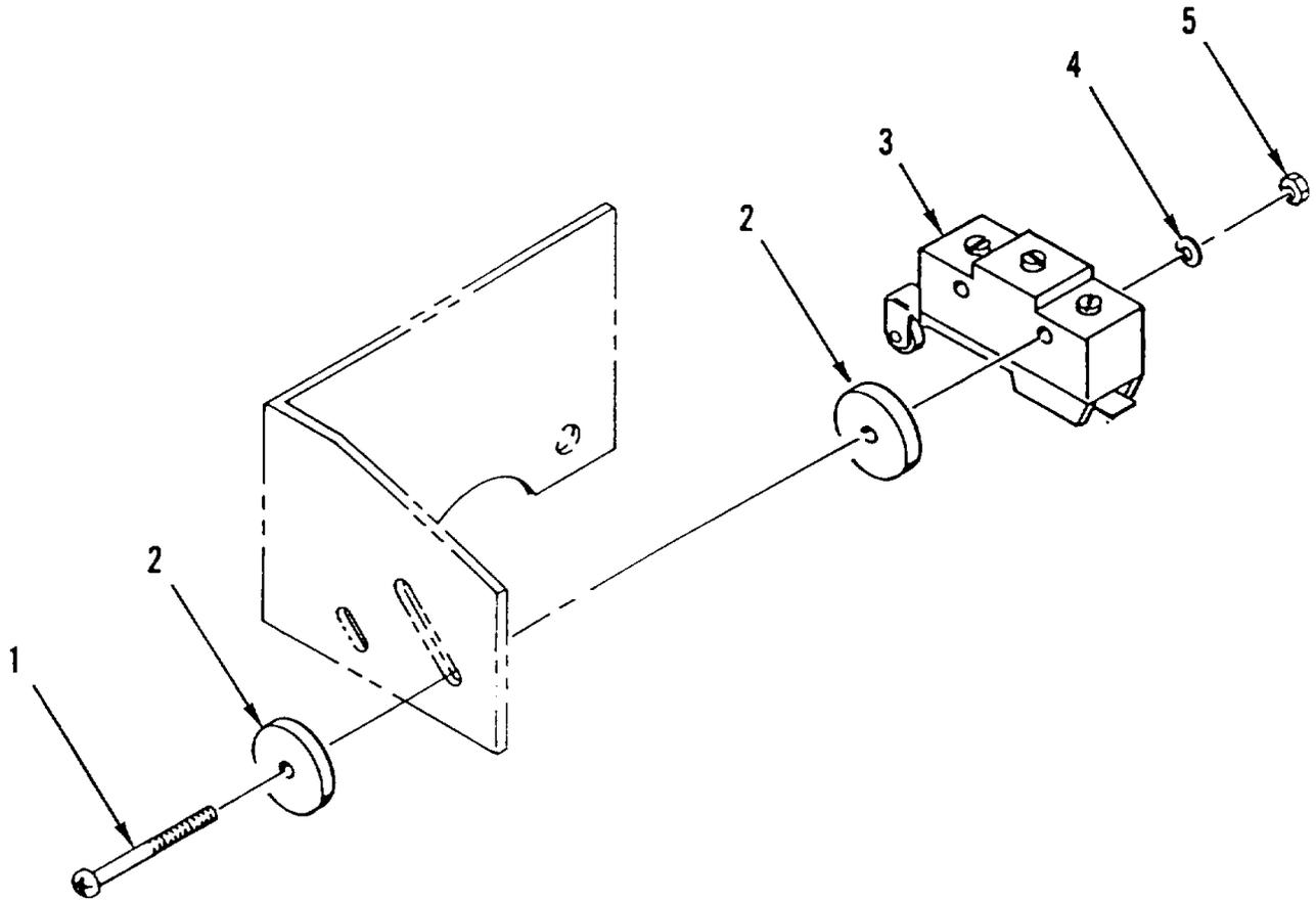
Figure 5. Brake Light Switch
