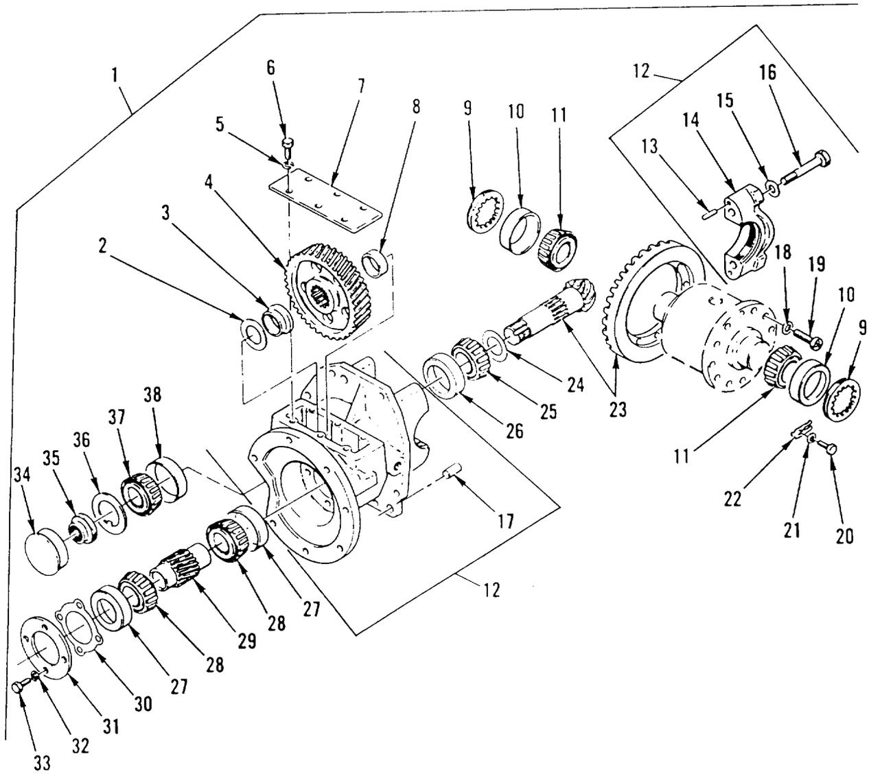
Figure 19. Transmission Assembly
