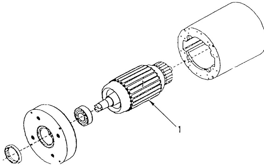
Figure 67. Steering Motor Armature
