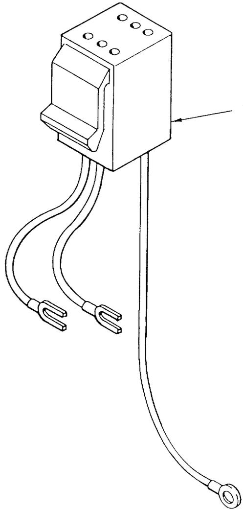
Figure 18. Control Panel Wiring Harness
