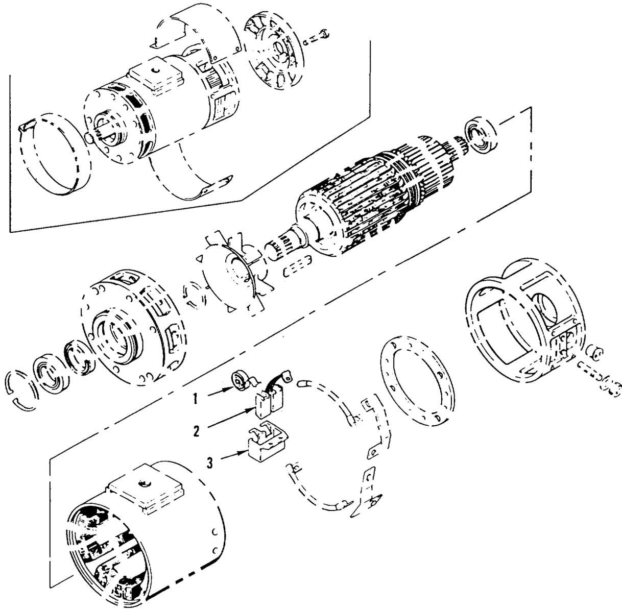
Figure 71. Traction Motor Brushes
