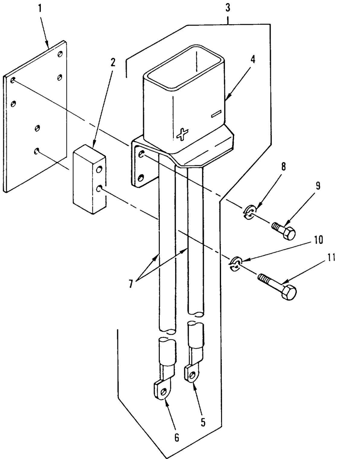
Figure 9. Battery Connector
