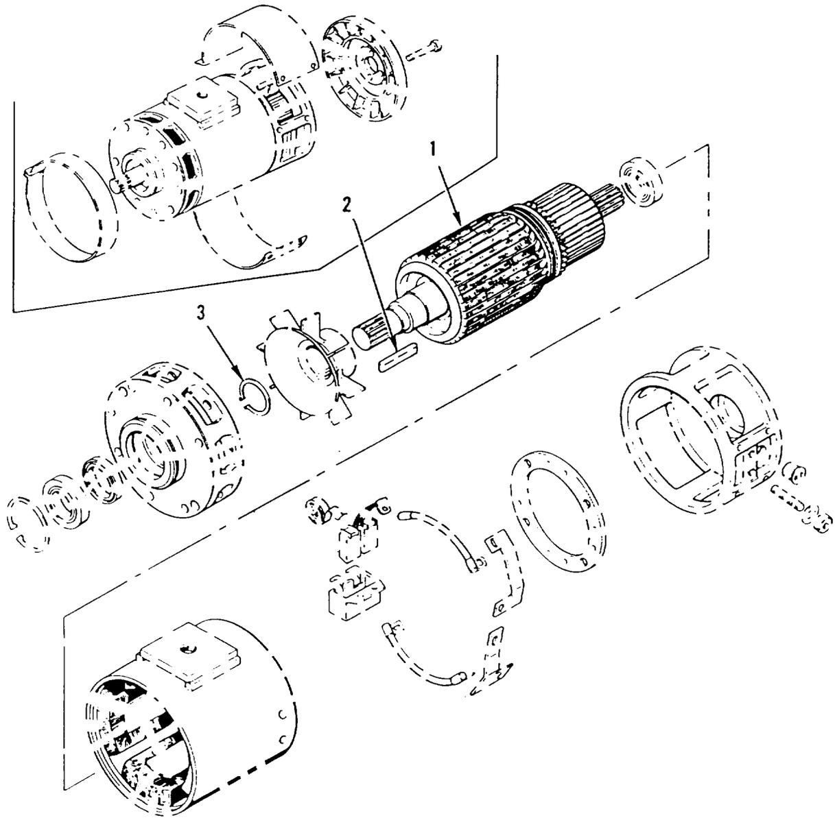
Figure 68. Traction Motor Armature
