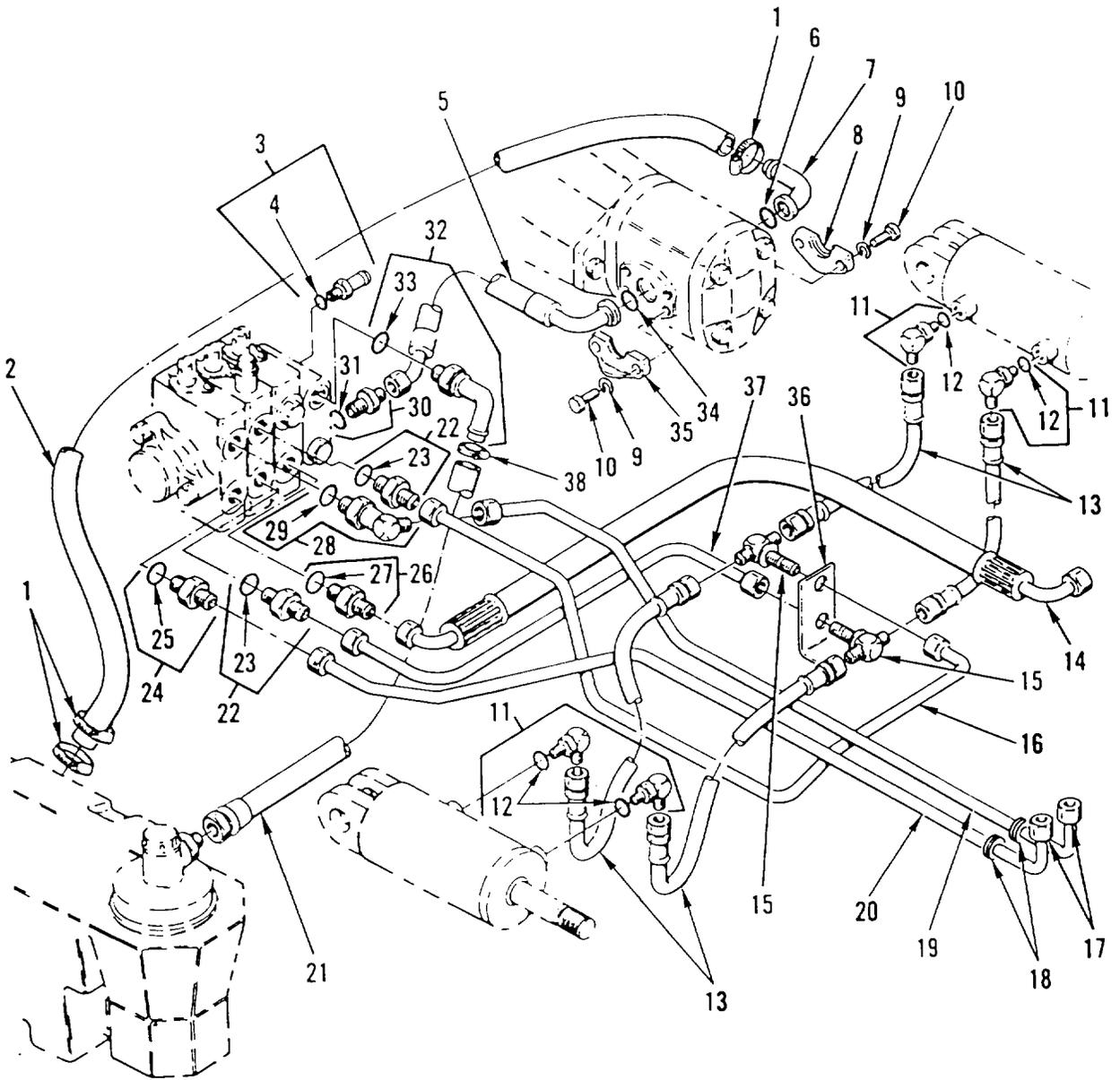
Figure 61. Hydraulic Assembly
