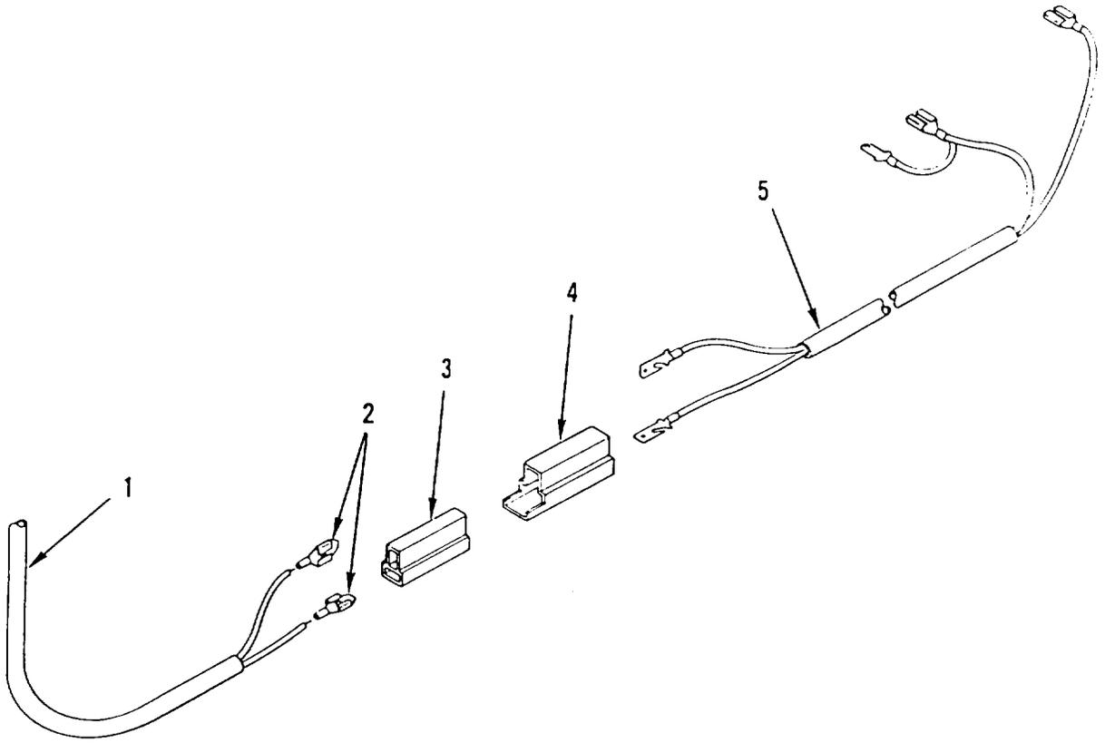
Figure 13. Headlight Wiring Harness
