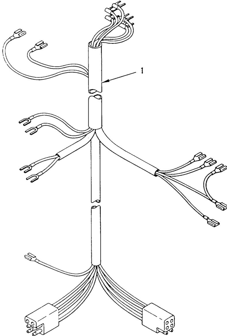
Figure 16. Steering Column Wiring Harness
