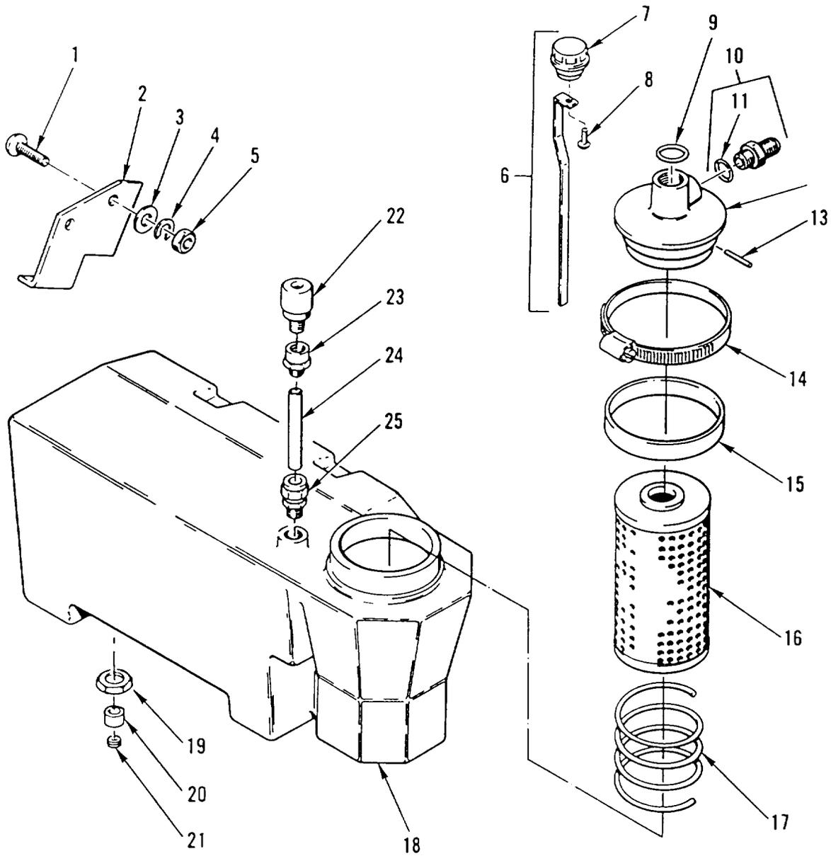
Figure 63. Hydraulic Tank
