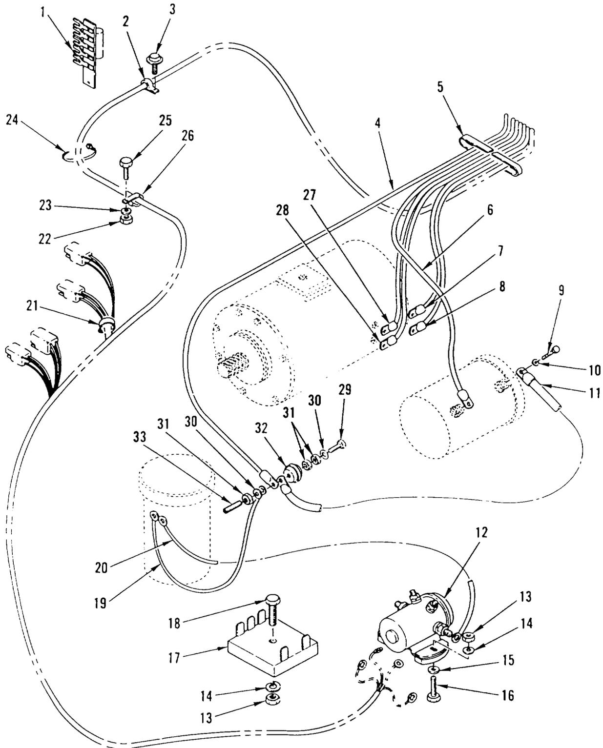
Figure 10. Electrical Installation
