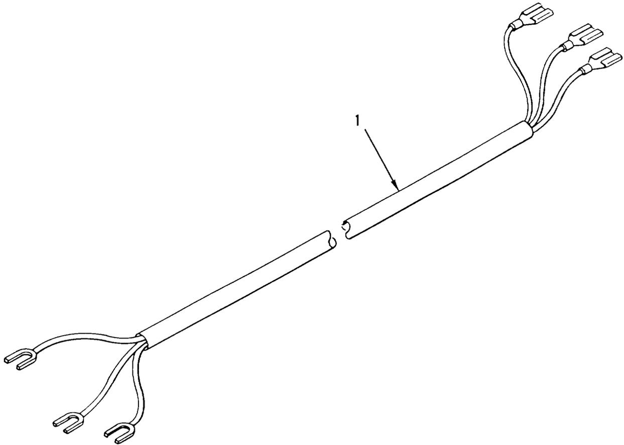
Figure 12. Instrument Panel Wiring Harness
