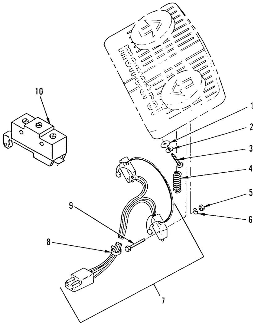
Figure 81. Directional Control Switch
