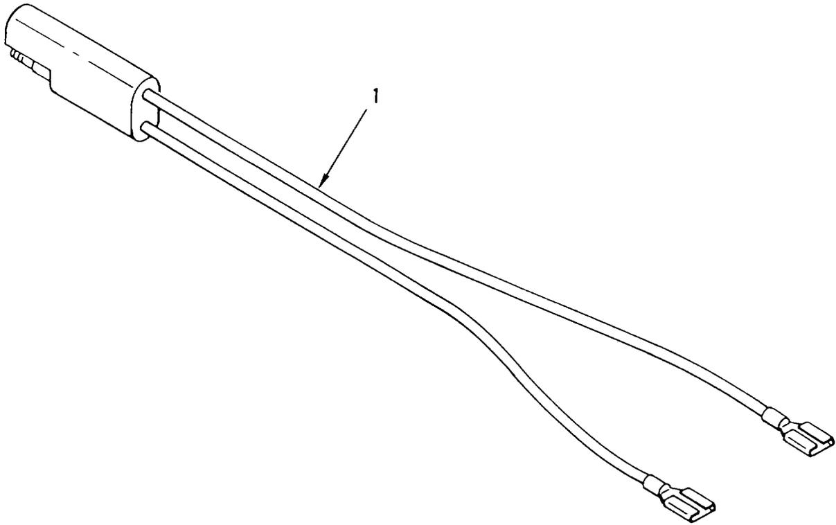
Figure 15. Seat Brake Wiring Harness
