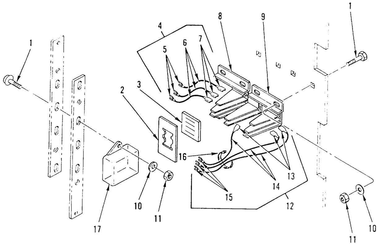
Figure 80. Control Valve Blade Switches
