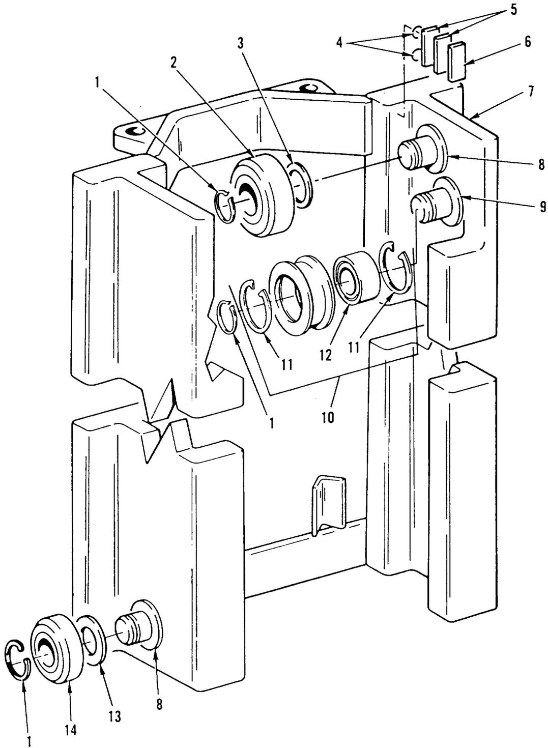
Figure 50. Intermediate Assembly
