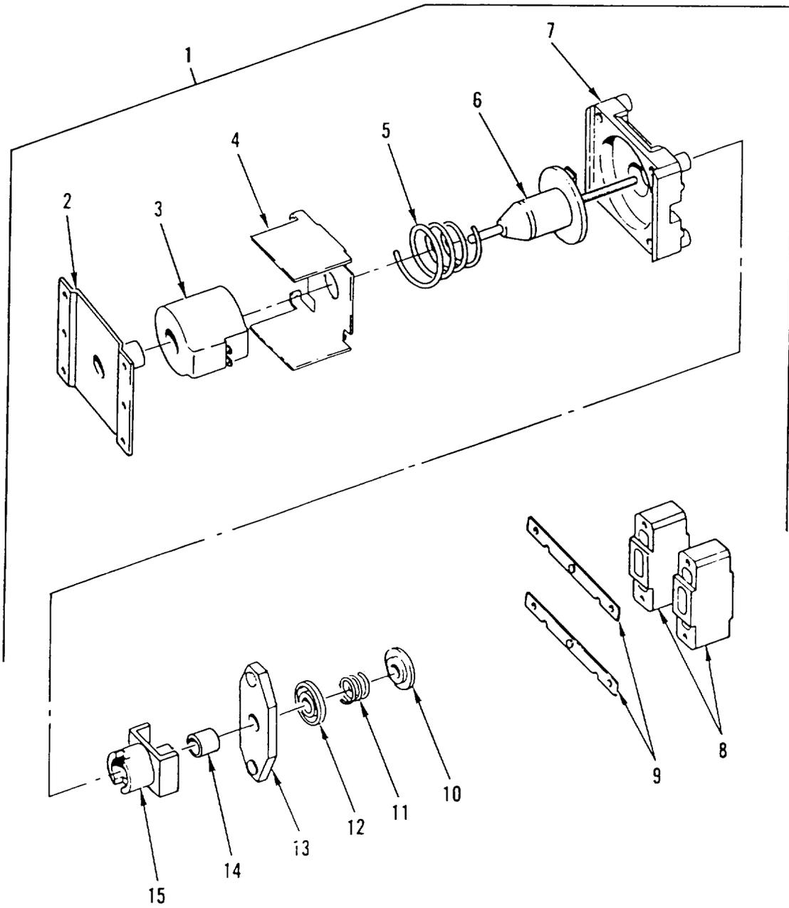
Figure 77. 1a/FW/Pump Contactor
