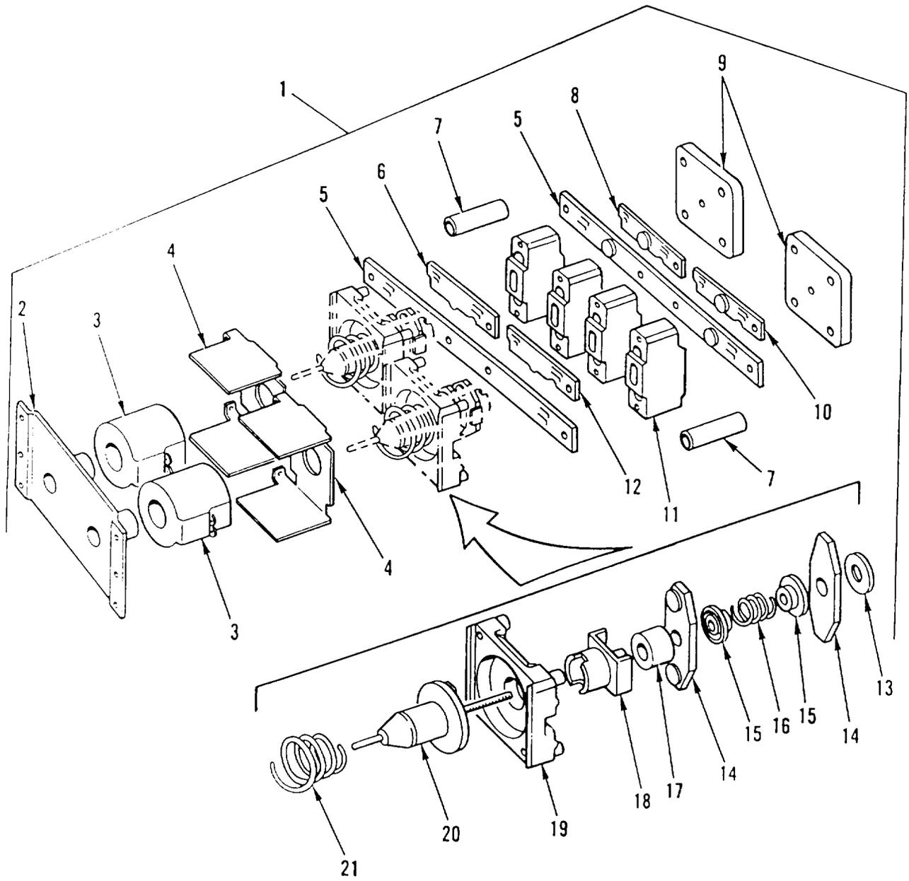
Figure 76. Forward/Reverse Contactor
