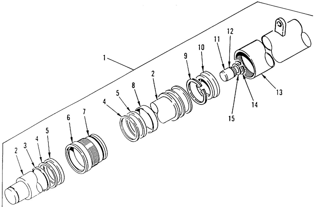
Figure 53. Main Lift Cylinder
