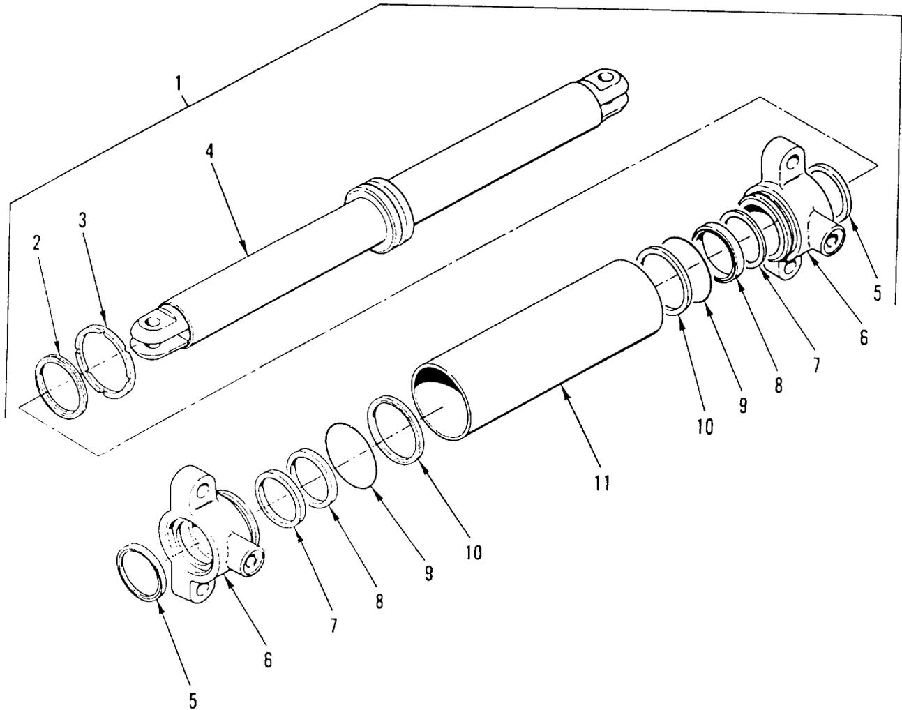
Figure 36. Steering Cylinder
