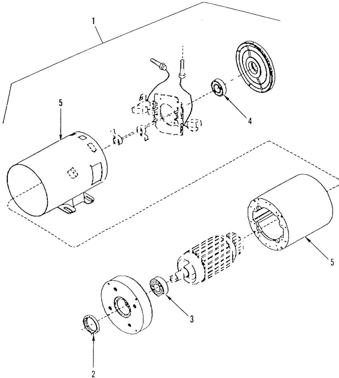
Figure 64. Steering Motor
