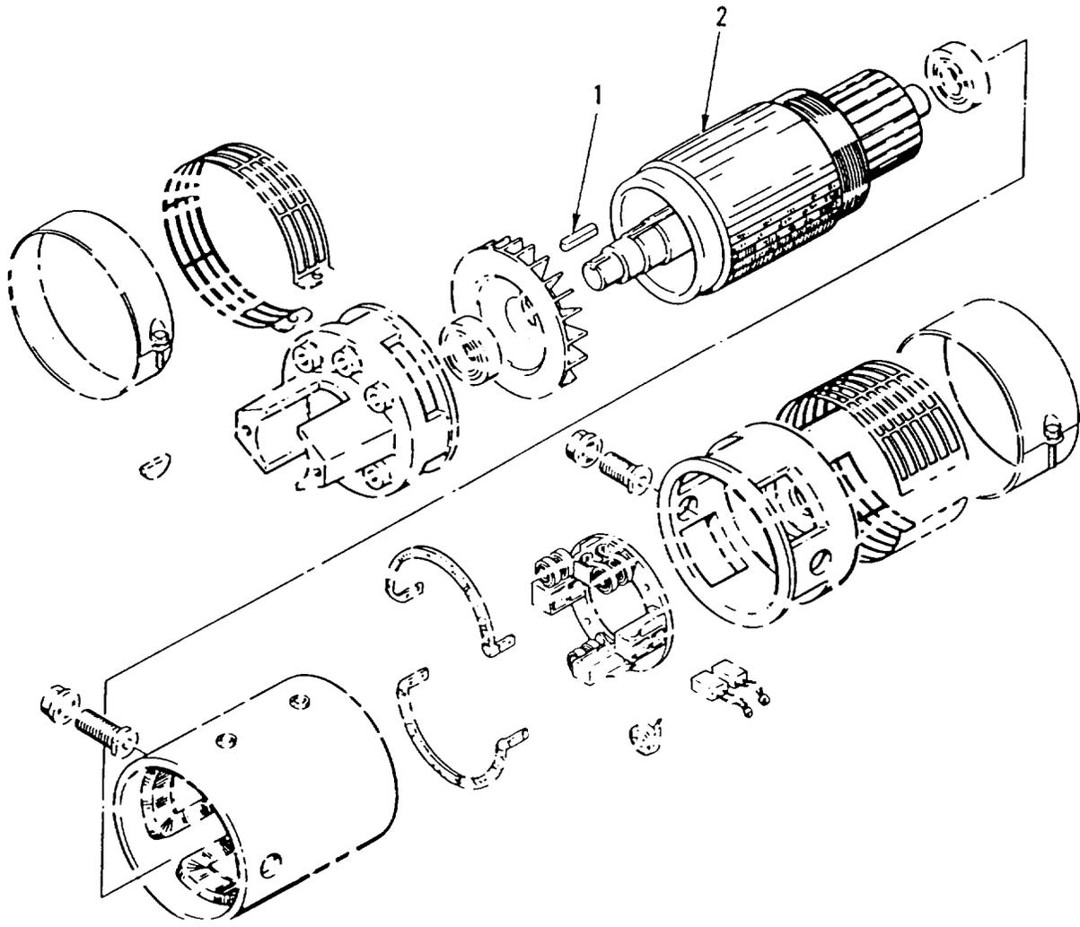
Figure 66. Hydraulic Pump Motor Armature
