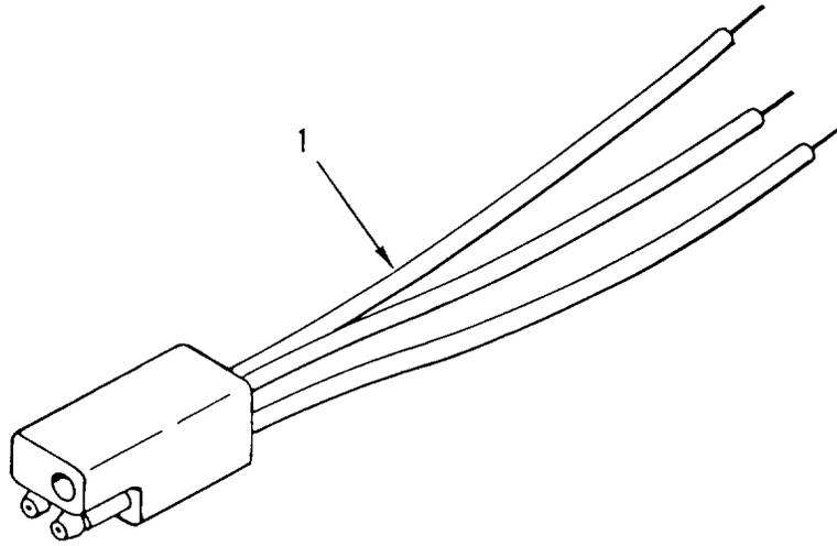
*Figure 17. Potentiometer Wiring Harness*
