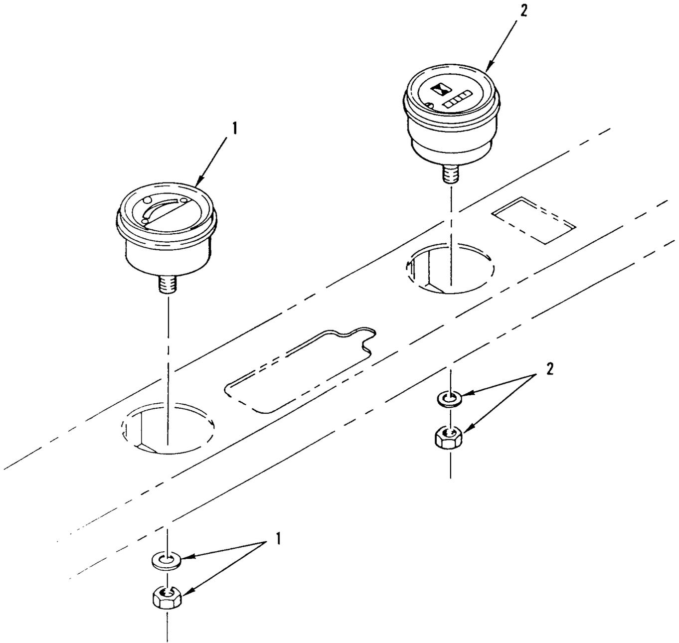
Figure 1. Instrument Installation
