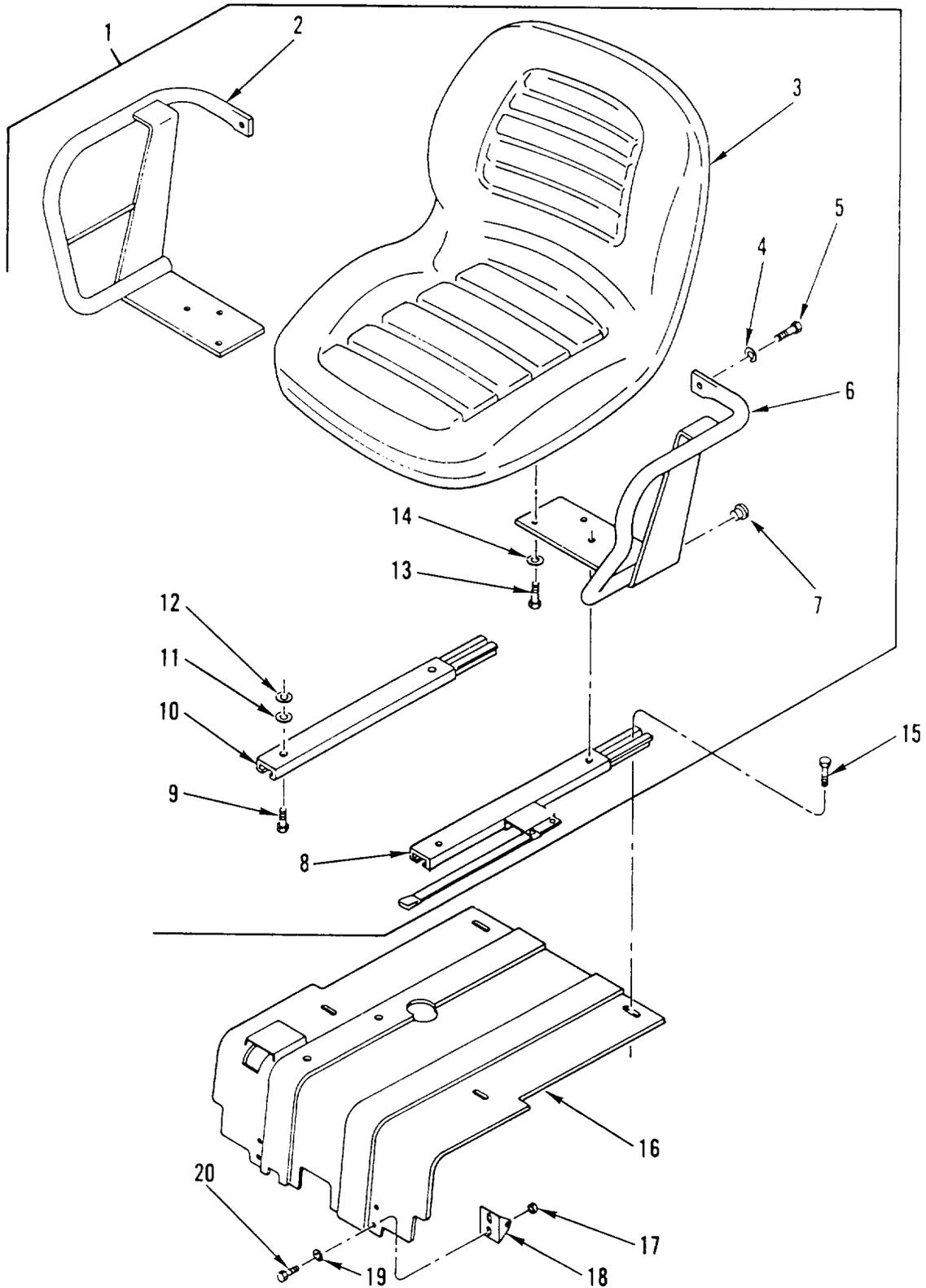
Figure 41. Seat Assembly (Sheet 1 of 2)
