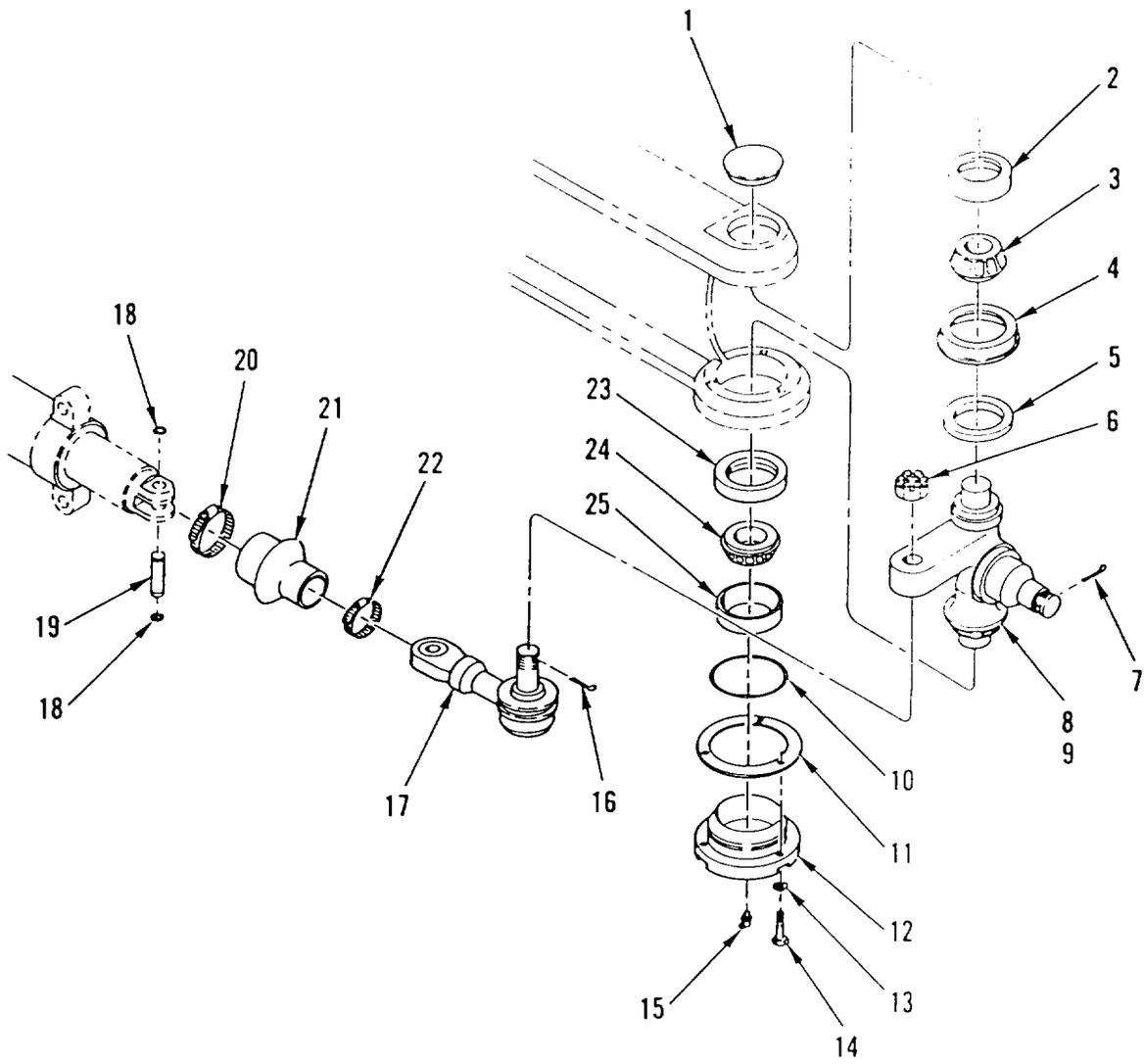
Figure 23. Steering Axle & Tie Rod Assembly
