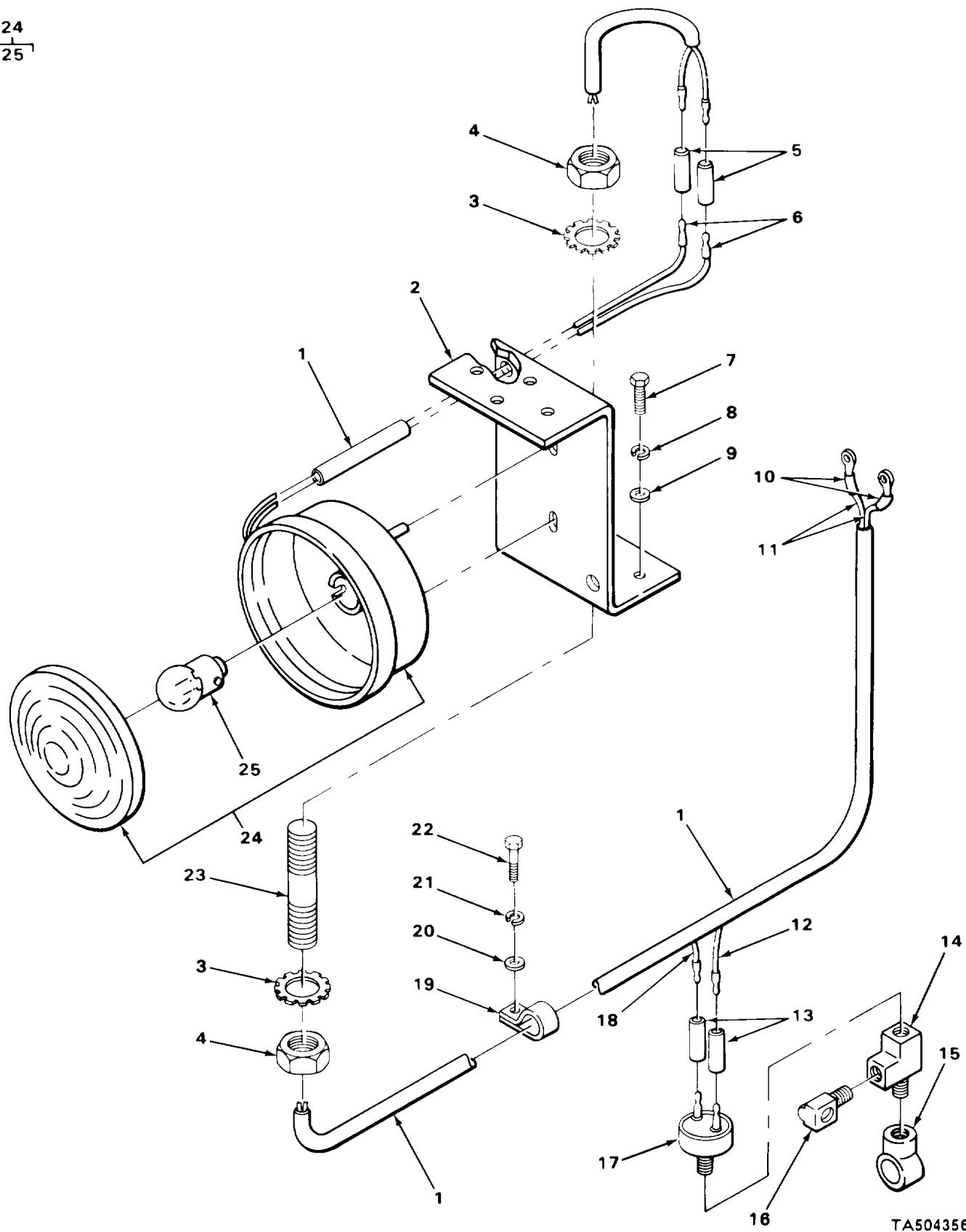
FIGURE 38. TAILLIGHT ASSEMBLY AND MOUNTING PARTS.
