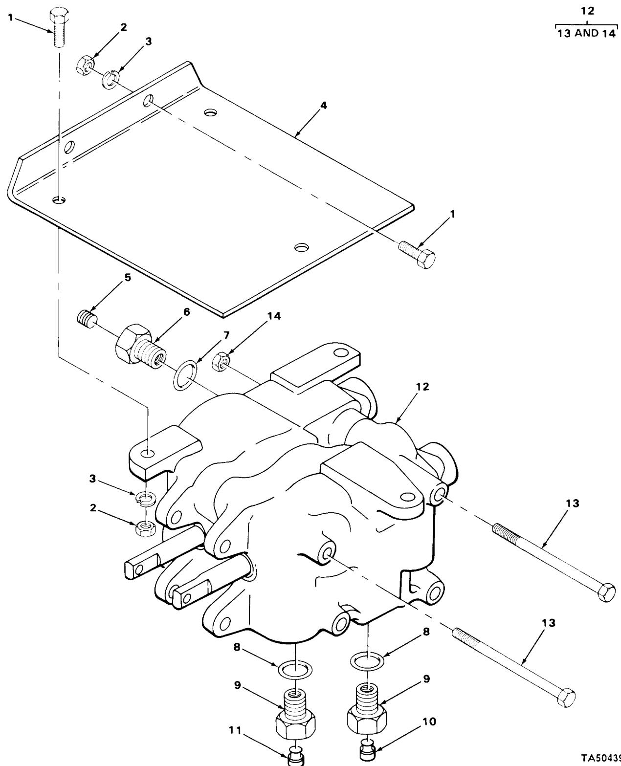
FIGURE 80. CONTROL VALVE ASSEMBLY AND RELATED PARTS.
