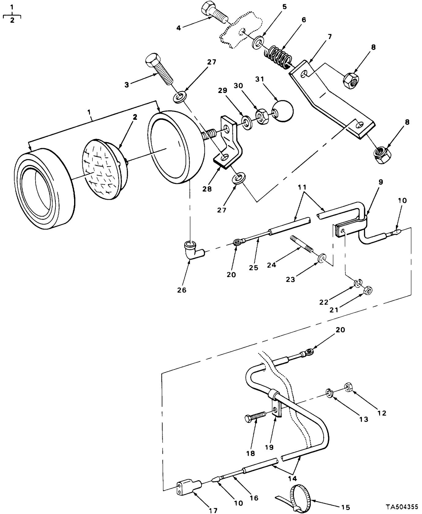
FIGURE 37. HEADLIGHT ASSEMBLY AND MOUNTING PARTS.
