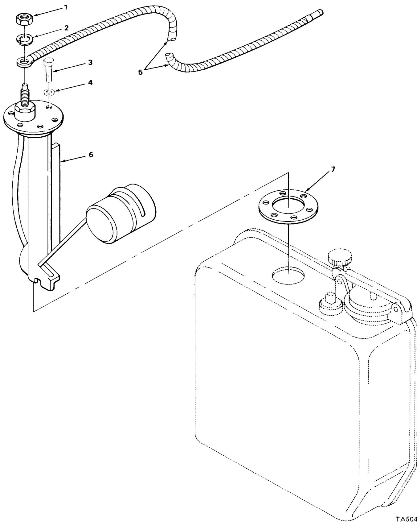
FIGURE 39. FUEL TANK TRANSMITTER AND RELATED PARTS.
