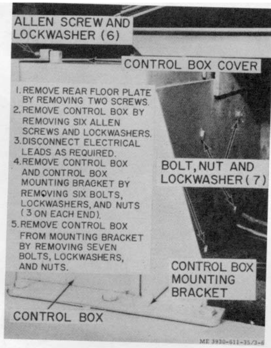
Figure 3-6. Control box, removal and installation.
