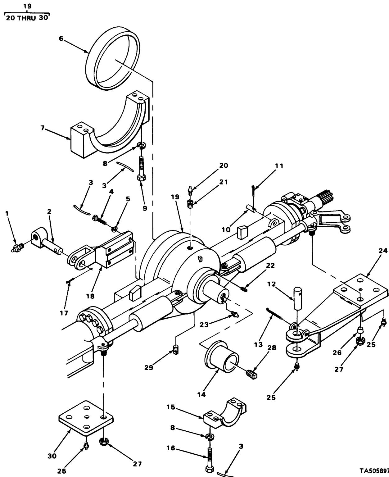
FIGURE 58. FRONT AND REAR AXLE.
