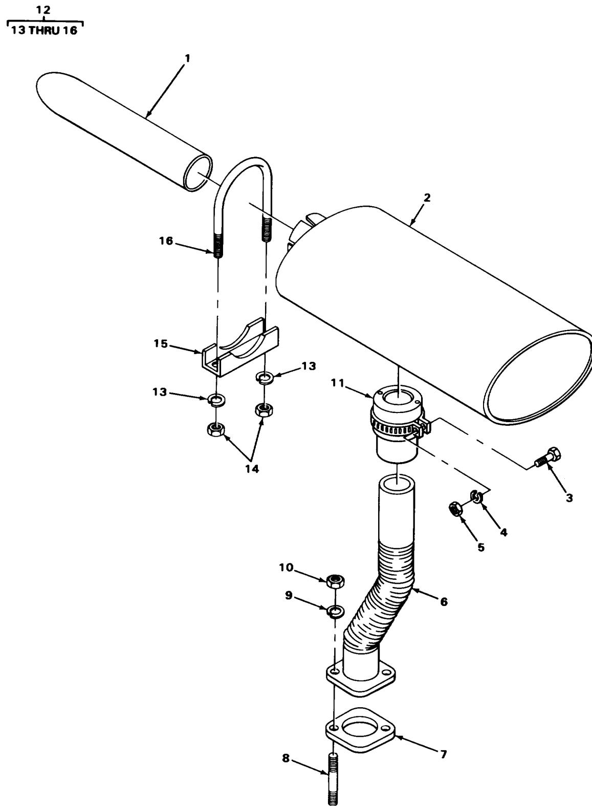
**FIGURE 18. MUFFLERS AND PIPES.**
