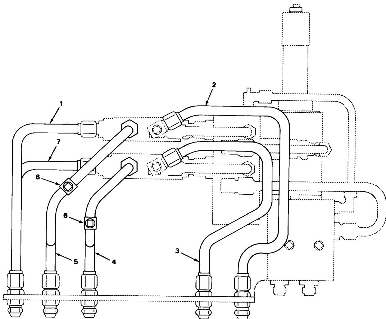
FIGURE 80. LOCK CYLINDER TUBING.
