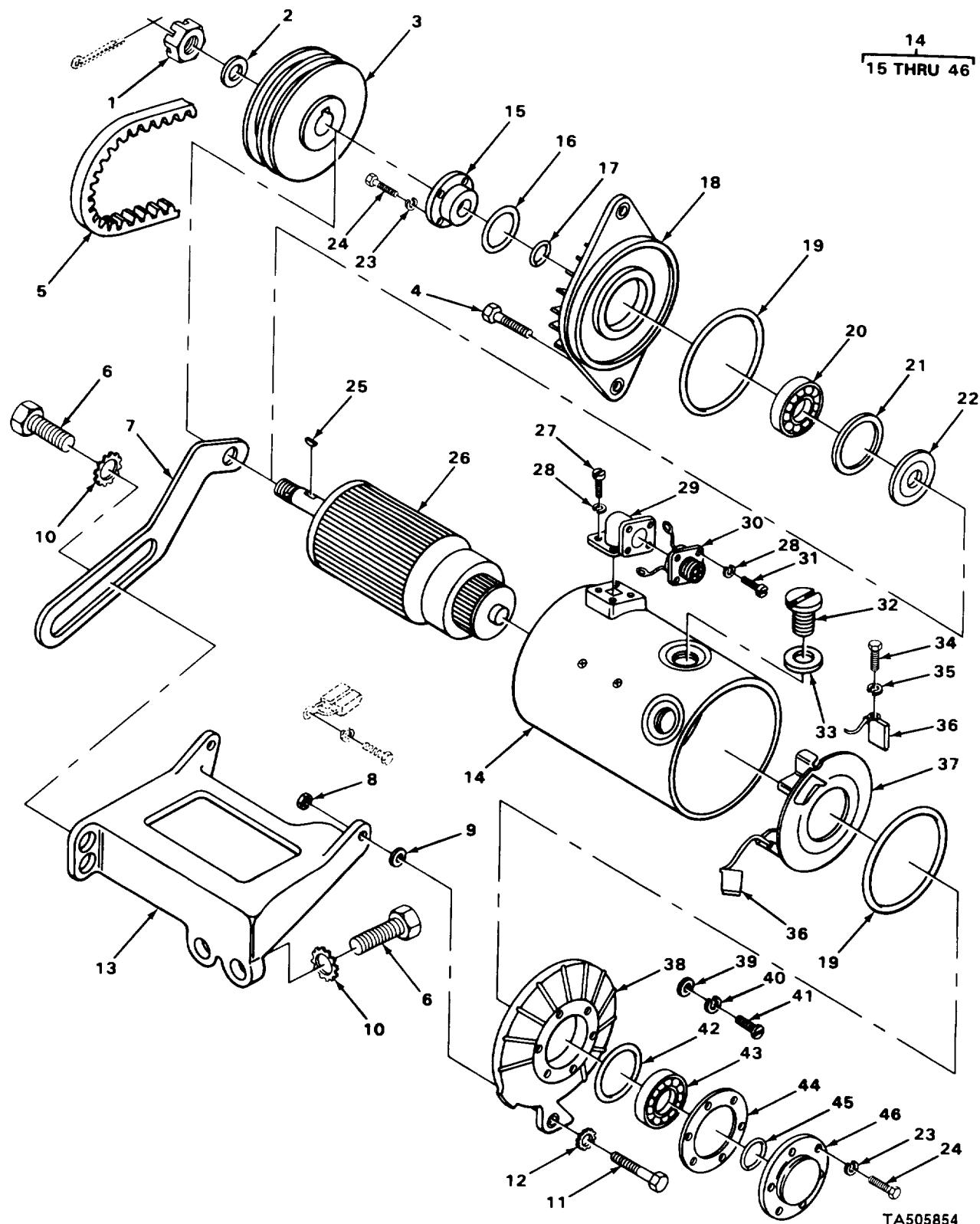
FIGURE 29. GENERATOR ASSEMBLY (MODEL RTL10).
