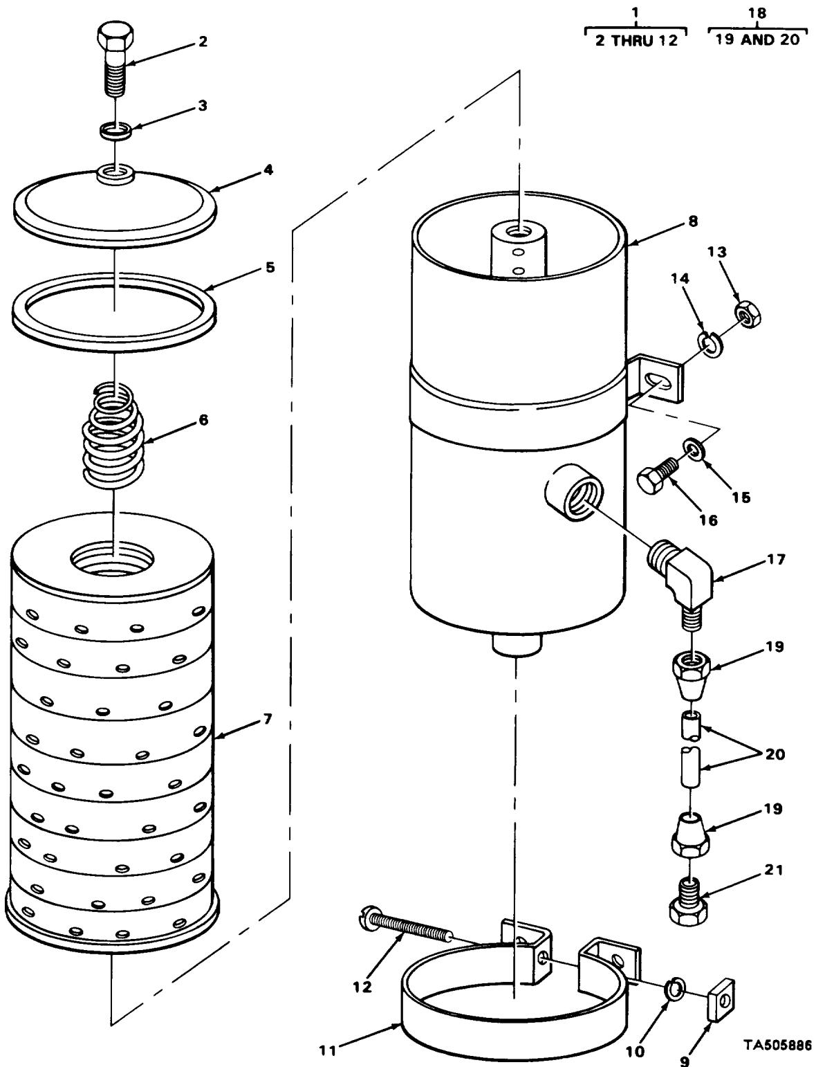
FIGURE 52. TRANSMISSION OIL FILTER.
