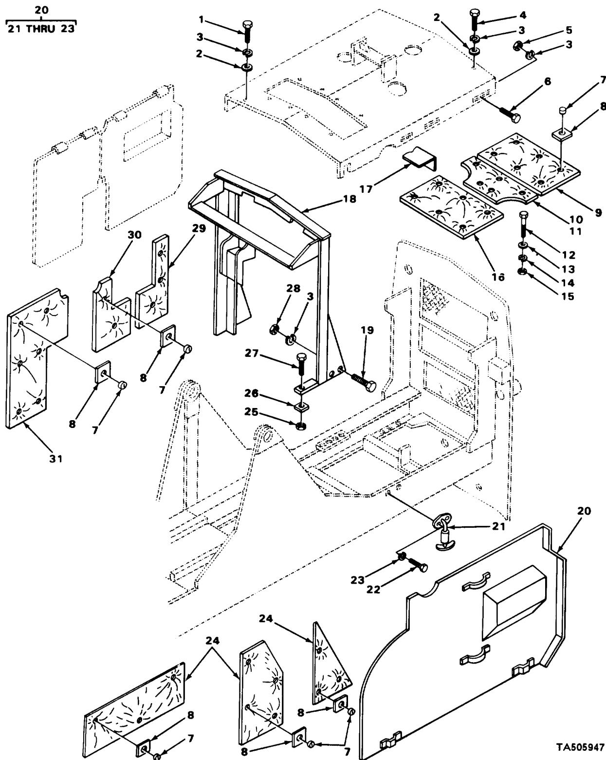
**FIGURE 94. ENGINE HOOD AND SIDE MOUNTING HARDWARE AND ABSORPTION.**
