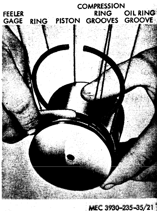
Figure 21. Measuring ring groove clearance.
