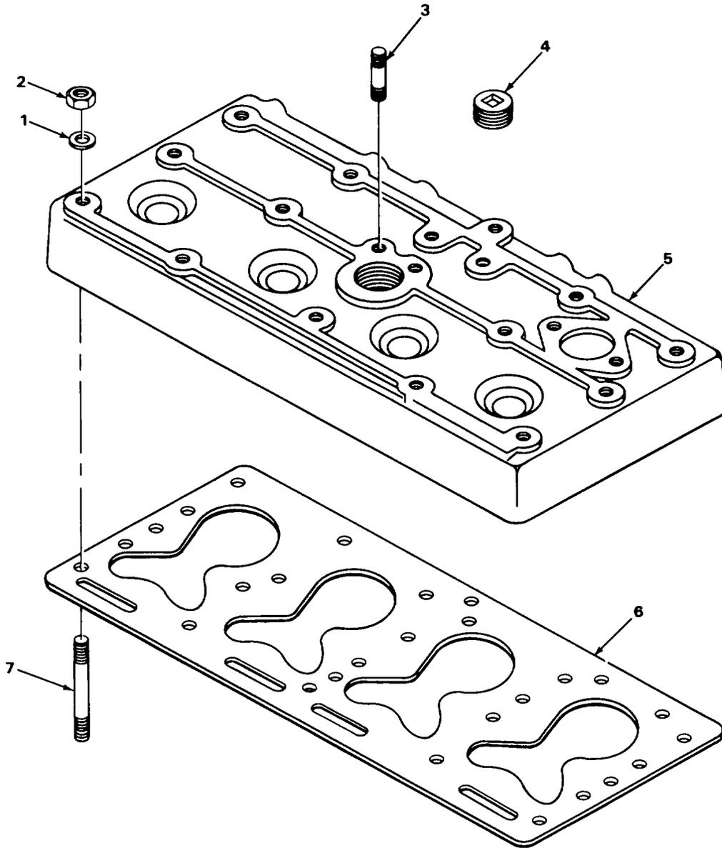
FIGURE 3. CYLINDER HEAD.
