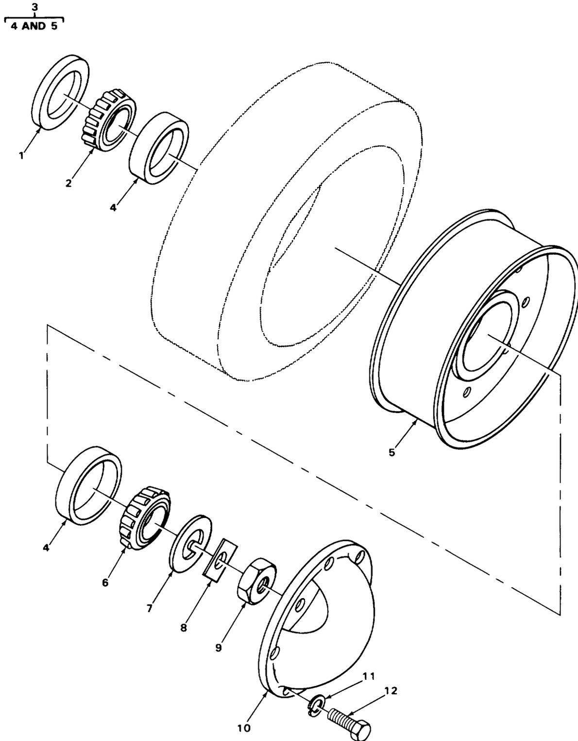
FIGURE 69. REAR AXLE WHEELS AND BEARINGS, MODEL MHE 191.
