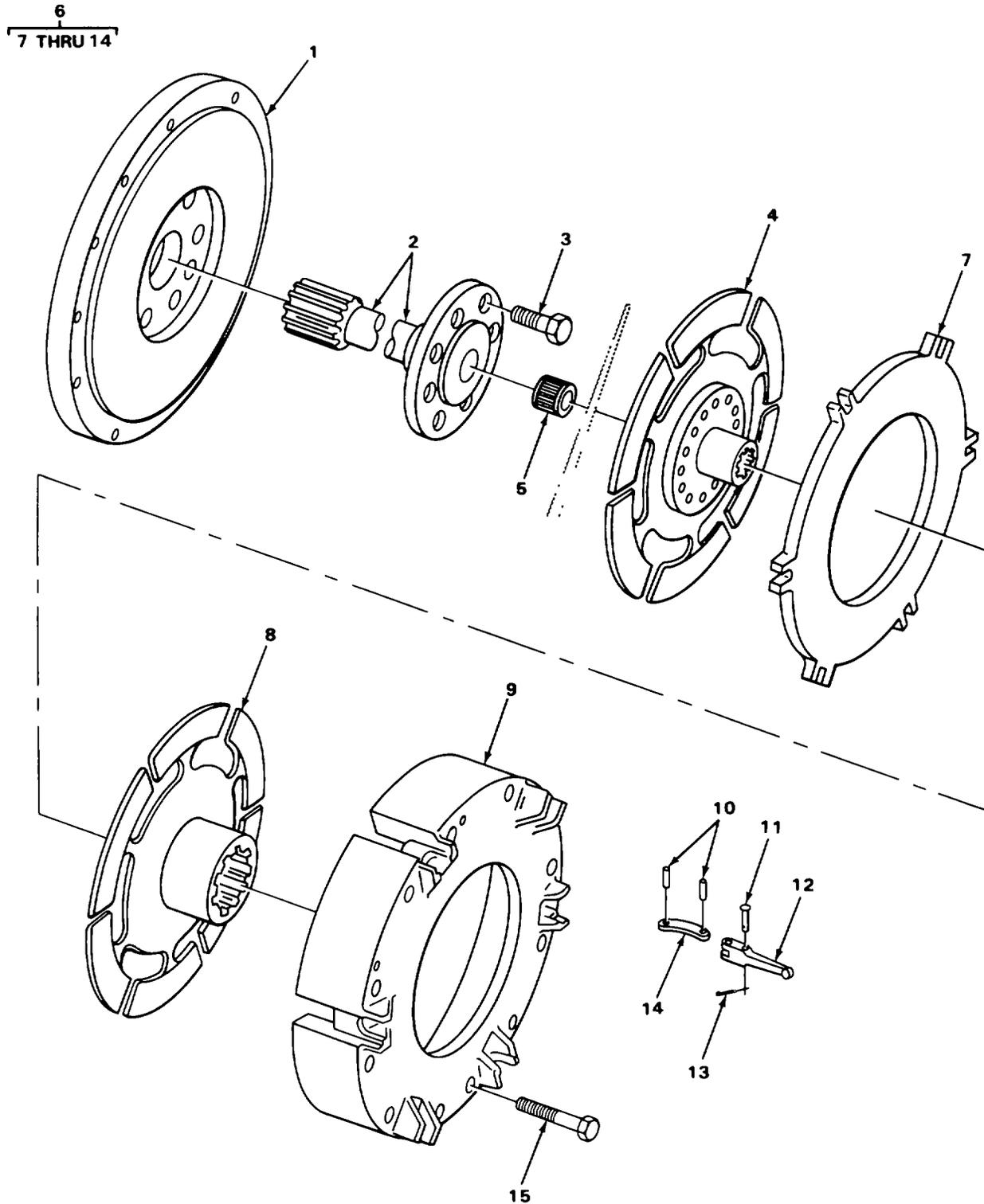
FIGURE 45. CLUTCH ASSEMBLY.
