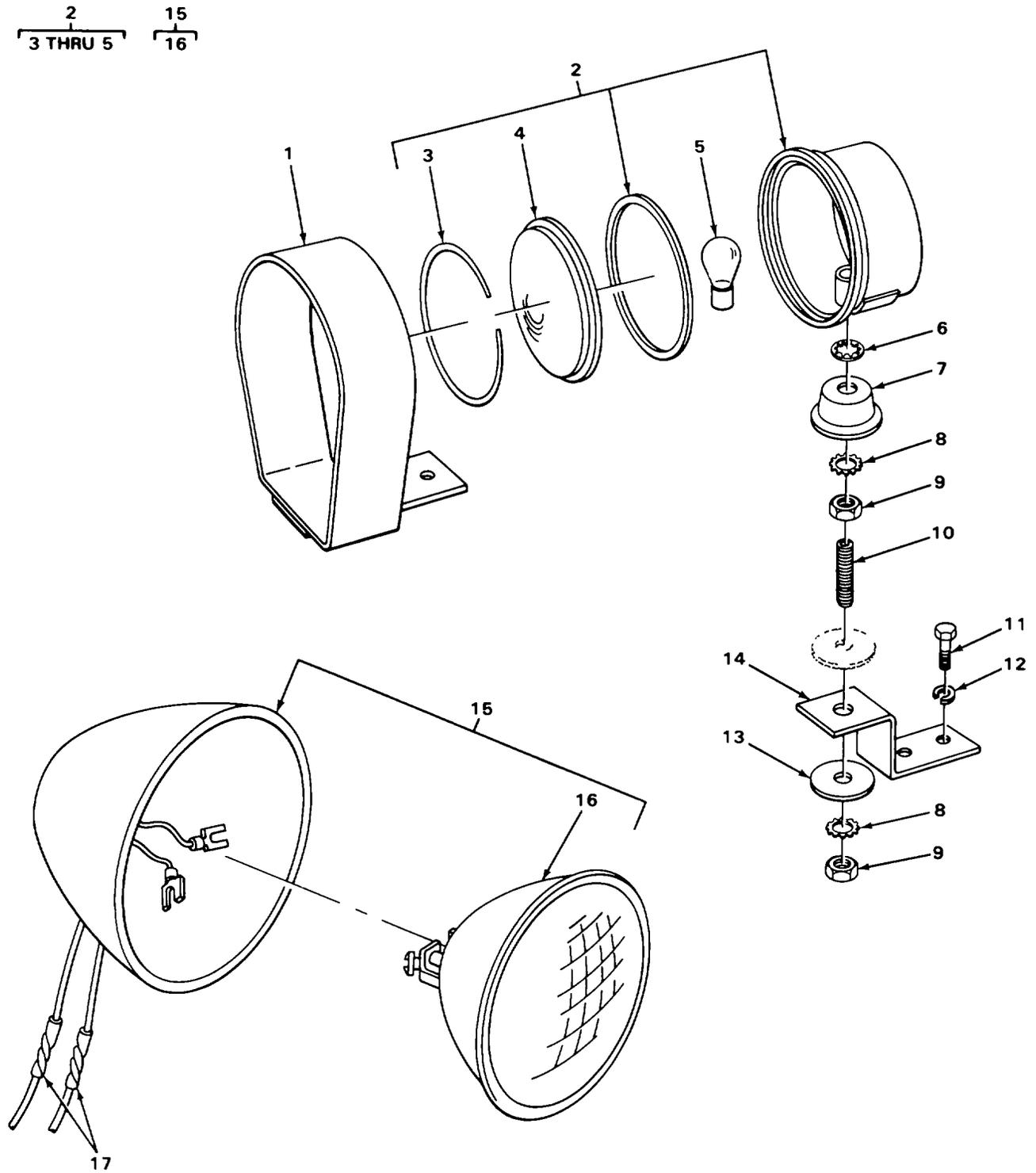
FIGURE 37. STOP AND TAILLIGHT AND HEADLIGHT.
