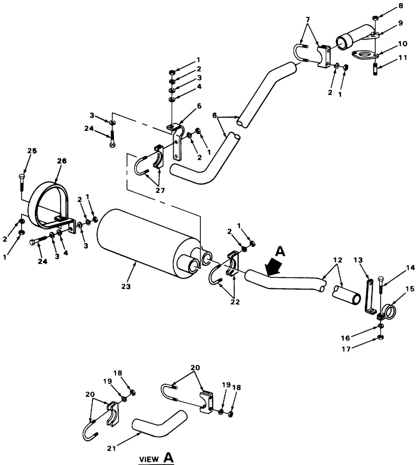
FIGURE 23. MUFFLER AND PIPES.
