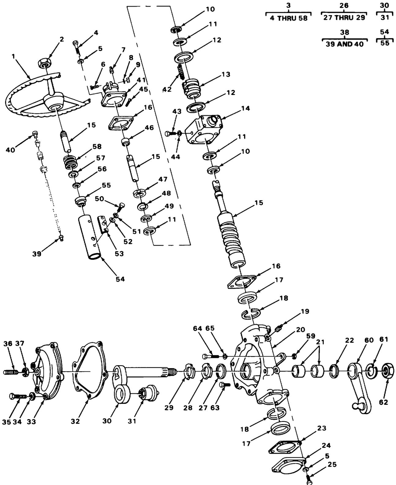
FIGURE 72. STEERING GEAR.
