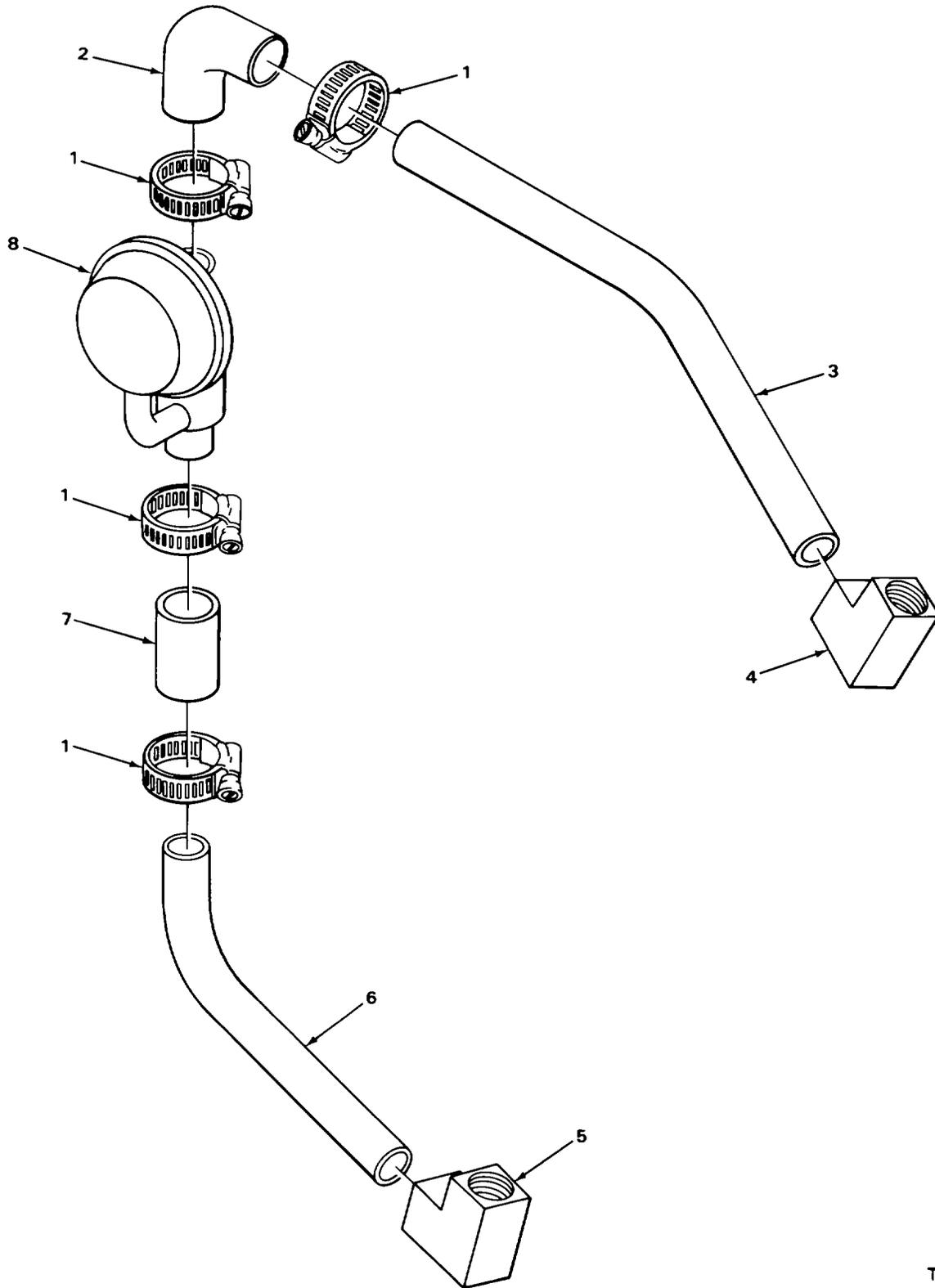
FIGURE 4. CRANKCASE VENTILATION.
