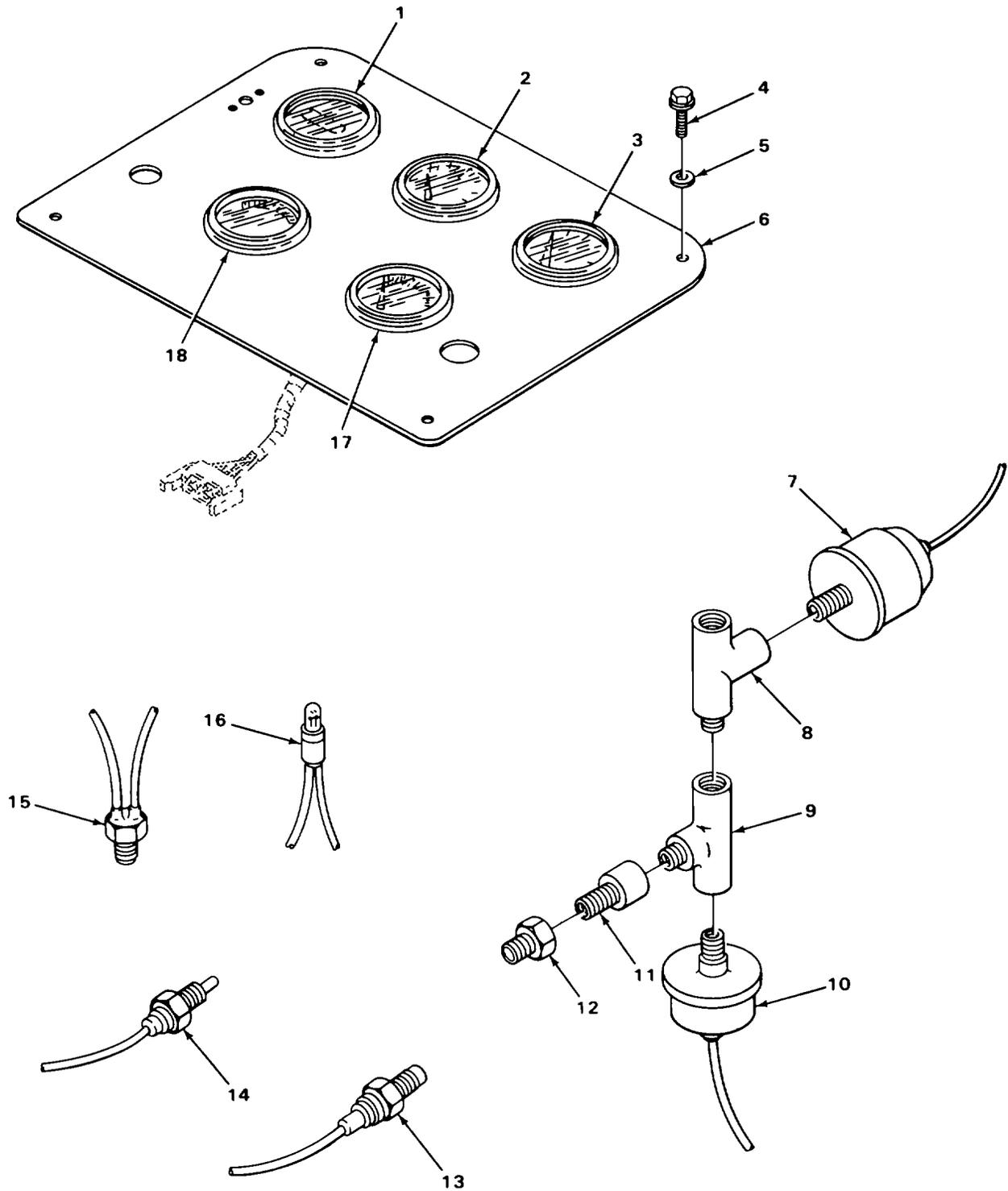
FIGURE 35. INSTRUMENT PANEL, GAGES, AND WARNING SWITCHES.
