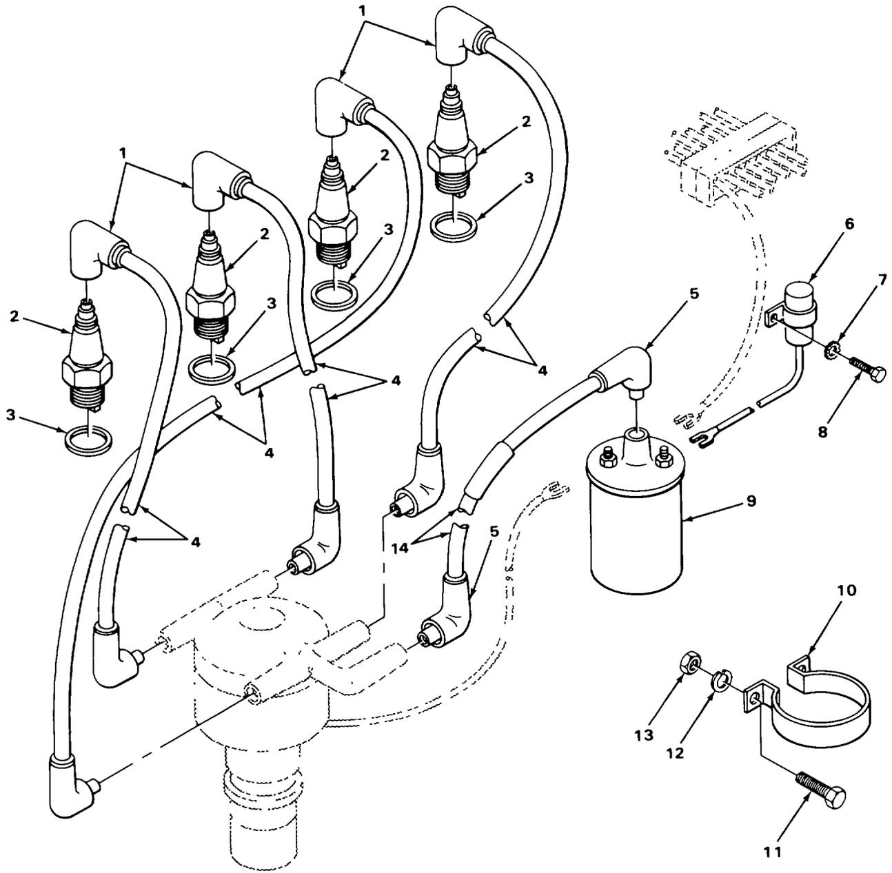
FIGURE 34. SPARK PLUG, COIL.
