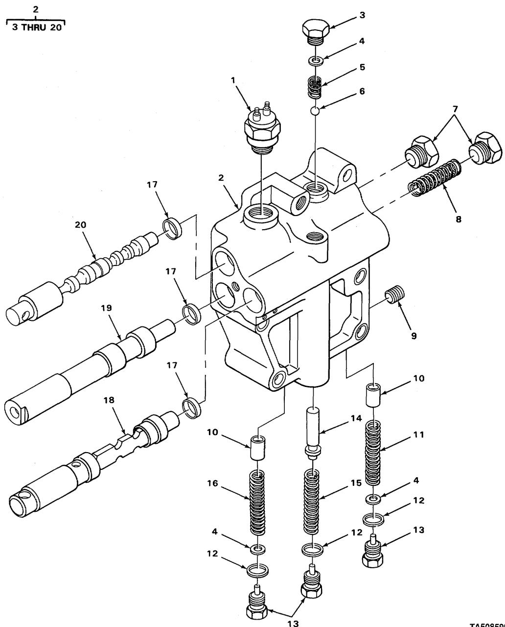
FIGURE 38. CONTROL VALVE (MHE178 AND MHE178A).
