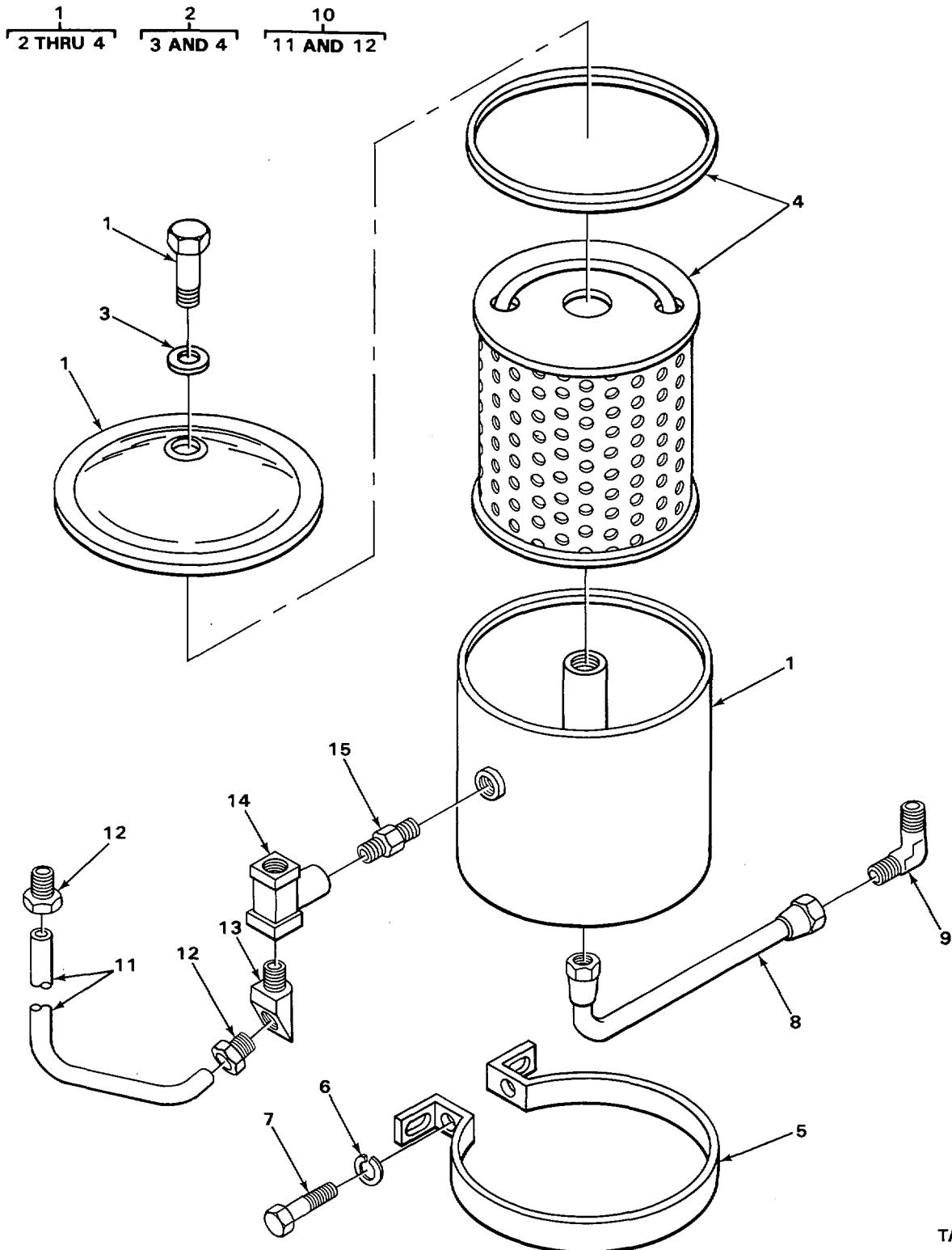
FIGURE 7. OIL FILTER AND LINES.
