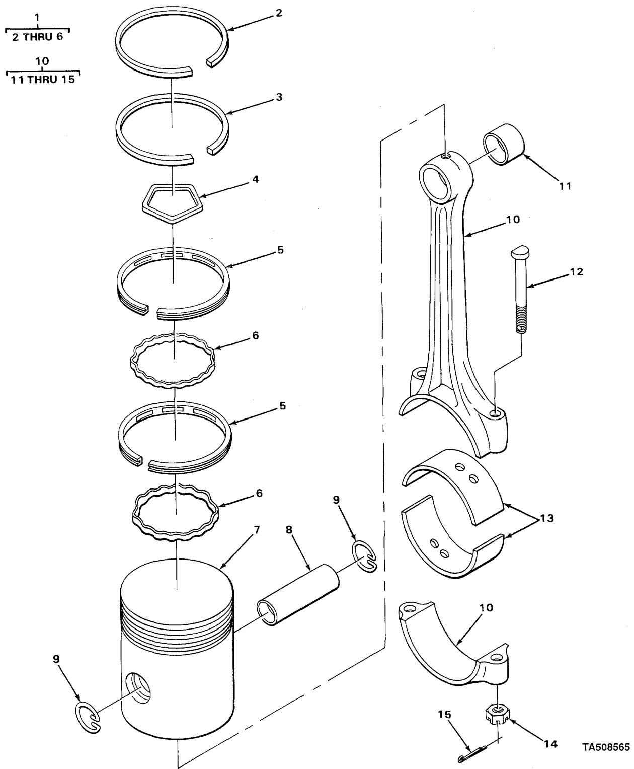
FIGURE 4. PISTON AND CONNECTING ROD.
