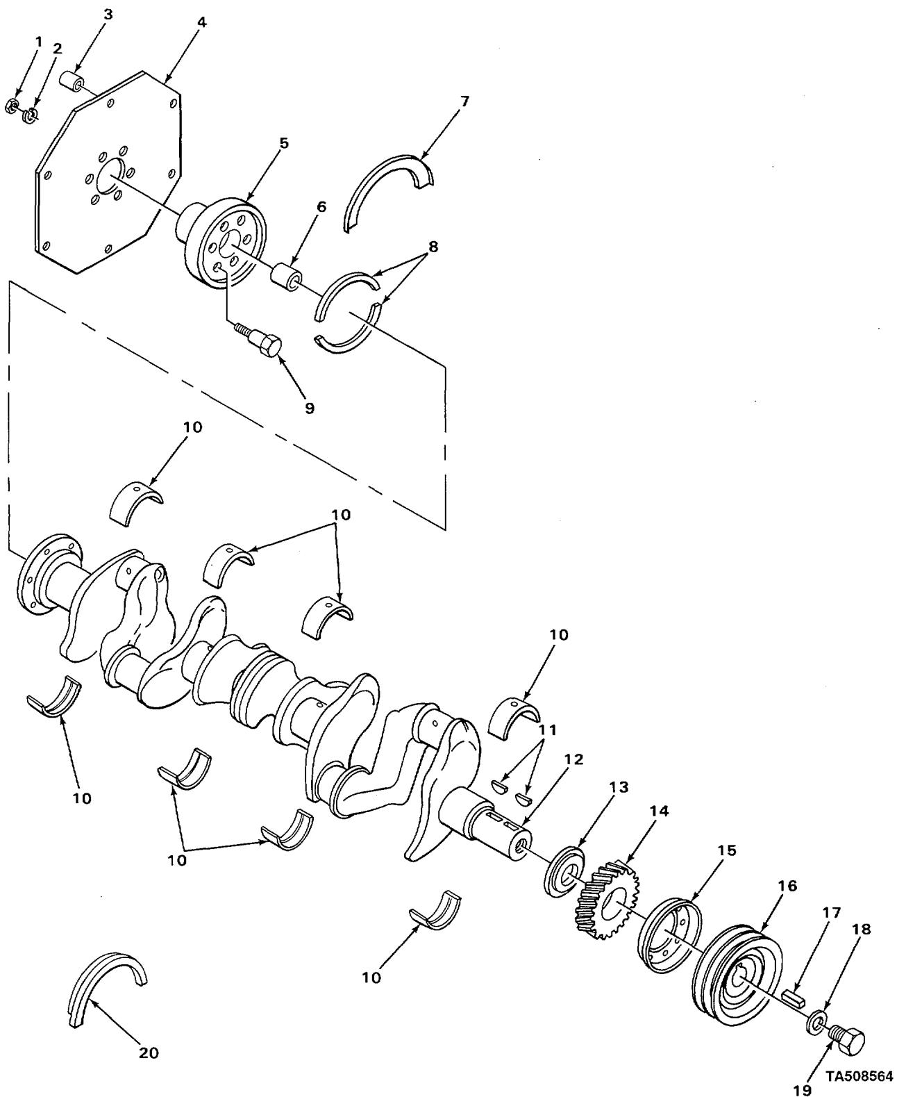
FIGURE 3. CRANKSHAFT.
