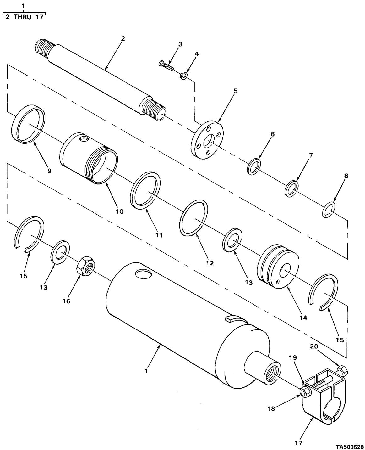
FIGURE 67. POWER STEERING CYLINDER (MHE178B, MHE178C, AND MHE223).
