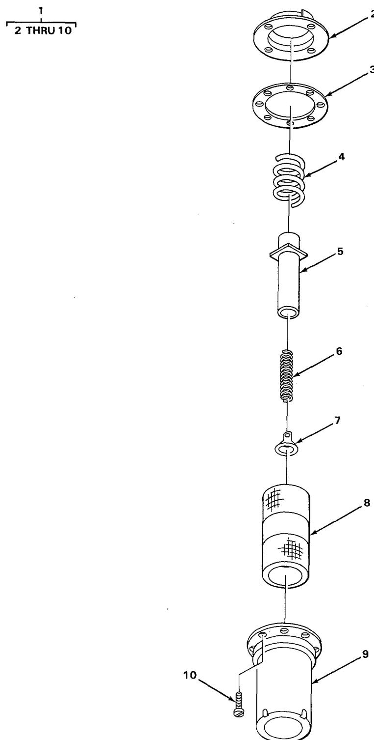
FIGURE 80. HYDRAULIC OIL FILTER.
