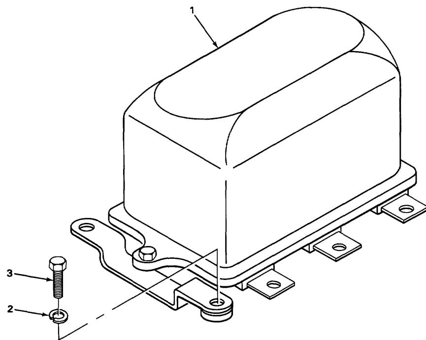
*FIGURE 23. GENERATOR REGULATOR VOLTAGE.*
