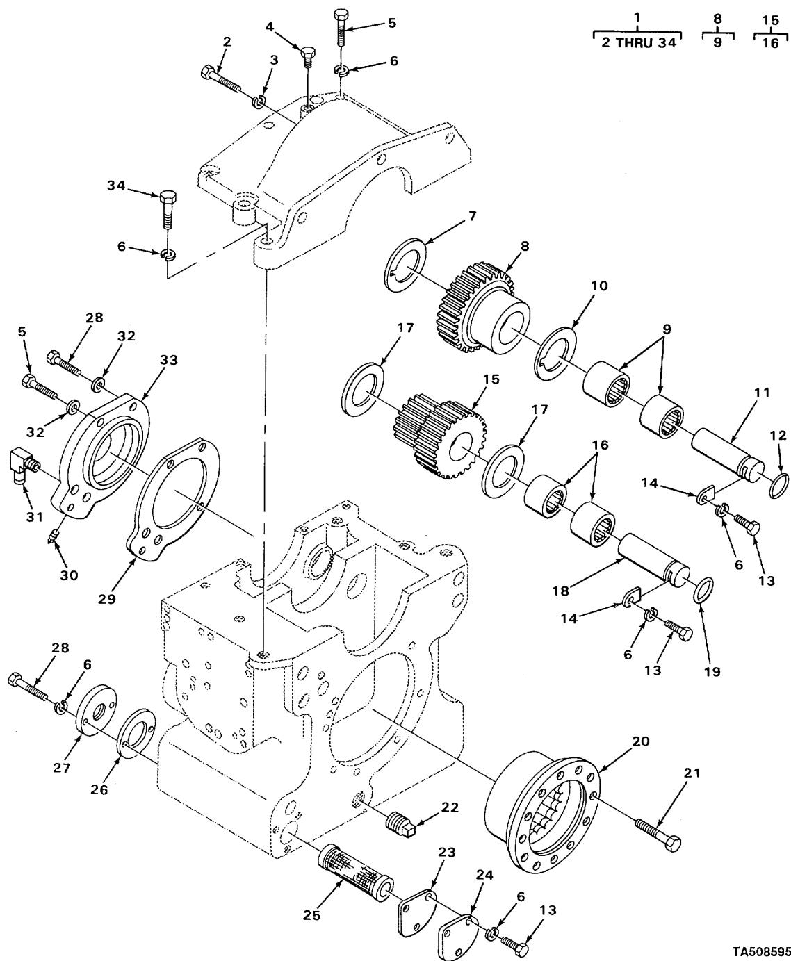
FIGURE 34. TRANSMISSION ASSEMBLY.
