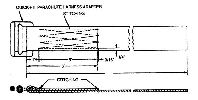
Figure 2-12. A-7A Cargo Sling Stitching Details
