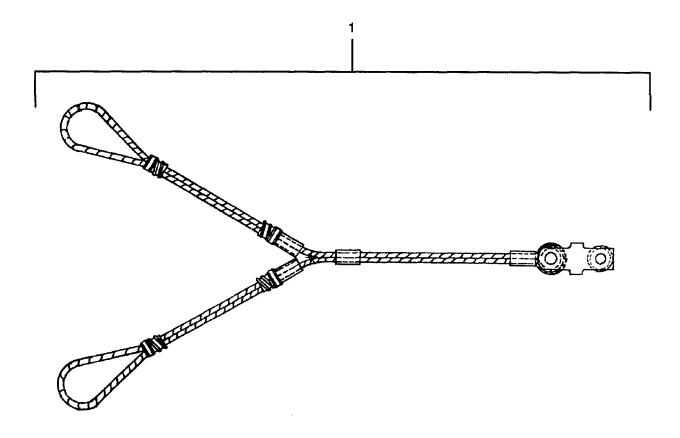
Figure C-30. Cable Harness Assembly
