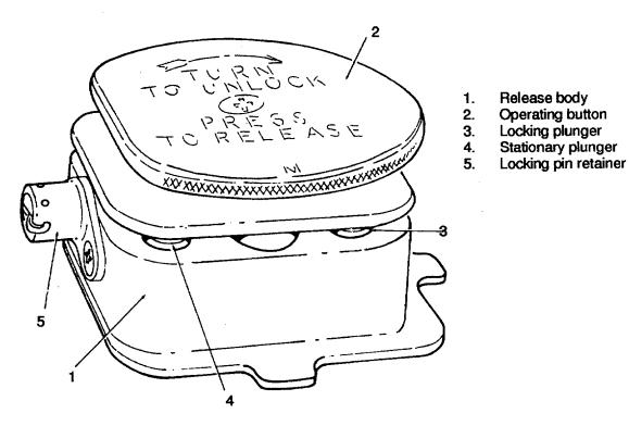
Figure 1.4. Quick Release Assembly
