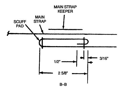
Figure 2-18. Main Strap Keeper Sewing Details
