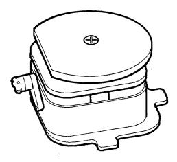
Figure 2-14. Quick Release Assembly
