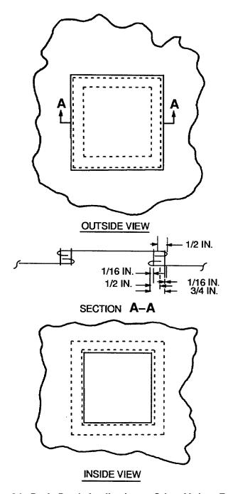
Figure 24. Basic Patch Application to Other Airdrop Equipment
