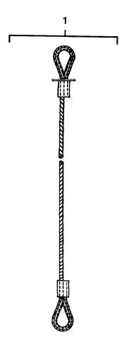
Figure C-28. Cable Assembly, Initiator
