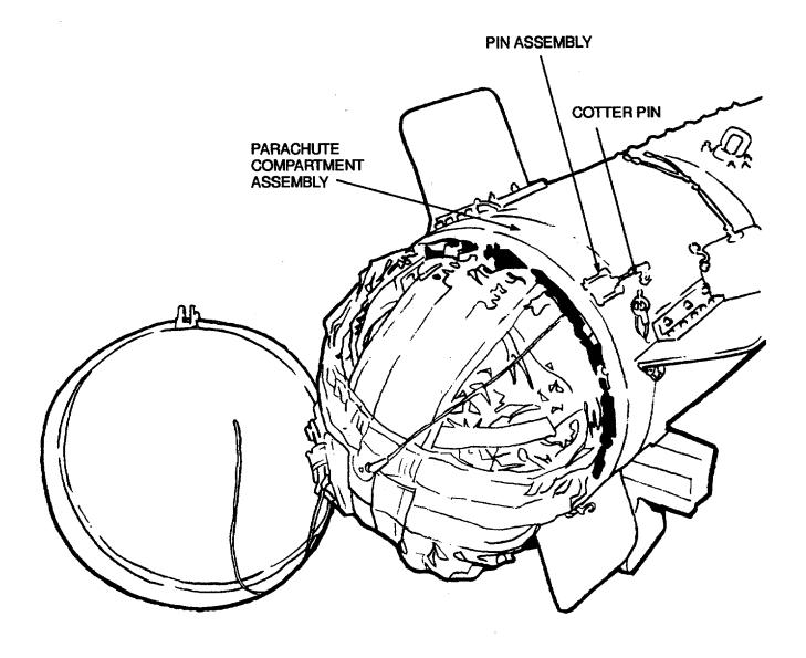
Figure 2-36. Parachute Compartment Assembly
