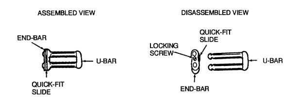
C. The Quick-fit Parachute Connector Link Assembly.
