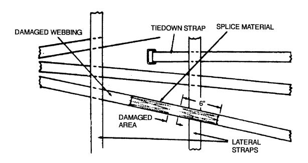
Figure 2-23. Splicing Details for a Damaged Support Web
