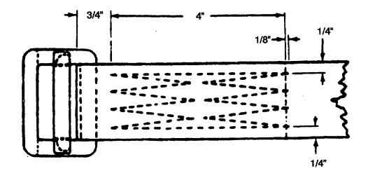
Figure 2-26. Quick-fit Adapter Installation Details
