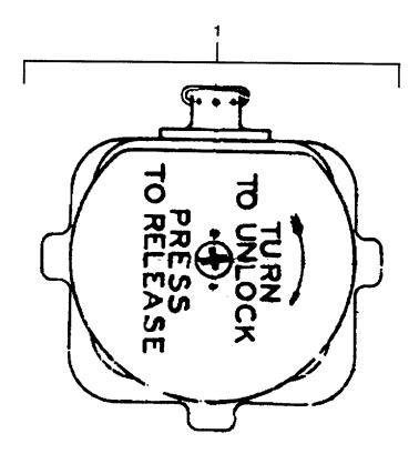
Figure C-7. Quick Release Assembly
