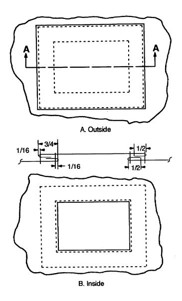
Figure 2-13. Patching Details for Cover
