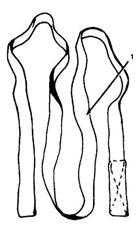
Figure C-32. Connector Strap, 120-inch
