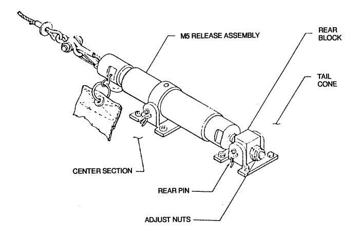
Figure 2-32. M5 Cartridge-Actuated Release Assembly
