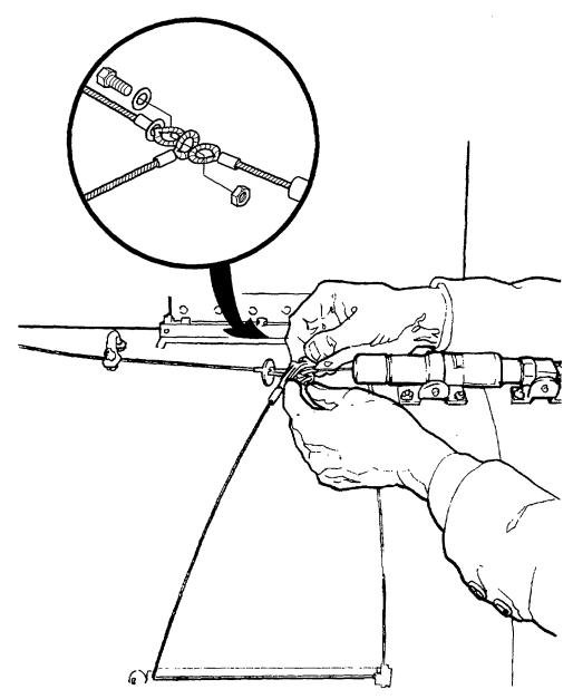
Figure 2-29. Parachute Cable Release Assembly
