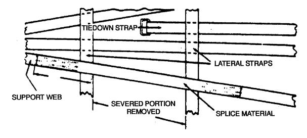
Figure 2-24. Splicing Details for a Severed Support Web
