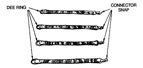
Figure 2-28. Type A-22 Cargo Bag Suspension Webs
