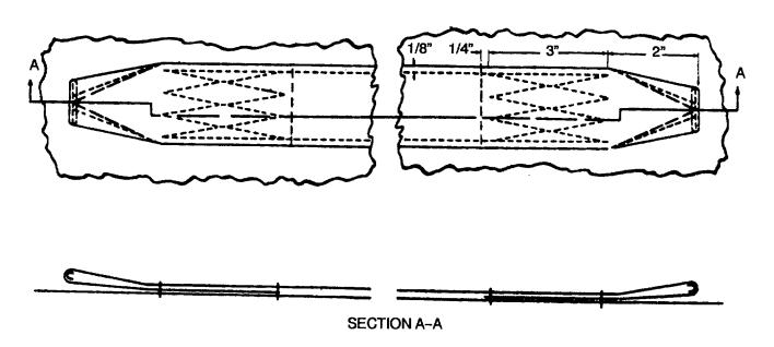
Figure 2-22. Installing Cover Lacing Loop Strap
