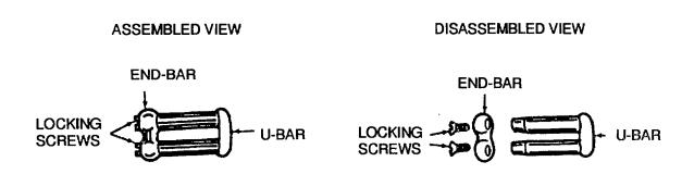
B. The U-bar Parachute Connector Link Assembly.
