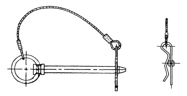
Figure 2-39. Connector Pin Assembly
