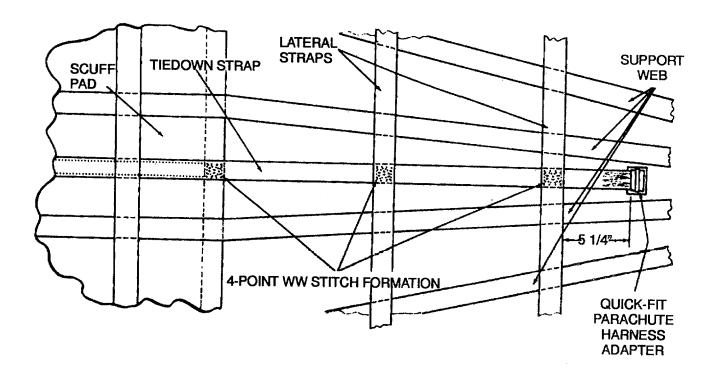
Figure 2-27. Tie-down Strap Installation Details
