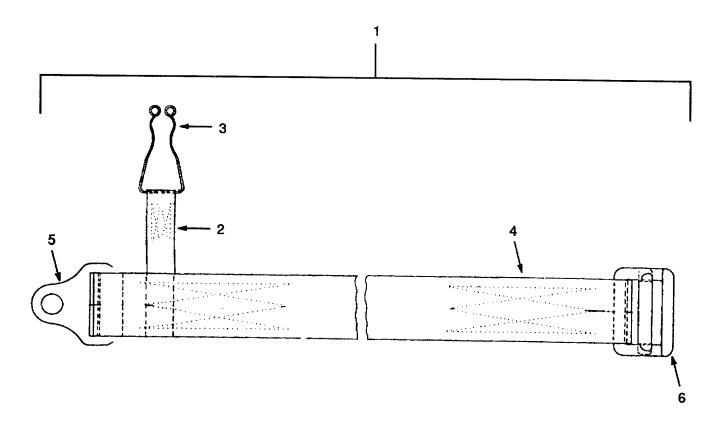
Figure C-4. Strap, Quick Release, Fixed
