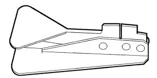
Figure 2-6. The Parachute Connector Link Separator
