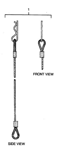
Figure C-22. Cable Assembly, Parachute Release
