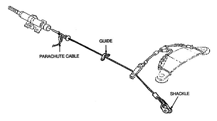
Figure 2-31. Initiator Cable Assembly
