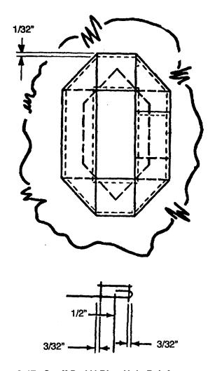
Figure 2-17. Scuff Pad V-Ring Hole Reinforcement Details
