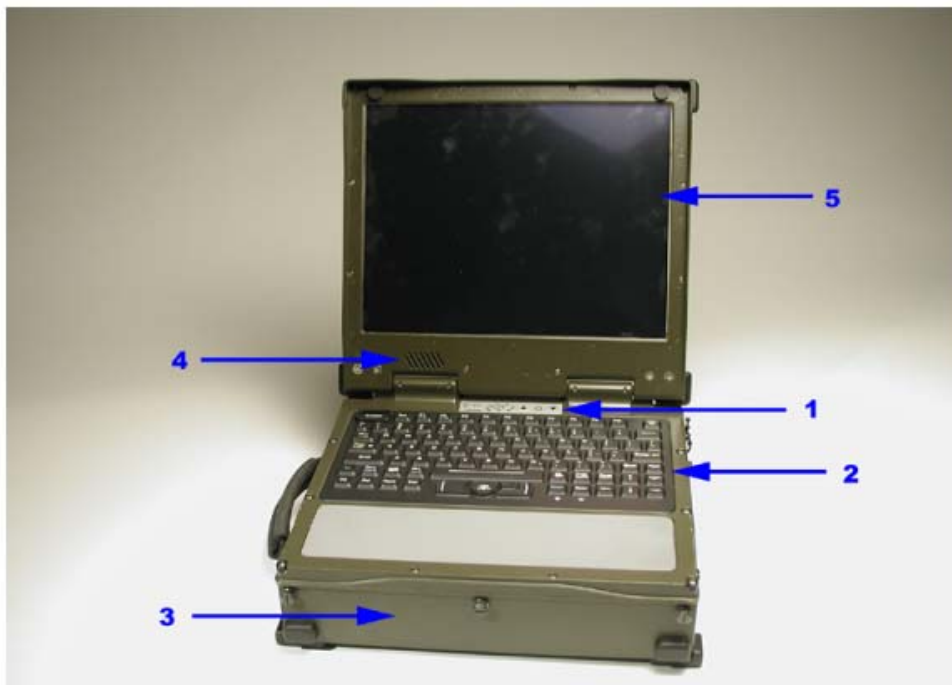
Figure 1. PCU Front View Controls and Indicators
