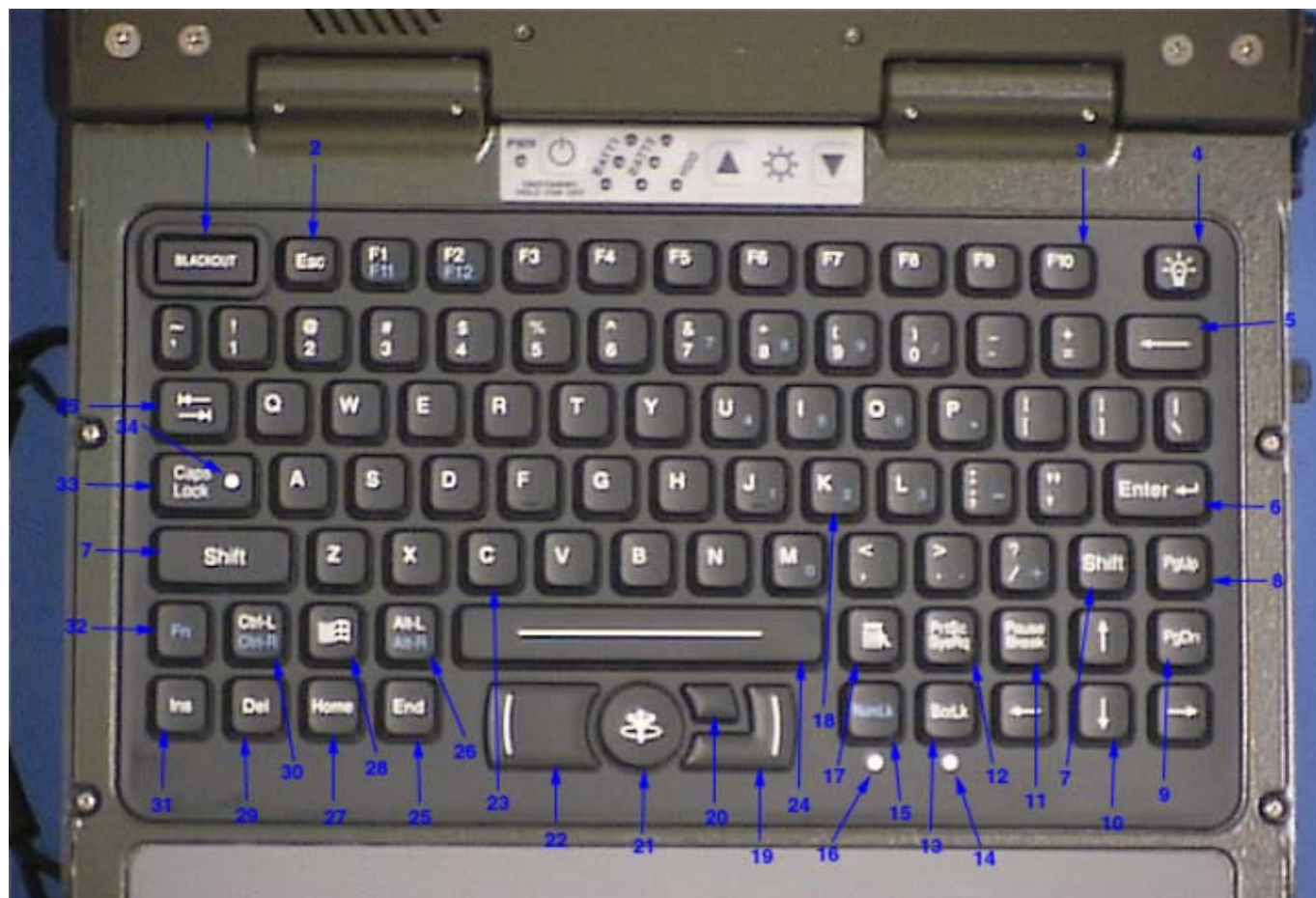
Figure 7. PCU Keyboard Controls and Indicators
