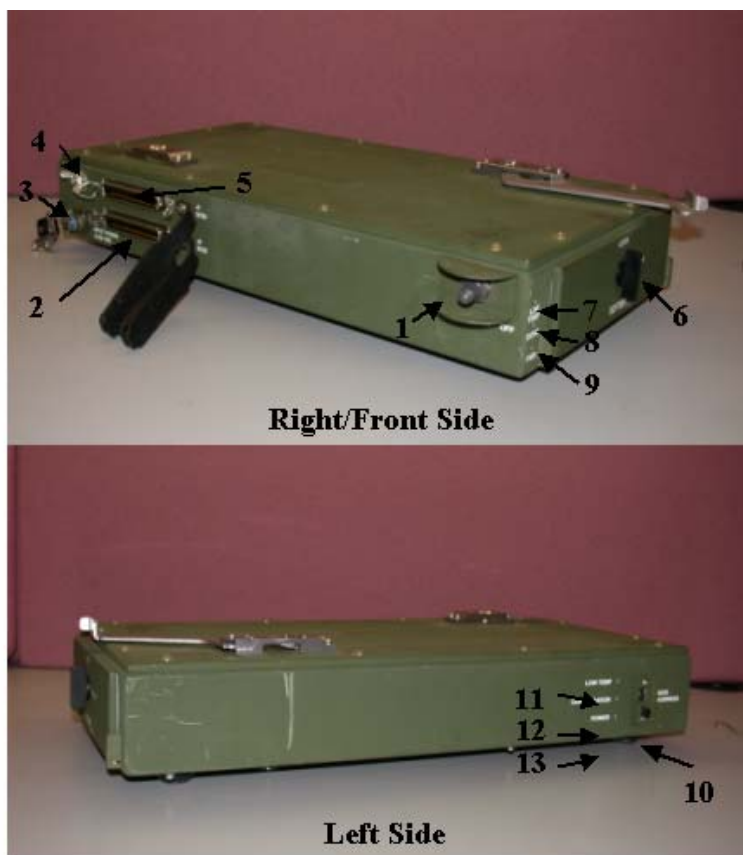
Figure 10. MU-1114/s Smith Industries Data Transfer Module Receptacle (SDTMR) Controls, Indicators, and Connectors
