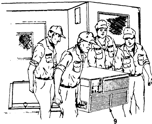
8. Lift ECU (9) onto fold-down shelf (2) with control panel (13) facing toward inside of shop.
