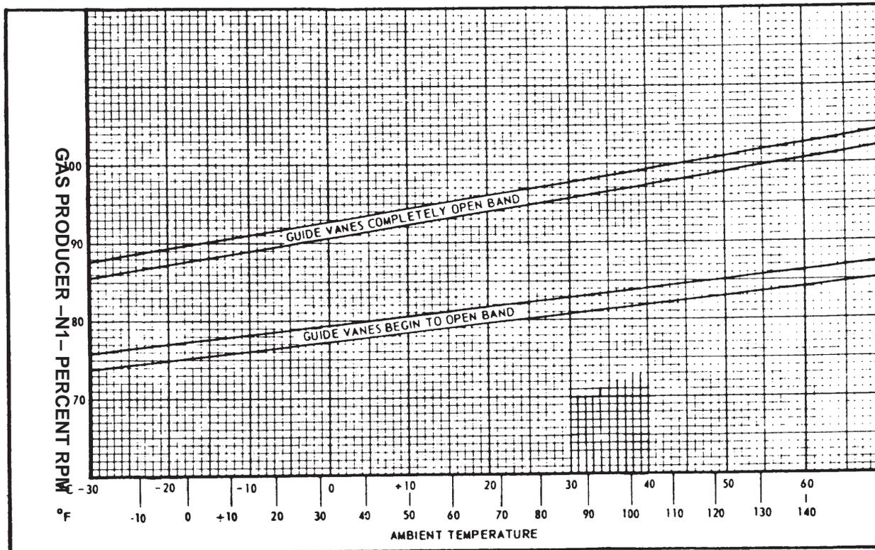
Figure 5-2. T53-L-703 Variable Inlet Guide Vane Chart
