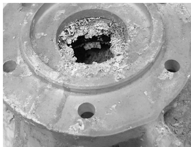
Figure 3-24. Magnesium Corrosion Products
