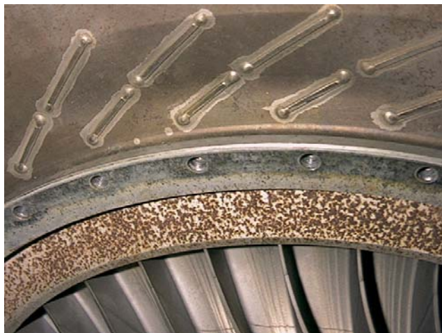
Figure 3-22. Hot Corrosion on Engine Components
