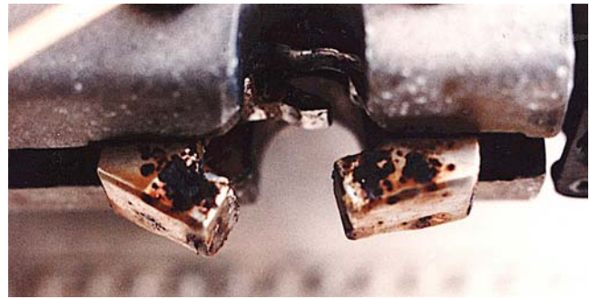
Figure 3-28. Failed Chromium Plate
