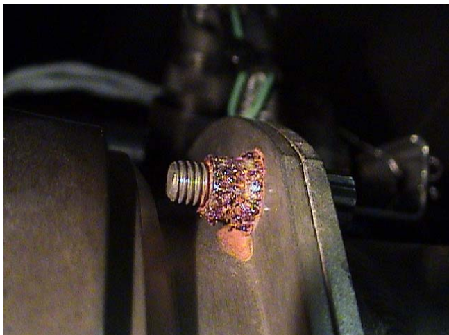
Figure 3-21. Hot Corrosion on Fasteners
