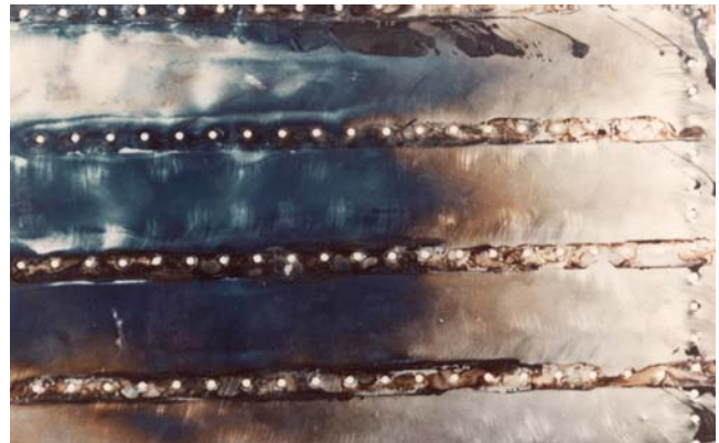
Figure 3-26. Color Changes in Titanium Due to Heating
