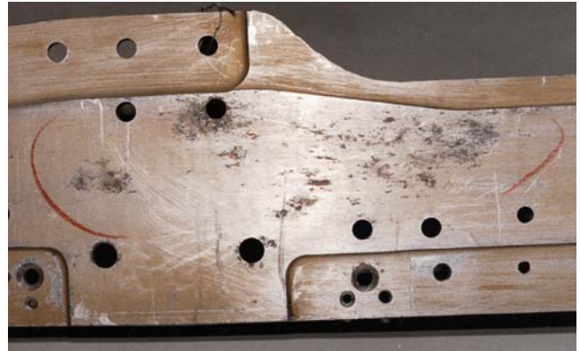
Figure 3-10. Pitting of an Aluminum Wing Assembly
