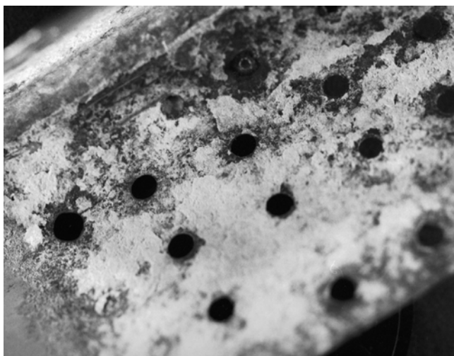
Figure 3-23. Aluminum Surface Corrosion Products
