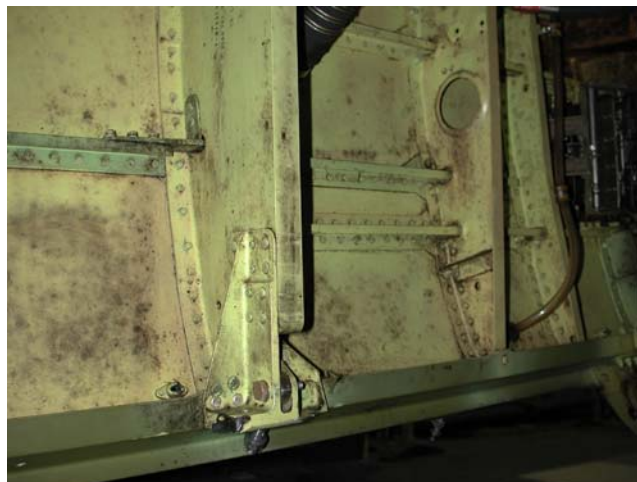
Figure 3-30. Biological Growth on Helicopter Wall
