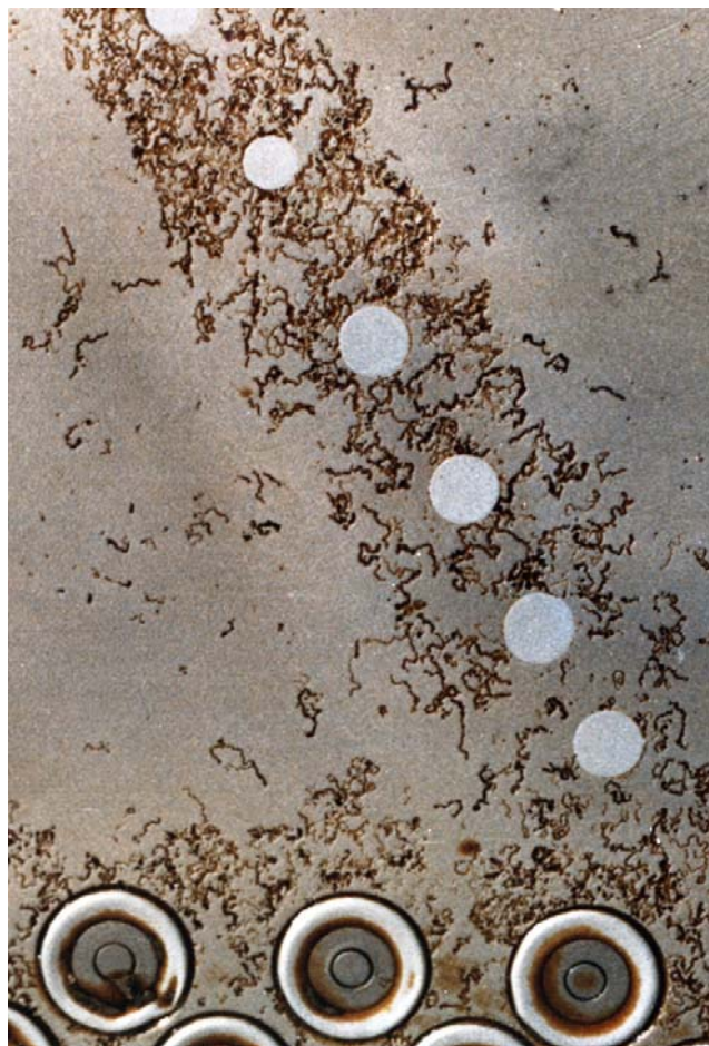
Figure 3-17. Filiform Corrosion Found Under Paint Coating on a Magnesium Panel
