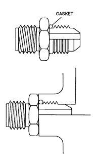
Figure 4-19. MS Fitting Gasket Installation
