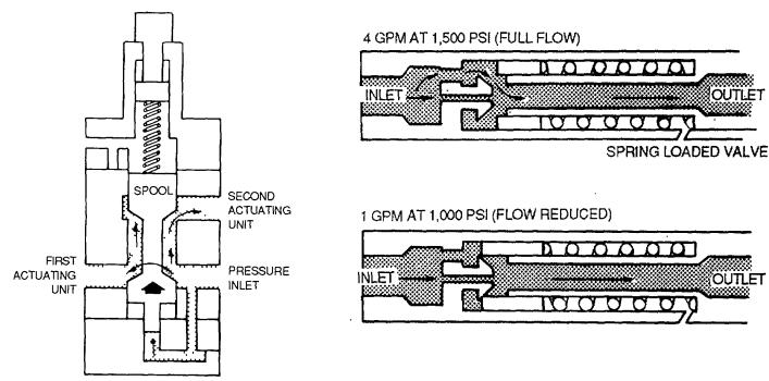
Figure 4-130. Pressure-Actuated Sequence Valve
