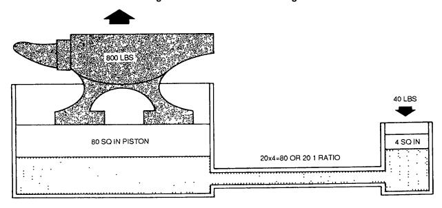
Figure 2-5. Application of Mechanical Advantage
