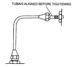
Figure 4-14. Tube and Fitting Alignment
