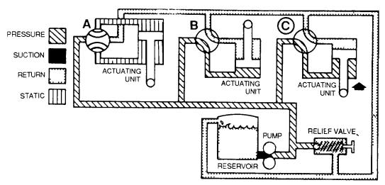
Figure 4-147. Selector Valve C Open
