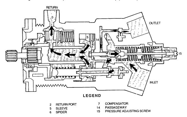
Figure 4-106. Stratopower Effective Stroke Pump (Zero Flow ) 4-113
