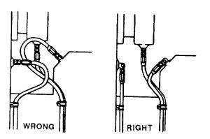
6 USE ELBOWS AND ADAPTERS TO INSURE CLEANER INSTALLATIONS FOR EASY INSPECTION AND MAINTENANCE
