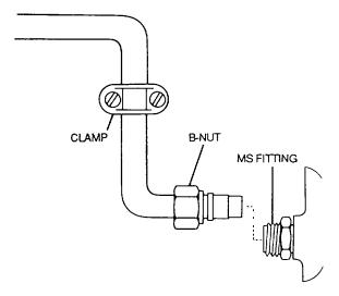
Figure 4-20. Tubing Alignment
