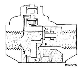
Figure 4-99. Differential Pressure Indicator (Normal Flow)
