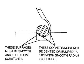
Figure 4-60. Removing O-Ring
