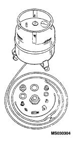
Figure 3-1. Typical Hydraulic System Filler and Bleeder
