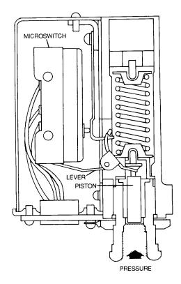
Figure 4-114. Pressure Gauge
