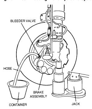
Figure 4-161. Gravity Method for Brake Bleeding
