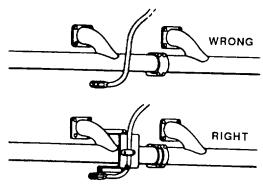
2 WHEN HOSE LINES PASS CLOSE TO A HOT EX-HAUST MANIFOLD, PROTECT THE HOSE WITH FIRE-PROOF BOOT OR METAL BAFFLE
