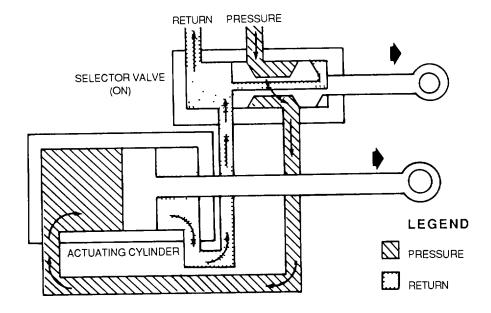
Figure 4-134. Double-Action Actuating Cylinder (Extension)
