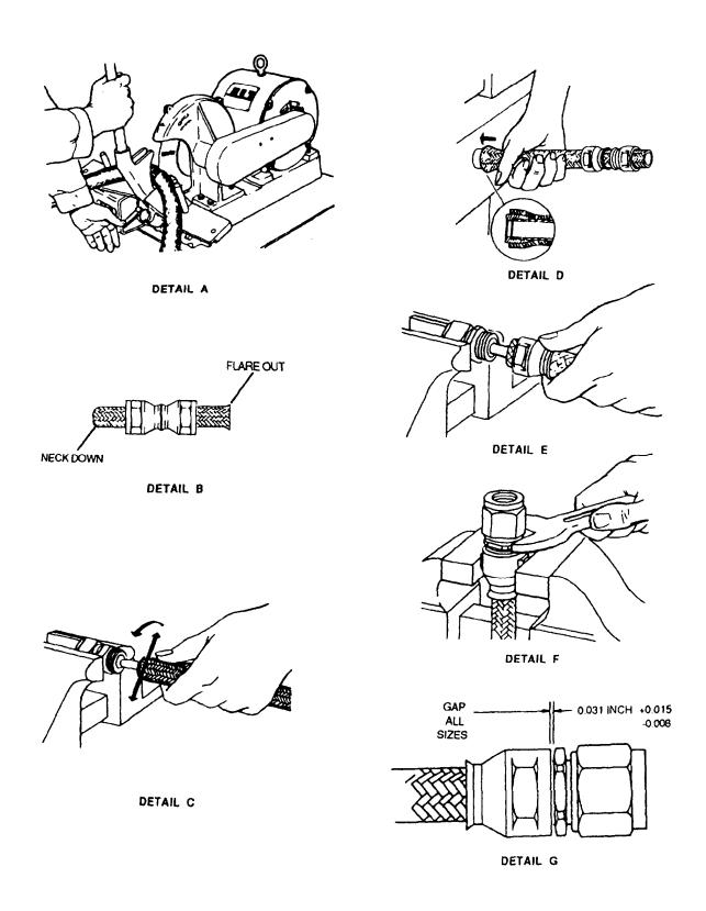
Figure 4-50. Field Assembly of High-Pressure Teflon Hose, MIL-H-38360.
