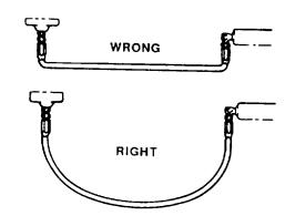
5 KEEP THE BEND RADII OF THE HOSE AS LARGE AS NECESSARY TO AVOID KINKING OF LINE AND RESTRICTION OF FLOW
