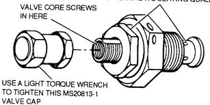
VALVE CORE INSTALLED
