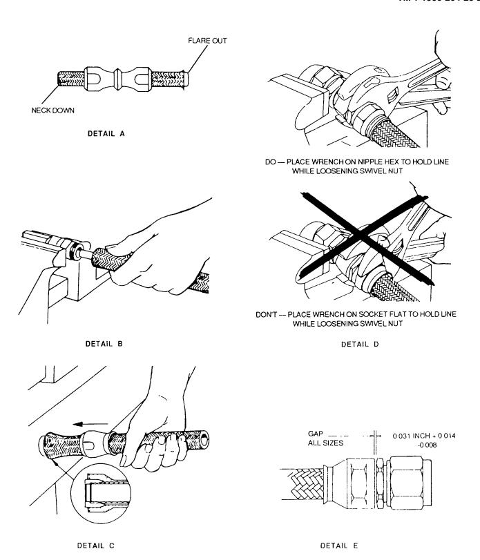
Figure 4-48. Medium-Pressure Teflon Hose Assembly Procedure (Sheet 1 of 3)
