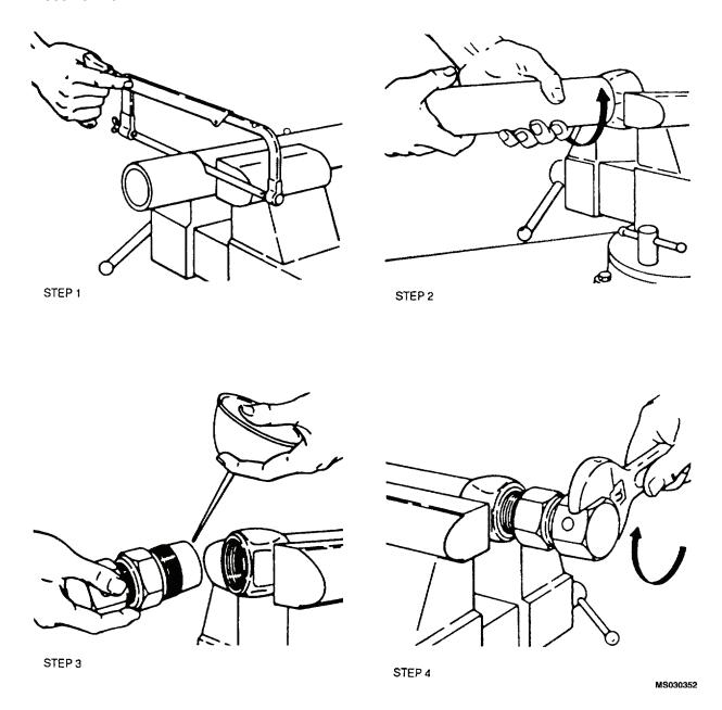
Figure 4-43. Assembly of Medium and Low-Pressure Hose Assemblies
