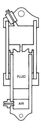
Figure 4-173. Floating Piston Shock Strut
