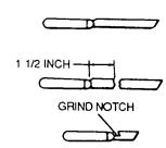
Figure 4-39. Knife for Cutting Flexible Hose
