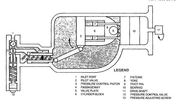
Figure 4-107. Vickers Stroke Reduction Pump (Zero Flow)
