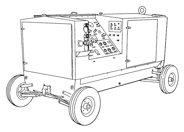
Figure 3-2. Typical Gasoline Engine-Driven Hydraulic Test Stand
