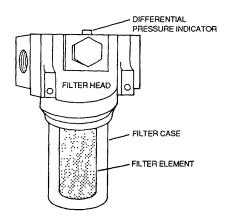
Figure 4-96. Fluid Filter Assembly
