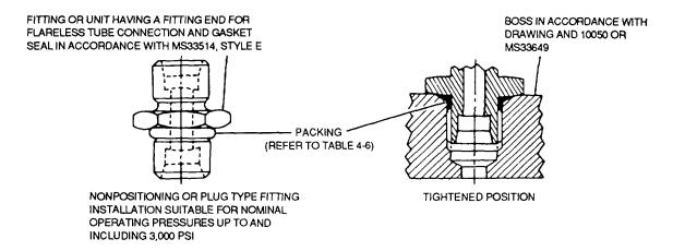
Figure 4-25. Installation of MS33514 Fitting End
