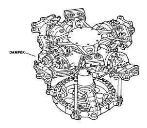
Figure 4-165. Main Rotor Assembly with Piston Dampers
