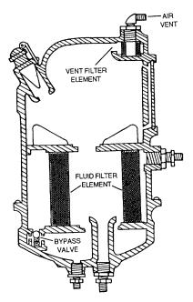
Figure 4-94. Reservoir with Filter Elements
