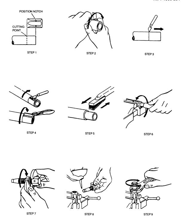
Figure 4-41. Field Fabrication of High-Pressure Hose Assemblies
