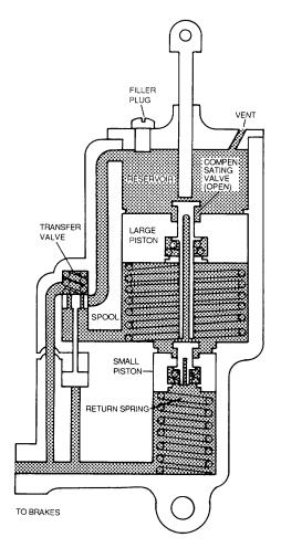
Figure 4-149. Compound Master Cylinder
