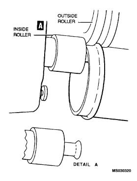
Figure 4-12. Beading Large Tubing
