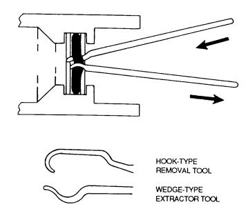
Figure 4-62. Internal O-Ring Removal (Wedge-Type Extractor)
