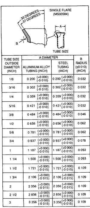
Figure 4-7. Dimensions for Single-Flared Tubing
