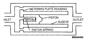
Figure 4-140. Hydraulic Fuse Assembly
