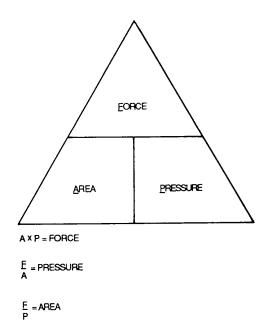
Figure 2-1. Computing Force Pressure, and Area
