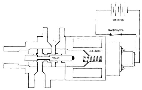
Figure 4-125. Solenoid-Actuated Control Valve (Energized)
