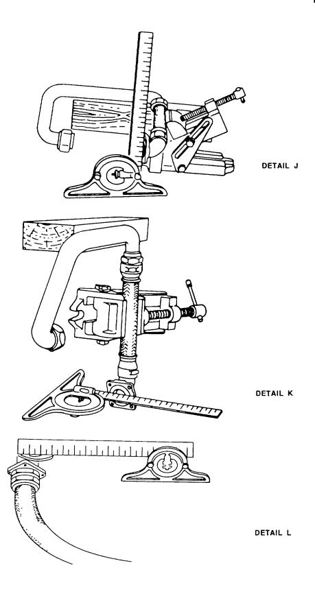
Figure 4-48. Medium-Pressure Teflon Hose Assembly Procedure (Sheet 3 of 3)
