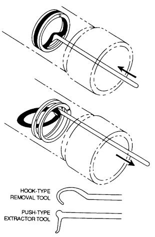
Figure 4-63. Internal O-Ring Removal (Push-Type Extractor)
