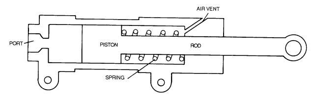
Figure 4-133. Single-Action Actuating Cylinder
