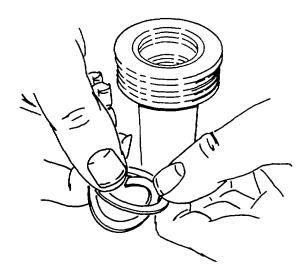
Figure 4-72. Stretching Teflon Backup Ring
