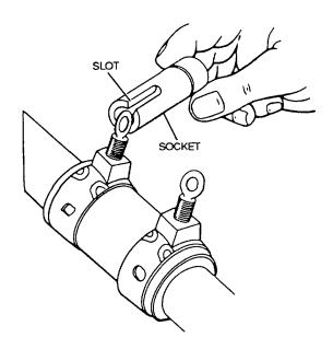
Figure 4-32. Tightening Hose Clamp with Socket
