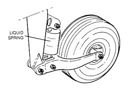
Figure 4-176. Tailwheel Liquid Spring
