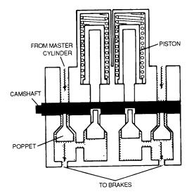
Figure 4-156. Dual Parking Brake Valve
