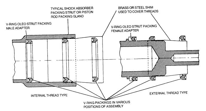
Figure 4-71. V-Ring Packings in Various Positions of Assembly 4-85
