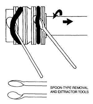
Figure 4-65. External O-Ring Removal (Spoon-Type Tools)
