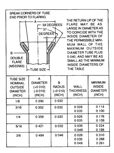
Figure 4-8. Dimensions for Double-Flared Tubing
