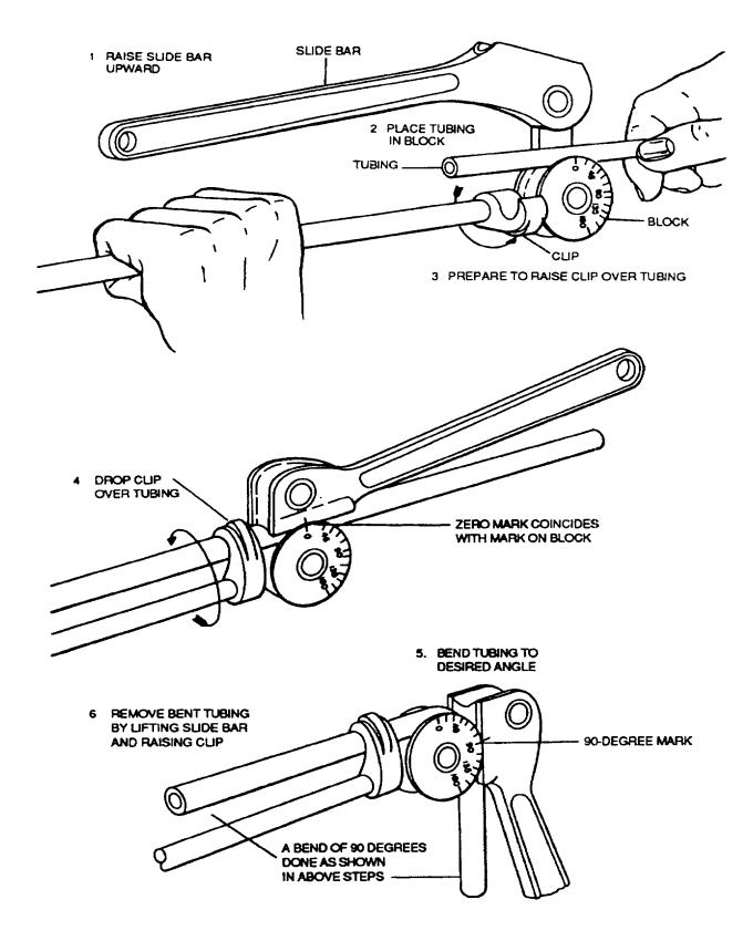
Figure 4-4. Bending Tube with Bending Machine
