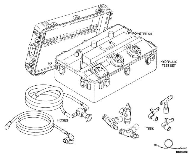
Figure 3-5. Typical Master Gauge Unit
