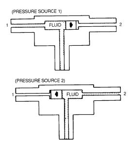
Figure 4-132. Floating-Piston Shuttle Valve
