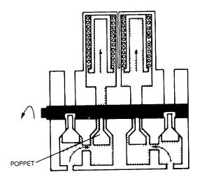
Figure 4-158. Dual Parking Brake Valve (On)
