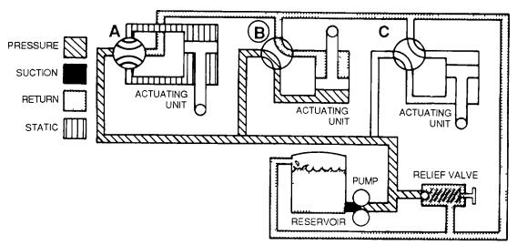
Figure 4-146. Selector Valve B Open
