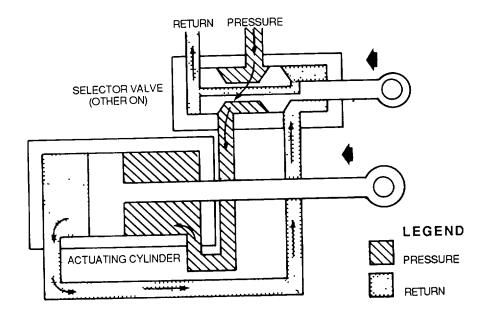
Figure 4-135. Double-Action Actuating Cylinder (Retraction)
