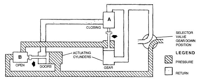
Figure 4-129. Landing Gear System Using Mechanically Actuated Sequence Valves
