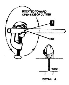
Figure 4-3. Cutting Tube with Tube Cutter.
