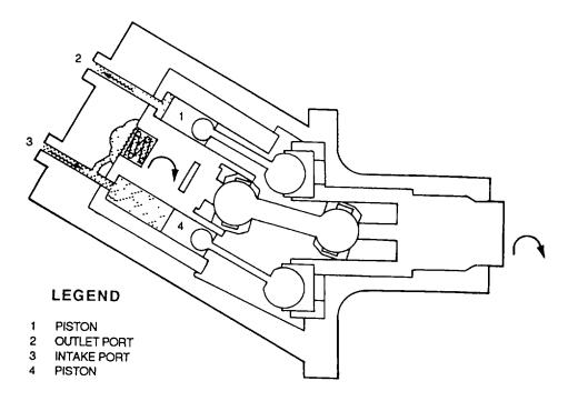
Figure 4-103. Constant Volume Pump (Piston Operation)
