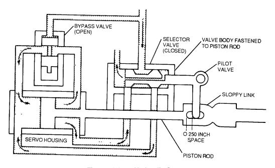
Figure 4-138. Hydraulic Servo
