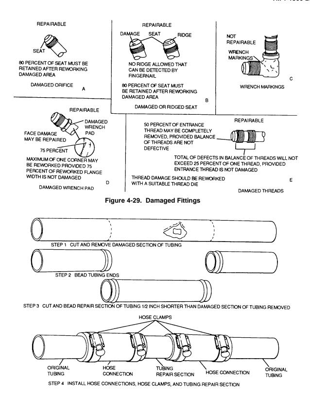
Figure 4-30. Repair of Low-Pressure Tubing
