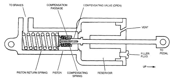
Figure 4-148. Simple Master Cylinder
