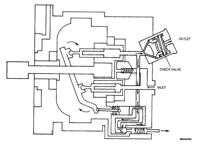
Figure 4-110. Kellogg Stroke Reduction Pump (Reduced Output)
