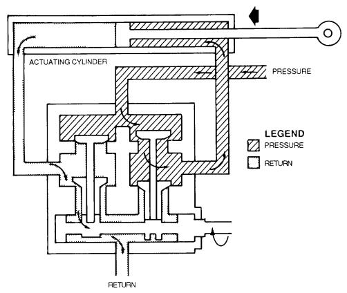
Figure 4-122. In-Line Cam-Operated Selector Valve (Actuator Retracting)
