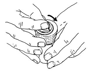
Figure 4-73. Installing Teflon Backup Ring
