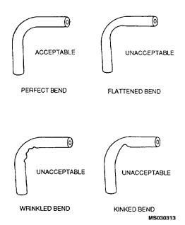
Figure 4-5. Acceptable and Unacceptable Tubing Bends
