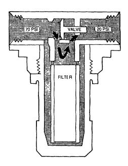
Figure 4-98. Fluid Filter (Clogged)
