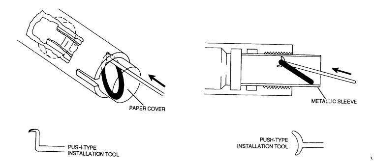
Figure 4-67. Internal O-Ring Installation(Paper Cover)
