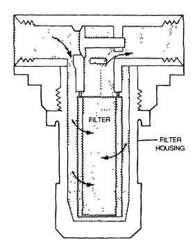
Figure 4-97. Fluid Filter (Normal Fluid)
