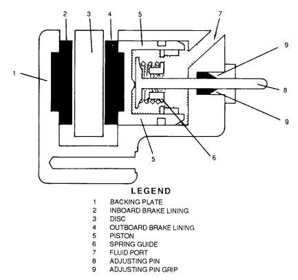
Figure 4-155. Disc Brake Assembly Cross Section
