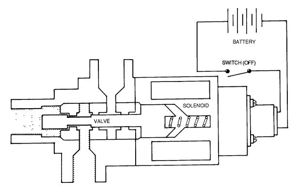
Figure 4-126. Solenoid-Actuated Control Valve (De-energized)
