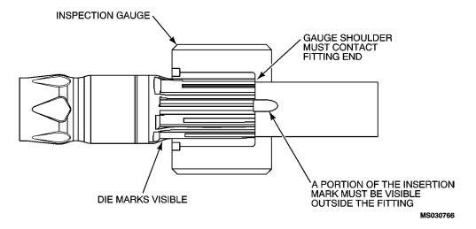
Figure 4-81. Using Inspection Gauge
