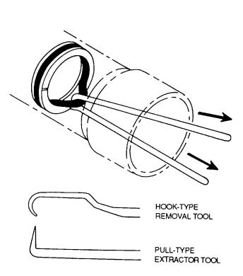
Figure 4-61. Internal O-Ring Removal (Pull-Type Extractor)
