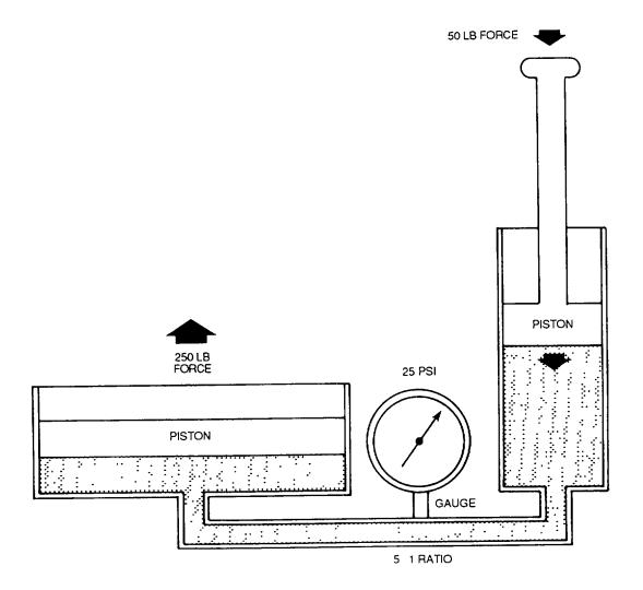
Figure 2-4. Mechanical Advantage
