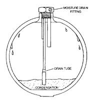
Figure 4-95. Spherical Air Cylinder
