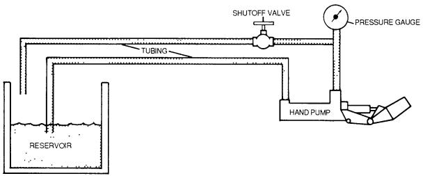
Figure 4-112. Hand Pump Test Circuit
