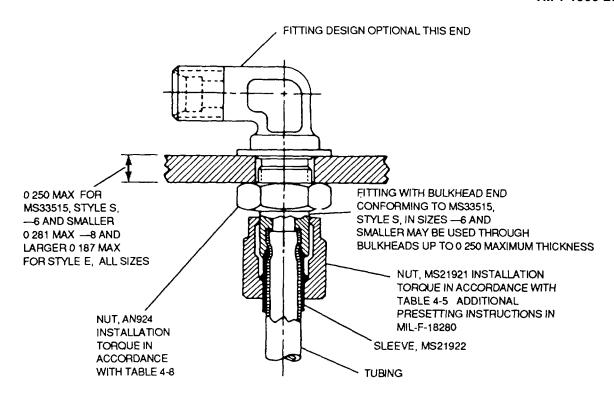
Figure 4-24. Bulkhead Flareless Fitting Installation
