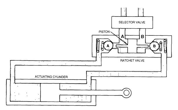
Figure 4-136. Ratchet Valve (Static)
