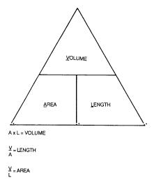
Figure 2-2. Computing Volume, Length, and Area
