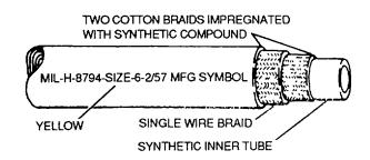
Figure 4-34. Flame and Aromatic-Resistant Hose, MIL-H-8794
