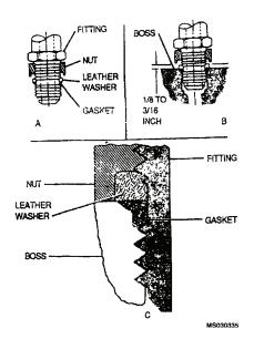
Figure 4-27. Combination Bulkhead and Universal Fitting Assembly
