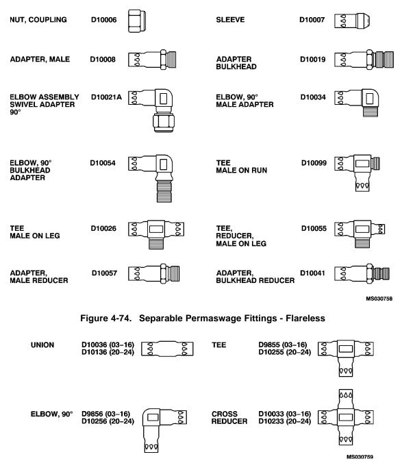
Figure 4-75. Permanent to Permanent Permaswage Fittings
