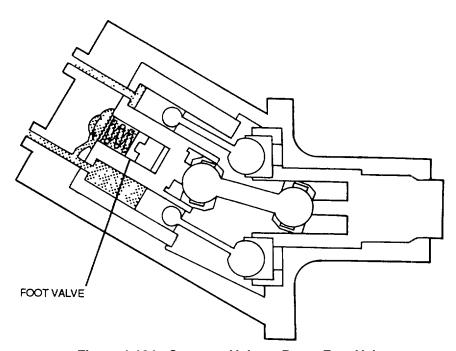
Figure 4-104. Constant Volume Pump Foot Valve
