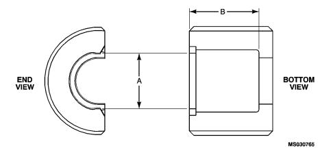
Figure 4-80. Inspection Gauge
