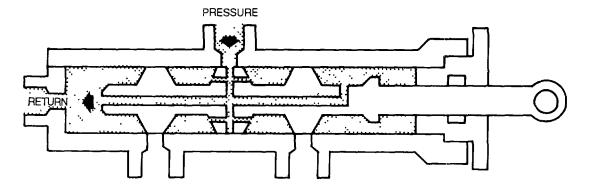
Figure 4-121. Spool-Type, Open Center Selector Valve (Closed)
