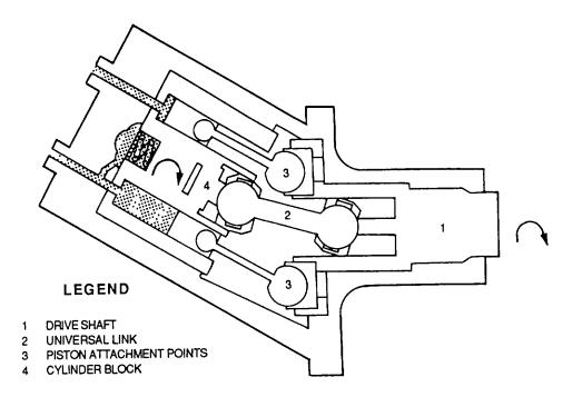
Figure 4-102. Constant Volume Pump (Piston Installation)
