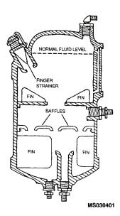
Figure 4-91. Reservoir with Baffles, Fins and Finger Strainer
