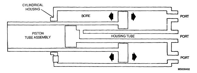
Figure 4-92. Fluid-Pressurized Reservoir (Unpressurized)
