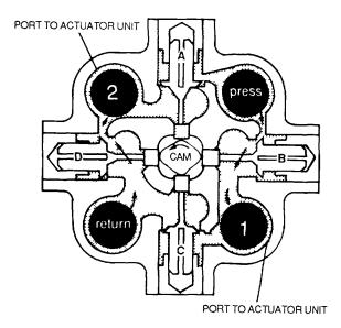
Figure 4-124. Radial Cam-Operated Selector Valve
