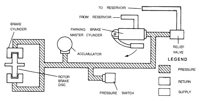
Figure 4-159. Rotor Blade Brake System
