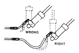
3 WHEN A HOSE ASSEMBLY IS TO BE SUBJECTED TO CONSIDERABLE FLEXING OR VIBRATION, REMEMBER THAT THE METAL HOSE FITTINGS ARE NOT PART OF THE FLEXIBLE PORTION
