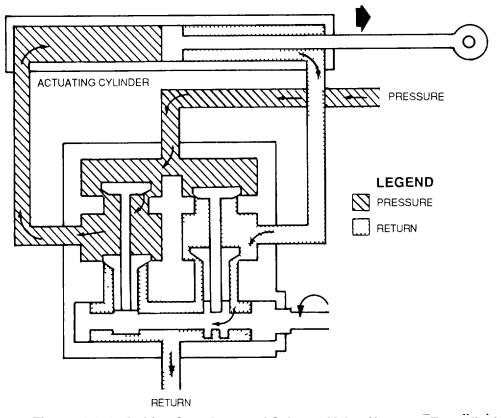
Figure 4-123. In-Line Cam-Operated Selector Valve (Actuator Extending)
