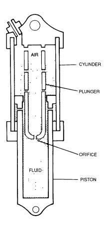
Figure 4-172. Complex Shock Strut (Plunger)
