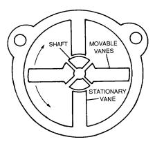
Figure 4-167. Vane Damper Cross Section
