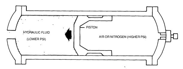
Figure 4-118. Cylindrical Accumulator
