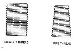
Figure 4-26. Straight Thread and Pipe Thread
