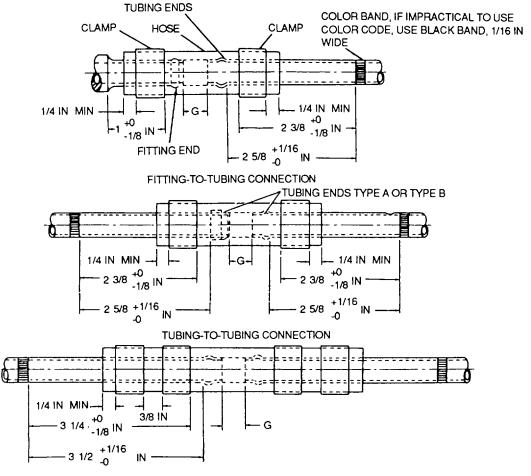
USE OF DOUBLE HOSE CLAMPS PERMITTED ONLY WITH THE SPECIFIC APPROVAL OF AVSCOM (UNLESS SPECIFIED ON ORIGINAL INSTALLATION DRAWING)
