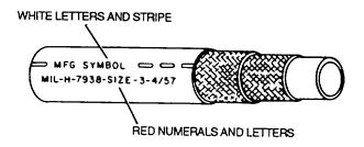
Figure 4-36. Flame Aromatic, and Oil-Resistant Hose MIL-H-7938
