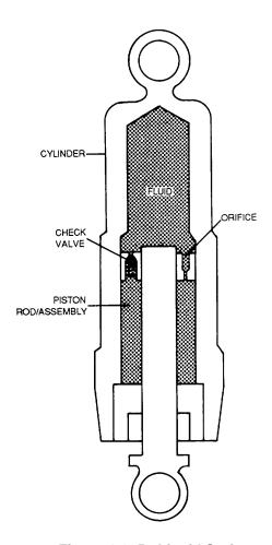
Figure 4-175. Liquid Spring
