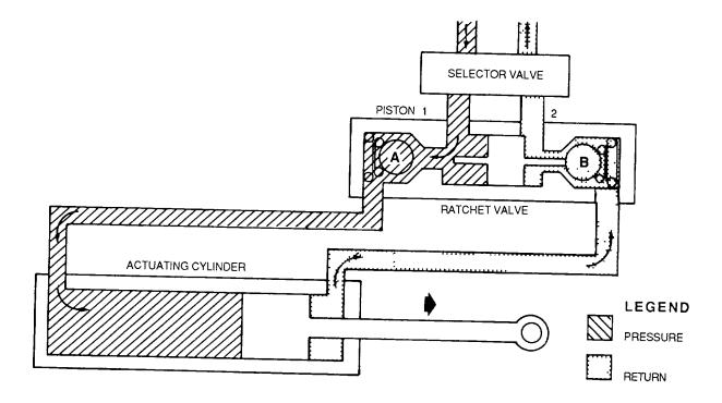
Figure 4-137. Ratchet Valve (Moving)
