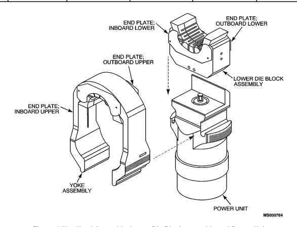
Figure 4-79. Head Assembly, Lower Die Block assembly and Power Unit
