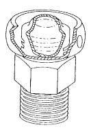
Figure 4-53. Steel Protective Dust Cap
