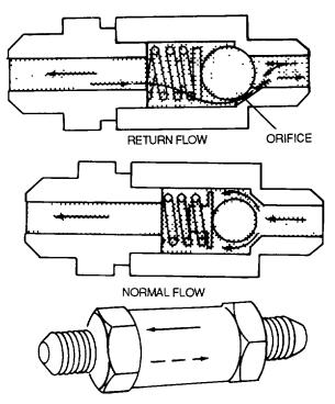
Figure 4-128. Orifice Check Valve
