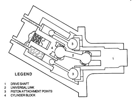
Figure 4-101. Bent-Axis Constant Volume Pump
