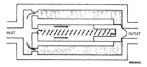
Figure 4-142. Hydraulic Fuse (Blocked Flow)
