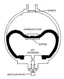
Figure 4-119. Spherical Accumulator
