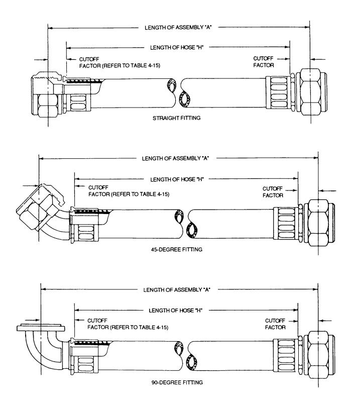
Figure 4-40. Determining Hose Assembly Length
