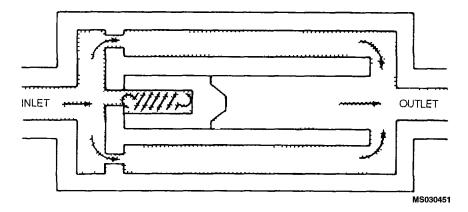
Figure 4-141. Hydraulic Fuse (Full Flow)
