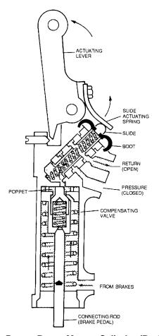
Figure 4-151. Power-Boost Master Cylinder (Brake Released)
