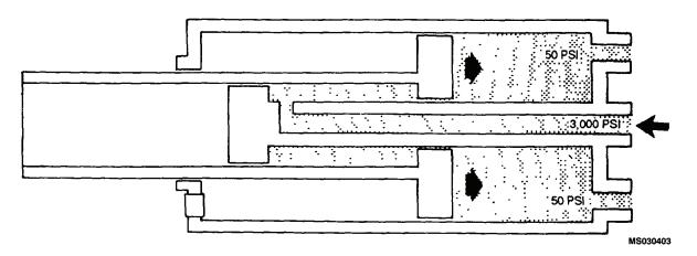
Figure 4-93. Fluid-Pressurized Reservoir (Pressurized)
