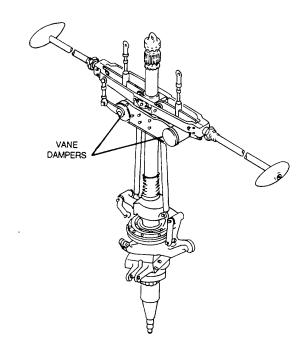
Figure 4-169. Stabilizer Bar with Vane Dampers
