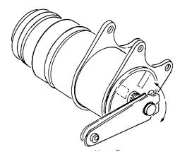
Figure 4-166. Vane Damper
