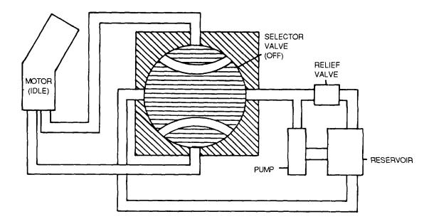
Figure 4-120. Rotary-Type, Closed Center Selector Valve
