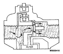
Figure 4-100. Differential Pressure Indicator (Clogged Filters)
