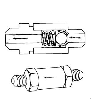
Figure 4-127. Simple Check Valve
