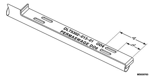
Figure 4-79. Insertion Marking Tool
