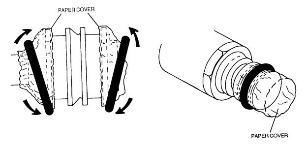
Figure 4-69. External O-Ring Installation
