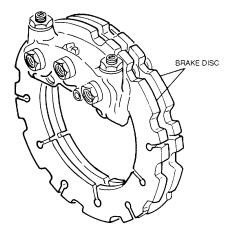
Figure 4-154. Disc Brake Assembly
