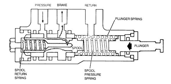
Figure 4-152. Power Brake Control Valve (Brakes Applied)
