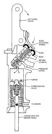
Figure 4-150. Power-Boost Master Cylinder (Brake Applied)
