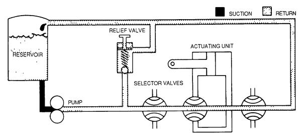
Figure 4-143. Open-Center Hydraulic System (Valve Closed)
