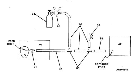
Figure 4. Resistance gage performance check, equipment setup.
