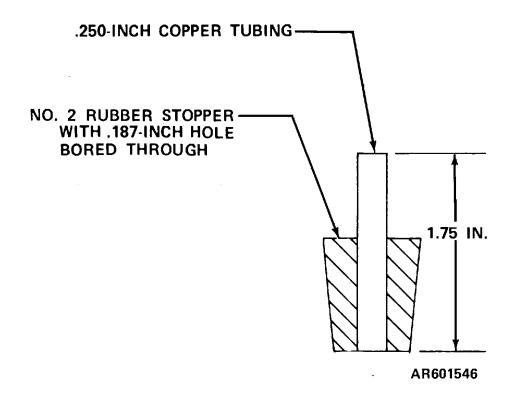
Figure 1. Fabrication instructions for connector (B1).
