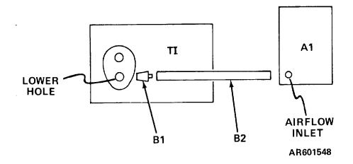
Figure 3. AIR FLOW gage performance check, equipment setup.
