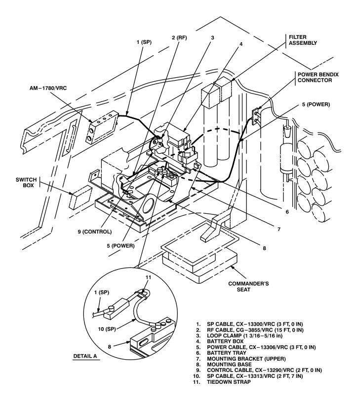
Figure 5-7 (2). Cable Installation: Power, SP and RF Cabling
