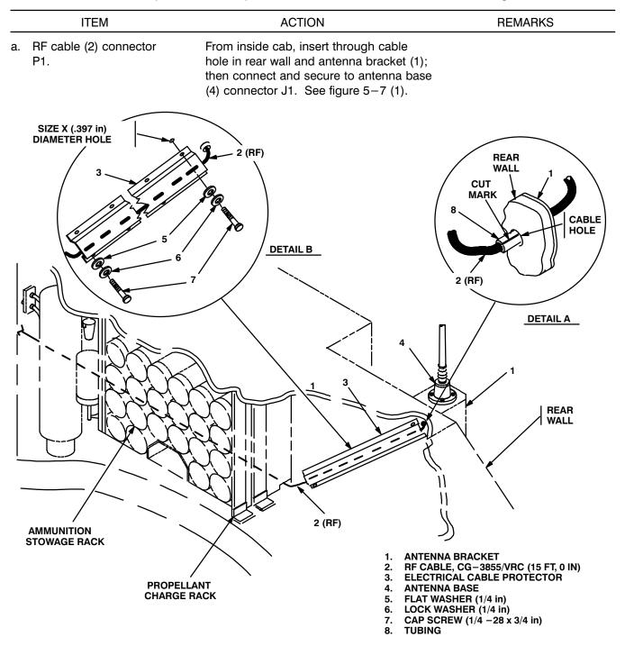
Figure 5-7 (1). Cable Installation: RF Cabling
