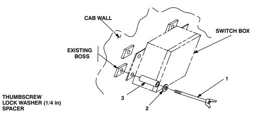
Figure 5-2 (2). Modifying Vehicle: Installing Mounting Hardware
