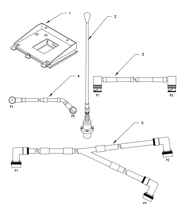
Figure 4-1. MK-2865/VRC Illustrated Parts List
