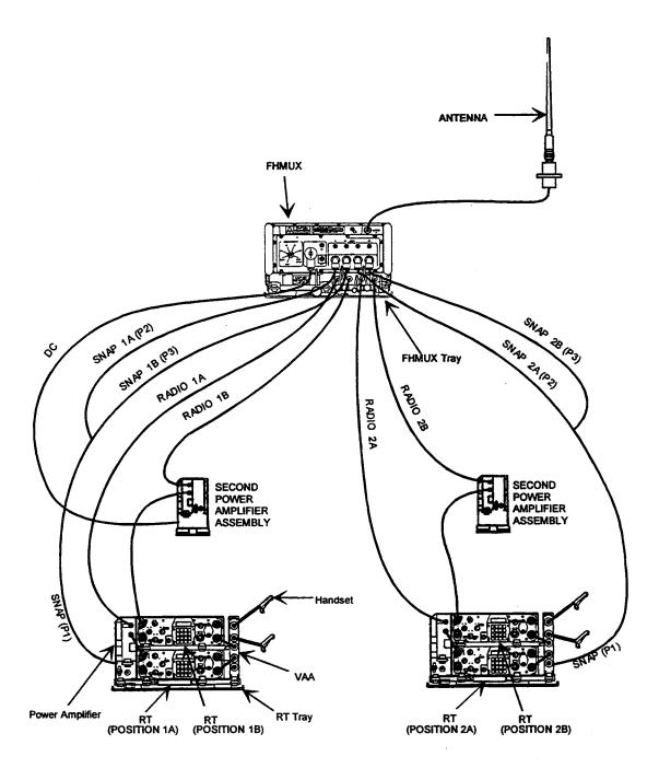
Figure 5-4. Cable Diagram: For TD-1456/VRC
