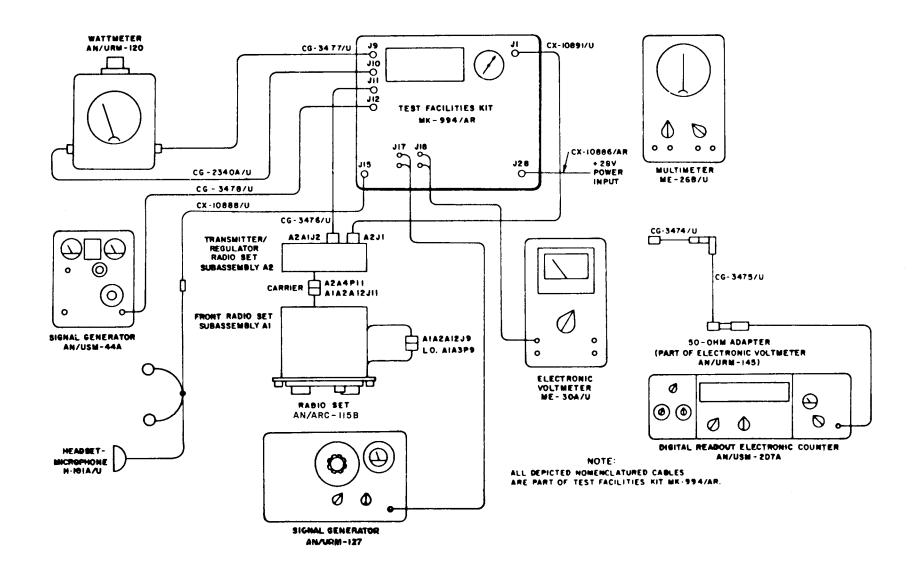
Figure 2. Radio Set Test Setup Diagram
