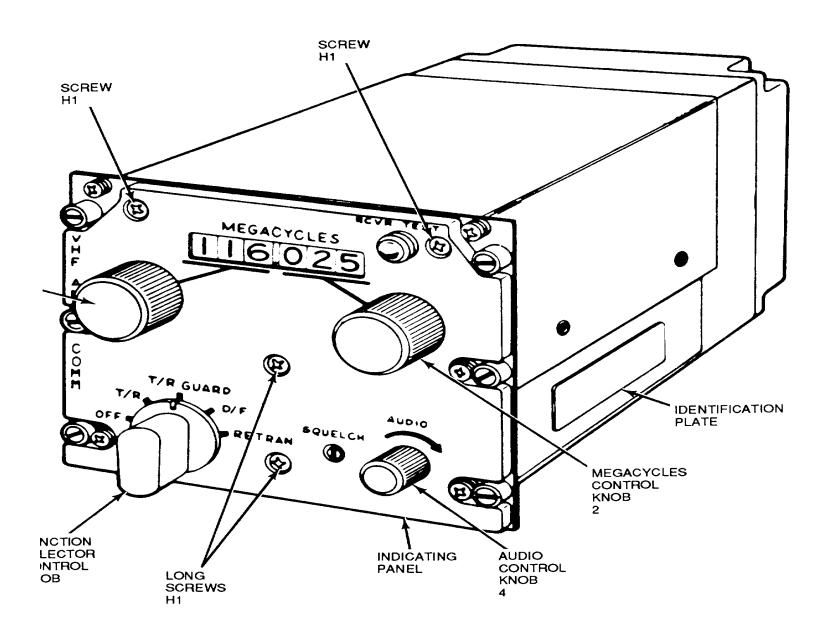
Figure 1. Location of Front Panel Controls and Attaching Hardware
