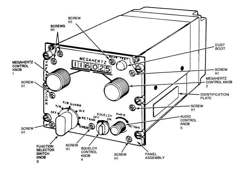
Figure 1. Location of Front Panel Controls and Attaching Hardware
