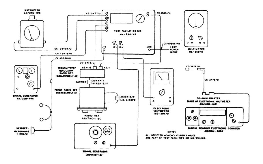
Figure 2. Radio Set Test Setup Diagram
